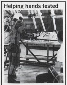
Mechanical hands could ease the task of astronauts clothed in bulky pressure suits or working in hostile space environments. Master-slave manipulators would enable the spacemen to repair spaceborne nuclear reactors, turn on tiny switches or even adjust dials. The experimenter above is performing a series of NASA tests with a pair of such manipulators at the Argonne National Laboratory.
