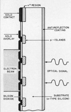
Main elements of Dactron's structure consists of p-type islands diffused into an n-type silicon substrate. The substrate is isolated from the scanning beam by a silicon dioxide coating. A gold overlay on each p-type island increases effective beam landing area of each diode.
