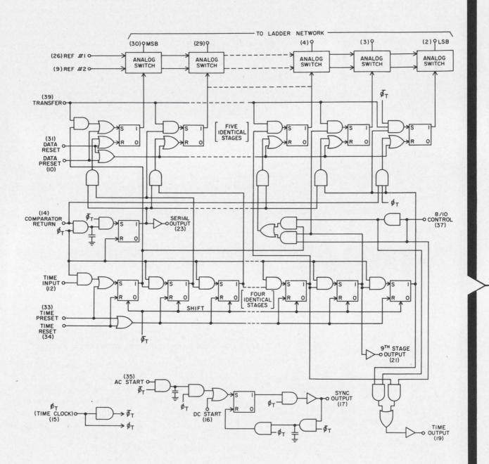
**Another ACTOS First**...This Monolithic A/D-D/A Converter incorporates General Instrument's exclusive MTOS (Metal-<u>Thick</u>-Oxide-Silicon) process which provides Large Scale Integration without the need for high-cost discretionary wiring.
