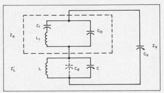
1. Equivalent circuit of an inductance-loaded crystal oscillator. The crystal has a capacitive impedance,  $Z_x$ . The parallel circuit of LC<sub>d</sub>C has the inductive impedance,  $Z_{L'}$ . The tuning capacitance,  $C_v$ , has a capacitive impedance,  $Z_y$ .  $C_d$  is the distributed capacitance of the coil.
