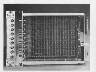
**Both these scalers use integrated circuits.** The 8-channel multiscaler (left) designed by LeCroy Research Systems Corp. operates to 500 MHz. Wires across the tops of the microcircuits are bus lines. The scaler at right with 7-digit Nixie readout is under development at Hamner Electronics. It includes an addressable register for computer compatibility.
