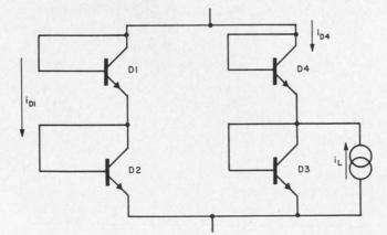
2. A diode quad of npn transistors on a single chip features very close current/voltage match between the transistors' base-emitter junctions.
