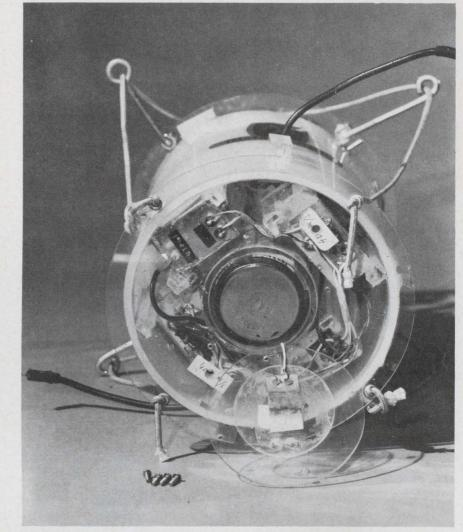
**Balloon-borne refractometer** measures radio propagation in the lower atmosphere. The unit contains two 400-MHz vhf transmitters, temperature and refraction sondes, and battery (Paper 3/1).
