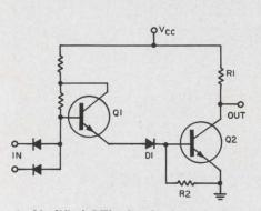
1. Modified DTL circuit. A critical input voltage swings the output high or low.
