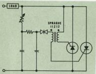
This breakdown-diode / transformer triggering circuit is a typical application for Type 11212 Trigate Pulse Transformers.
