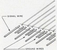
Signal wires are flanked by ground wires. This basic three-wire unit is repeated 20 times across the cable. ductor spacing for a required impedance and high propagation velocities. Attenuation losses are also held down since TFE's dissipation factor also is low (about 0.0002).
