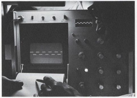
How do you combine the direct-write features of oscillographs with the high-frequency measuring capabilities of modern oscilloscopes? Simple, if you use the electron beam of a specially designed Sylvania fiber-optic CRT to provide immediately available direct printout recordings of high frequency analog data and video signals.
