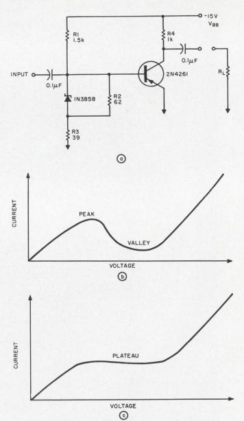
Nanosecond pulses are shaped with the circuit shown in (a). R2, approximately equal to the dynamic negative resistance of the diode, changes the familiar tunnel-diode IV-curve (b) to the one with a constant-current plateau (c).
