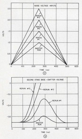
3. The spread of input pulses is applied to the circuit in four runs (one master and three succeeding runs) (a). Corresponding output plots of the base-emitter voltage for the second stage are shown in (b).
