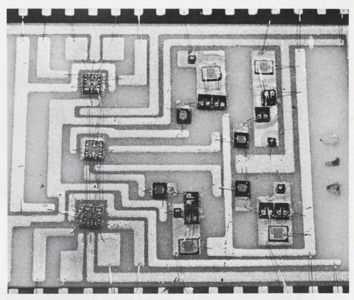
2. Transistors mix with integrated circuits in this 3/8-by-3/8-inch flat pack.
