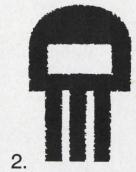
PET TO-5 is rated from 550 mW to 1.2 W at  $25^{\circ}$ C (chip dependent).
