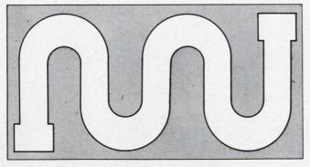
4. Heat spots won't occur at the bends, if the resistors have no sharp elbows and no constrictions. If the distance between the loops is equal to their width, include it in heat calculations.
