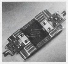
**Reciprocal latching phase shifter** from Syracuse University Research Corp. has digital and analog control of the insertion phase in S-band. The ferrite planar substrate is 20 mils thick (Paper 16/1).
