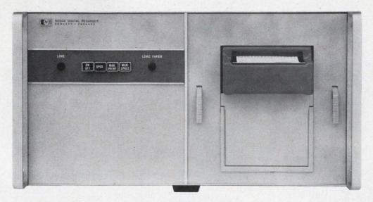
The HP 5050A Digital Recorder is no quitter. New mechanical techniques make this 20-lineper-second printer rugged, quiet, economical and simple. For example, there are no rotating electrical contacts for decoding, and no start-stop operation of printwheel and ink ribbon. Instead, photo-electric decoding is used, and the print drum rotates continually against an ink-impregnated roller. Fewer parts lead to
