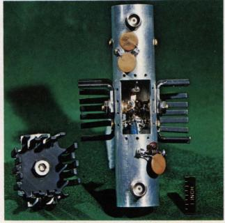
**Coaxial transistor amplifier** uses four overlay transistors in parallel. Developed at RCA's David Sarnoff Research Center, the amplifier has a saturated power output of about 90 watts at 370 MHz (Session 7).
