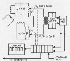
2. **Over-all diagram.** Up-down counter backtracks divider settings for correct angle.
