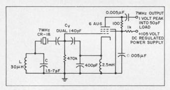
3. Typical oscillator circuit uses inductive loading. L is 34 turns of #18 tinned wire wound on a 2-inch-diameter ceramic form with a winding length of 3 inches. The output voltage is virtually independent of the position of  $C_v$ .
