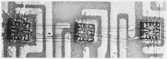
Hybrid circuits combining ICs and transistors can improve on circuits that use either type of
