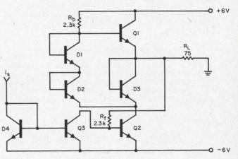
3. The complete all-npn Class-B stage built around the quad (D1, D2, D3, Q1) has very low idling current.
