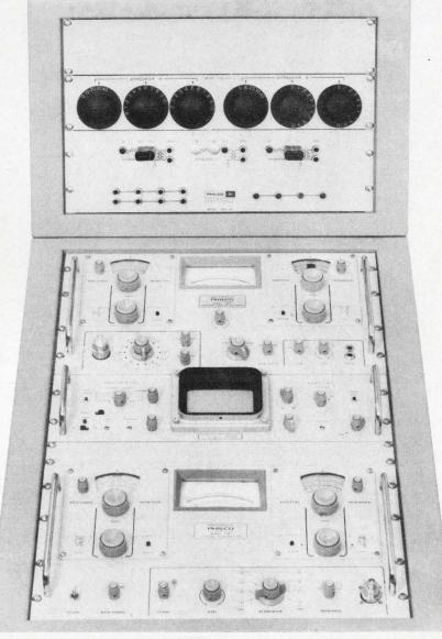
**Console contains complete transmission tester.** The set combines all the functions of a selective voltmeter, tracking generator, spectrum display, attenuator and impedance-matching panel in one. Page U178.
