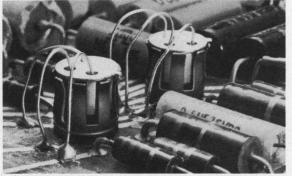
**Special insulating coating** – Insulube 448, a special non-hygroscopic finish developed by IERC, combines excellent dielectric properties, 50 K megs insulation resistance, and high heat emissivity. Also protects against salt spray, fungus, etc.
