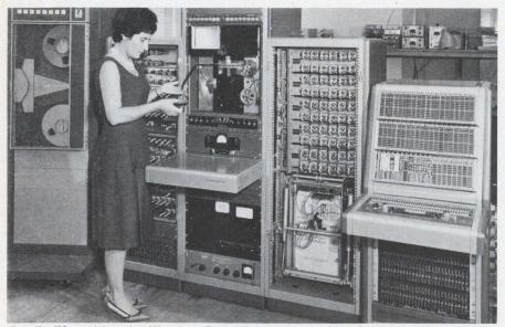
**Fosdic IV** enables the Weather Bureau to retrieve data from microfilm, shown being threaded onto a transport. The recorder is at left. Other racks contain logic, memory, scan control and film-advance circuitry.
