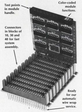
Laminated power bus bars installed and wired in each module case. Reduces noise, eliminates power inter-connections, cuts hours from assembly and test time. Indicator lights display system operation.
