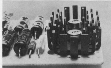
To cool off low-to-medium power transistors in TO-5 and TO-18 cases, use IERC's efficient LP's. Patented, staggered-finger design maximizes radiation and convection efficiency, radiates heat directly to ambient. Available in single or dual mounting for thermal mating of matched transistors.
