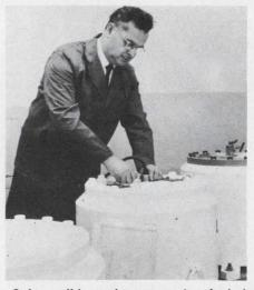
Submersible nuclear generator, fueled with strontium 90, produces 3 watts.
