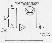
Transistor temperature transducer circuit eliminates the effects of recombination-generation current and surface leakages.
