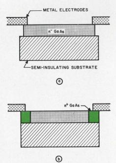
1. Fringing fields at the contacts of bulk oscillators, created by conventional mounting techniques (a), are eliminated by the deposition of  $n^+$  type GaAs (b) that serves as a base for the contacts.
