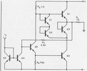
4. Even more efficient circuit than that of Fig. 3 can be made with only slight modifications. Its frequency response is flat from dc to well beyond 30 MHz; its propagation delay is less than 5 ns.
