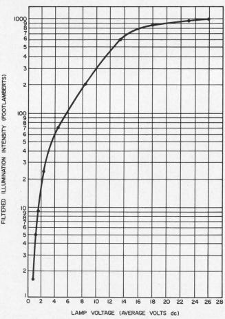
5. **Illumination intensity** as a function of average applied voltage combined with the curve of Fig. 4 narrows down the choice of the lamp.
