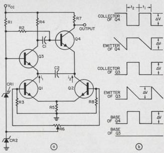
2. **Pulse generator** is controlled by Q1 and Q2 which, in turn, are controlled by the setting of R6 (a). Voltage waveshapes at various points within the circuit are shown in (b).
