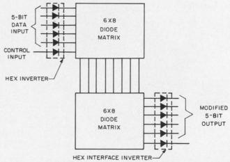
2. Use diode matrices and interface circuits to convert codes. A 5-bit data input is converted to a modified 5-bit output using the same 4 circuits as in Fig. 1.
