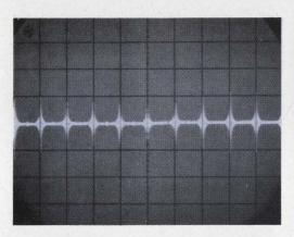
Oscillogram of a 10 to 110 MHz sweep with 10 MHz birdie markers added to show excellent sweep linearity. Specified 0.5% linearity and 1% frequency accuracy permit easy identification of intermediate sweep points, eliminating need for tedious pre-calibration.
