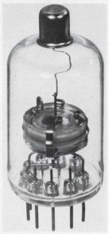
**Dynamic capacitor** housed in vacuum tube is part of electrometer that measures currents down to  $10^{-17}$  amps (Paper 59/4).
