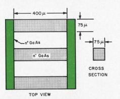
2. Schematic configuration of a GaAs oscillator shows dimensions for a unit that operates at 1 GHz in the LSA mode. Since in this mode the frequency does not depend on the length of the sample, it is shaped to obtain good heat transfer necessary for cw operation.
