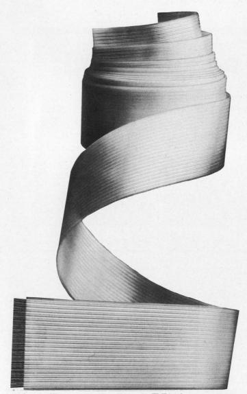
**Ribbon cable saves space.** Using Teflon TFE as the dielectric,  $95 \cdot \Omega$ , 20-signal transmission line can replace coaxial with a 90% space saving and easy assembly. Page U128.
