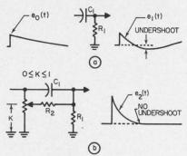
Fig. 1. Waveforms show results without pole-zero cancellation (a) and with it (b).
