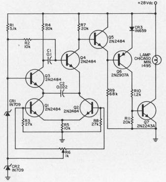
3. Addition of three transistors to the pulse generator of Fig. 2 completes the "lossless" lamp control circuit.
