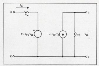
4. Though not as versatile as the Ebers-Moll equivalent, the low-frequency n-parameter model is often very useful because of its simplicity. Generally this type of model is not available in automatic transient programs because of the dependent sources. SCEPTRE, however, has provisions for accommodating this type of model.
