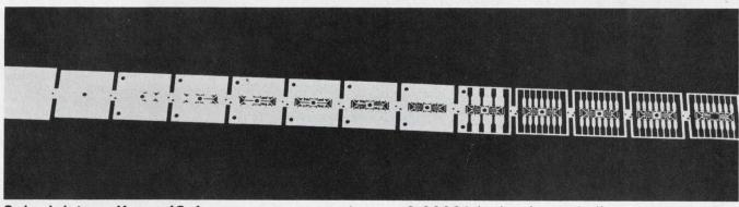
Subminiature Kovar IC frames are stamped by 13-stage progressive carbide dies. The
