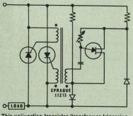
This unijunction-transistor/transformer triggering circuit is a typical application for Type 11Z13 Trigate Pulse Transformers.
