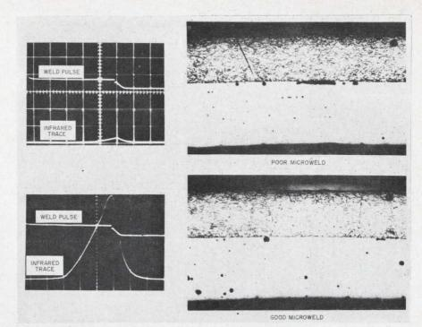
**Infrared detection** picks out bad welds that would be passed by qualified visual inspection (top). On the oscilloscope (top left) the feeble thermal response calls attention to the large void in the joint (top right). A large response with exponential decay (bottom left) characterizes good thermal conductivity through the joint. Note that the void disappeared (bottom right) from the welded joint. (Session 61).
