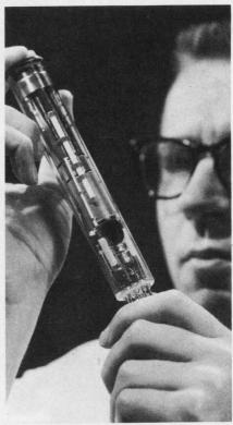
New television tube—called a Dactron—is held by M. H. Crowell of Bell Telephone Laboratories. It may be used in future models of the utility's Picturephone visual telephone.
