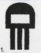
PET TO-18 is rated from 360 to 675 mW at 25°C (chip dependent).
