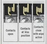
Here's how: As the contacts open and close with high tip open and close with high tip pressure, they provide a scrub-bing action that keeps the points clean—assures positive make and break for greater contact fidelity. Even after millions of operations. And under all kinds of operating conditions conditions.
