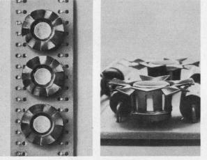
Fan-top dissipators for T0-5 and T0-18 cases drop temperatures dramatically; cost just pennies. T-shape adds almost nothing to board height; allows components to snuggle close to transistors. Spring fingers provide fast, press-on installation.
