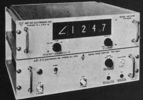
Type 524A3 with indicator. Computer alone (bottom panel) can produce analog output to drive recorder and d.c. digital voltmeter. Price \$999.
