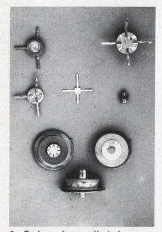
3. Package types affect frequency and power range. Both stud-mount stripline (upper right) and large coaxial packages (bottom) work up to about 2 GHz and dissipate about 5 watts. Small coaxial (right center), stripline (left) and pellet (center) types go up to and beyond 6 GHz and dissipate less than a watt.
