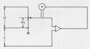
**Ratio of two voltages** can be read out directly by use of any of several commercially available recorders in the above configuration.
