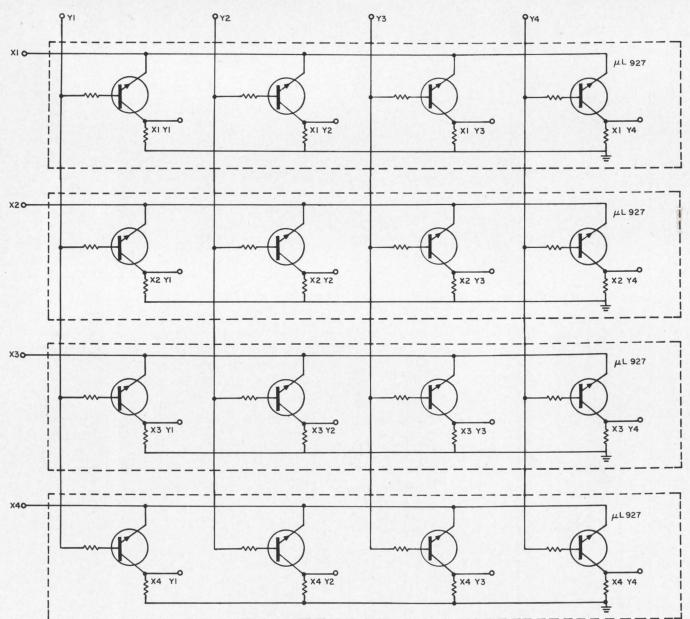
Integrated 16-bit matrix is built with four  $\mu\text{L927}$  packages. This compares with 32 diodes and 16 resistors
