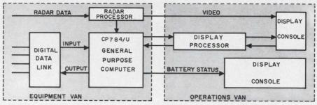
Missile Mentor block diagram, showing the data flow between the two vans that house the system.
