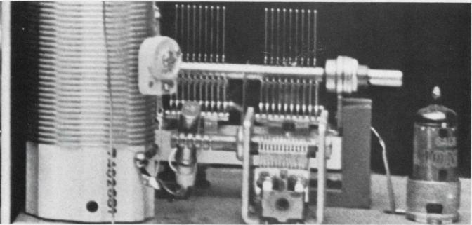
Inductor increases the bandwidth of crystals to 2 per cent—20 times that of conventional
