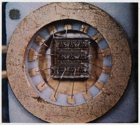
Nine-bit NDRO computer memory developed by RCA contains 90 silicon-onsapphire MOS field-effect transistors (Session 15/2).
