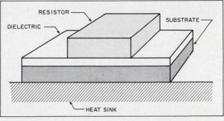
3. Calculate the thermal resistance between the resistor and the substrate to determine whether or not a particular configuration can handle the power that the circuit requires.
