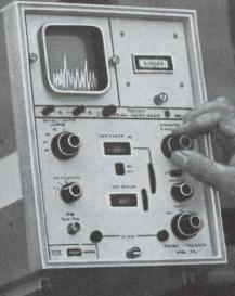
Battery- or line-powered Portable TA-2 analyzer main frame
