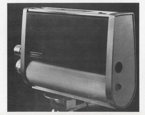
Hand-held vidicon camera sports optical viewfinder and fluted grip. A single cable carries input power, audio and video outputs and provides remote control of video tape.
