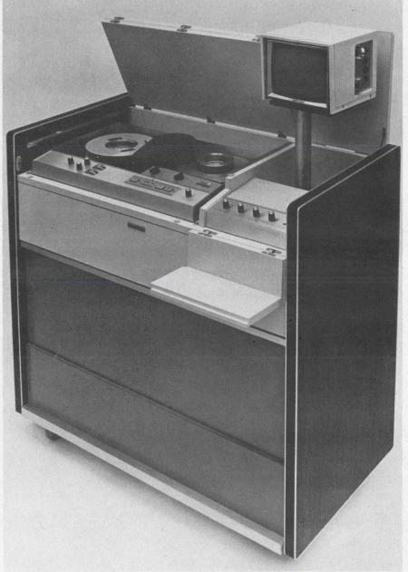
Videotrainer for school use contains video tapedeck, audio and video amplifiers, pop-up monitor and plenty of room for mikes, tripod, splicer and cables. Everything folds into a unit which can be secured with a single lock.
