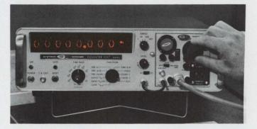
Tune transfer oscillator until a zero beat—any zero beat—appears on the built-in scope. The transfer oscillator is now phase-locked to the input.
