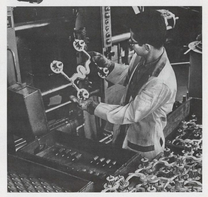
Rotors are so important to fractional horsepower motor running characteristics that we die cast our own. This is an example of how we maintain precise controls on the quality of our parts...to be sure of consistent and dependable operation of Bodine motors.
