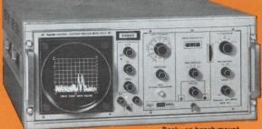
Rack- or bench-mount RTA-5 Analyzer main frame
