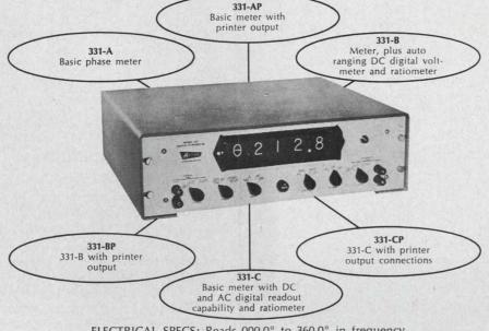
ELECTRICAL SPECS: Reads 000.0° to 360.0° in frequency range from 30Hz to 500KHz; accurate to  $\pm 0.5^{\circ}$  200Hz to 35KHz; Reads DC (when provided) 0.001-600 volts, and AC (when provided) 0.1-300 volts.
