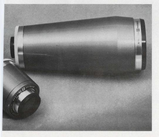
Spatial filter and lens family uses "parent" filter housing to accommodate all other elements. Positioning stages remain with housing and are controlled by radial knobs (x and Y) and coax ring (z).
