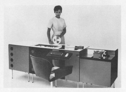
Data station transmits 8-bit ASCII at 120 characters/second. Design modularity allows system flexibility. Input/output capabilities include paper tape, punched cards, printer and keyboard-teleprinter units and an optical scanning input device.
