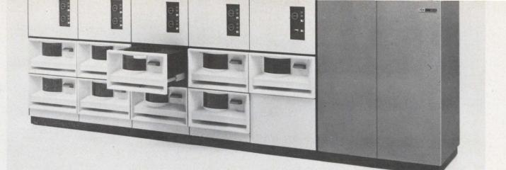
**Direct access storage facility.** Each section slides out providing easy access for removal of its magnet drum.
