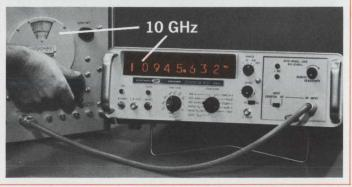
When you change the input frequency, the reading changes right along with it. All automatically. No operating adjustments whatever. That's why we call our plug-in "ACTO" for "Automatic Computing Transfer Oscillator." It enables people with very little technical skill to make precise measurements rapidly and without mistakes.
