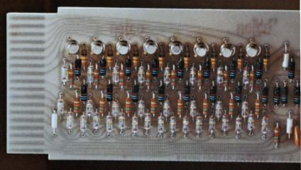
FLIP CHIP T.M. Modules—The Digital Equipment Corporation trademark for a new kind of digital system module uses Allen-Bradley hot molded resistors exclusively.
