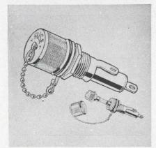
A high-voltage, low-current transformer is specifically designed for photomultiplier applications. The transformer is potted with a corona-resistant silicone compound in a diallyl phthalate case. The unit will operate in temperatures up to  $130^{\circ}$ C at altitudes up to 200,000 ft.
