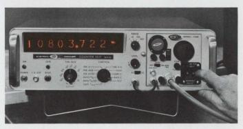
2. Adjust harmonic preset until the reading appears. Notice the counter reads "10,803.722 Mc," an actual microwave frequency presented with counter accuracy.
