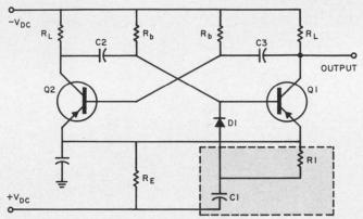
**Differentiating network** consisting of R1-C1 provides astable multivibrator with a self-starting capability.
