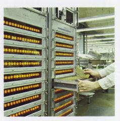
Decade counting assemblies for all solid-state counters undergo a temperature of 80° C for 2 hours to force failure of any marginal components. Despite this torture, the failure rate of decades is less than 0.5%. The assemblies are also operated for 22 hours at room temperature.
