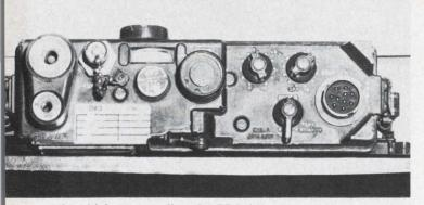
An old Army standby, the PRC-10, was pulled off the shelf for Vietnam duty. It is an FM voice set operating at 38 to 54.9 MHz. Weight is 26 pounds with batteries. Designed for jungle use, it puts out about a watt.
