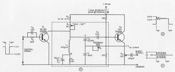
**Burst oscillator** is simple, stable and synchronous. Here (a) the tank circuit is "kicked on" to produce the oscillation, instead of interrupting the current flow through the inductor. Shifts in the reference level and noise appearing between bursts do not occur. If the feedback control  $R_2$
