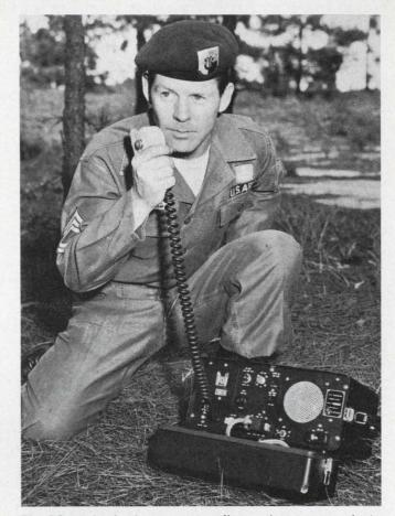
The TR-20 is the base-camp radio used to communicate with the HT-1s carried by Montagnards on patrol. It puts out 20 watts at 30 to 40 MHz and weighs 20 pounds. Sgt. Chambers demonstrates operation.
