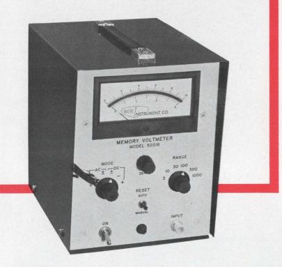
The Model 5201 memory voltmeter is a dc to 20 mc instrument which measures and stores indefinitely the maximum peak voltage applied, including continuous or one shot pulses as short as 50 nanoseconds. A memory reset-switch on the front panel allows the 5201 to monitor peak values of a varying waveform, either positive or negative going.
