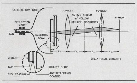
1. Beam direction in the scanlaser is selected by the CRT electron beam. The lenses enable the cavity to support many different modes with equal gain.
