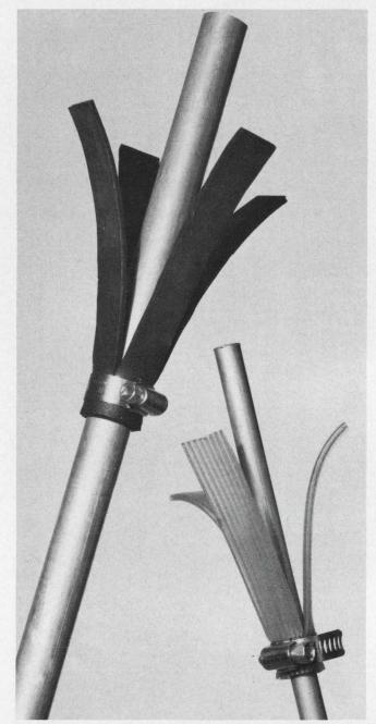
Flat rubber sheets protect antenna elements by absorbing and dissipating mechanical energy due to wind.
