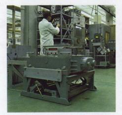
Here's a small part of hp's extensive in-house test facility where instruments are tested under extreme shock, vibration, temperature, humidity and electromagnetic conditions.
