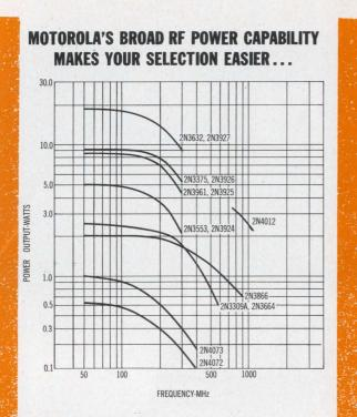
The power-frequency curves indicated here, cover only the EIA-registered device numbers available within Motorola's broad RF Power Transistor line. They are intended to help you narrow the range of possible choices for your specific application.
