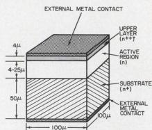
Sandwich Gunn-effect oscillator devices are grown epitaxially from gallium arsenide of varying resistivity to different thicknesses. Bell Laboratory scientists report improved cw power over a wide frequency range. Resistivity in the active n region is  $0.3 \Omega/cm$ ; in the n<sup>+</sup> region,  $0.001 \Omega/cm$ ; and in the n<sup>++</sup> region,  $0.0001 \Omega/cm$ .
