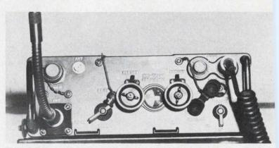
**The PRC-25**, a transistorized set, is replacing the PRC-10. It covers a wider range (30 to 75.95 MHz) at higher power (1.5 to 2 watts). Weight is 24.7 pounds. Its lower power drain means longer battery life.
