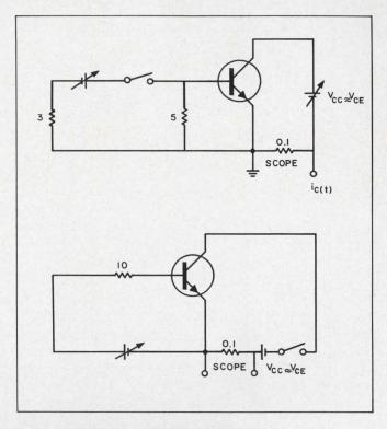
6. **Test circuits** for establishing Soar regions B, C and D (see Fig. 5) for the pulse operation of power devices are exhibited. Shown are the networks for pulsed base-drive (top) and pulsed collector-supply (bottom) modes.
