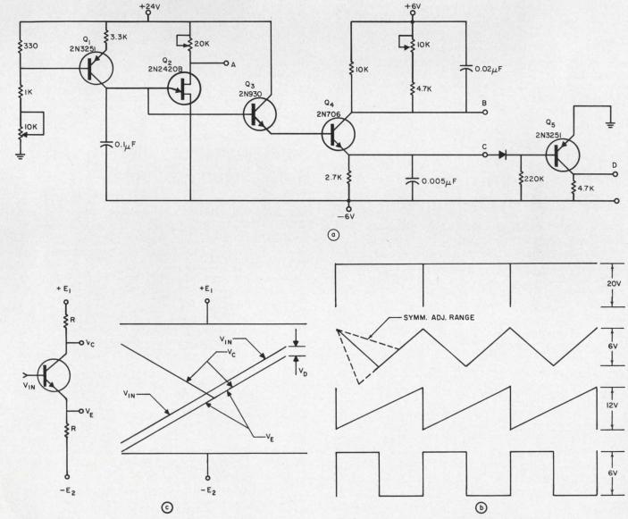
**UJT** and four bipolar stages are used in a compact multiwaveform generator (a). Circuit produces (b) pulse train, triangular wave, sawtooth and square wave. Npn stage  $Q_4$  (c) functioning as "signal bender" is mainly responsible for over-all simplicity and compactness. Stage  $Q_5$  may be omitted if a square-wave is not desired.
