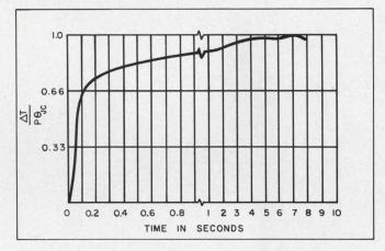
7. Normalized junction temperature response vs time plot is used to make safe-operating-area calculations for pulse widths in excess of 1.0 ms. Here  $\Theta_{\rm JC}$  refers to the thermal resistance, junction-to-case.
