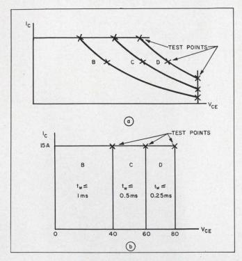
5. Safe operating area is a function of pulse width. The  $I_{\rm C}-V_{\rm OE}$  curve is broken into three distinct regions (B, C and D), each bounded by a hyperbola (a). When a specific transistor type is involved (b), straight-line approximations may be used to save test procedure down time.
