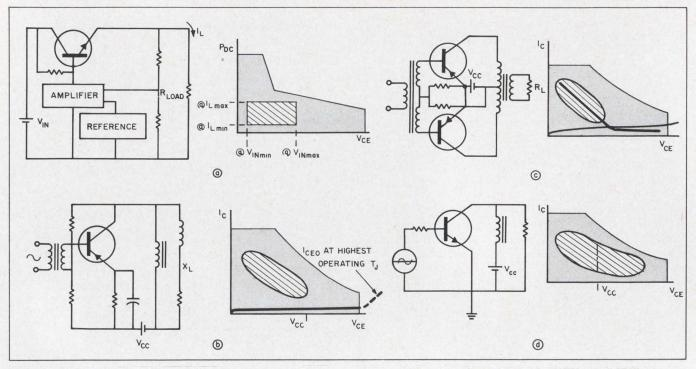
3. Safe operating area (Soar) for power transistor applications is designated by the crosshatched portions on the  $I_{\rm C}-V_{\rm OE}$  characteristic. Shown are a series dc regulator (a), a Class-A amplifier (b), a Class-B amplifier (c) and an
