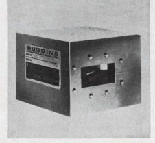
The MA-8319-1C3 switch is used for hot-standby operation in which two RF transmitters, tuned to the same frequency, are switched into a single transmit antenna. When one fails, operation is switched to the standby transmitter. The unit can switch up to 7 W cw in 500 ns. Bias power is 1/4 W and isolation is 90 dB. Insertion loss is 1 dB and vswr is 1.15 in the 6.5- to 7.2-GHz frequency range.
