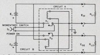
2. Equivalent circuit representation of regulator uses relays in place of the transistor elements. The interconnections here demonstrate the switching, regulating and feedback functions. Relay  $K_1$  represents  $Q_1$  and  $K_2$  is the  $Q_2$  element. Loads  $R_{L1}$  and  $R_{L2}$  depict the oscillator and dc-to-dc converter respectively (see Fig. 1).
