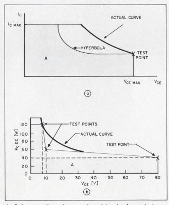
1. Safe operation of power transistor in dc mode is established by hyperbola relating  $I_{\rm C}$  to  $V_{\rm CE}$  (a). As  $V_{\rm CE}$  increases, the device's dissipation capability diminishes, and a derating curve must be used (b).
