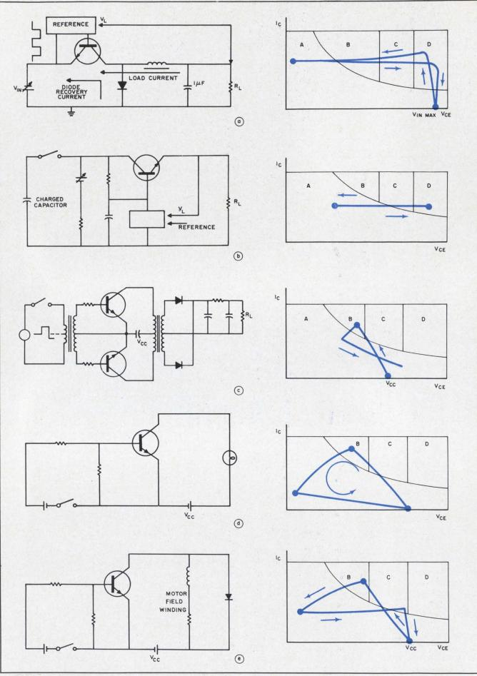
ing regulator (a), a series regulator, transient case (b), a capacitive load, inverter turn-on (c), an incandescent load turn-on (d) and a motor start-up circuit (e).
