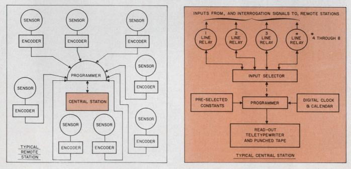
1. Typical air-quality monitoring system of the type recently installed in Chicago by Datex Corp. consists of eight remote data collection stations. Each station automatically measures air pollution content and meteorological data, digitizes the information and transmits it to a central computer station by means of telephone or teletype lines.
