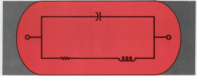
**'Kick on' the tank circuit** for synchronouskeyed burst oscillation instead of interrupting
