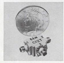
For use from 9.1 to 9.5 GHz in an ambient temperature range of -55 to 80°C, this X-band plug-in isolator has a vswr of 1.15 max. The J-7881 has an isolation of 40 to 50 dB and an insertion loss of 0.3 to 0.4 dB. A 4-port device with two internal terminations, the unit has a design compatible with strip-line assemblies. It is 1 X 0.75 X 0.625 in. and weighs 1 oz.
