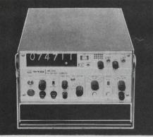
Greater portability Compact— 12.0" wide × 6.0" high × 14.6" deep Lightweight—24.5 lbs Durable Power—DC 12/24V and AC 115 V Withstands use under rugged conditions Low power consumption—34W Built-in power line noise filter Built-in wWV receiver—5/10MHz High input sensitivity—50mV rms/min High degree of measuring accuracy available instantly. No waiting for crystal oscillator oven temperature to build up. Specifications:
