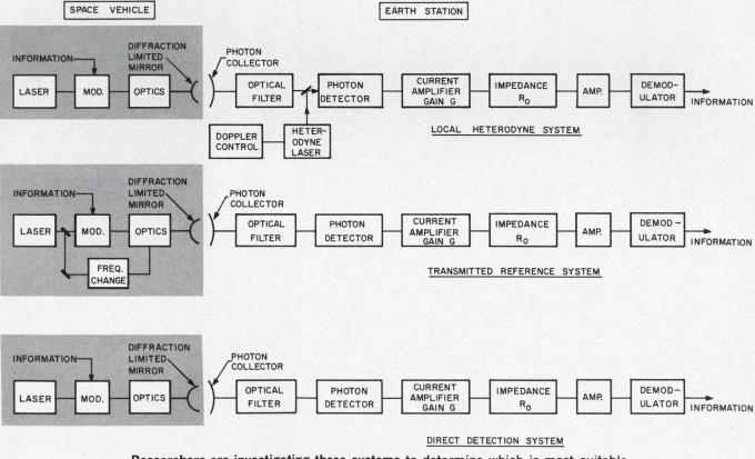
**Researchers are investigating these systems** to determine which is most suitable for deep-space video data communication. The direct detection system presently appears most promising.
