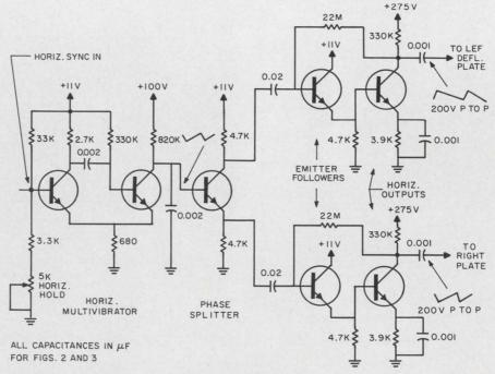
3. Horizontal deflection for electrostatic deflection is obtained from an emittercoupled multivibrator feeding phase shifters which drive push-pull amplifiers.
