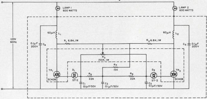
Triac power-controller establishes a tandem dimmer. Potentiometer R<sub>3</sub> determines relative lamp brightness.
