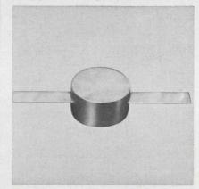
Capacitors for microwave stripline use are offered in a range from 10 to 1000 pF. Available for 1/4- or 1/8-in. ground plane spacing, the devices are rated at 0.5 W dissipation at 25°C and have a maximum voltage of 100 V. They have ribbon leads spaced midway between the ground planes. All contact areas are gold-plated.
