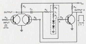
Temperature stability better than  $\pm 0.5\%$ , from -10 to +70°C, is achieved in this standard IC multivibrator by addition of resistors  $R_1$ ,  $R_2$  and the two diodes shown.
