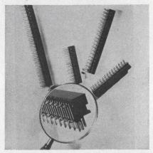
Strip mounted connectors with 3 to 51 contacts snap into PC boards without staking. The "split leg" design connectors feature one leg per contact. Contacts are retained in the strip by formed tabs extending through the upper surface. Contacts are gold plated phosphor bronze mounted on 0.1-in. staggered centers and are available with upper or lower rows only on 0.2-in. centers.
