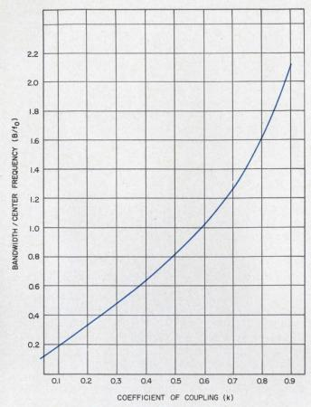
4. The coefficient of coupling (interstage) is affixed by the bandwidth to center frequency ratio.
