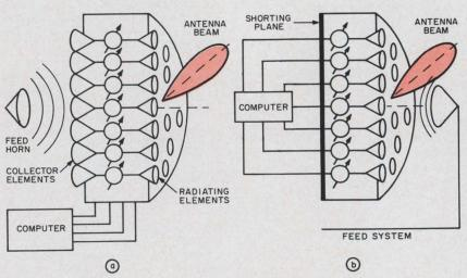
3. Optical feed systems. A lens array is shown in (a) and a reflector array is depicted in (b). These arrays eliminate need for power-distribution networks. Array phase shifters are computer controlled.
