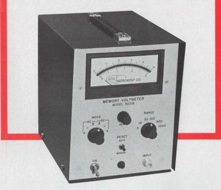
The Model 5201 memory voltmeter is a dc to 20 mc instrument which measures and stores indefinitely the maximum peak voltage applied, including continuous or one shot pulses as short as 50 nanoseconds. A memory reset-switch on the front panel allows the 5201 to monitor peak values of a varying waveform, either positive or negative going.
