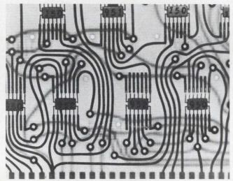
**Up-down counter** includes four flip-flops, preset and reset inputs and all gating. Page 96.
