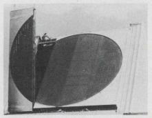
HAPDAR phased-array radar shown during final assembly. Its 30-ft. dia. planar lens, illuminated by a single power tube, has successfully tracked reentry vehicles.
