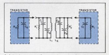
Interstage connections must account for all stray and shunt values of resistance and capacitance. Their influence must be accommodated by the RC products fixed by resonance.
