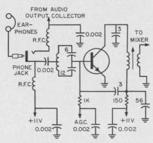
2. The earphone lead serves as the antenna in the tiny set. RF chokes prevent RF grounding.
