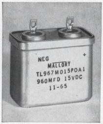
The TL offers the superior performance which is characteristic of Mallory wet slug capacitors. It has exceptional stability of capacitance and power factor, both over a broad temperature range from  $-55^{\circ}$ C to  $+125^{\circ}$ C, and throughout extended operating life and shelf tests. DC leakage is low; maximum values at top mfd-volt ratings are in the order of 10 microamps, with actual test values typically around 1 to 2 microamps.
