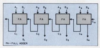
2. Carries ripple through the full-adder stages of this 4-bit ripple-carry adder. Eliminating the stage-by-stage ripple increases the adder's speed of operation. Ripple time limits the speed of this adder.
