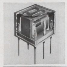
A 1/4-in.<sup>3</sup> MIL-spec transformer features a laminated core. At 1 kHz, insertion loss is less than 3 dB. Frequency range is 400 Hz to 250 kHz and droop is 5%, overshoot is 10%, and rise time is 100 ns for square wave operation. Power rating is 1 W max. Turns ratios to 100:1 are available.
