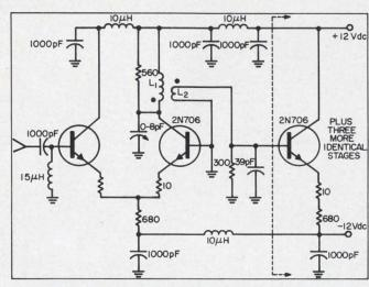
Complete IF strip consists of four stages, has over-all gain of 30 dB over a bandwidth of 30 MHz and a center frequency of 45 MHz.
