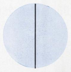
0.000069" rolled metal magnified 500 times.
