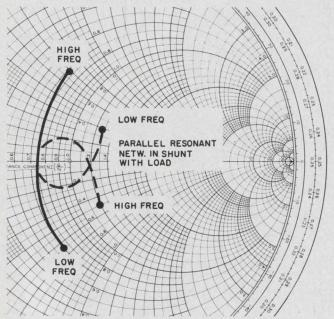
2. Parallel resonant circuit, in shunt with the load, wraps certain impedances into a smaller circle, and thus improves the match.
