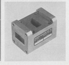
This iridited aluminum X-band waveguide E-plane tee is readily adapted as a holder for oscillating, limiting, and spst and spdt switching microwave diodes. Frequency range is 8.2 to 12.4 GHz. Model X160 has 3 cover-type flanges with 8-32 tapped holes that mate with UG-39/U waveguide.
