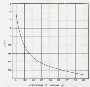
5. The RC component values are established by the loaded-Q figure. The relationship between the coefficient of coupling and  $Q_{\rm L}$  sets the RC product of each stage.
