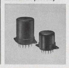
A 50% size reduction over conventional 6 pdt relays is represented by this 2.2-oz, 1-in. high, 1-in. diameter relay. It is designed for drycircuit to 2-A applications. Coil resistance is 200  $\Omega$  at 25°C and initial contact resistance is 0.05  $\Omega$  max. Pull-in voltage is 14 Vdc max and drop-out voltage is 2 Vdc min. Operate and release times are 10 ms max at 26.5 Vdc. Insulation resistance is 1  $\Omega$  min.
