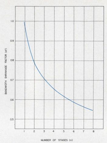
3. Bandwidth shrinkage factor is determined by using this plot of shrinkage vs number of stages.
