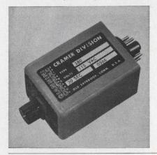
Four standard time ranges and 2 levels of accuracy are offered by this time delay relay. Available as a plug-in or a panel-mount, it has standard delays of 15, 30, 60, or 120 s. Standard accuracy is  $\pm 10\%$  with repeat accuracy of  $\pm 5\%$ . Reset time is 30 ms and lifetime is claimed to be  $10^7$  operations.
