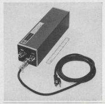
A low-noise, single-reversal, permanent magnet traveling-wave tube amplifier is designed for the 8 to 12 GHz band. Specifications include a 9-dB maximum noise figure, a 25-dB minimum small signal gain and 13-dBm minimum power output. Input and output vswr are 2 max. Primary voltage is 115 ±3 Vac.
