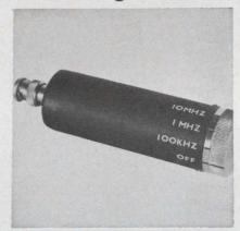
A new pocket-sized self-contained time mark generator is for use as a calibrator or frequency standard. Three preselected frequencies (100 kHz, 1 MHz, and 10 MHz) having a tolerance of  $\pm 0.005\%$ , or an optional  $\pm 0.0025\%$ , are standard. A standard BNC interface for direct plug-in and internal battery power source are featured.
