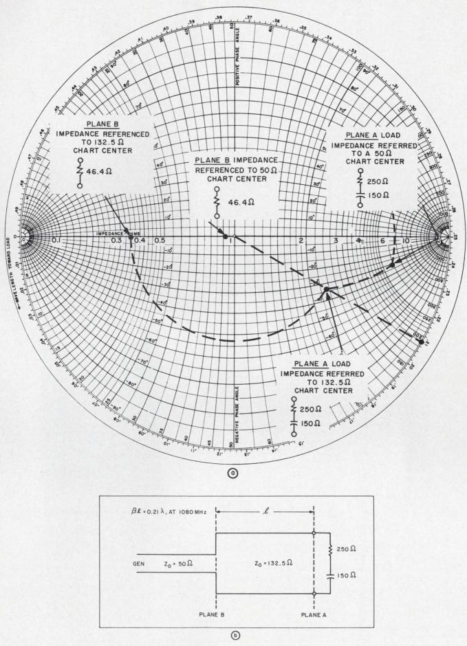
4.  $Z_{\Theta}$  chart, combined with the Smith Chart, is helpful in the design of in-line transformers to match impedances
