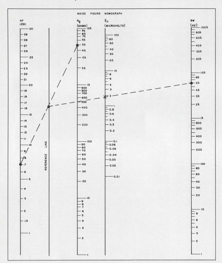
Here is a nomograph that permits designers to find out quickly the equivalent noise voltage at the input to an ampliner.
