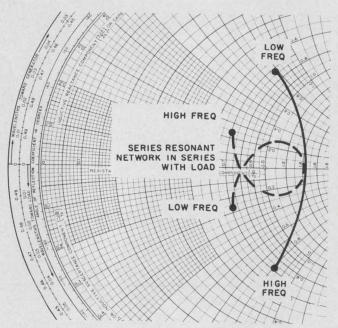
Series resonant circuit, in series with the load, improves the match for impedances represented by the solid line.
