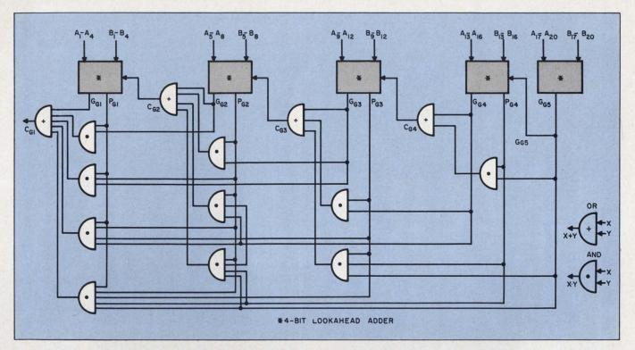
4. Carry-look ahead techniques are especially useful in large capacity adders. The circuit shown here illustrates
