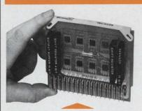
MICROSYSTEM® is a new, simplified method of interconnecting flat pack integrated circuits in "sticks," each containing as many as 10 I.C. flat packs with standard, multilayer, interconnecting matrices.
