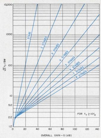
2. To determine the number of stages needed in an IF amplifier strip, the gain-bandwidth relationship must be considered. The ordinate here uses the ratio of gain-bandwidth cut-off to over-all bandwidth, and the abscissa is over-all gain.
