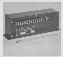
Seven transistors and one thermistor give this audio amplifier frequency response of  $\pm 1$  dB, 20 to 20,000 Hz, and a harmonic distortion less than 1%. Gain exceeds 80 dB. A shielded input transformer permits use with 50- to 150- $\Omega$  microphones. Transformer output has an 8- $\Omega$  and a 500- $\Omega$  winding capable of delivering 200 MW. The unit draws approximately 100 mA.
