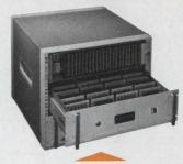
Complete hardware for EECoLogic consists of: swing-out card files, card drawers, power supplies and all necessary accessories.
