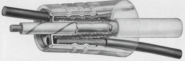
Uniring combines inner and outer ferrules in unitized construction. Simply insert a stripped conductor and tap wire, then crimp. One crimp does it. No heat. No burnt cables. Result: A vibration-resistant, noise-free connection that is mechanically and electrically stable. A uniform connection that takes virtually no time to make.
