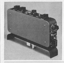
The NF1 amplifier is a wideband, direct coupled electrometer with neutralizable input capacity. It has  $10^{11}~\Omega$  input resistance, input leakage current of  $10^{-12}~\mathrm{A}$  and a gain of 3. Frequency response extends from dc to over 1 MHz. A six-position, low-pass filter selects cutoff frequencies of 300 Hz, 1, 3, 10, 30 kHz, and maximum bandwidth.
