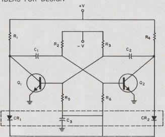
Diodes and capacitor provide astable multivibrator with a guaranteed self-starting capability.
