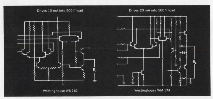
You can drive sizable inductive, capacitive, or resistive loads directly with either of these two IC op amps. They're unmatched for "muscle". Using them, you can omit an intermediate driver stage or power amplifier in many applications.
