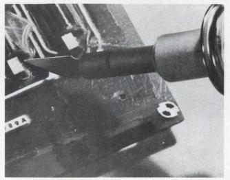
Low-cost iron simultaneously cuts and heat seals PC board epoxy encapsulants. Page 90.
