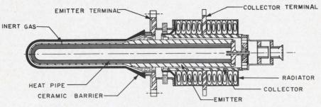
1. This thermionic-converter design uses a molybdenum-alloy heat pipe to concentrate heat from the flame-heated burner to the converter emitter. Thirty-six of these diodes, built by RCA, will be combined to develop a 3-kW generator for Army field use.
