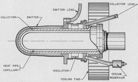
2. In this thermionic converter, a heat pipe conveys the heat rejected by the collector to external cooling fins. Designed by Thermo Electron Engineering Co., the device will del.iver 100 watts when the hemispherical end is placed in a 1400°C flame-heated burner.
