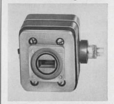
A positively-pulsed, 1 kW, Kuband tunable beacon magnetron tunes over the 16 to 16.5 GHz range with a 0.5- $\mu s$  pulse width and a 0.001 duty ratio. Peak anode voltage is 3 kV and peak anode current is 1.6 A. Input connections are made through flexible leads or solder lugs and the output connector mates with a UG-541/-U choke flange.
