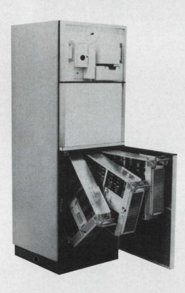
Shown:  $1\frac{1}{2}$  million bits (98K words) of core memory. Standard  $5\frac{1}{4}$ " ICM-40 mounts vertically in standard 19" x 24" cabinet. Memory module swings out, tilts for easy access to module side or wired side of hardware.
