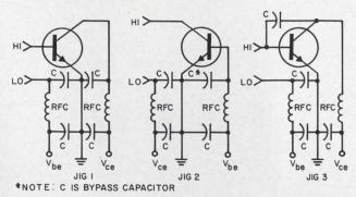
For each of the above measurements the Boonton  $R_x$  meter, Model 250-A, is first nulled at the desired frequency, and the appropriate jig is then placed across its terminals.  $V_{ce}$  is adjusted to the desired
