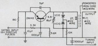
Oscillator uses back-to-back Varicaps to provide electronic tuning capability. This circuit produces a selected signal that is 40 dB above adjacent harmonics.
