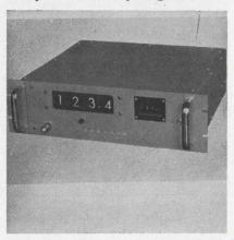
A solid-state, elapsed time digital programer programs contact closures. The unit can start or stop a test at selected times by thumb-wheel coding switches mounted on the front panel. Minimum resolutions are 0.1 s with a 60 Hz time base. The unit is available in ranges of up to six decades of time information.
