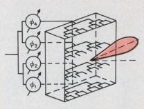
2. **Pencil beam** obtained with planar array is provided by vertical and horizontal feeds.
