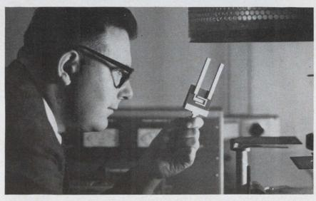
M. P. Lepselter examines beam-lead model (enlarged about 300 times). Beams were thermally aged in 360° C steam for 1000 hours, centrifuged to 130,000 G, bent 90° twenty times without failure. Beams can be tapered for smooth impedance matching, widened to act as heat sinks.
