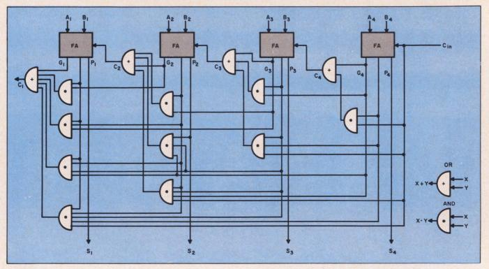
This 4-bit adder uses the auxiliary functions generate
