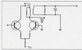
1. Simplified wideband, double-tuned amplifier uses a common-collector, common-base combination. This mode yields a resistive-capacitive input and a flat gain response.
