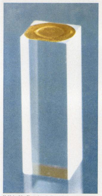
**Multiple thin films** deposited on single-crystal sapphire rod function as efficient acoustic transducers at micro-wave frequencies. (paper 37.1)
