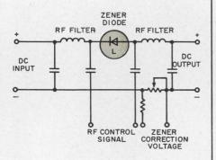
is applied to the dc blocking capacitors across the zener diode, its impedance drops to a very low value and therefore permits essentially full direct-current flow from the dc input to output terminals.
