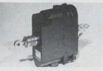
A thrust-vector actuator can gimbal velocity control engines.
