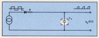
13. Integrator network is formed by resistor R and the transducer in this circuit.
