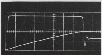
7. Step-up display performance: Coil voltage and coil current data taken from a single-ended deflection amplifier show good agreement with calculated values. For  $E_e = 18$  volts,  $L = 25 \mu$ h,  $R_L = 0.5$  ohms and  $T_c = 50$  ns, the system exhibited a settling time of 17.0  $\mu$ s. One vertical centimeter represents 5 units (volts and amps) and each horizontal centimeter 2  $\mu$ s. Voltage is displayed as a step function and current as a ramp.
