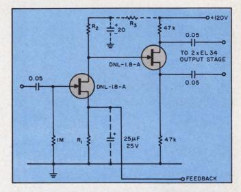
5. To obtain higher output levels in audio stages, a FET source-coupled phase inverter may be put to work. However, the balance here is not sharp, unless the generator source impedance is 100 kohms or more.
