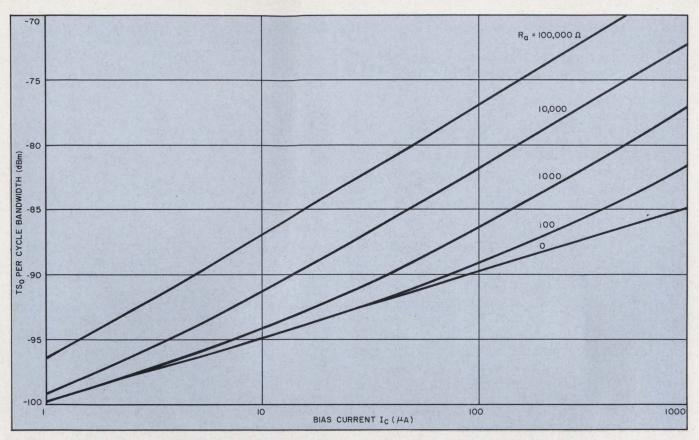
8. The dc tangential sensitivity,  $TS_o$ , decreases with increasing bias current and with increasing  $R_a$ .  $R_a$  is the
