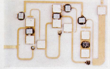
Early breadboard of power amplifier for Texas Instruments phased-array radar had as its aim 2 watts of pulse power at 2.25 GHz (paper 45.1).
