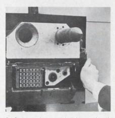
5. Car coupler contains large electrical connector. Dixie Howell presses plate to removê shield.
