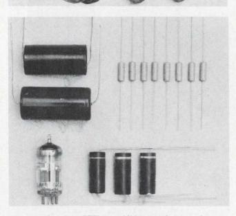
**Reap another beneFET!** In addition to the superior performance FETs offer in audio equipment, they require (top) less in the way of associated components and size than bipolar (middle) and tube (bottom) counterparts.
