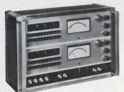
on the electronically-balanced meters. Setting up the first one or two digits of this reading on push-button decade controls makes the balancing automatic; the meters can read the first, second, third or fourth digits. The Bridge produces analog voltage propor-tional to the meter readings and BCD (in a 1248
