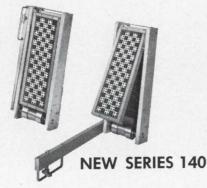
MAC Panel's Series 140 Plugboard Programming Systems are available in a wide range of sizes ... each designed and engineered to withstand the severest shock and vibration under operating conditions. Tested to 50G without self-generated contact noise. And life tested to 10,000 cycles with only random variation in contact voltage drop.
