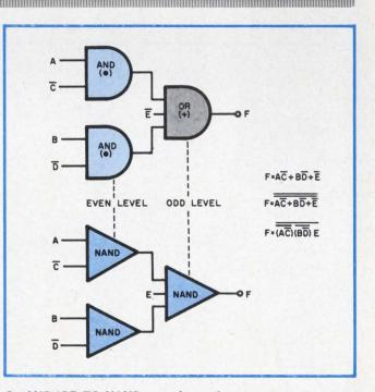
2. AND/OR TO NAND transformation results in the complementing of all variables that are present at odd levels. Variables at even levels are not.
