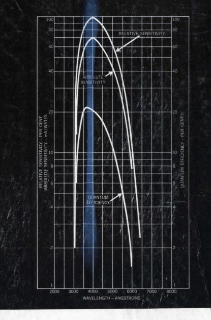
The Bialkali Photocathode is now available in many new RCA tube designs as well as in variants of most of RCA's commercially known photomultipliers. This new photocathode provides advantages in higher quantum efficiency and lower dark current. Designed for scintillation counting and other low-light-level detection and measurement systems, units with the RCA Bialkali cathode offer
