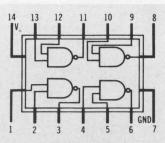
SN15946/SN15846 Quadruple 2-input NAND Gate
