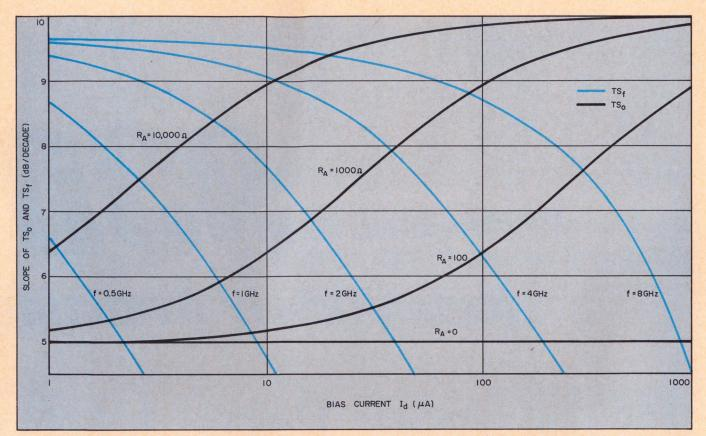
11. **Optimum bias current** for a specified frequency, f, and noise resistance,  $R_a$ , may be found from the intersection of these two sets of curves. The curves indicate the
