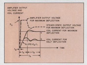
6. **Overdriven stages aren't faster!** The plot of output vs time for various overdrive conditions shows that settling time  $t_s$  remains fairly constant. Since overdriving does not speed up the settling time, it is not a recommend operating mode. Moreover, greater power is called for.
