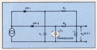
12. **Dc output voltage** that is a linear function of transducer capacitance is produced by this rectifier-type circuit. Either one or both of the capacitors may be a transducer.
