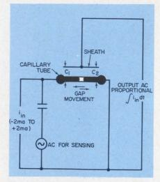
$C_1$  and  $C_2$  are differentially proportional to the position of the electrolytic gap, thus proportional to the time integral of the input amplitude.
