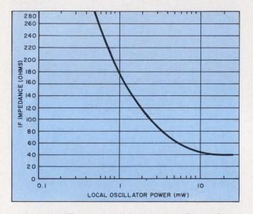
6. At typical IF (30 to 60 MHz) the impedance of hotcarrier diodes is a pure impedance and depends only on the level of the local oscillator drive signal. For -hpa-2350 diodes the impedance is around 180 ohms at the optimum local-oscillator level of 1 mW. In the case of balanced mixers the combined impedance is about 90 ohms, eliminating the need for extra matching circuits for IF amplifiers.
