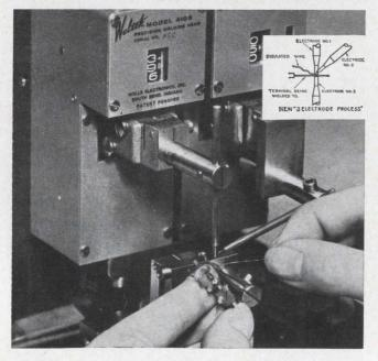
Get rid of costly wire stripping operations... ask about our new AC-10/410-E system. It welds through insulated wire (up to .010' dia.) in less than 1/3 second. Send samples. **Precision Welders** by WELLS ELECTRONICS, INC. 1701 S. Main Street, South Bend, Indiana, U.S.A. ON READER-SERVICE CARD CIRCLE 840
