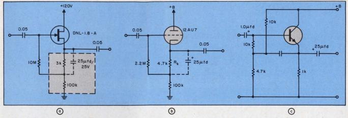
1. The FET source-follower stage is a basic audio circuit (a). It exhibits high input impedance and low output impedance because of the negative feedback employed in the source. Use of the FET yields higher gain and lower,
