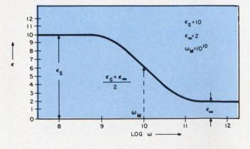
1. Dielectric constant decreases with increasing electricfield frequencies of about  $10^9$  Hz and higher. This is shown for a low-density material.
