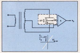
11. **Output current** in this ratio-type arrangement is proportional to the displacement of the common electrode of the transducer.
