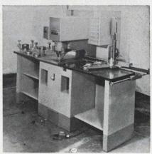
Using ultrasonics, this new model WU-100 wire bonder welds a wide range of power transistors such as TO-3's, TO-66's, stud packs and other large devices. It bonds wire from 5 to 40 mils.
