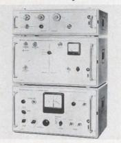
Diodes, rectifiers, transistors, and FETs are checked by model 259 in- or out-of-circuit. It measures both transistors and diodes, in-circuit, for reverse leakage down to 500 ohms of loading. It also measures FETs for leakage and transconductance, and both low and high power transistors for Beta  $(h_{fe})$  within a 1 to 100 range.
