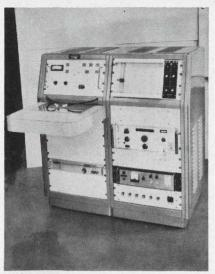
**Wide-range filter test set** was developed by Sylvania Electronic Systems for use in high-volume filter production (paper 28.1). (28.2, Tues./p.m./SS)
