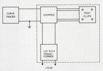
**Diodes are quickly and simply matched** when this test jig is used in conjunction with a curve-tracer. The chopper is employed for viewing the low-voltage portions of the E/I curves. For higher level portions, a reed relay should be substituted for the chopper.
