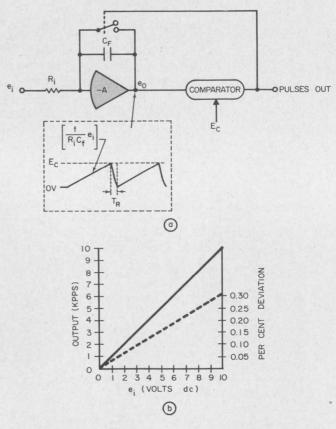
1. Conventional analog-to-frequency converter (a) operates with an output of 0-10 Kpps and has linearity of 0.5%. Integrator's reset time ( $T_R$ ) limits linearity of the response, especially at high pulse rates. Curve shows the relationship between input voltage, output pulse rate and deviation from linear response (b). Note error due to  $T_R$ .
