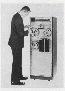
Speed of 1200 words per minute is offered by the System 311, which can operate over standard telephone lines.
