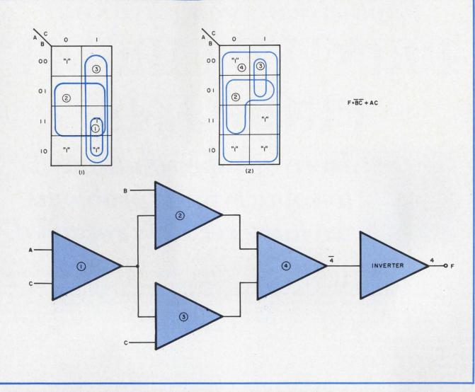
9. Inverter is needed at the output when 'O'' blocks are generated by the map-factoring method. This is because
