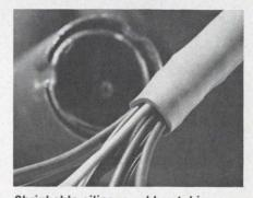
**Shrinkable silicone rubber tubing** can be the answer where wiring harness and electronic devices or components must be protected. Silastic<sup>®</sup> brand heat shrinkable tubing simplifies processing – reduces cost – where quick, easy fabrication of a close-fitting insulating covering for splices, leads, or components is required. Shrinks to <sup>1</sup>/<sub>2</sub> dia. when heated to 300 F or higher ... in length less than 5%. (Circle No. 853)
