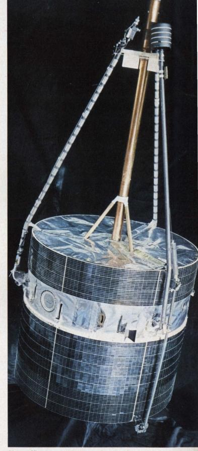
**Pioneer VI** space vehicle was launched on Dec. 16, 1965 to provide data on interplanetary environments. It's electronic equipment is powered by 10,368 individual solar cells. (paper 67.2)
