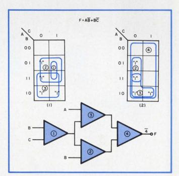
Fig. 7. Each NAND block corresponds to one of the loops generated on the map by the inhibiting process.
