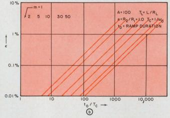
the ideal case and C(t) the actual signal. The amount of ramp delay is a function of both amplifier gain and bandwidth, and (of course) the system time constants ( $T_L$  and  $T_o$ ) (b).
