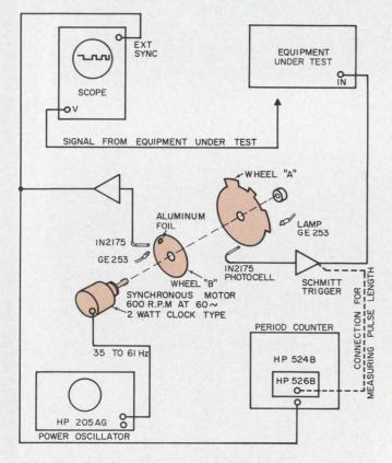
**Teletype signals are generated** by this variable-speed photochopping system. Wheels A and B produce the various facsimile and timing pulses. The system is also capable of viewing teletype signals.
