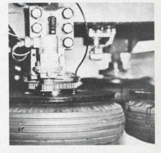
7. **Guide wheels** keep train on tracks. Gear driven odometer sends mileage to transmitter aboard car.
