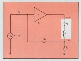
4. Greater coil inductances exhibit large resistances. For larger yokes, the resistor's influence on the transfer function must now be considered. Here  $R_{\rm e}$  denotes the coil resistance, which modifies the gain and feedback values, according to its comparison with the load.
