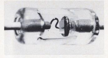
9. Schottky-barrier diode has a multiple pad surface which allows whisker contact to any one of the metal pads.
