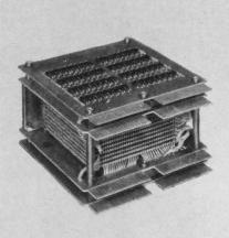
Customer: Honeywell 64 x 64 x 9 stack for H-200 computer
