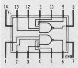
SN15944/SN15844 Dual 4-input Expandable NAND "Power" Gate
