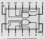
SN15932/SN15832 Dual 4-input Expandable Buffer
