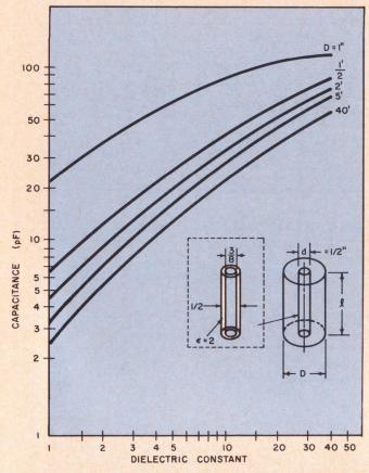
4. Probe capacitance varies as a function of dielectric constant as well as the diameter of the outer electrode.
