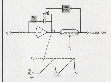
2. The simple addition of a feedback resistor and a one-shot to the circuit of Fig. 1a produces an A-to-F converter that operates up to 250 Kpps with a 0.01% linearity figure.
