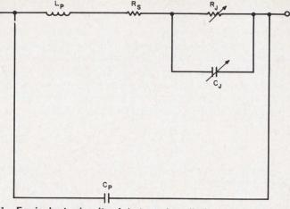
1. Equivalent circuit of hot-carrier diode shows important parameters. Typical values are: 11 ohms series resistance, 0.15 pF package capacitance, and 3 nH package inductance.
