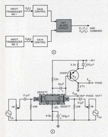
Two closely spaced transducer audio input signals are combined in a FET mixer (a). Complete circuit (b) shows high isolation ( $Z_{\rm in} = 10 \text{ M}\Omega$ ), good linearity (400 mV dynamic input range) and dual outputs (0° and 180° phase shifts).
