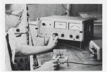
2. Hewlett-Packard vector voltmeter is used to provide voltage and relative phase measurements at a glance.
