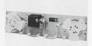
**Ohr-Tronics paper tape readers** can handle tapes of up to 8 channels at speeds of 30 charac/sec.
