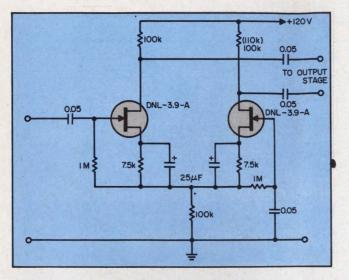
4. **Hi-fi power amplifiers may be driven** by this directcoupled FET phase-splitter. High gain and low distortion are provided by the phase-splitter and source-follower FET combination. The dashed components are used for filtering.
