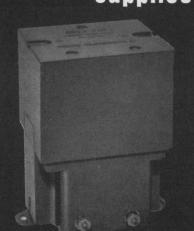
**Building-block construction provides** a basic transformer, rectifier, and where necessary a regulating device. The three molded elements bolt together quickly and maintenance is simplified. Output is completely isolated. DC voltage is filtered and provides 5% or less ripple. Most units rated for 5 ma, current. Input 115V, 60 cycle. Units available from 15 volts to 100-KV-DC.
