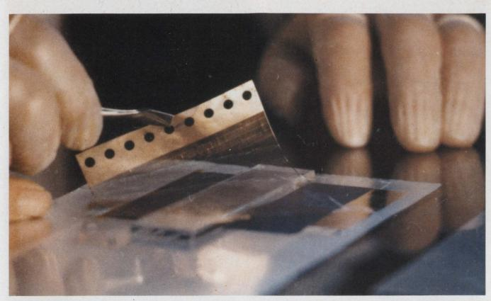
Thin-film polycrystalline solar cells are now under development at RCA Laboratories. (paper 77.2)
