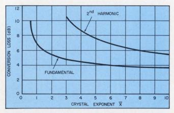
4. The actual conversion loss at the diode's junction may be expressed in terms of  $\overline{x}$ , which is d log i/d log v (a logarithmic relation of the diode's V-I characteristics). The loss decreases rapidly as  $\overline{x}$  increases. These curves were plotted while the image frequency in the mixer was matched. As a result, the diode has wide dynamic range.
