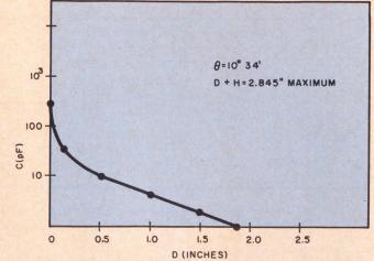
6. Large displacements of the transducer are possible with the coaxial-cone arrangement, because of the minimizing of fringing effects.
