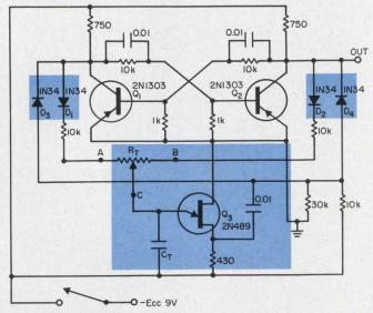
UJT, steering diodes and potentiometer add to versatility of bistable multivibrator.  $Q_3$ ,  $D_1 - D_4$  and  $R_T$  enable symmetry, pulse width and repetition rate to be independently controlled.
