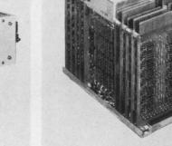
Customer: Honeywell 128 x 128 x 9 stack for H-2200 computer
