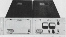
This rack holds two HS power supplies. Each power supply is rated at 12 volts, 20.5 amps.
