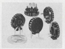
Trimmer needs in printed-circuit test, measurement and communications equipment are met by a new miniature closed-construction potentiometer. It features a rotational life in excess of 25,000 cycles and is 0.696" in diameter and 0.250" deep (including knob). Designated the Model 9, its range is 100 $\Omega$  to 10 M $\Omega$  (1/5 W) in the linear version and 200 $\Omega$  to 1 M $\Omega$  (1/10 W) with a non-linear taper. 20% tolerance is standard; 10% optional.
