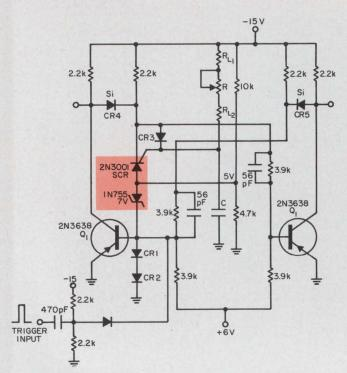
This modified one-shot multivibrator uses an SCR-zener combination for longer time delays and squarer outputs. In effect, these components isolate the timing elements from the switching network.
