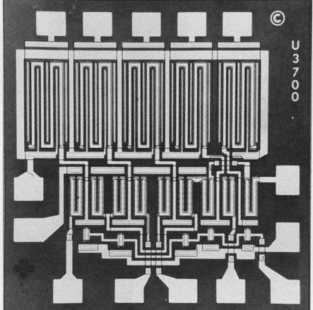
Multi-channel IC commutator has low on-resistance.
