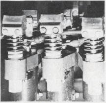
3. Articulated pantograph, or brushes, tap rails for three-phase power. Brushes contact rails from bottom.
