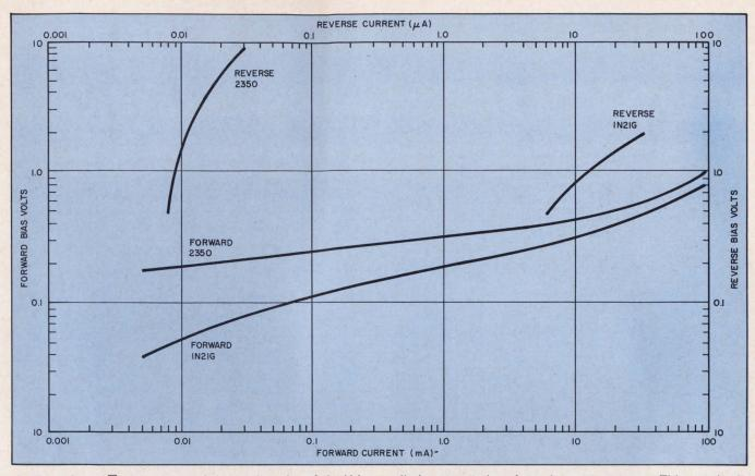
5. The value of  $\overline{x}$  is the slope of the log-log plot of the V-I characteristics, shown here. For hot-carrier diodes  $\overline{x}$  is much larger and remains constant over a larger range of
