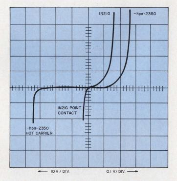
2. Voltage vs current profiles of a hot-carrier diode and a point-contact diode show the higher reverse breakdown voltage of the hot-carrier type.
