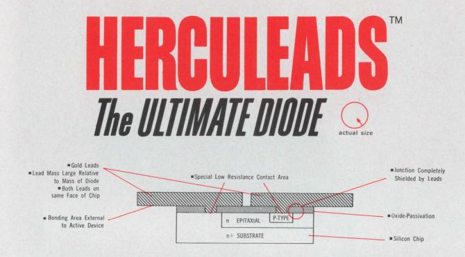
General Instrument's HERCULEADS beam-lead diode is a self-contained diode package with total environmental immunity-the smallest discrete diode available - and it is virtually indestructible.
