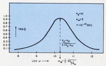
2. **Resonant-like characteristic** is exhibited by the dielectric constant when it is considered to be made up of a real and an imaginary component.
