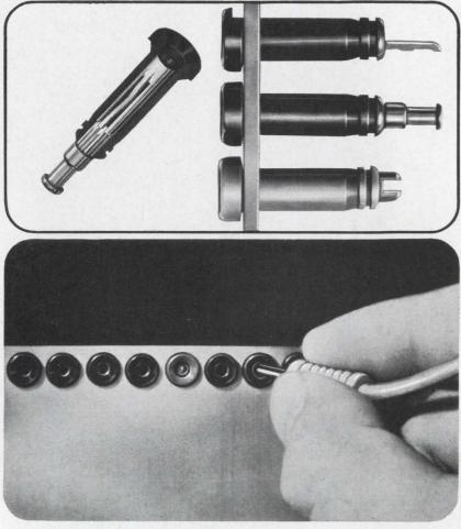
Now Ucinite offers you press-in test jacks for high-density, low-weight applications. Using nylon insulators available in 11 colors, these new test jacks have stamped or screw-machined closed-entry, beryllium-copper contacts that meet the performance requirements of MS-16108. They are available in a variety of terminal styles, and finishes. For complete details write for Bulletin 7072.
