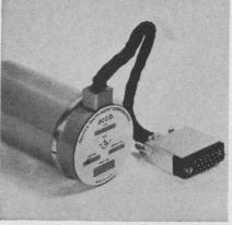
Containing a D'arsonaval torquer, the 20IG type C40D permanent magnet torquer rate integrating gyro is said to eliminate magnetic restraints, hysteresis, saturation non-linearities and power drain from a reference field. The 0.1% torquer linearity holds for 300,000 degree/hours torquer rate and the company guarantees 5000 hours as the dynamic wearout wheel bearing life.
