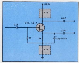
3. **Phase-splitting can also be achieved** with a FET. The circuit basically is a source-follower, with the load shared by both the drain and source. Lower distortion levels (in comparison with higher-driven tube counterparts) are achieved.
