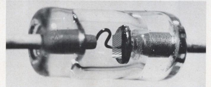
Schottky-barrier diode bridges the gap. 178
