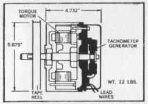
turned from conventional tape transport designs and developed a unique militarized system capable of optimum tape handling without damage or distortion. This modern, miniaturized design provides rapid reversal (less than 6 milliseconds) so programming is not restricted, high controlled acceleration and deceleration, (empty reel: 570 rad/sec<sup>2</sup>, full reel: 270 rad/ sec<sup>2</sup>), wide dynamic speed ranges (1000/1).
