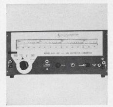
A 1 ppm resolution is featured in the Model H04-3460A Digital Voltmeter. An integrating-potentiometric unit, it measures 100 mV within 0.005% of reading. Accuracy is retained for at least 90 days. Designed for automatic operation in digital data acquisition systems, the unit's four ranges, up to  $\pm 1000$ V, can be selected.
