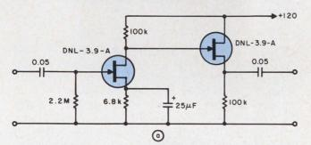
2. **Direct-coupled source-follower circuit** employs a FET to obtain a high gain-bandwidth product (a). This stage makes for an excellent audio preamplifier output stage. A comparison of its overload characteristics with those of other basic audio circuits (b) shows its low-distortion and high-output capability.
