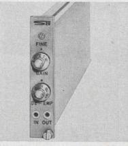
Features of the Model S-29 telemetry amplifier include a switchable de-emphasis circuit and a frequency response of 300 Hz to 2 MHz at a gain of 5 or less. In addition, dual inputs provide a low impedance for summing the outputs of the manufacturer's line of VCOs containing built-in mixing resistors. Output voltage is 20 V and current is 100 mA.
