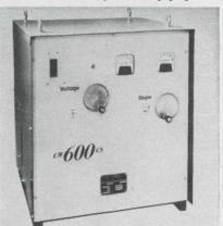
The regulated supplies SPS-2055 and 2062 are designed especially to provide dc power to integrated circuits. The model shown, SPS-2055, has a voltage adjustment range from 1 to 6.5 V and can continuously deliver 0 to 300 mA. Line and load regulation is better than 3 mV dc and ripple is typically 1 mV. Both use silicon transistors and include overload protection.
