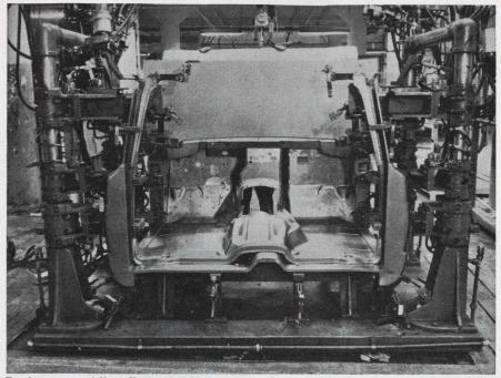
**Resistance-welding fixture** at Kaiser Jeep Corp. incorporates simplified tooling plus standardized welding equipment (paper 29.1)
