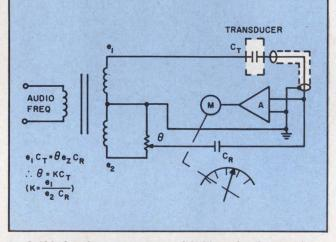
9. Self-balancing servo type of bridge circuit provides a continuous measurement of capacitance. The capacitance value is indicated by a motor-driven potentiometer.
