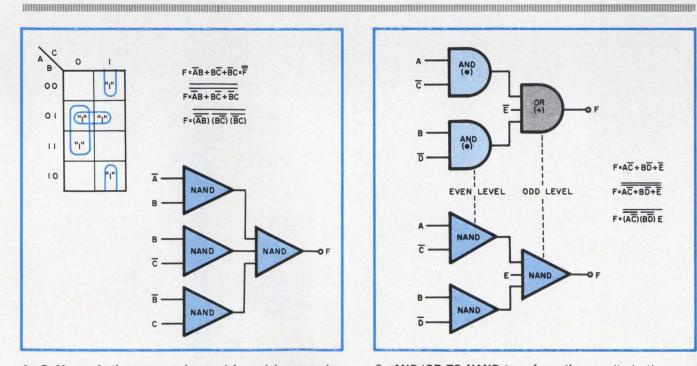
1. DeMorgan's theorem can be used for quick conversion of a function to a NAND form. But the results contain complemented and uncomplemented variables.
