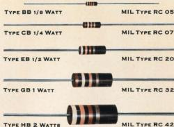
HOT MOLDED FIXED RESISTORS are available in all standard EIA and MIL-R-11 resistance values and tolerances, plus values above and below standard limits. Shown actual size.
