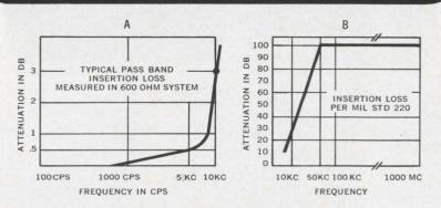
Graphs A and B show typical characteristics of Potter signal line filters. These filters are used on systems which must meet Defense Communications Agency criteria and provide maximum attenuation above the pass band with less than ½ db attenuation in the pass band. ■ Write for further information on these and other Potter filters.
