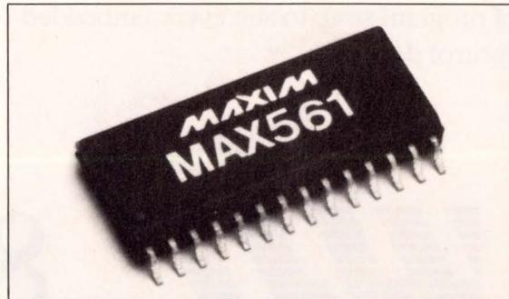
**This RS-232C transceiver from Maxim Integrated Products implements the new EIA/TIA-562 standard, which guarantees operation with output voltages as low as  $\pm 3.7V$ . The device can operate at voltages as low as 3.0V at a data rate of 20 kbps.**
