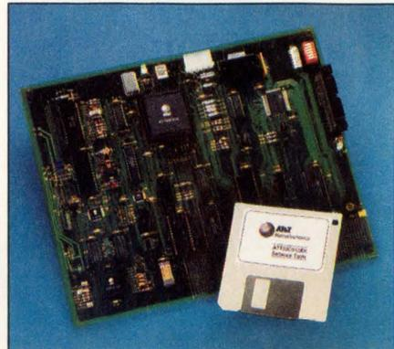
Evaluation boards for specialized DSP chips, such as the AT&T Microelectronics 93C010 created for hard-disk applications, give your embedded design a real head start.
