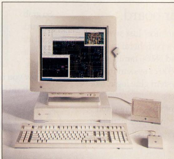
**SPARCstation 10 is the first Sun workstation to use MBus modules for multiprocessing.**
