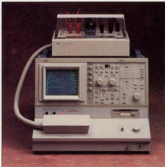
Testing components at power levels as high as 3000W is possible using the 317A Programmable Curve Tracer from Tektronix.
