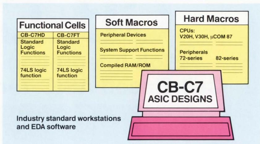
For example, the library of mega-function blocks contains cores of our  $\mu$ COM87, V20H and V30H microprocessors, plus intelligent peripheral functions such as those provided by NEC's 72-series and 82-series standard peripheral devices. And because most of these megafunction blocks are hard macros, derived directly from the chip layouts of our standard parts, they have fully characterized timing parameters and can be tested with the standard part test vectors.
