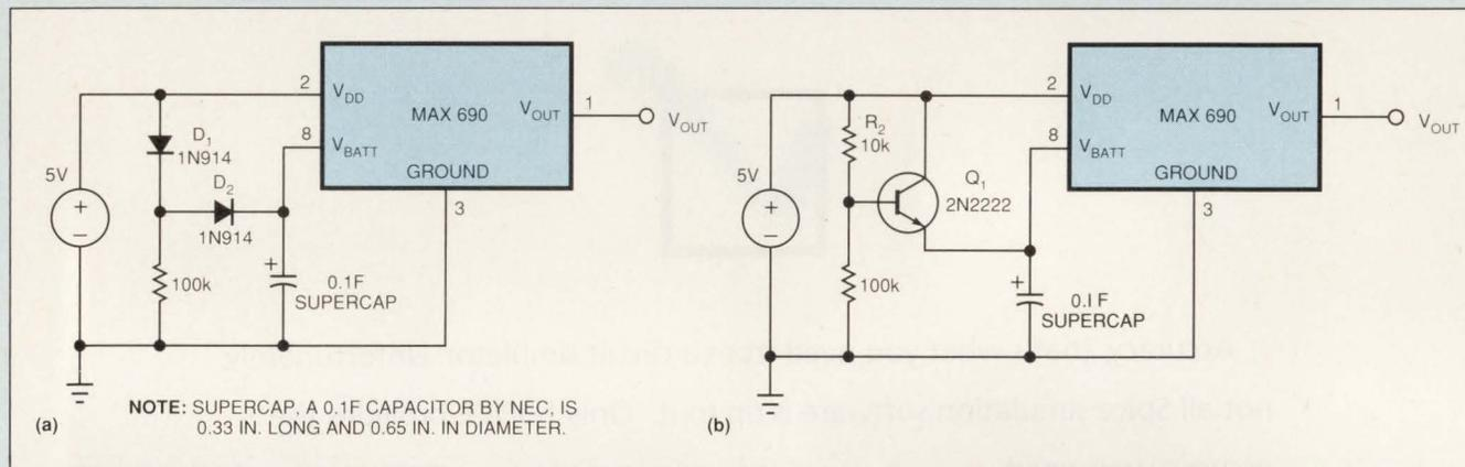
**Fig 1**—Teamed with a switch-over IC, large capacitors can serve as battery backup in certain applications. The 100-k $\Omega$  resistor in (a) ensures that  $D_1$  is forward biased so that normal variations in  $V_{DD}$  don't mistakenly trip the IC. The presence of  $Q_1$  and its associated resistors in (b) shorten the delay between power on and backup capability.
