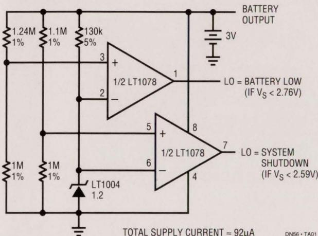
Figure 1. Low Battery Detector with System Shutdown
