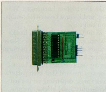
You can debug 68HC16 target code without an ICE. To monitor and control execution, the ICD16 links to the target  $\mu\text{C}$  via background mode.
