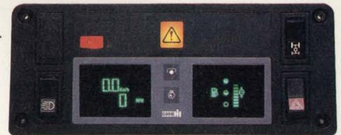
*Electronic Instrument Panel to J.I. CASE Tractors.*
