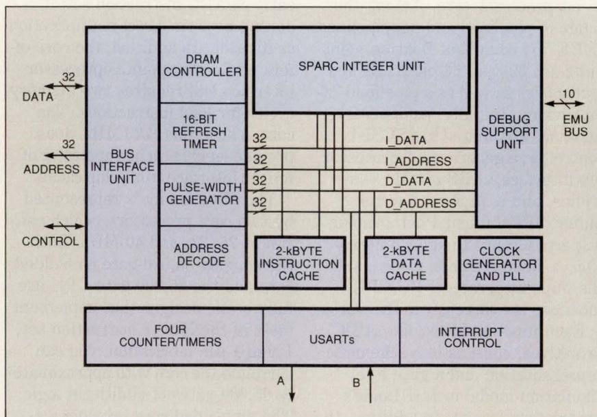
SPARC RISC fits embedded systems. The SPARClike  $\mu\text{C}$  combines a SPARC CPU with on-chip cache, timers, and an interrupt controller.
