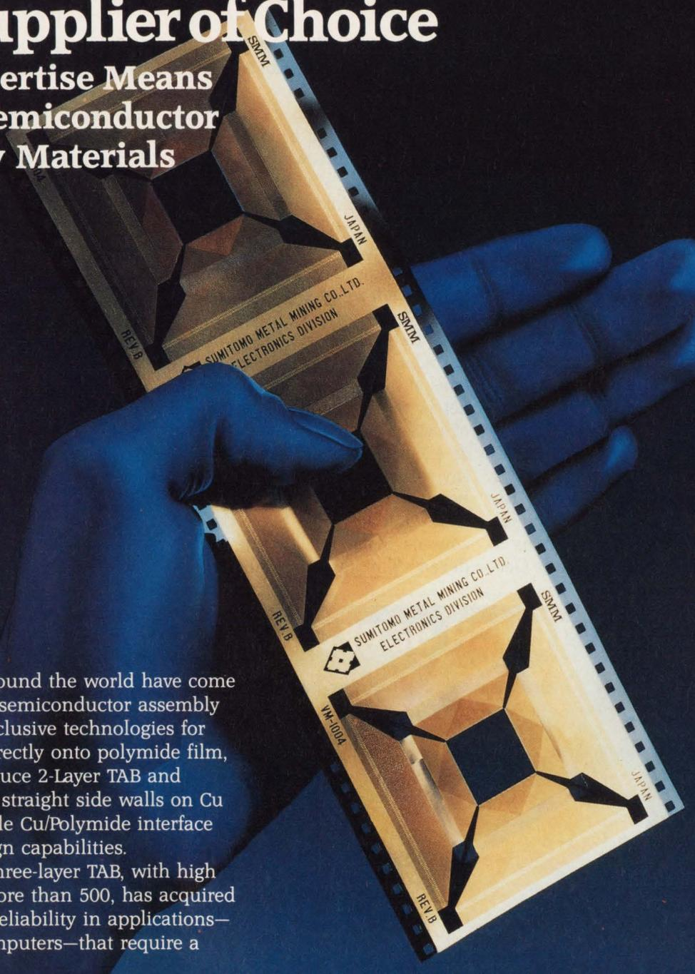
Device makers around the world have come to rely on SMM's semiconductor assembly materials. Our exclusive technologies for copper plating directly onto polyimide film, for example, produce 2-Layer TAB and 2-Metal TAB with straight side walls on Cu leads, a low profile Cu/Polymide interface and flexible design capabilities.
