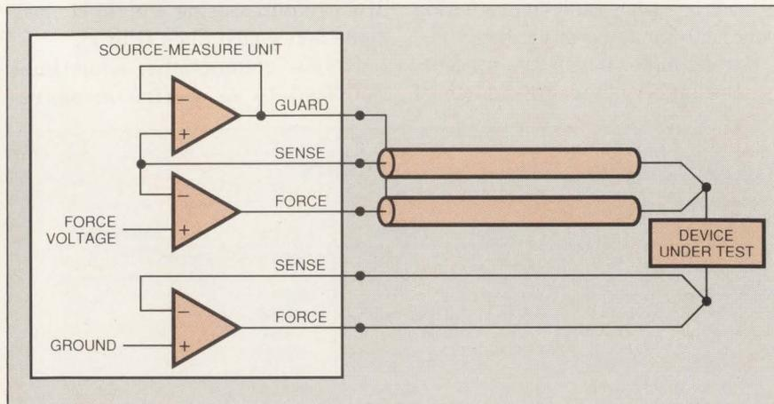
**Fig 1**—Kelvin connections avoid measurement inaccuracies caused by voltage drops in the current-carrying force line by sensing and correcting the voltage to the device under test. The guard line shields the force and sense lines from current leakage that would otherwise cause inaccurate current measurements.
