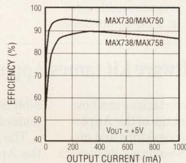
The MAX730/MAX750 and MAX738/MAX758 deliver high efficiency over a wide load range.
