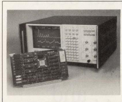
the analyzer's CPU. The two processors exchange data via DMA and simultaneous register transfers. The analyzer, which accepts plug-in front-end modules, handles signals to 1 GHz. You can install the DSP board in the analyzer. \$2995.
