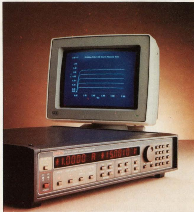
Source-measure units connected to a computer for control and display let you create a parameter analyzer or test system to suit varied requirements. The model 238 from Keithley Instruments offers current to 1A.
