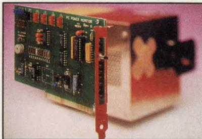
Designed as a diagnostic aid for PC/XT/EISA systems, the Wintek PC Bus Power Monitor Card (\$195) provides a quick way of checking the power supply in a personal computer. LEDs provide a real-time indication of power quality, as well as remembering momentary out-of-tolerance operation. A deluxe model (\$249) has an audible alarm, a system clock monitor, and a refresh signal monitor.
