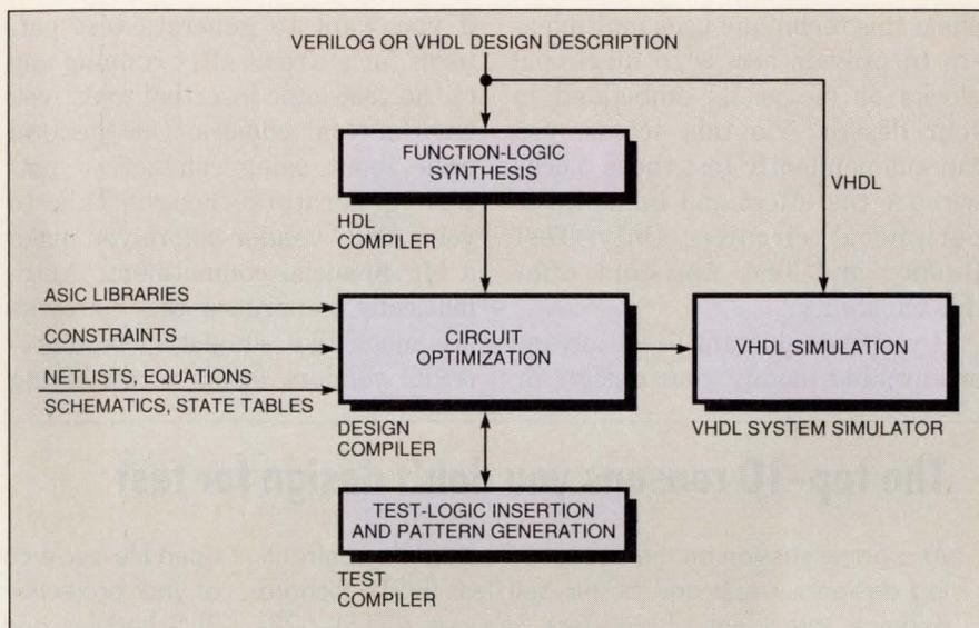
**Beginning with either Verilog HDL or VHDL, Synopsys' test strategy is to first synthesize and optimize your function logic, then insert the test logic and generate patterns.**
