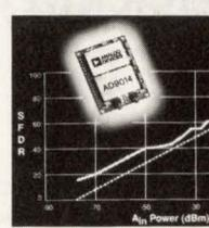
The AD9014, a 14-bit ADC, guarantees encode rates up to 10 MSPS. Faster than any comparable solution, the ECL-compatible ADC also guarantees the widest dynamic range among ≤14-bit competitive devices. While the AD9014's ac characteristics are optimized for high-speed spectrum analysis designs, its dc specifications also make it well suited for oversampling low frequency inputs.
