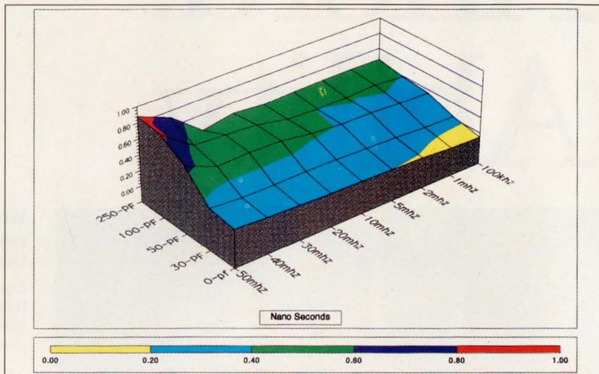
**Fig 3—Guaranteed skew specs aren't necessarily the results of thorough testing. However, National Semiconductor does provide extensive test data such as this graph, which shows how output capacitance and clock frequency affect the output-to-output skew of the CGS74B2525.**
