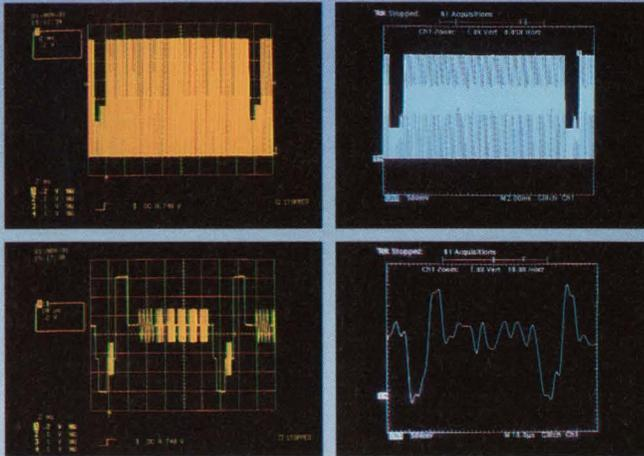
In many applications, there's no substitute for a really long memory. The screens above show a complete TV field captured at 2 ms per division. The benefits of the long memory are shown when the waveform is expanded to view a single TV line.
