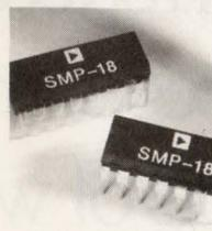
With acquisition time to 2.5 μs, the low-cost octal sample-and-hold amplifier SMP-18 also provides an on-chip 1:8 demultiplexer. It's complete with on-chip hold capacitors and is well-suited for applications where setting voltage levels are required. Applications include ATE, comparator and time delay generator circuits, process control system set points, and more.
