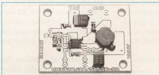
The MAX730 application circuit components fit into 1/2 in<sup>2</sup> (3.2cm<sup>2</sup>) of board space.
