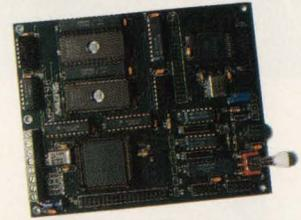
The MP-196 is a single board computer targeted for 80C196KC based embedded control applications. Board features include 16 MHz operation, power and ground planes for noise minimization, processor supervisory circuit, optional paged memory support, and optional A/D and D/A daughterboard. In addition to CPU resources, a DUART chip provides two serial ports, and two parallel ports. Optional development software is also available.
