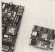
The ADDS-2111 EZ-Tools (EZ-ICE™ and EZ-LAB™) are low-cost and easy-to-use support tools for the fixed-point ADSP-2111 DSP. EZ-ICE is an in-circuit emulator for debugging code and testing systems; the EZ-LAB is a demonstration and evaluation board.
