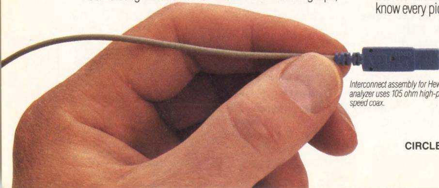
Interconnect assembly for Hewlett-Packard logic analyzer uses 105 ohm high-performance, high speed coax.
