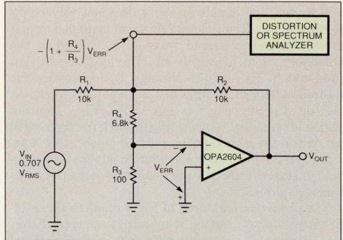
**Fig 4—Adding  $R_4$  combines selective amplification with signal separation for the inverting amplifier.**
