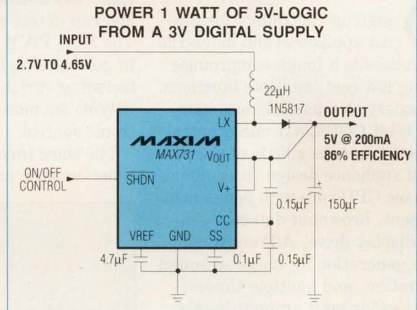
The MAX731 surface-mount circuit fits in 0.65in<sup>2</sup> (4.2cm<sup>2</sup>) and has 86% efficiency while delivering 200mA at 5V from a 3V source.
