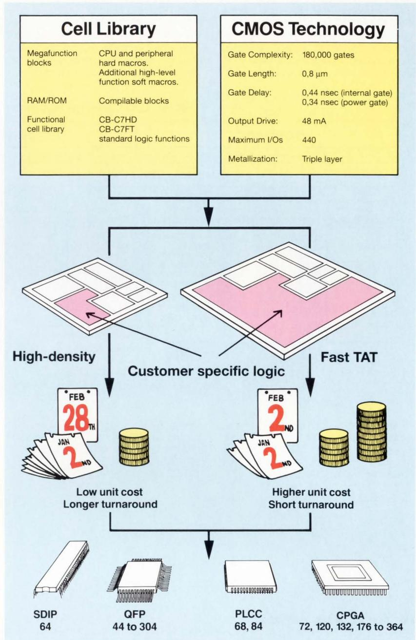
blocks and optimizing user-defined logic. It is then floor-planned using ChipPlan, simulated with System Hilo or Verilog, and placed and routed using Cell-3 Ensemble. After post-layout simulation and design-rule checks, we pass pattern generation data to one of our wafer fabrication facilities in Japan, the USA or Europe.
