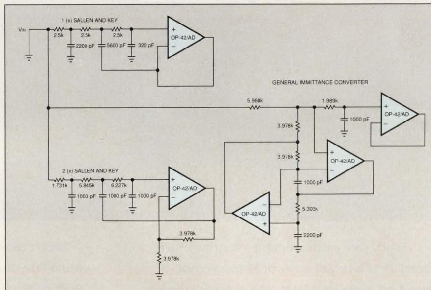
(Author's reply: The first difference Michael Wyatt points out is in the cutoff frequency that Fig 5 [in the article] had for the Sallen and Key filter. He says that simulations of this circuit show it has a cutoff frequency of about 29 kHz, not 40 kHz as specified. Upon examining my data and doing my own Spice simulations, I find that Wyatt is correct. The reason for this and the associated peaking that the filter exhibits is that the 1.731- and 6.227-kΩ re-
