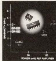
Analog Devices' OP-282 (dual) and OP-482 (quad) op amps provide excellent speed at ultralow supply currents. Slew rate exceeds 7 V/μs with supply current under 250 μA per amplifier. These op amps are well-suited for battery-powered systems or power-restricted applications; their input common-mode range includes a positive supply for high-side signal conditioning.
