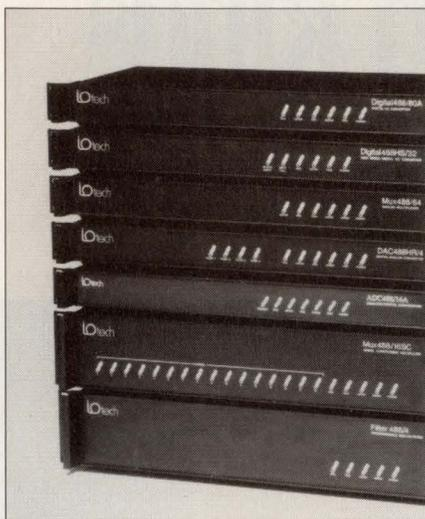
**Iotech's Data Acquisition Instruments family now includes ADCs, DACs, filters, multiplexers, and digital I/O interfaces**
