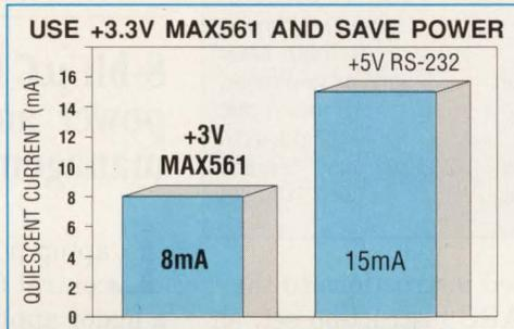
The +3.3V powered MAX561 uses 1/2 the power of +5V RS-232 devices.
