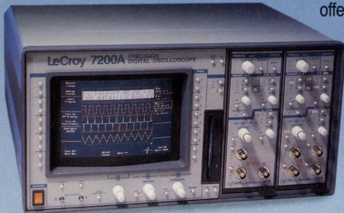
The new 7200A Series, our high performance line with high resolution color display, features 500 MHz bandwidth at 2 GS/s with 200k memory standard and 1 Meg/channel optional. Modular architecture allows the user to choose 2, 4 or even 8 channels, all with super-long memory. Floppy and hard disk drives are standard features.
