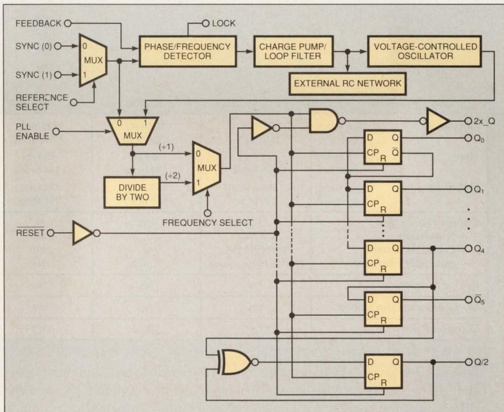
**Fig 1—Phase-locked loops are popping up in purely digital designs for two reasons: They can produce multiples of an input clock reference, and they enable you to control the phase difference between that reference and the output. Motorola's MC88915 provides one output at  $2\times$ , six at  $1\times$ , and one at  $\frac{1}{2}\times$  the input frequency.**
