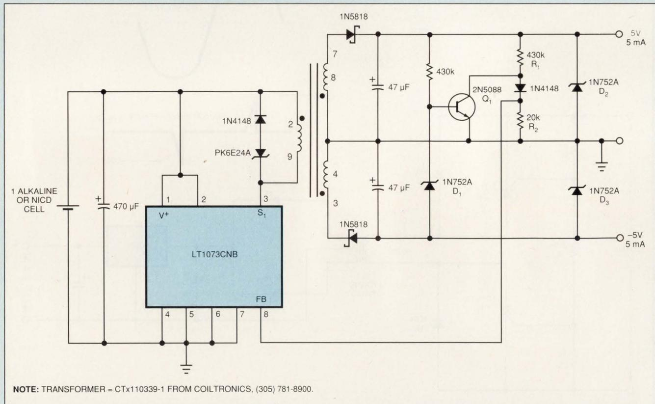
Fig 1—To produce a split supply from a single cell, this circuit uses a micropower dc/dc converter to supply  $\pm 5V$  and any 10-mA current combination.
