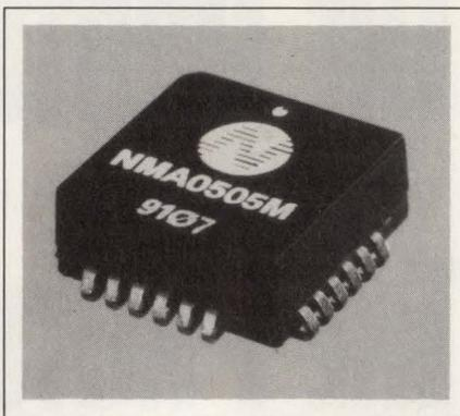
of ±5, ±9, ±12, or ±15V. Each output provides 1W of output power. The converters feature 1000V dc isolation, 80% efficiency, and operate over a -50 to +85°C range with no derating. \$19.50. **International Power Sources Inc**, 200 Butterfield Dr, Ashland, MA 01721. Phone (508) 881-7434. FAX (508) 879-8669. **Circle No. 396**
