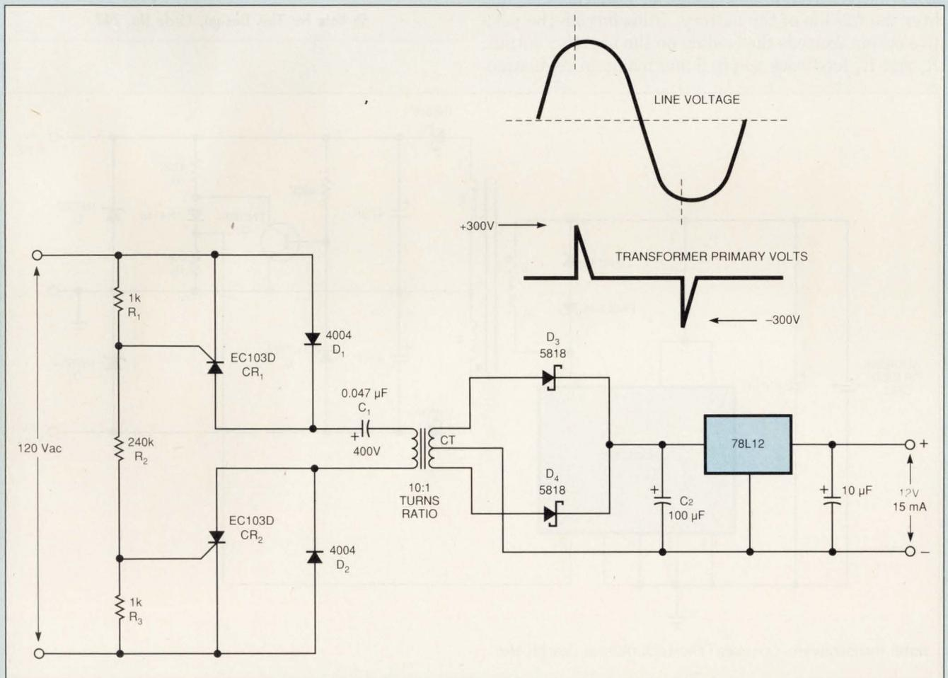
Fig 1—Smaller and cheaper than many other off-line power supplies, this low-power circuit transfers power from a 120V ac line to a voltage regulator by discharging a capacitor through a small, high-frequency transformer.
