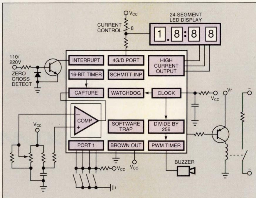
Smart appliances can be controlled with a single low-end, 8-bit  $\mu\text{C}$ , the COP820CJ. In a 20-pin DIP, the chip supports small displays, motor control, power management, and user appliance control.
