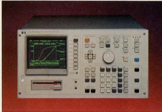
Comprising four SMUs integrated into a benchtop instrument, the HP4145B provides programmable data acquisition and display. You can store test setups and data, using the floppy-disk drive, or control the instrument through an IEEE-488 bus interface.
