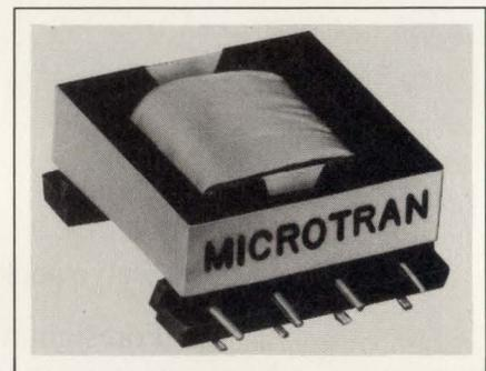
coupling and hybrid applications. They feature 0.5% max distortion, 26-dBm return loss, 60-dB min longitudinal balance, and 1500V rms dielectric strength. The transformers are constructed from materials that have a UL 94V-0 flammability rating. Units with pins for through-hole-mounting applications are also available. The units measure  $0.87 \times 0.66 \times 0.32$  in. and weigh 0.2 oz. Approximately \$3 (OEM qty).
