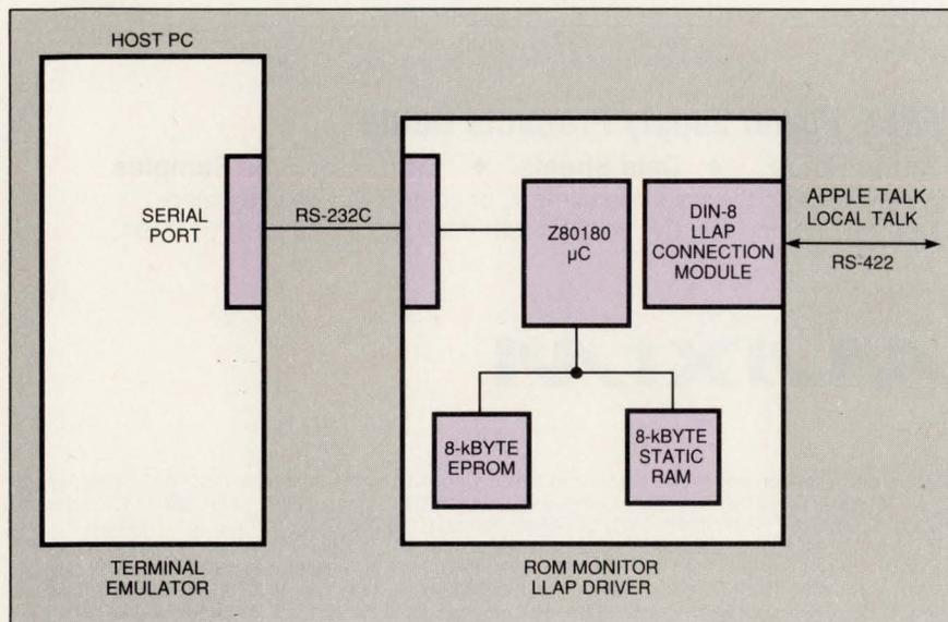
Help for the toughest part of the Appletalk communications protocol is available in a kit that includes source code and a Z80181  $\mu$ C-based board.
