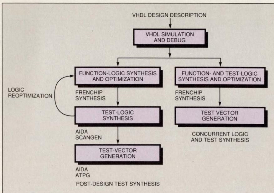
Post-design test insertion requires evaluating the impact of the added test on your design. Teradyne recommends specifying the test structures from the start.
