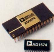
**The AD1674 retains the pinout and functionality of the AD574, AD674 and AD774, while integrating a high-bandwidth sample/hold circuit, higher speed, lower power, and lower price – from \$14.15 (suggested, 100s). The AD1674 accepts input signals of  $\pm 5V$ ,  $\pm 10V$ ,  $0-10V$  or  $0-20V$ , while operating from its standard  $10V$  on-chip voltage reference (available for driving external loads).**
