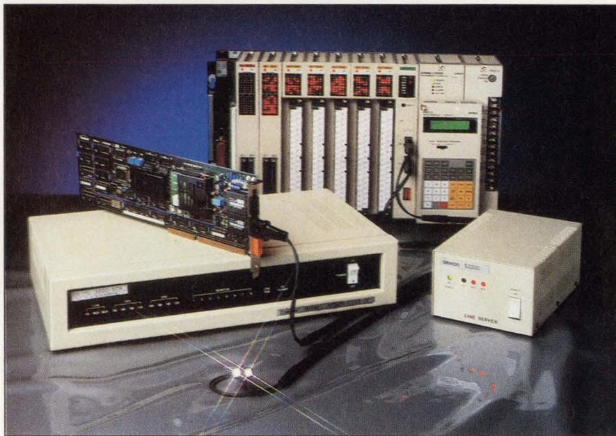
Proprietary networks can benefit specific applications that industry-standard networks often can't. Omron Electronics Inc.'s (Schaumburg, IL) Sysmac Net is a high-speed, fiber-optic token-ring LAN for industrial applications that require high noise immunity. The vendor claims that its plastic-fiber cable is easier to work with than glass-fiber cable. Systems cost approximately \$4000/node.
