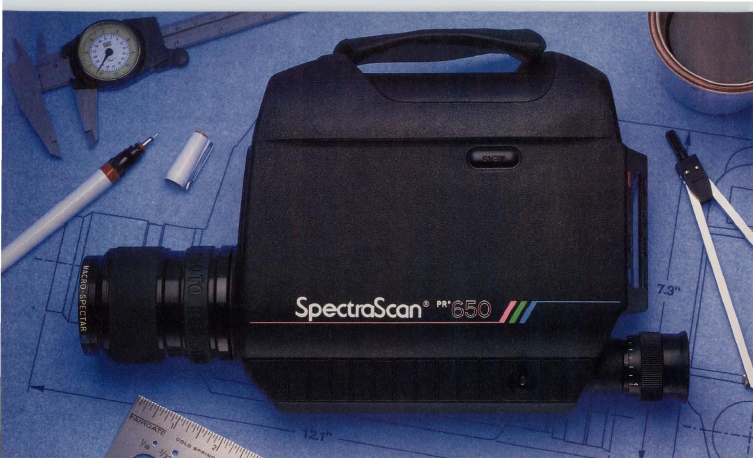
Now you can perform NIST-traceable, spectrally-based photometric and colorimetric measurements anywhere, anytime. With the battery-powered Photo Research® PR-650 SpectraColorimeter™. You no longer need to settle for the inaccuracy of filter instruments just for the convenience of cost-effective portability.
