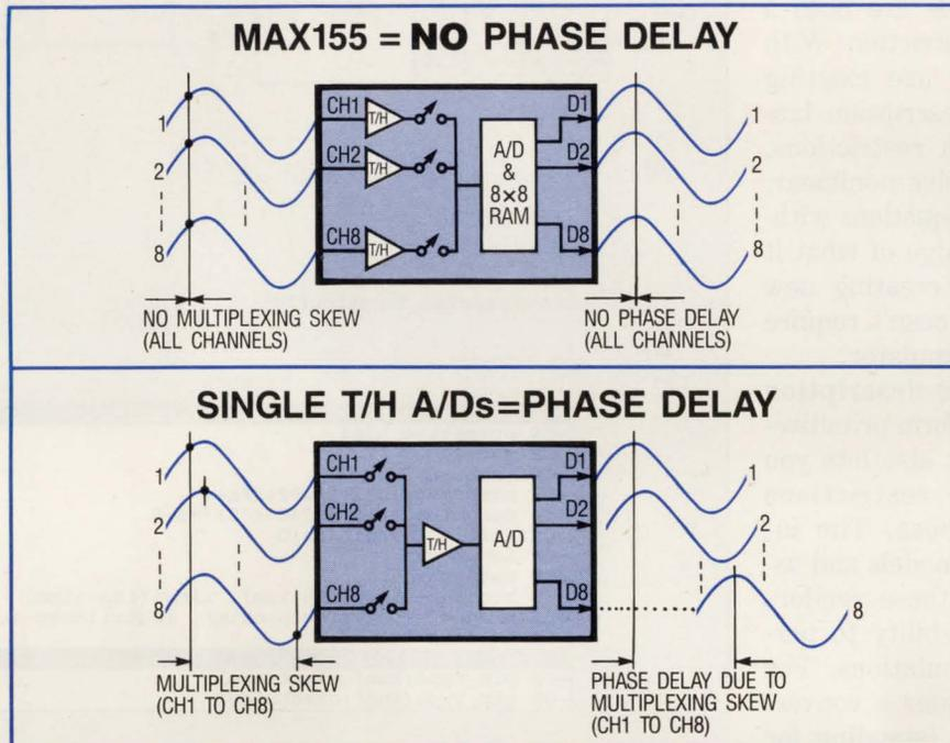
8 T/Hs simultaneously sample to reduce channel-to-channel phase delay to less than 4ns, compared to several microseconds for A/Ds with a single T/H.
