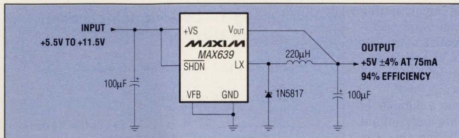
High-efficiency step-down regulation is simple using the MAX639.
