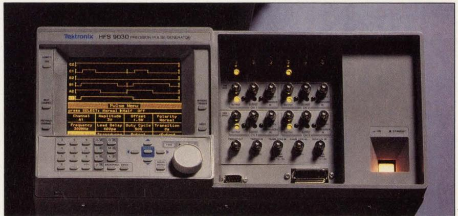
*Modular pulse generators let you choose the performance and number of channels you need. You can choose two, four, or six channels for the instrument shown here from Tektronix. The two channel modules are available in two performance versions.*
