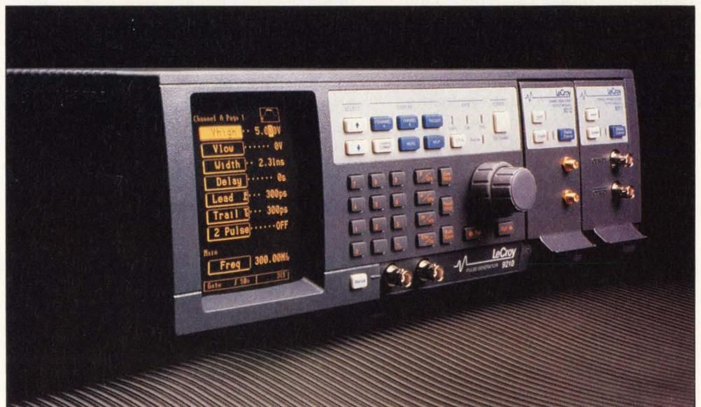
*Touch-screen menus allow easy programming of the 9210 pulse generator from LeCroy. The instrument provides one or two channels, which you can select from any of three module types.*
