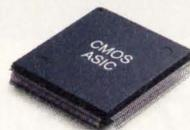
ASIC solutions in both Sea-of-Gates and standard-cells.
