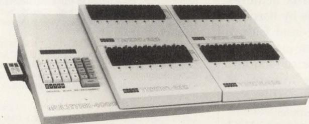
The MULTITRK-4000™'s "mix & match" capability sets a new standard in programming. Using an 8 socket attachable "TRAKCel", the MULTITRK lets you program unusual device packages in combinations of 8 to 32 devices.
