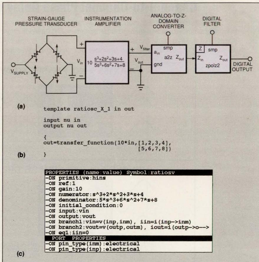
**Fig 1—Graphical design software makes using a hardware-description language easier.** For this pressure sensing circuit (a), Analog's Design Star front end generates the underlying code (b) for the transfer-function instrumentation amplifier based on user-supplied parameters and equations (c).
