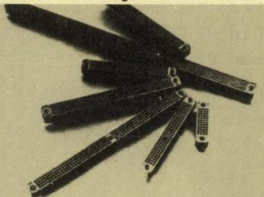
KA/254 Printed Circuit Board Connectors are available with 4 row models with from 48 to 392 positions, and 5 row models with from 230 to 490 positions. These connectors meet D55302 performance requirements. Crimp, flow solder, Wire Wrap, and solder cup terminations are available on .100" x .100" grid spacing.
