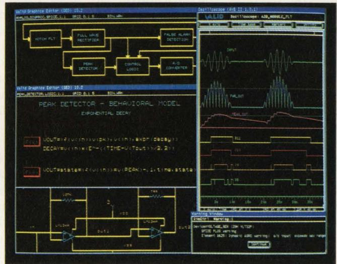
*Behavioral modeling isn't necessarily synonymous with ideal modeling. This model of a peak detector, implemented with Valid's Profile option, includes decay effects. The software also notifies the user that the ADC's input exceeds its input range.*
