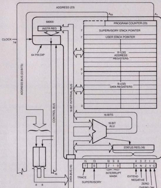
**Hardware notes:** 1. Diagram of basic 16-bit 68000. Family offers growth path from 8- to 16- to 32-bit  $\mu$ Ps. Performance results from multiple ALUs, 32-bit internal operation, and nonmultiplexed address and data buses.
