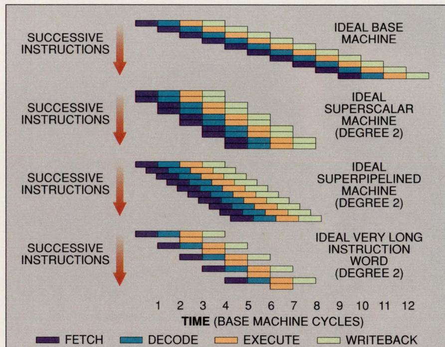
Fig 1—Ideal 2nd-degree superscalar and VLIW machines finish executing 10 instructions a half cycle faster than a 2nd-degree superpipelined CPU. Unfortunately, data dependencies, conditional branches, and instruction mixes cause deviations from the ideal.
