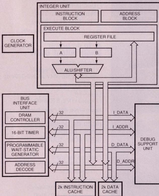
**Software note:** There are four stages (five in Fujitsu's ASIC core) of pipelining. Optimizing compiler prevents pipeline breaks by inserting a delay instruction before branch instructions.
