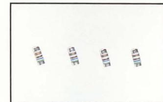
Philips 9BI406 MELF precision resistor benefits from technology used in manufacturing leaded metal film resistors—even though it comes in a surface mount package.
