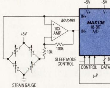
The **MAX135** low-noise, 5V-powered, multi-slope integrating ADC provides ±0.005% accuracy at 16 conversions per second, while requiring only 125μA of supply current over temperature (10μA in sleep mode). Resolution is extended to 18 bits with 3 sub-LSB bits and data averaging. 8-bit data bus and 3 logic control lines simplify μP interfacing.
