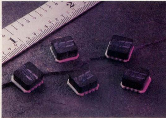
*Accurate to better than  $\pm 0.25\%$ , Model 1431 absolute pressure sensors from IC Sensors are housed in a surface-mount package measuring  $0.3 \times 0.3$  in. They operate from either a constant-current or constant-voltage supply, measure pressure levels of 15 to 300 psi, and have a 60-mV typical output span.*
