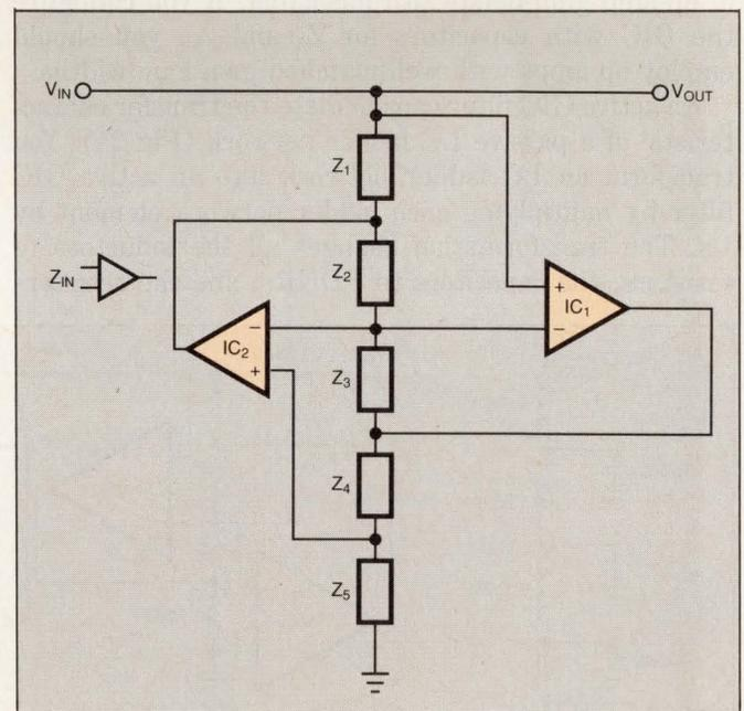
**Fig 1—The topology of a Generalized Immittance Converter (GIC) can simulate the impedance of any passive component, including a frequency-dependent negative resistor (FDNR).**
