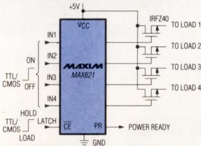
The **MAX621/620** drive 4 low-cost 35A/0.028Ω N-MOSFETs from 4.5V to 16.0V inputs. It combines a power supply, four latched MOSFET drivers, protection circuitry — all in a single 18-pin IC. The MAX621 has internal charge-pump capacitors; MAX620 costs less and requires 3 inexpensive external components.
