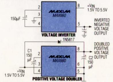
The **MAX660** charge-pump voltage inverter converts a +1.5V to +5.5V input to a -1.5V to -5.5V output. It is a pin-compatible high-current upgrade of the ICL7660. 100mA is supplied with only a 0.65V voltage drop, compared to only 15mA with the ICL7660. Efficiency exceeds 90% for most applications.
