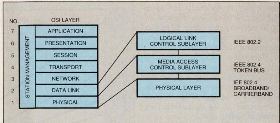
**Fig 1**—Based on the 7-layer ISO/OSI communications model, the Manufacturing Automation Protocol (MAP) was devised by system integrators at General Motors to unite the “islands of automation” created by the computerization of individual manufacturing processes. The IEEE 802 LAN standard provides the specific implementation of the first two layers of the model.
