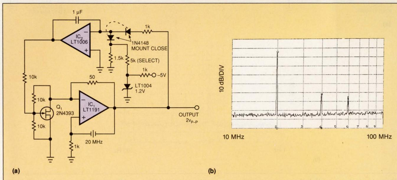
**Fig 5**—An electronic gain-control circuit that uses the voltage-controlled on-resistance of a FET stabilizes the output amplitude of this 20-MHz crystal oscillator (a). In b, you see that the output's harmonics are at least 47 dB below the fundamental.
