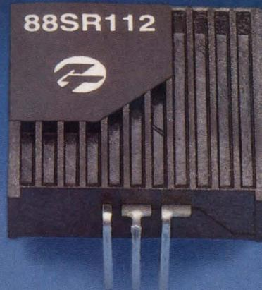
*A fully self-contained 1 MHz step-up Boost Converter*
