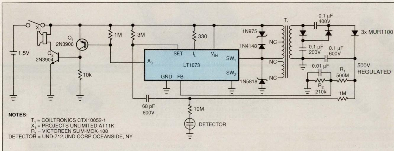
**Fig 1**—To detect radiation and cosmic rays, this circuit provides 500V of bias to the radiation detector, whose impedance drops sharply when a ray passes through it.
