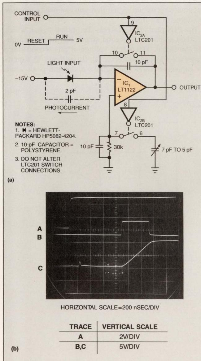
**Fig 2**—The basic photodiode amplifier is the basis for this integrator, which has a resettable output (a). When the control line is high (b, trace A), the circuit integrates (trace C) the incoming signal (trace B).
