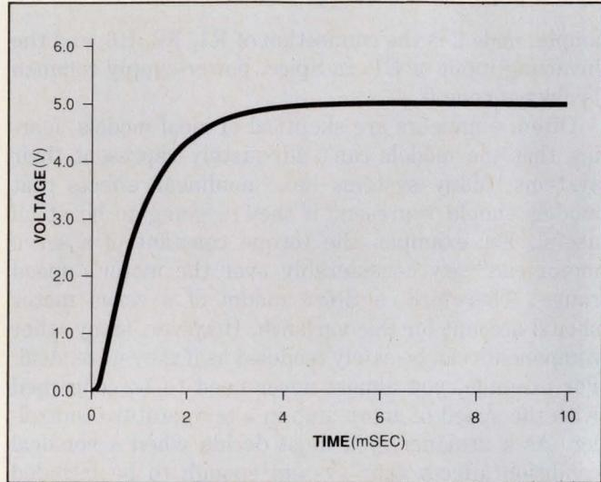
**Fig 5**—The transient (time domain) response of Fig 3's system shows no overshoot with the cutoff frequency of the lowpass filter set to 2000 Hz ( $C1=0.0082 \mu F$ ).
