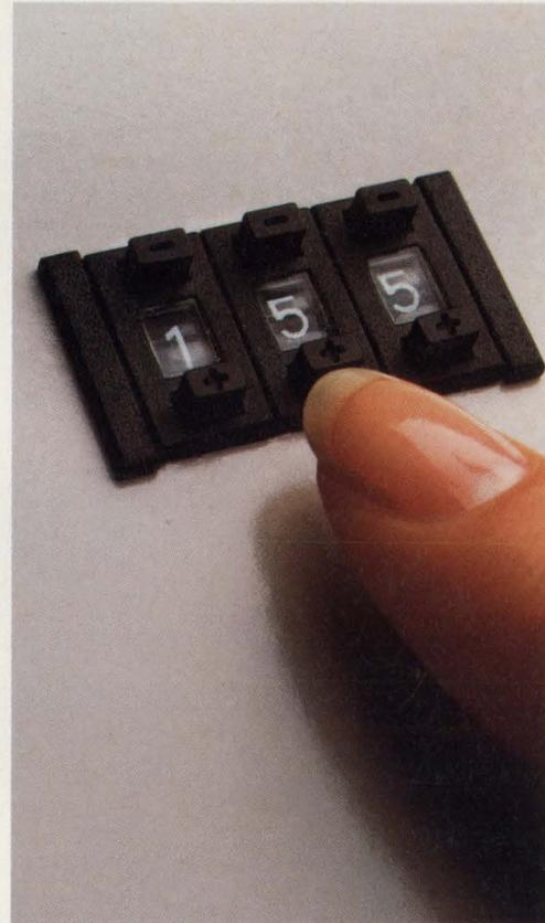
Changing an *Address Switch* takes only one step: punch in the "address" on the back of the computer. Maximum downtime: 20 seconds.
