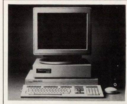
40-Mbyte/sec VSB interface is available as an option. A 3.5x16x16-in. enclosure fits on top of the DECstation enclosure. Compilers for both C and Fortran generate downloadable code. The system comes with a vector and signal-
