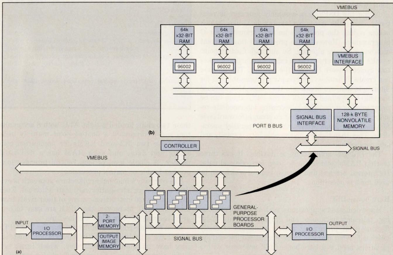
DSP chips are building blocks for large-scale processing systems. Spectrum's Vasp (a) is a scalable, multiprocessor system built around Motorola's 96002 (b). The system was designed for aperture radar applications.
