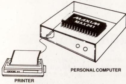
The **MAX241** is a complete serial port on a single chip. It features 4 drivers and 5 receivers in a 28-pin SO package. A separate shutdown mode reduces supply current to a mere 1µA.
