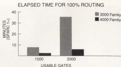
*New algorithms have reduced place and route times by a factor of four.*
