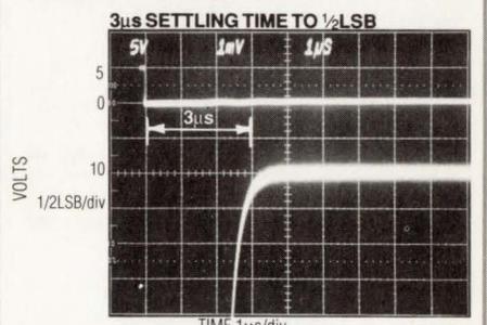
The monolithic **MAX526** replaces 4 DACs and 4 op amps. Monotonic 12-bit performance guaranteed with ½LSB relative accuracy over temperature for all 4 outputs and 1LSB total unadjusted error with no zero- or full-scale adjustments at +25°C. Outputs settle to ½LSB in 3μs.
