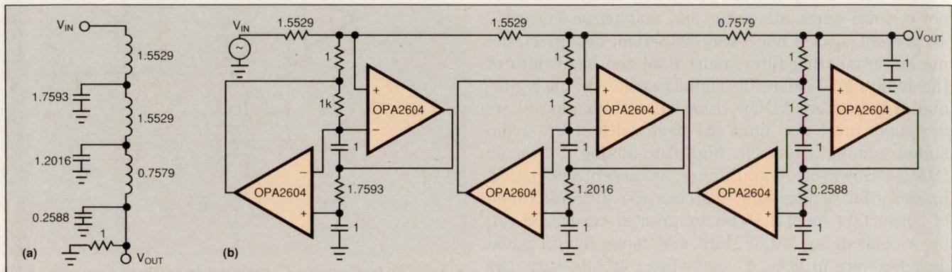
Fig 2—An LC ladder network generates any lowpass-filter polynomial (a). You can simulate the filter's transfer function by multiplying each element value by  $1/s$  and realize the filter using GICs (b).
