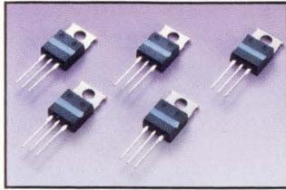
TOPFET® provides over-temperature protection for  $T_j$  above 150°C...short-circuit load protection...rugged overvoltage clamping for inductive load repetitive switching...input ESD protection...and reverse battery protection.
