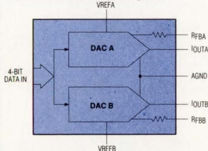
The **MAX759** current-output, four-quadrant multiplying DAC features 1% resistance match between DACs, making many dual applications possible. The new DAC has ±½LSB max integral nonlinearity, ±5ppm/°C max gain temperature coefficient, and operates from a single +5V to +15V supply. Pin compatible to AD7549.
