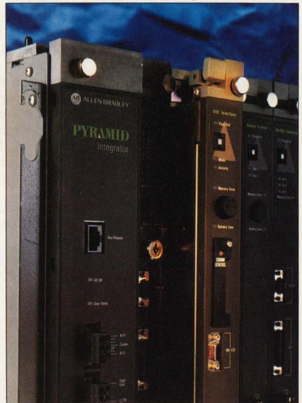
*If you need to tap into a MAP LAN, many proprietary networks offer gateways like this Pyramid Integrator for Allen-Bradley's Data Highway Plus LAN. Using such gateways lets you eliminate "islands of automation" that arise when the controllers from competing vendors can't exchange data.*
