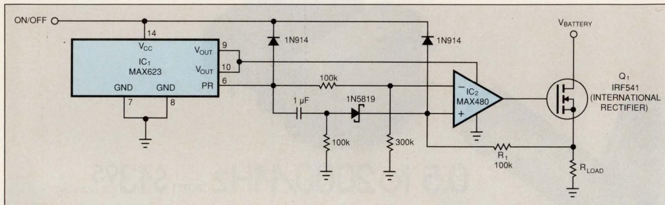
Fig 1—A regulated charge-pump IC generates a gate drive equal to  $V_{BATTERY} + 10V$  for the high-side power switch  $Q_1$ , an n-channel power MOSFET.
