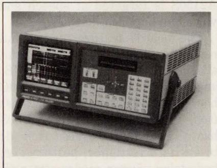
The TIA plugs directly into the LR33000 PGA socket of the board being tested. This direct connection lets users collect information on CPU activity. This activity can then be disassembled by the ML4400 into LR33000 instruction mnemonics. Full disassembly of the LR33000 instruction and data cycles, with tables of as many as 10,000 symbols, is also provided. The TIA registers CPU signals to improve analyzer timing margins
