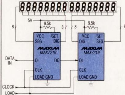
The new **MAX7219** has an easy-to-use serial 3-wire interface and digital/analog brightness control. Only one external resistor is required to set the segment current for all LEDs. The MAX7219 has 1kHz per digit scan rate and is available in a compact 24-pin SO package.
