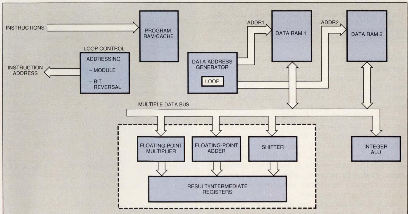
Fig 1—A generic 32-bit floating-point processor supports 3-memory addressing with automatic addressing and loop control. A low-overhead multiply/accumulate unit (MAC) calculates series.
