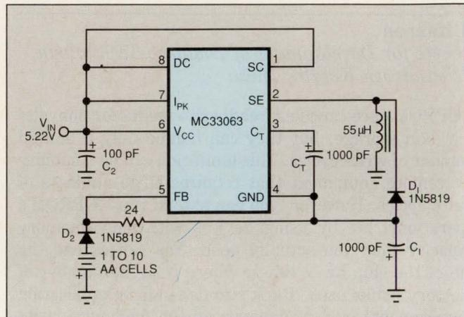
Fig 1—This switched-current regulator can charge anywhere from one to 10 1.5V NiCd cells using an input voltage of approximately 5.2V.
