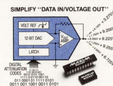
The **MAX507/508** combine a laser-trimmed DAC, a high-performance BiCMOS output amp, and a buried-zener voltage reference on a single IC, greatly improving reliability compared to multi-chip solutions. Data is transferred into the input register in 8+4-bit (MAX508) or 12-bit (MAX507) wide data formats.
