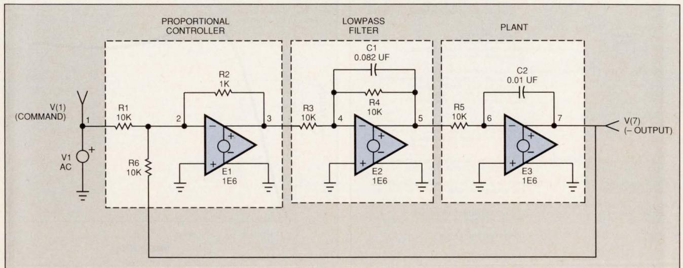
**Fig 3—Op amps and other components** model each of the three blocks—the controller, the filter, and the plant—of Fig 2's control system.
