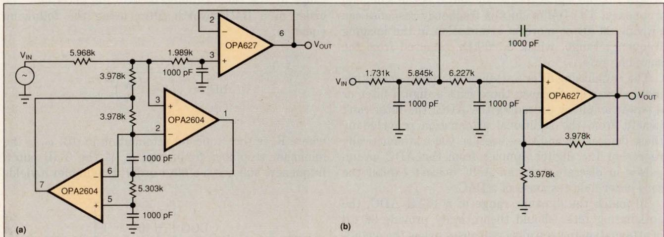
Fig 5—This unity-gain third-order Butterworth GIC filter has a 40-kHz cutoff frequency (a). The equivalent Sallen and Key realization requires twice the gain (b).
