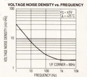
The **MAX412** provides the **best noise performance** — even at very low supply voltages. <2.4nV/√Hz @ 1kHz noise guaranteed! With a guaranteed output voltage swing of 7.3V/PP and greater than 97dB SINAD (Signal/THD+N) while operating from ±5V supplies, the MAX412 is ideal for 5V systems. 8-pin DIP/SO.
