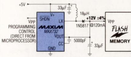
The **MAX732** 200mA step-up regulator is a simple, compact flash memory programming supply that has direct µP-controlled shutdown. It will step up from +5V to +12V±4% at 200mA with 88% efficiency. Pre-assembled evaluation kit available.
