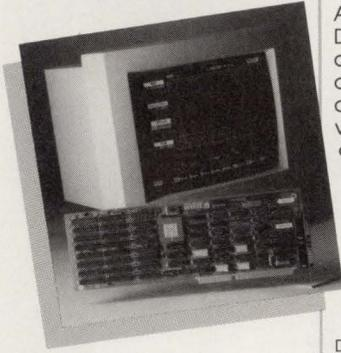
Start with the blazing speed of our DSP32C-based ZPB34 DSP processor board, then add the versatility of our upgraded **DSPay XL™** code development software. The unique combination forms one of the most powerful integrated DSP platforms available on an IBM® PC or compatible. Simple, painless, and powerful.
