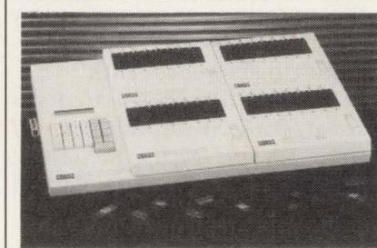
or multiple EEPROMs, or single or multiple sets can be downloaded into RAM and programmed simultaneously. The programmer features RS232-C and bidirectional-parallel I/O interfaces. \$4995. Delivery, four to six weeks ARO.
