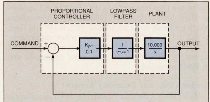
**Fig 2—This simple control system** consists of a proportional controller, a lowpass filter, and an integrating plant. The plant might represent an idealized motor or a mass in a frictionless system.  $K_P$  is the proportional gain, and  $\tau$  is the cutoff frequency in radians/sec.
