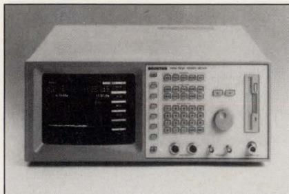
display-element color is user selected. Waveforms are digitized at a 1-MHz rate, and there's a dedicated DSP for high-speed measurements. Waveform data can be downloaded to a plotter.
