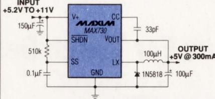
The **MAX730** is the smallest complete PWM step-down available. Its 8-pin SOIC package and all surface-mount external components fit into 0.55 square inches. It delivers up to 300mA from 5.2V to 11.0V inputs with 94% efficiency.
