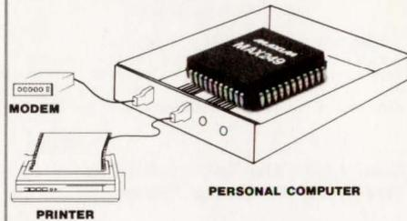
The **MAX249** has 6 drivers and 10 receivers — two complete Data Terminal Equipment (DTE) serial ports on one chip, making it ideal for space-critical applications. Plus, the MAX249 uses space saving 1µF capacitors and is guaranteed to operate at data rates up to 64kb/s.
