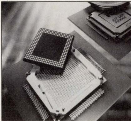
LGA device, a contact array, and an insulator-spacer. All of these components are sandwiched between a cover plate and a base plate. The insulator thickness is se-
