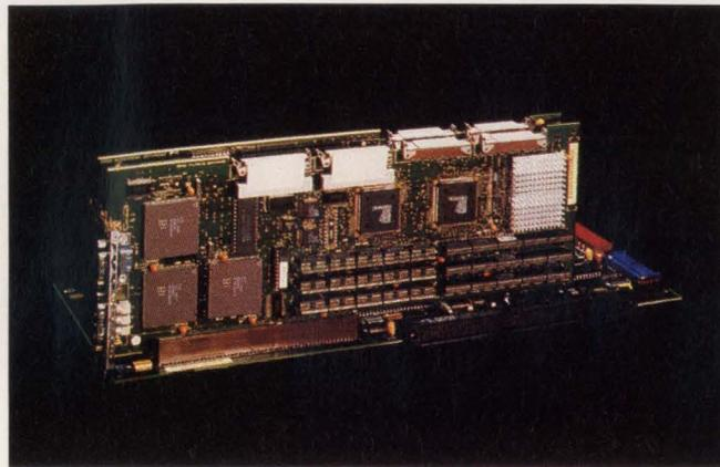
A typical multiprocessing DSP design is illustrated by the IBM GT4x graphics adaptor, which has six TI TMS320C30s in a 3-card subsystem. The adapter handles 2- and 3-D wireframes and 3-D surfaces with 1280 × 1024-pixel resolution.
