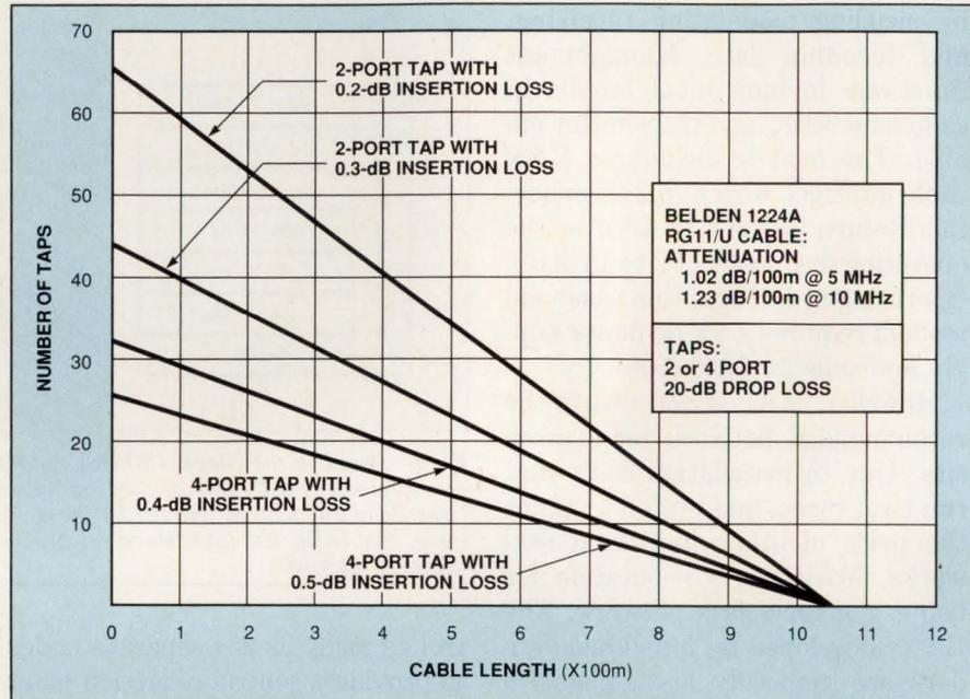
*This graph illustrates the relationship between carrierband cable length and the number of taps in a 5-Mbps network. Developed by IEEE 802.4 LAN design engineers at Motorola, it also shows that a 0.1-dB difference in insertion loss at each tap will significantly affect the number of taps a given length of RG11/U cable can accommodate.*
