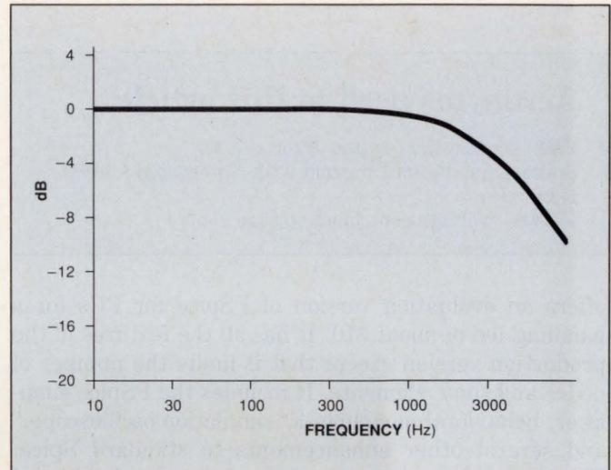
**Fig 7**—The Bode gain plot for **Fig 3**'s system, with a 2000-Hz filter, shows that the gain is flat to about 40 Hz; after that, the gain gradually declines. This plot indicates that the system is very stable.
