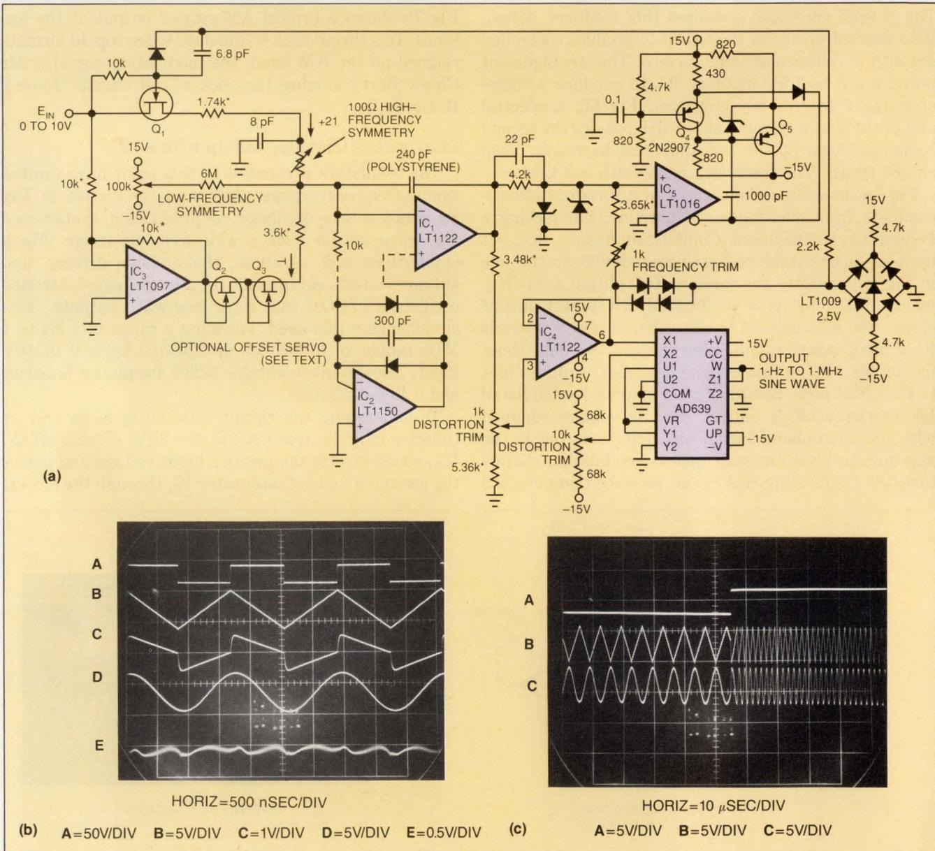
**Fig 8—A classic function generator, a, creates square and triangular waves whose frequency you can control with a dc voltage. A trigonometric-function generator IC converts the triangle to a sine. The traces in b show waveforms within the circuit. The lowest trace shows the residual distortion after you remove the output's fundamental-frequency component. In c, you see the circuit's quick and clean response to a command to change frequency.**
