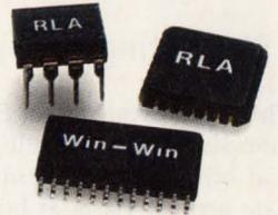
These Raytheon Linear Arrays (*RLAs*) act as a computer's early warning system. They monitor internal voltage levels to 0.3% accuracy—and signal a shut down before power surges can fry the system.
