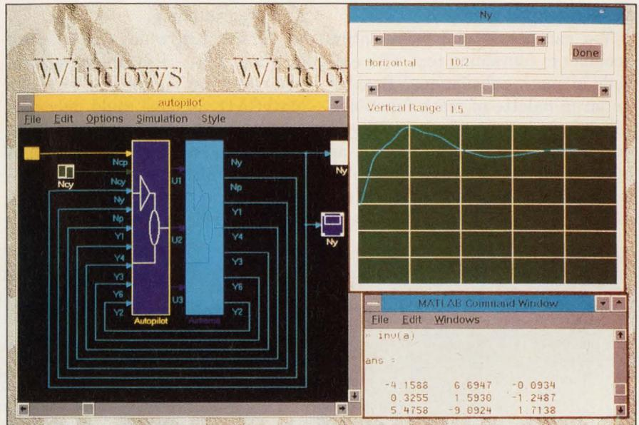
You can model linear and nonlinear networks having multiple inputs and outputs using Simulab, an extension to Matlab.
