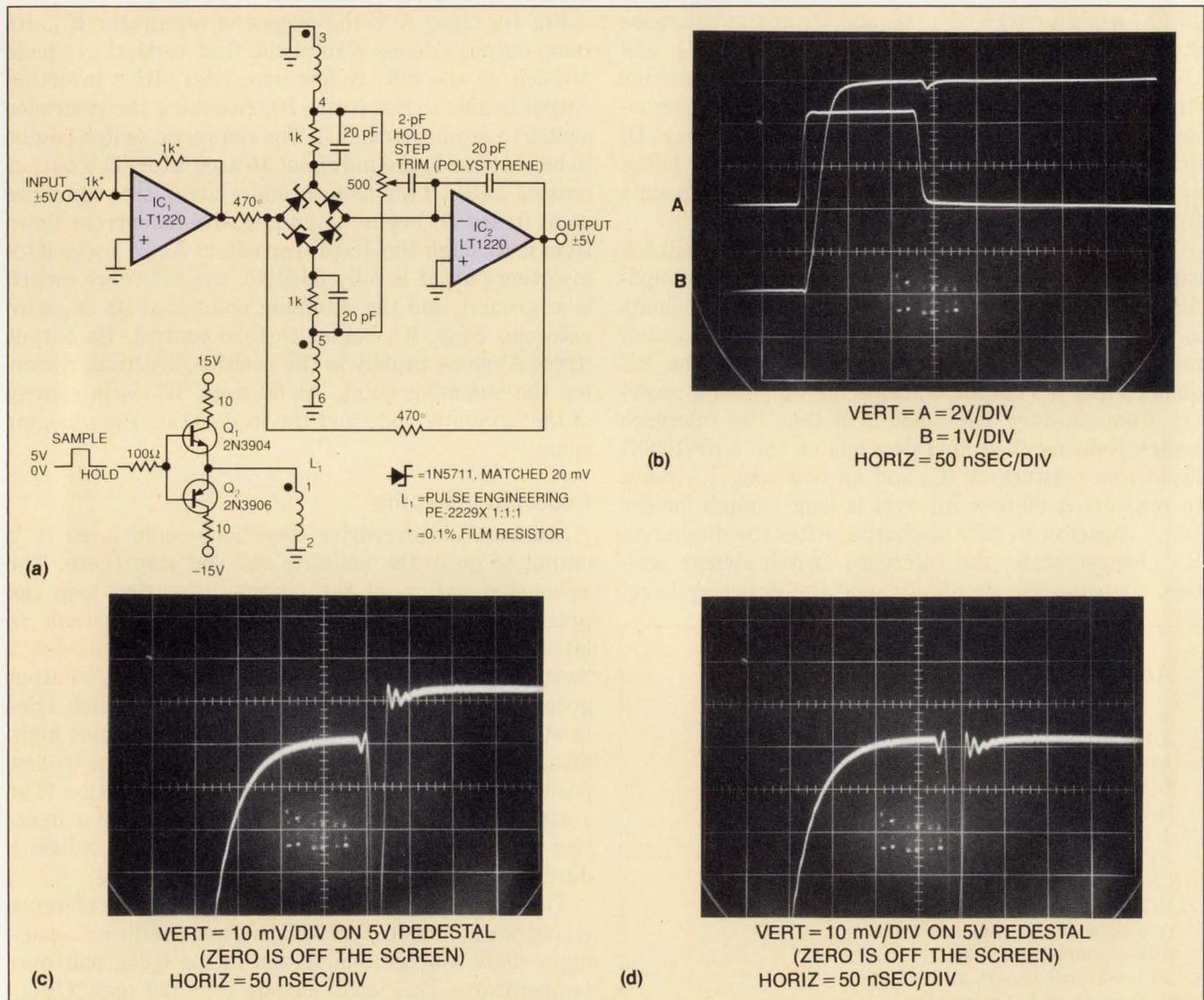
Fig 2—This very fast S/H circuit (a), acquires signals to 8-bit accuracy in 100 nsec. In b you see the waveforms within the circuit. Accurate operation depends on cancellation of the switching signals that feed through the bridge. In c, the compensation is disconnected. In d, you can see the effect of the compensation.
