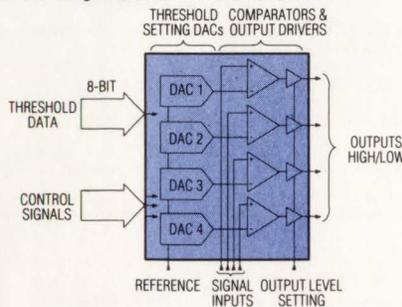
New **MAX516** automates calibration, minimizes part count with 4 BiCMOS comparators with DAC-programmed input thresholds in a single device. Features include 0.4% resolution, 1.5μs propagation delay and 50mW max power consumption.
