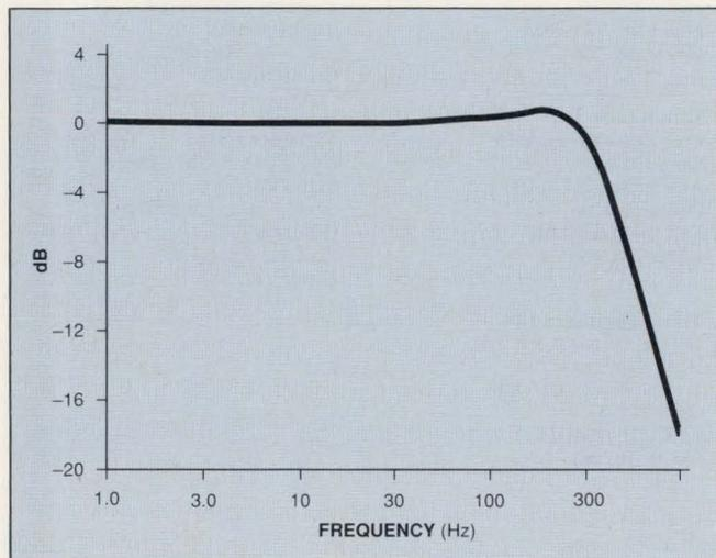
Fig 8—Additional peaking of about half a dB occurs when the filter's cutoff frequency is reduced to 200 Hz.
