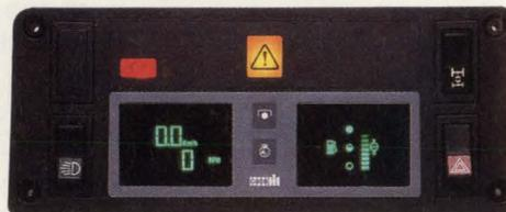
Electronic Instrument Panel to J.I. CASE Tractors.
