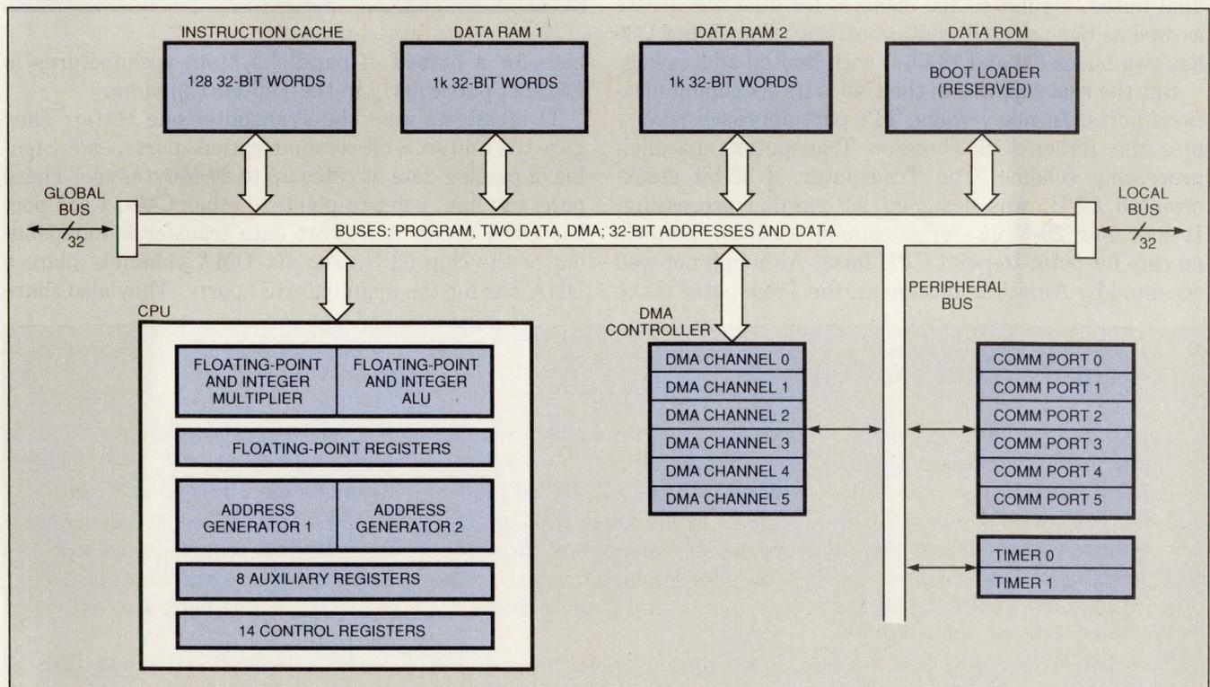
Fig 2—Featuring six communications ports and six DMA channels, Texas Instruments' TMS320C40 brings a new dimension to DSP multiprocessing. Designers can link multiple C40s point to point and move data as fast as 20 Mbytes/sec/port.
