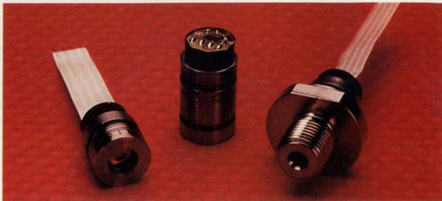
*Design flexibility is the primary advantage* offered by Novasensor's NPI pressure sensors. Capable of measuring pressures of 10,000 psi, the devices provide a 100-mV output, feature a  $\pm 2\%$  interchangeability, and are accurate to  $\pm 1\%$  over a 0 to 70°C operating range.
