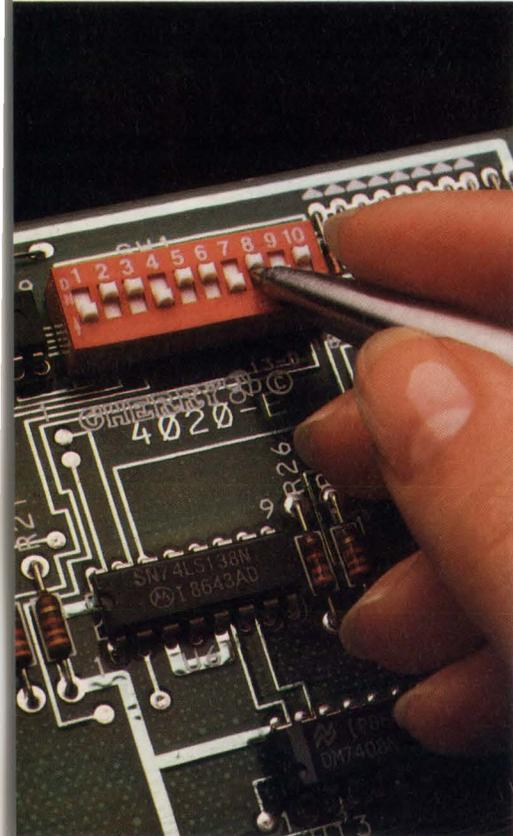
Changing DIP switches is a five stage process: disconnect the device, remove outer housing, reset the DIP switches, reassemble unit, and reconnect the device. Minimum downtime: 20 minutes.
