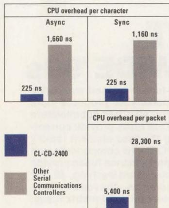
The CL-CD2400 has more intelligence for sophisticated error checking, special character matching, address recognition and automatic DMA management — with 1/7th the overhead\*.
