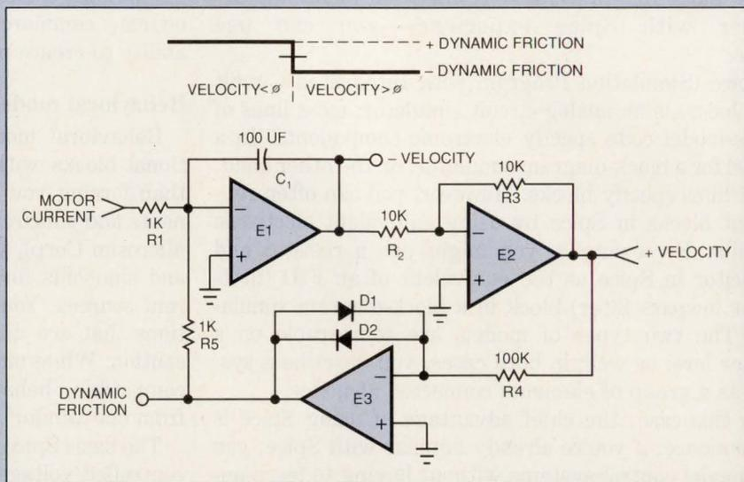
Fig A—This model of a servo motor with a frictional load uses an op amp with diodes in the feedback path to simulate dynamic friction.
