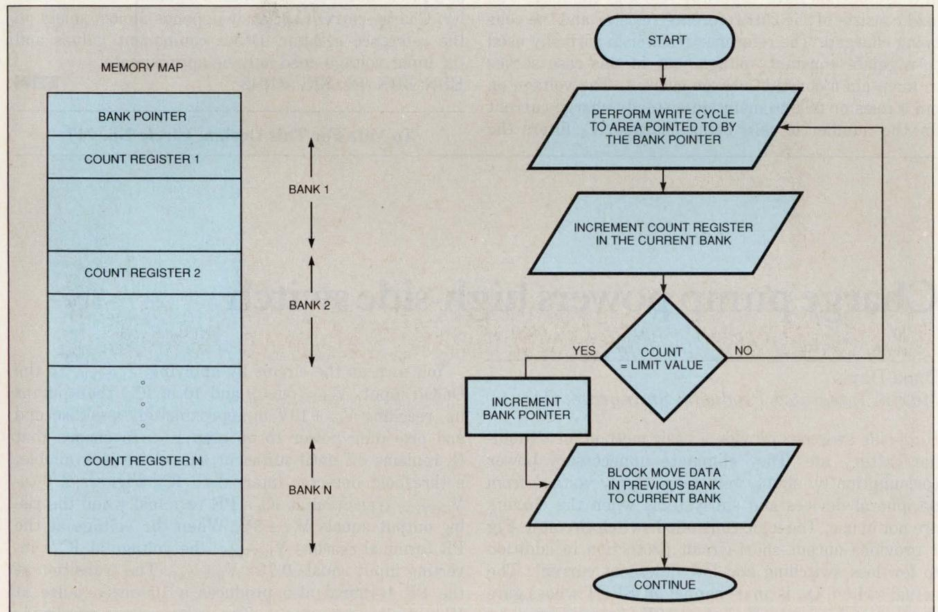
Fig 1—Creating  $N$  banks of memory extends an EEPROM write-cycle life by  $N$  times. The cost is the added memory.
