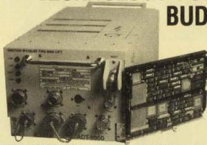
The SRT-5000 video tracking system is a non-developmental item (NDI), designed to provide high performance automatic tracking for many different scenarios. The modular VMEbus design features centroid, correlation and coast modes for dual-mode/dual-gate tracking. The open architecture allows for many other options. Commercial, ruggedized and military configurations are available.
