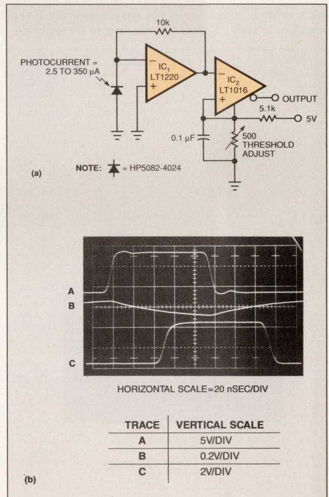
**Fig 3**—This simple optical receiver (a) has a fixed signal threshold. The outputs of IC<sub>1</sub> (b, trace B) and IC<sub>2</sub> (trace C) lag the input signal (trace A).
