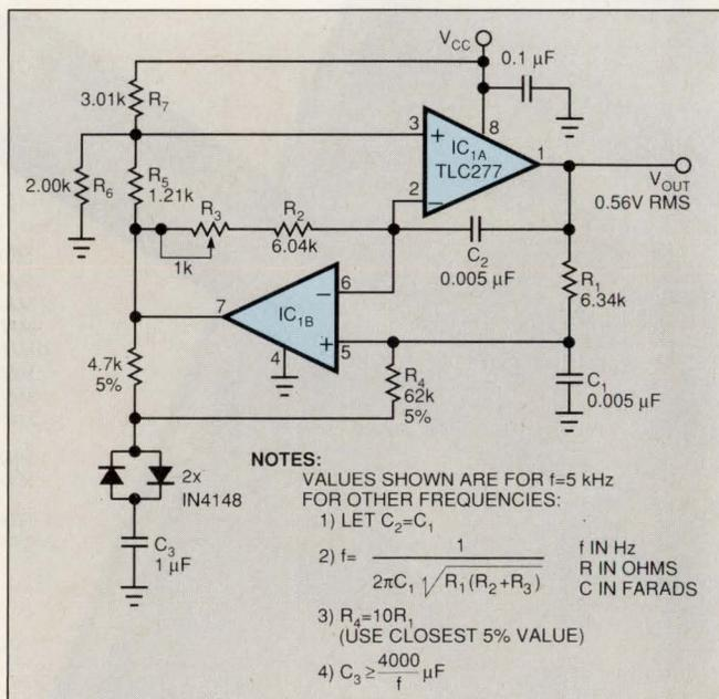
Fig 1—Based on a modified GIC bandpass filter, this 5-kHz sine-wave oscillator runs off 5V.
