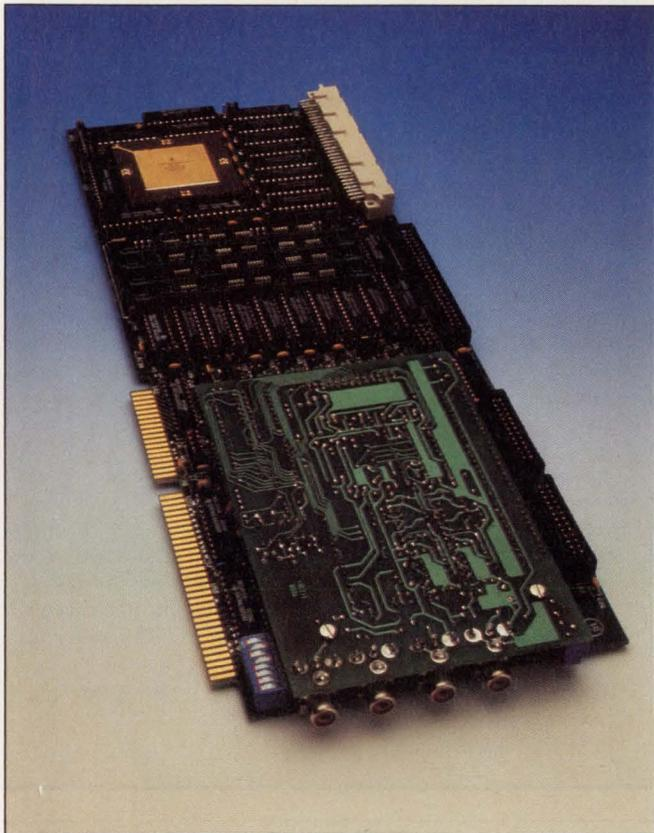
This PC plug-in DSP board has a peak performance of 60 Mflops, 64 Mbytes of DRAM, and a range of both input and output oversampling audio converters. Ariel Corp’s DSP-96 board is based on Motorola’s DSP96002 floating-point DSP processor.
