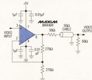
The **MAX404** video op amp has 0.01° differential phase and 0.05% differential gain while operating from ±5V supplies. Featuring 80MHz gain-bandwidth and 500V/μs slew rate, this amplifier is ideal for video and other high-speed applications. 50mA continuous output current is guaranteed.
