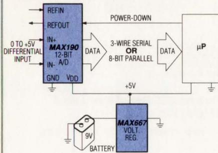
The **MAX190** converts rail-to-rail signals to either serial or parallel data in 7.5μs on battery power. Precision laser-trimmed reference, clock and track/hold included on-chip. The MAX190's already-low 15mW power consumption is reduced to 150μW during shutdown.
