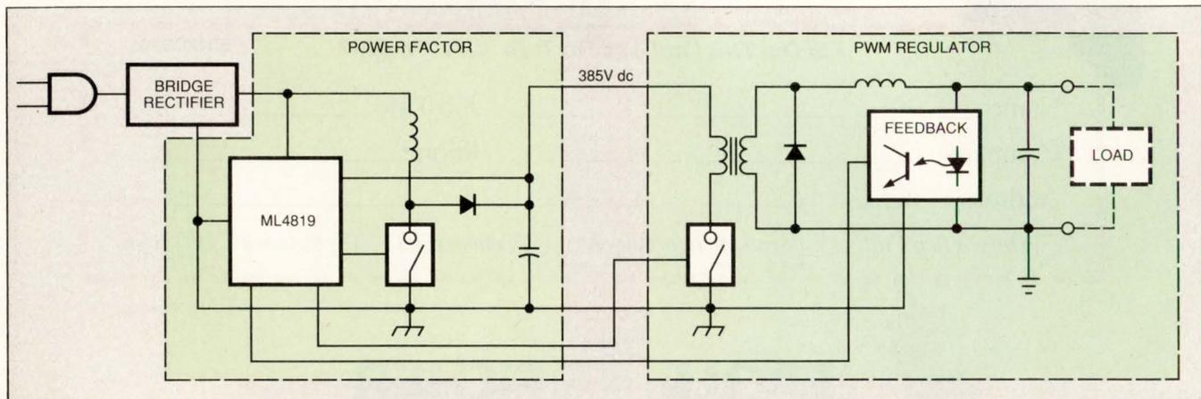
Fig 5—Combining PWM and power-factor controllers, the ML4819 from Micro Linear needs fewer components than other implementations.
