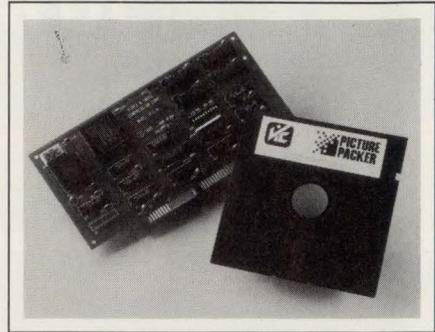
MS DOS 3.0 and later versions or Windows 3.0. It compresses full-color and gray-scale images using the proposed JPEG implementation standards and achieves compression ratios as high as 30:1. The software works with Targa, TIFF, PCX, and GIF file formats, and is compatible with existing desktop-publishing, presentation, animation, and word-processing programs. You can activate a memory-resident utility from within an application program to read a compressed file.
