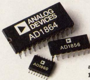
**Digital Audio Converters – The SOUNDPORT™ family of data converters comes complete with output amplifier, reference and digital logic interface. These mixed-signal ICs for high fidelity digital audio and multimedia applications achieve SNRs as high as 108 dB and THDs as low as 0.0025%.**
