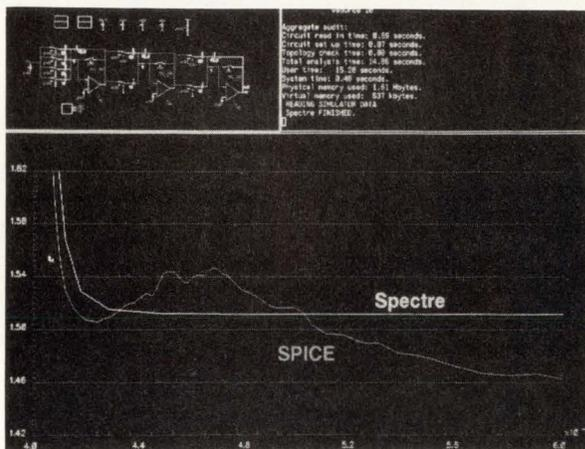
*Charge-conserving device models allow Spectre to produce more accurate results than Spice.*
