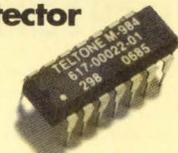
M-984 is a low-power 14-pin CMOS DIP that detects S.I.T.s (special information tones), OCC (other common carrier), dial tone (400 Hz), as well as many international call progress tones.
