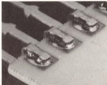
Precise amounts of the right solder and the shape of the "Claw" grip provide control of solder flow without a solder stop. This assures perfect mechanical and electrical bonding without wicking or bridging.
