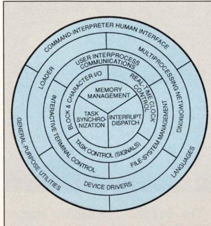
provides several priority-driven scheduling policies, including first in/first out. The timers in Lynxos go far beyond Unix timers and have nsec resolution for both absolute- and relative-timing operations. Lynxos 2.0 fully supports the Posix.4a threads concept as well as the thread model implied by Ada tasking.
