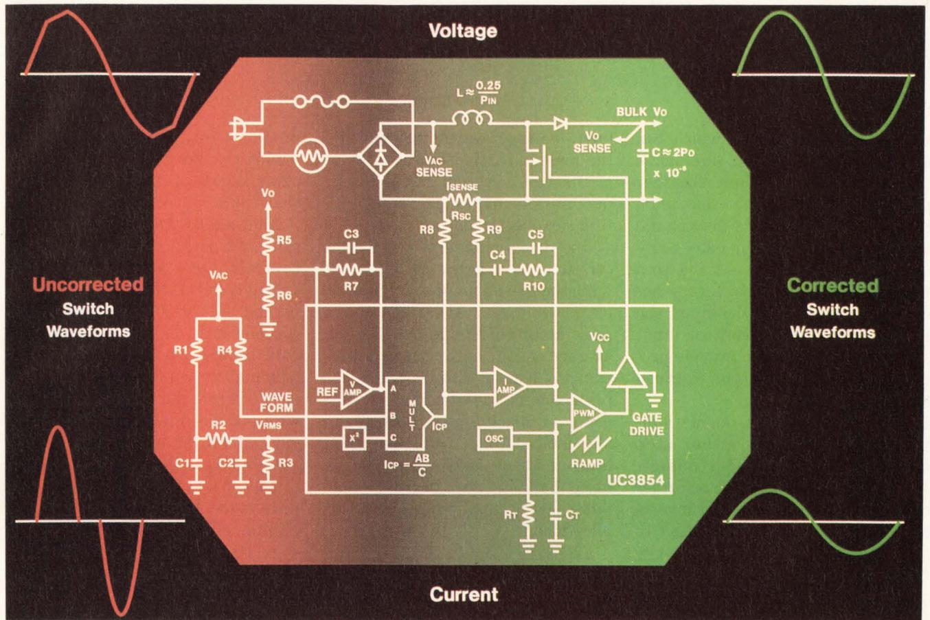
Because they don't deliver any power to the load, harmonics serve no useful purpose. Harmonics do, however, contribute to the total line loss, add to the current drain from the line, and dictate the need for higher-capacity wiring.
