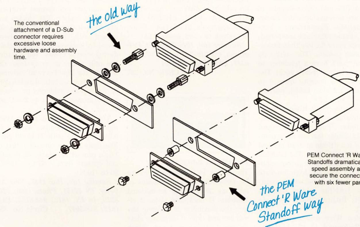
PEM Connect 'R Ware Standoffs dramatically speed assembly and secure the connector with six fewer parts.
