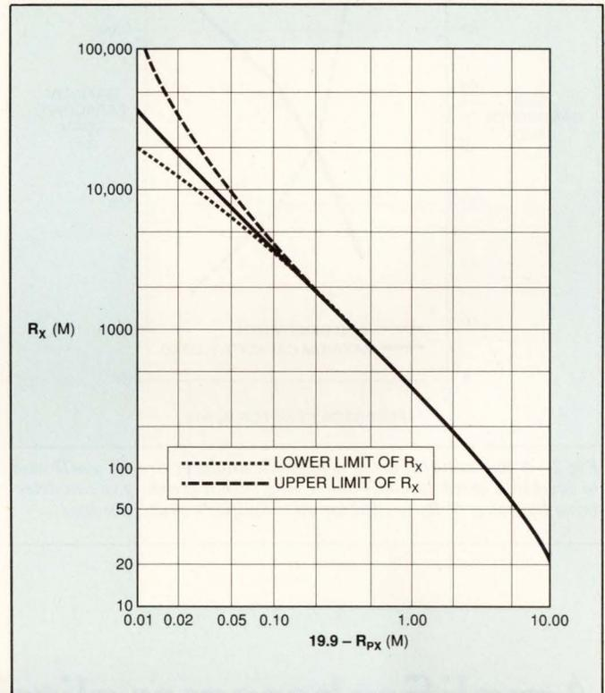
Fig 1—Using this chart and a high-value parallel resistor, you can measure resistances far beyond the range of your DMM.
