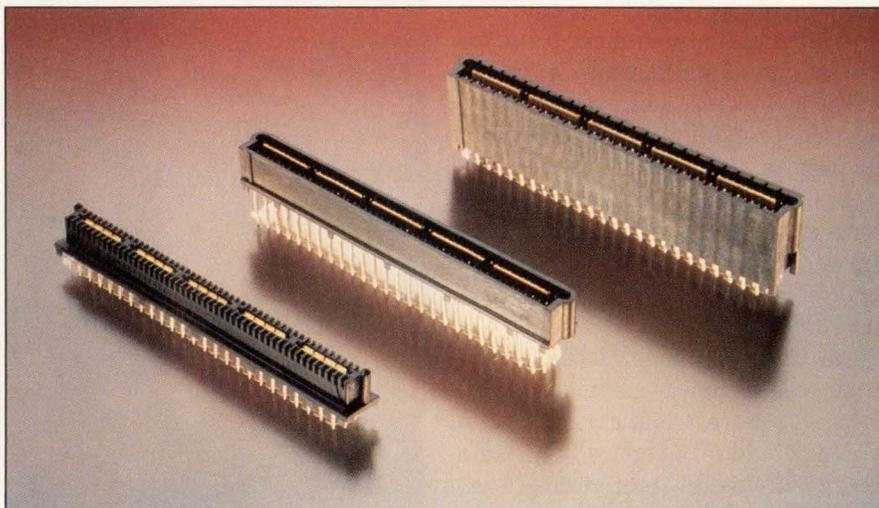
Capable of passing subnanosecond pulses with minimal noise and distortion, AMP's Micro-Strip connectors feature a contact design that presents a flat metal surface facing a ground plane. This design results in a controlled impedance transmission path.
