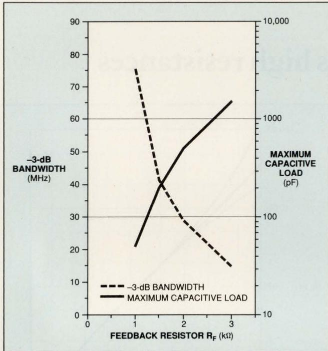
Fig 2—A few minutes using a network analyzer are all you'll need to develop a graph like this one. Using such a graph, you can determine the value of  $R_F$  needed for an amplifier's capacitive load.
