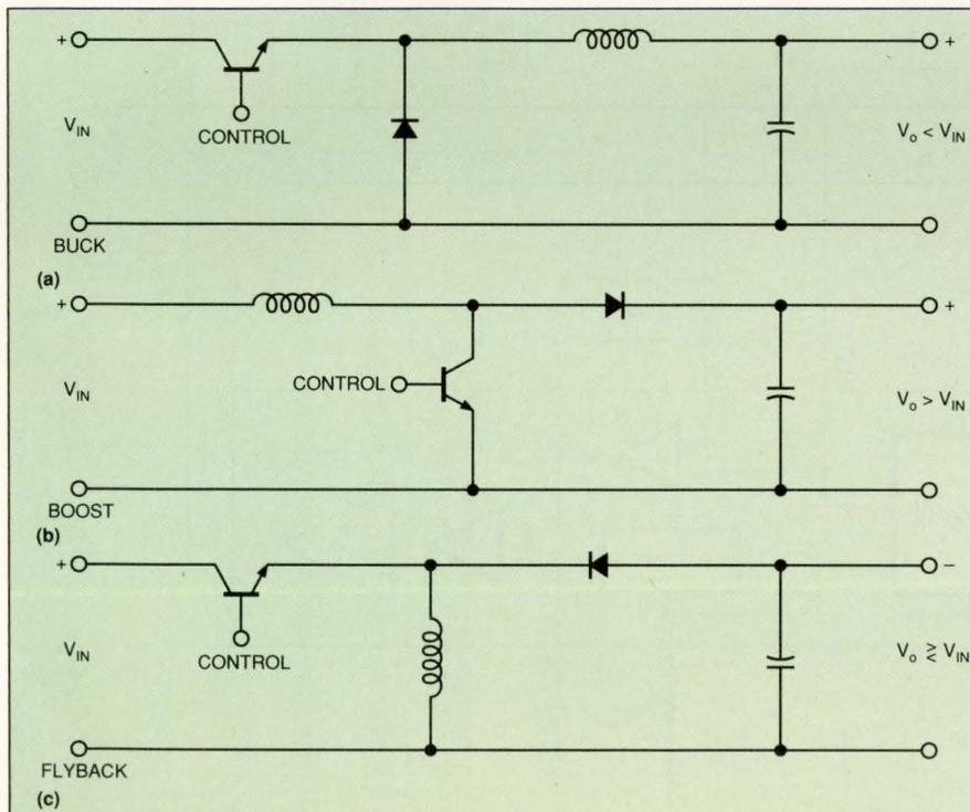
Fig 2—The three basic topologies used for power-factor correction are buck, boost, and flyback (buck-boost).
