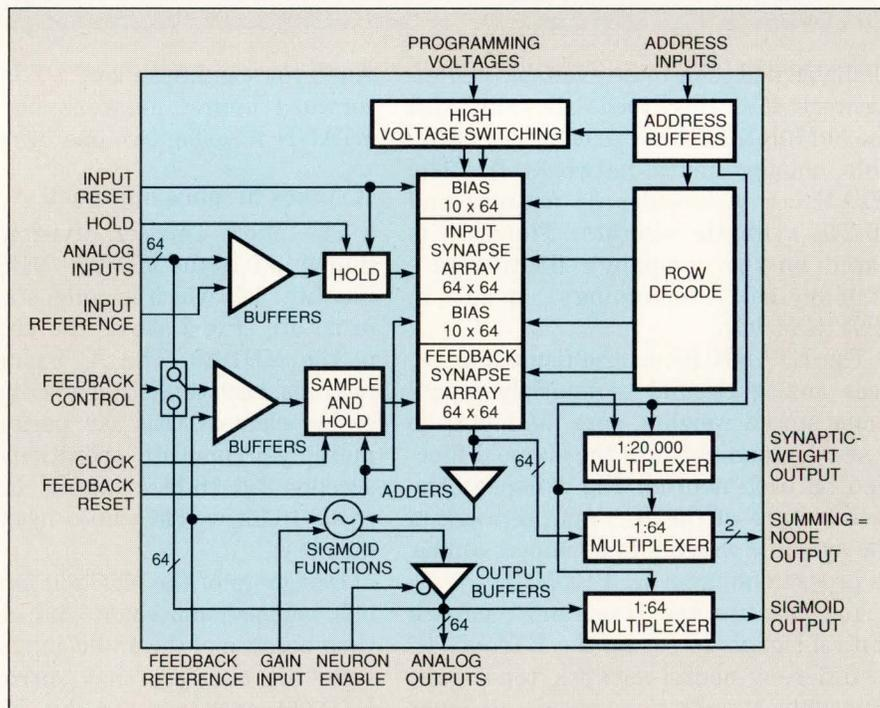
Fig 1—Based on floating-gate EEPROM technology, Intel's ETANN IC can store weights in memory cells. The chip uses analog circuits to perform multiply-accumulate operations.
