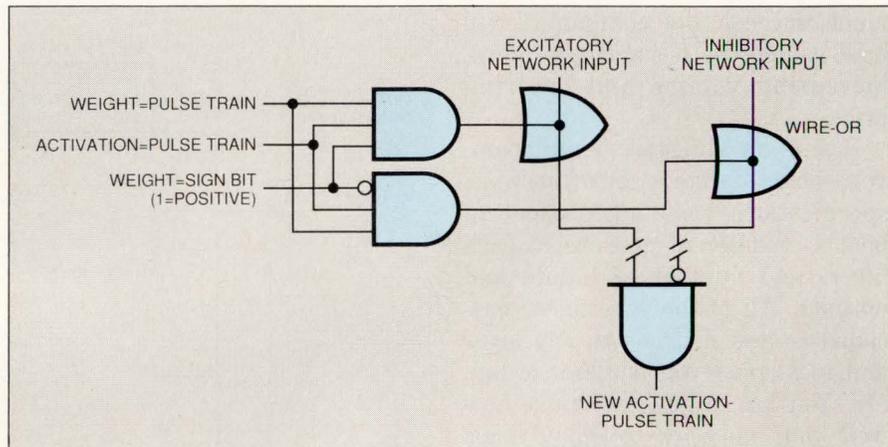
Fig 3—This multiply-accumulate model demonstrates how the NUSU32 IC from Neural Semiconductor uses pulse arithmetic to implement neural weights with less than 10 transistors per weight.
