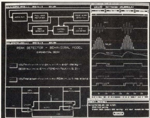
*Evaluate multiple-level circuit representations using Profile graphical and textual entry to the Analog Workbench II Spice-simulator.*
