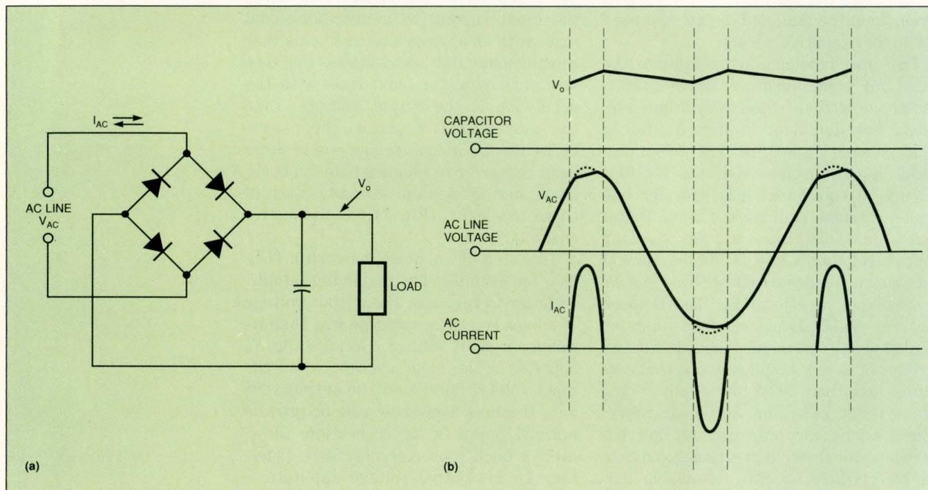
Fig 1—Power supplies using bridge-configured line rectifiers and a capacitor-input filter (a), draw current in a nonsinusoidal way (b). The full-wave rectifier charges the capacitor with pulses of current that occur only at the peak of each half cycle of the ac line voltage.
