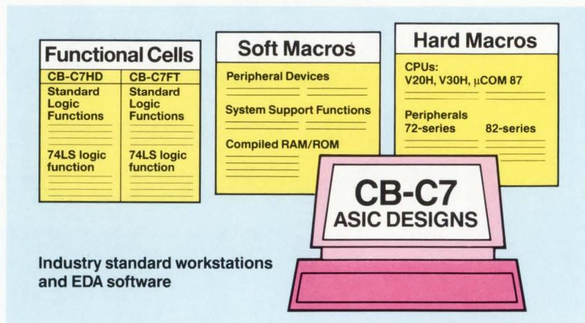
For example, the library of mega-function blocks contains cores of our μCOM87, V20H and V30H microprocessors, plus intelligent peripheral functions such as those provided by NEC's 72-series and 82-series standard peripheral devices. And because most of these megafunction blocks are hard macros, derived directly from the chip layouts of our standard parts, they have fully characterized timing parameters and can be tested with the standard part test vectors.
