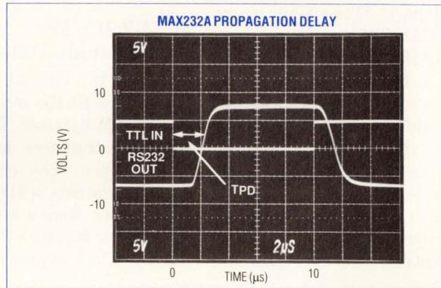
The MAX232A improves propagation delay and symmetry.
