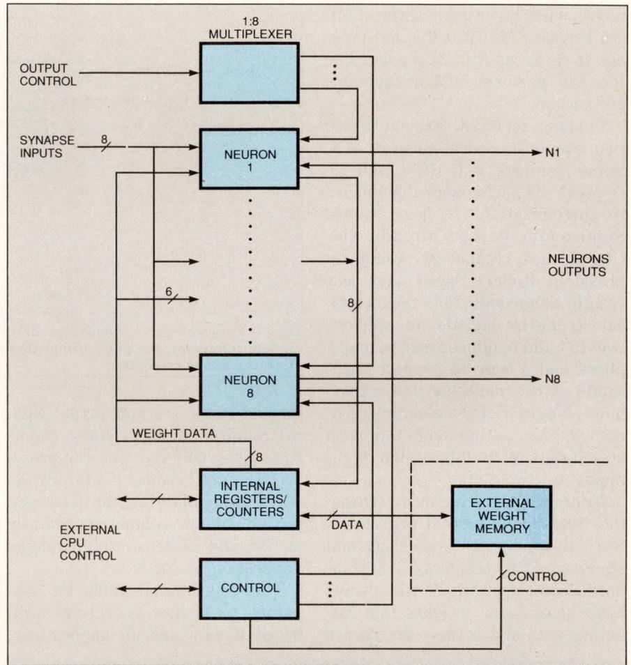
Fig 2—Eight neurons and 256 synaptic inputs make up the MD1220 neural-bit slice from Micro Devices. Via  $\mu$ P control, you can simulate large networks with a single IC, or you can cascade ICs and dedicate a neuron to every neuron in your model.
