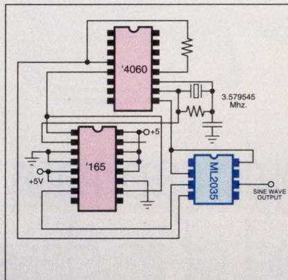
**60Hz Sinewave Output Using NTSC Color Burst Crystal**
