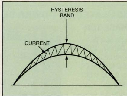
Fig 4—Using hysteretic current-mode control, the CS-3810 from Cherry Semiconductor generates a hysteresis band from a sinusoidal reference and an offset also derived from the reference. The average value of the waveform determines the inductor current.
