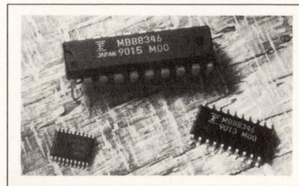
of the DAC accepts 2.5-MHz serial data. This data is loaded into internal data latches before the device converts the digital information into analog dc voltages in 60- $\mu$ sec settling time. The DAC provides a serial data output that allows you to cascade devices. In 20-pin DIPs and SOJs (small outline J-lead) plastic flatpacks, \$4.50 (1000).
