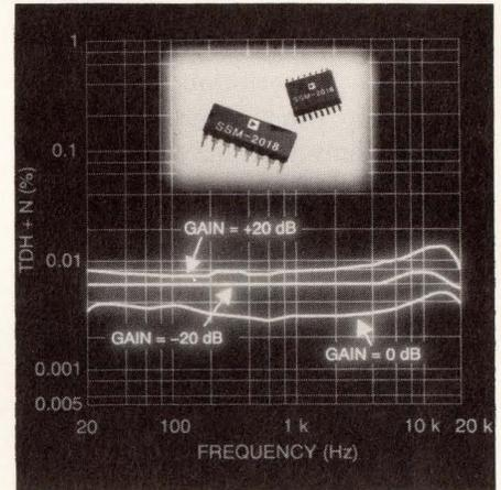
*Able to operate in either class-A or class-AB mode, the SSM-2018 voltage-controlled amplifier exhibits low THD + N over the 20-Hz to 20-kHz audio range.*
