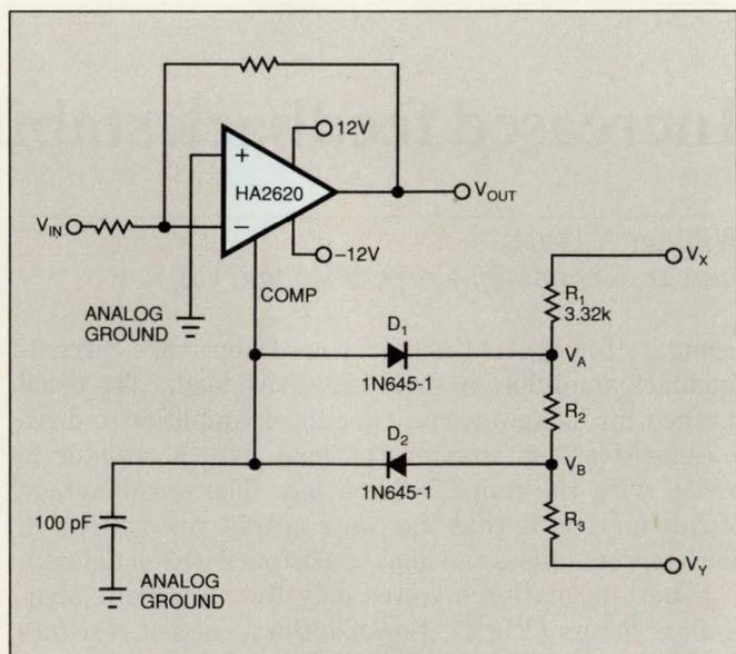
Fig 1—By putting the 2620 op amp's isolated bandwidth-control (COMP) pin to a novel use, the resistor-diode clamping network transforms the amplifier into an amplifier/clipper.
