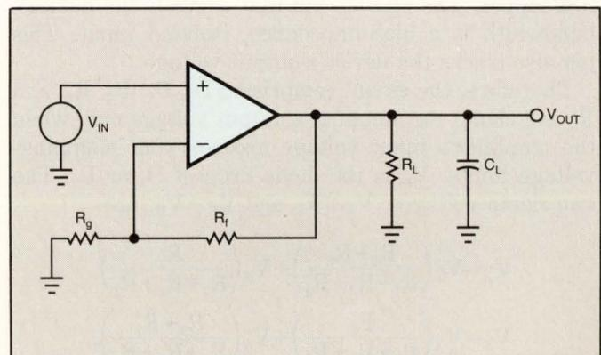
Fig 1—By adjusting the value of  $R_F$ , the feedback resistor that determines a current-feedback amplifier's bandwidth, you can optimize your circuit to drive almost any capacitive load.
