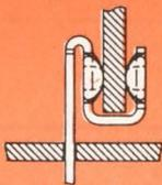
Preforms on edge clip terminals contain precisely the right amounts of the proper solder and flux for each application, and the exclusive NAS "Claw" grip holds each preform. This unique grip design provides direct contact between solder and conductor pads, a beneficial wiping action as clips are attached, and positive control of solder flow.
