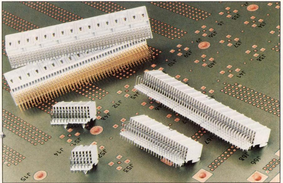
A modular system based on 2-mm centers, AT&T's Metral interconnects feature a basic building block that is 12 mm long and 4 rows wide. The modules are available in 4×6, 4×12, 4×24, and 4×48 sizes and are designed to stack end-to-end on a card edge or backplane without loss of positions.
