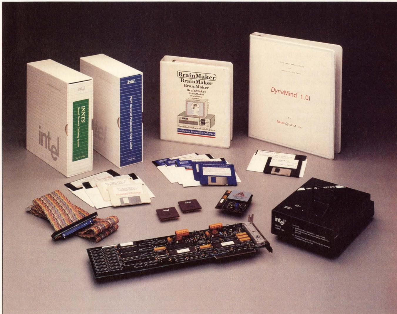
available and soon-to-be available neural-network ICs. Intel leads the way with the 80170NX ETANN (electrically trainable, analog neural-network) IC. The ETANN chip includes 64 neurons and 10,240 synaptic weights. The chip is based on the company's floating-gate memory-cell technology used in EEPROM ICs.
