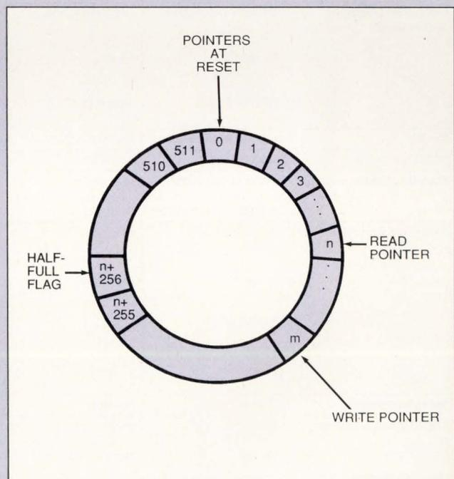
**Fig A**—Operating as a circular stack, the FIFO memory's pointers keep track of current data. Only 2 bytes remain in the FIFO memory, regardless of the write pointer's absolute value.
