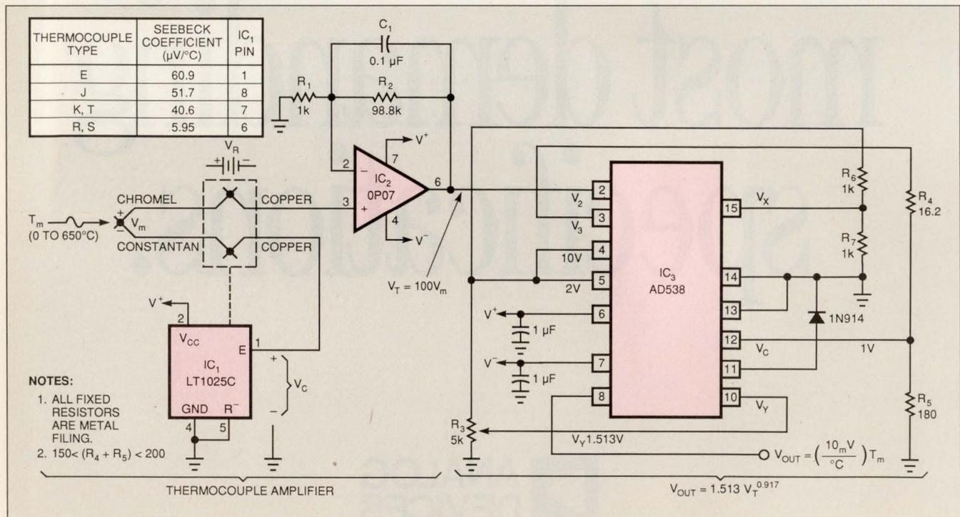
Fig 1—A cold-junction compensator, amplifier, and a computational IC linearize a type-E thermocouple with the help of a calculator's curve-fitting algorithm.
