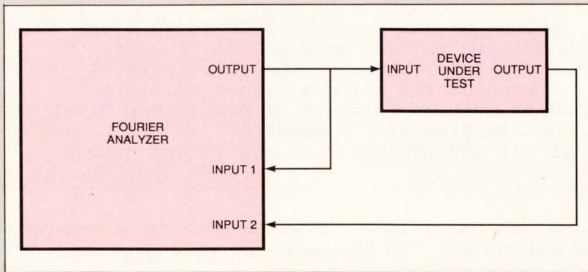
**Fig A**—A Fourier analyzer derives a frequency-response plot from the Fourier transforms of the input and output waveforms of the device under test.
