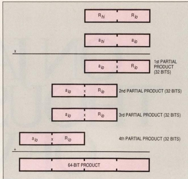
Fig 1—Computing a 64-bit product of two 32-bit numbers with a 16-bit, 2's-complement multiplier complicates the algorithm.
