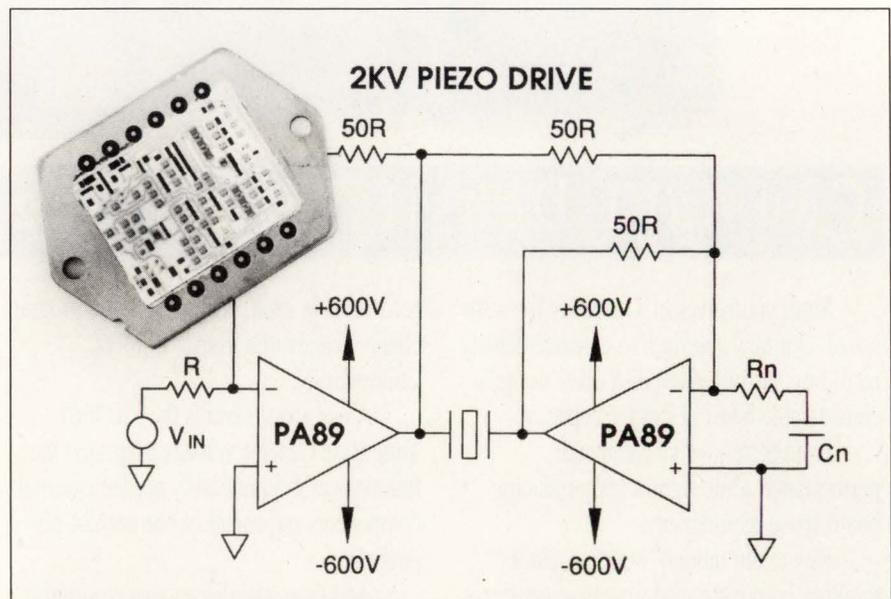
**Fig 4—This highly specialized power op amp from Apex Microtechnology is rated at 1200V. Applications include piezoelectric drive and electrostatic deflection.**
