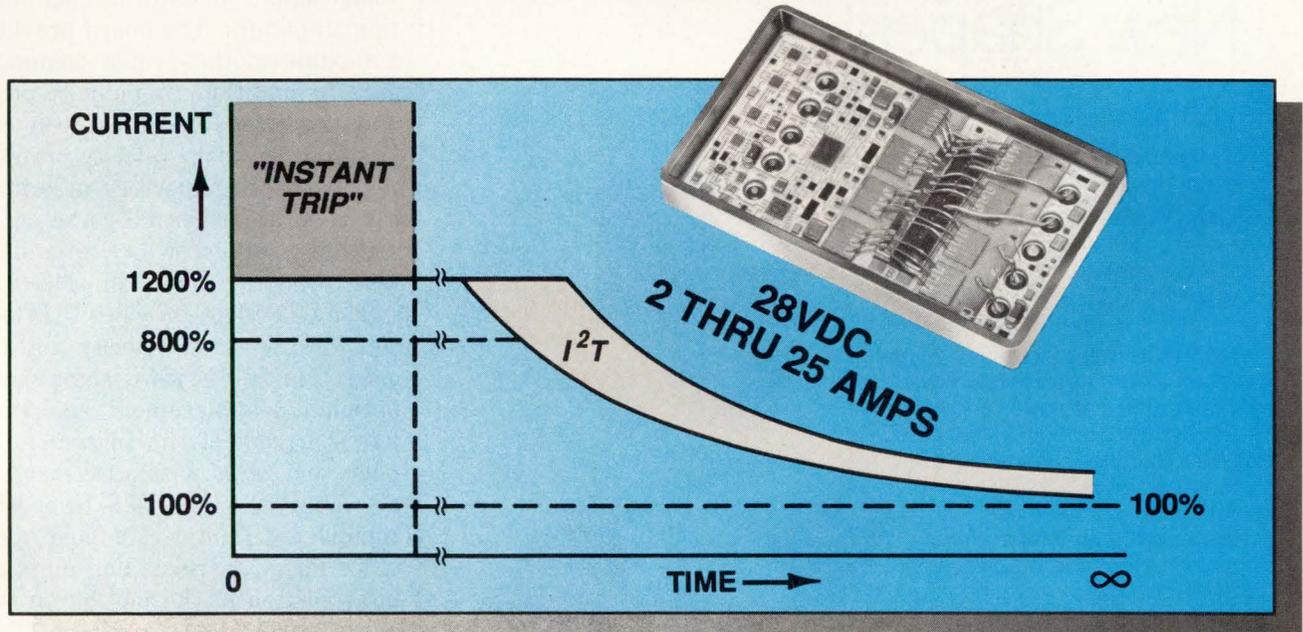
Solid-State Power Controllers (SSPCs) replace electromechanical circuit breakers in land, sea, air, and space vehicles. They provide status outputs and permit logic input control. DDC's 28 Vdc, SSP-21110 series, can be remotely located near the load because of the digital controls they support. The series offers five models, differing in rated current, so that fault ("instant trip") and true  $I^2T$  trip characteristics can be selected to protect wiring and loads.
