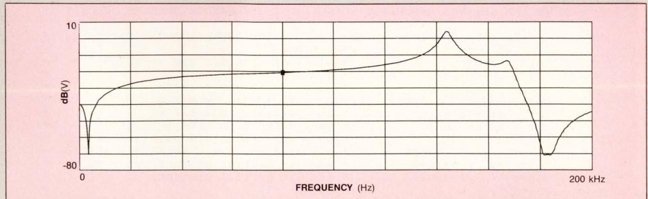
**Fig C**—A swept-sine analyzer's result is nearly identical to the Fourier analyzer's but takes much longer to derive.
