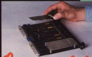
You can configure it with just the right amount of RAM and ROM you need. And you do not have to sacrifice features. Our Omnimodule™ modular I/O connector allows you to implement a wide variety of serial, parallel, SCSI, GPIB, analog, digital and other I/O options - all fitting into one slot. Other features include:
