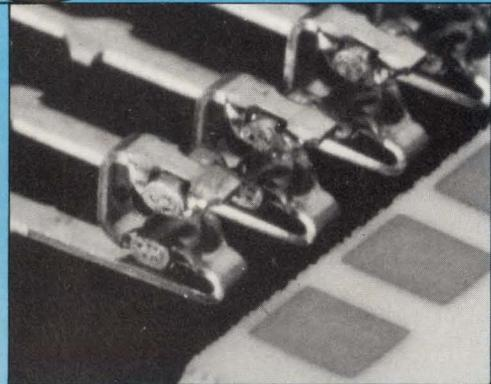
Interference fit holds clips firmly in position for reflow. Top and bottom preforms are reflowed in one operation.
