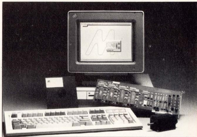
*Many boards employ commercially available motor-control ICs. The MC series of boards from Motion Engineering employs a Hewlett-Packard HCTL-1000 that receives instructions directly from the ISA bus host computer.*
