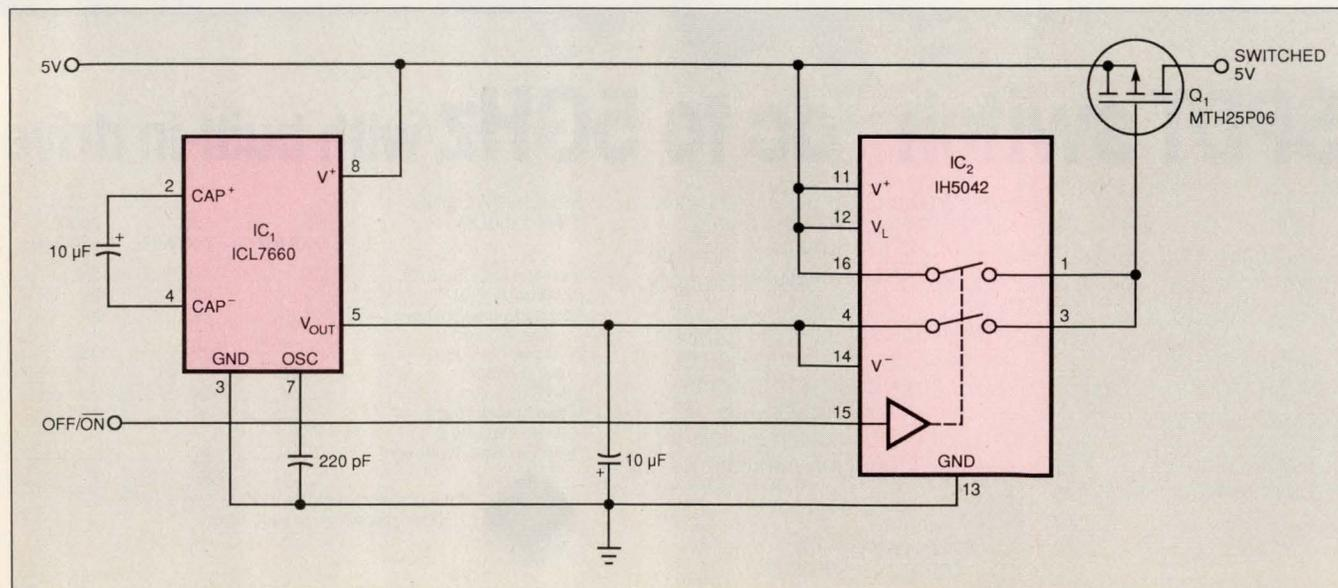
Fig 1—This circuit provides 5V under external control, exhibiting 100-m $\Omega$  on-resistance when on and 10  $\mu$ A of quiescent current when off.
