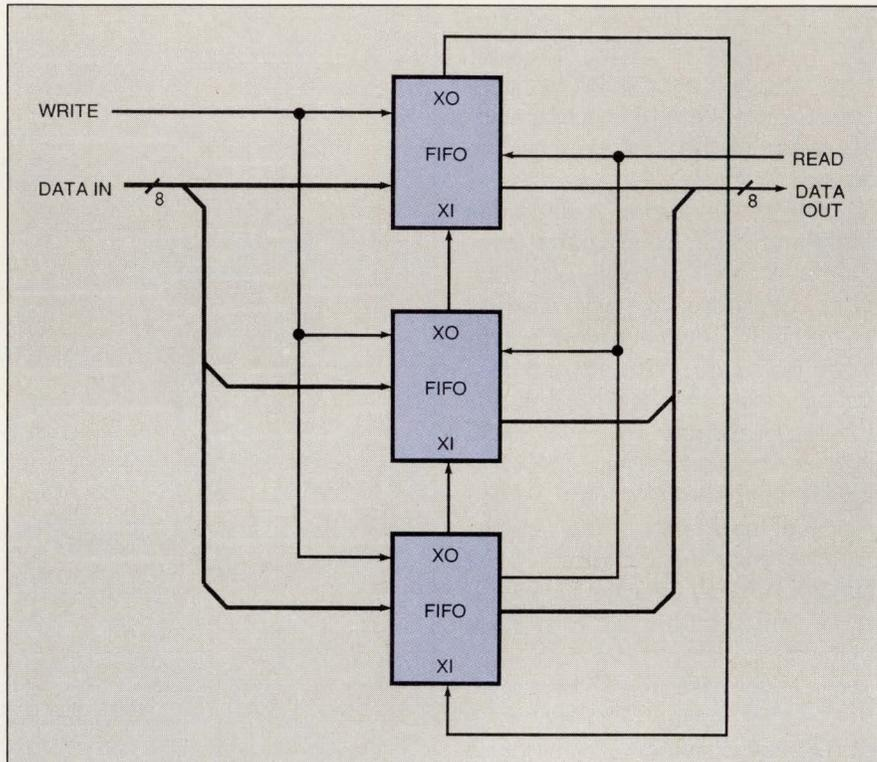
Fig 2—If you need to add more depth to your FIFO memory buffer you'll have to connect the devices in a daisy chain as shown. Doing so, however, can exact a performance penalty and adds loading to the data buses.
