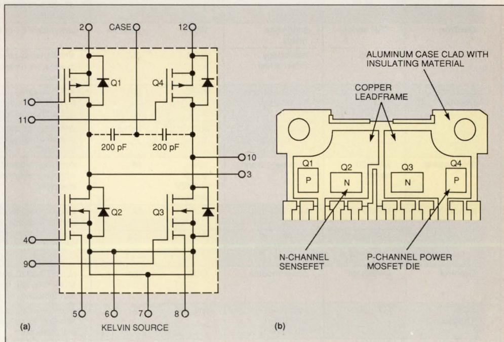
**Fig 1**—This H-bridge driver is rated at 100V and 8A. The MPM3002 circuit (a) from Motorola contains two n-channel and two p-channel power MOSFETS. Packaged in the company's 12-pin Icepak (b), the module has a power-handling capability of 62.5W.
