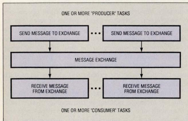
Fig 1—The message exchange—message buffers or mailboxes—allows multiple “producer” tasks to communicate with multiple “consumer” tasks.
