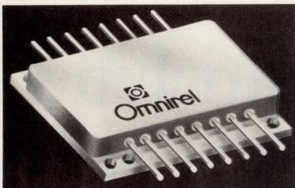
**Fig 2**—This 16-pin hermetically sealed package is used for Omnirel's OM9011SF. The power hybrid IC contains four n-channel MOSFETs, four Schottky diodes, and four high-speed rectifiers.
