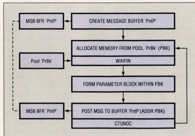
Fig 2—A typical producer task requests allocation of memory for a parameter block that will contain information the task needs to convey. The task waits (WAITFIN) for the OS to allocate the memory, then posts the parameter-block address to a message buffer and continues with no coordination (CTUNOC).
