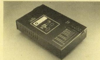
PILOT-144: Powerful PC-driven 40-pin programmer supports E/EPROMs up to 40-pins. Standard parallel port interface means fast thru-put and no need to install high voltage cards inside your PC. Built-in power supply. Upgradable to support 875x and 874x micros. \$795. SATISFACTION GUARANTEED.
