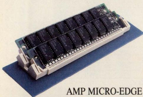
**AMP MICRO-EDGE SIMM sockets provide the highest security your memory or logic module could ask for: Each contact produces 200 grams normal force on each module pad. Minimum.**
