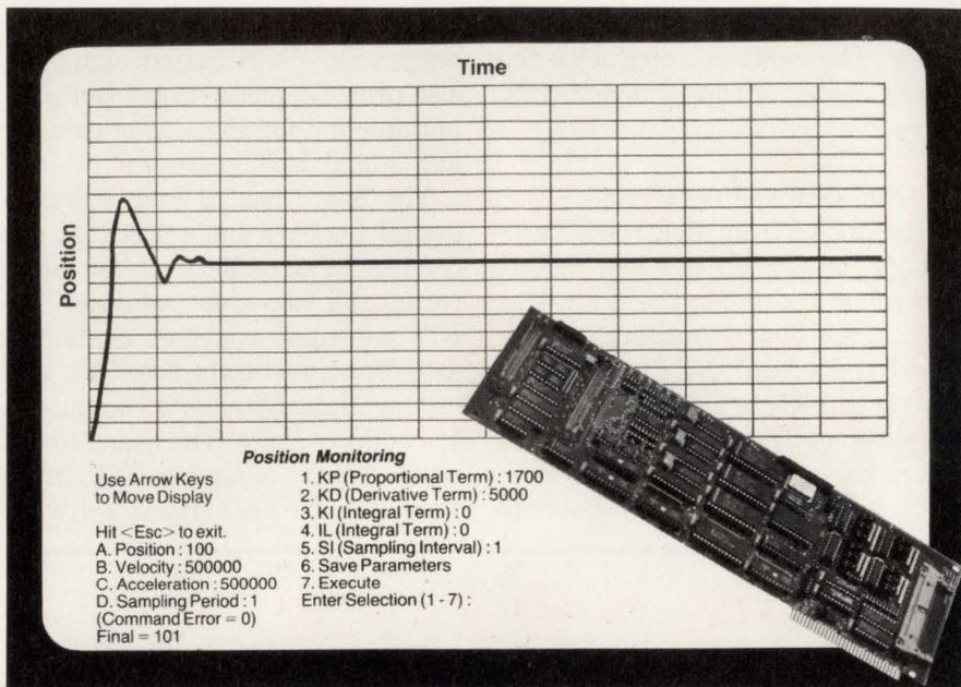
*Motor-control boards come with software to optimize servo-performance. The software for Technology 80 Inc's 5638 ISA bus board lets you observe the loop step response while you adjust the coefficients for a PID loop filter.*
