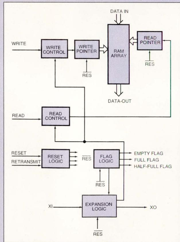
Fig A—Present-day FIFO memories are RAM-based, using pointers to keep track of data. The RAM-based architecture eliminates the "bubble-through" time required by earlier register-based devices.
