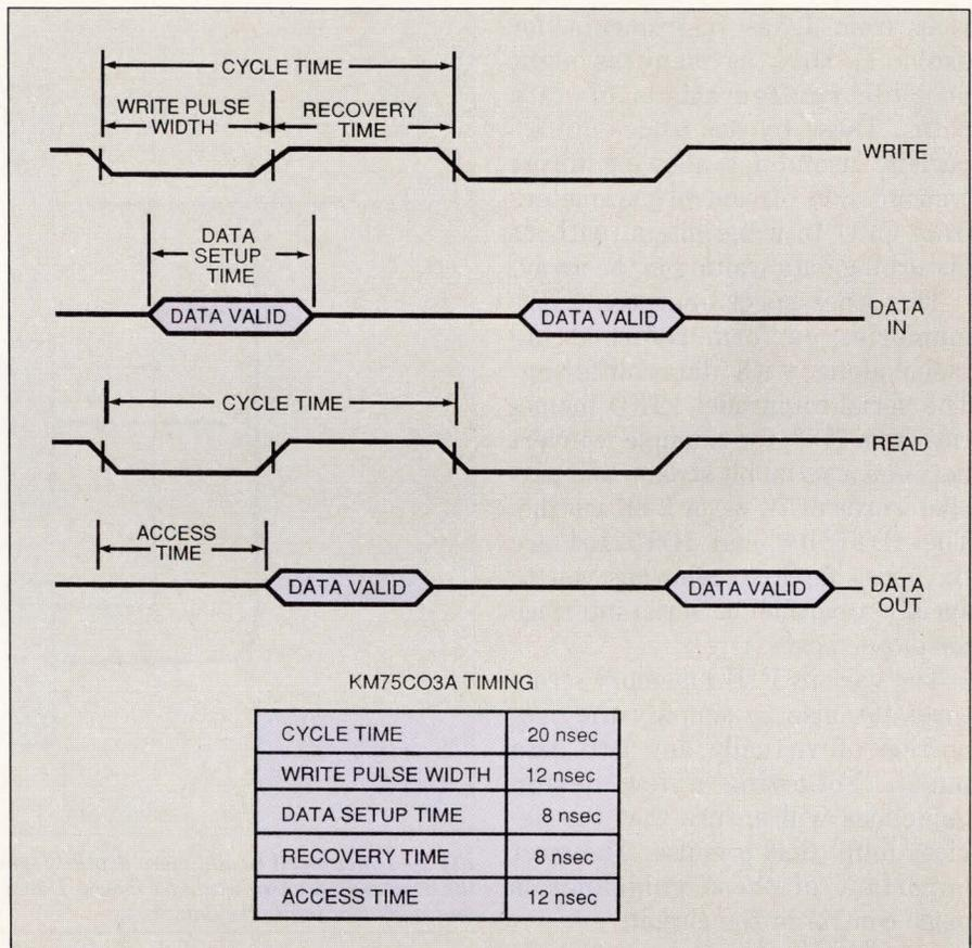
**Fig 1—Timing becomes critical at high speeds** when writing to asynchronous FIFO memories. The data setup time is nearly as long as the device's cycle time.
