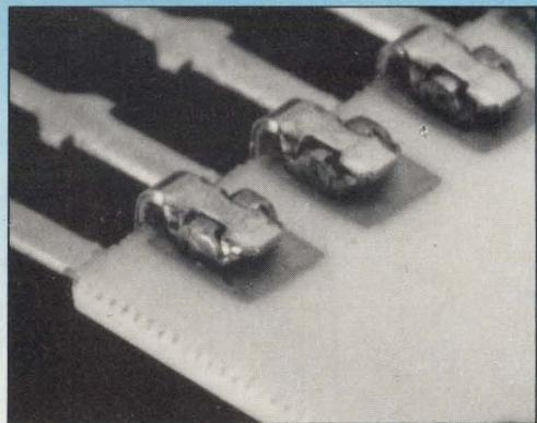
Precise amount of solder and the shape of the "claw" grip control solder flow without a solder stop. This assures perfect mechanical and electrical bonding without wicking or bridging.
