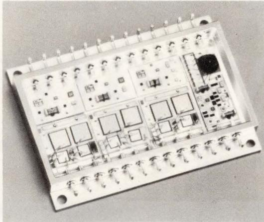
**Fig 3—This 3-phase, smart-power motor driver from ILC Data Device Corp meets MIL-STD-883C standards. In addition to digital control and protection circuitry, the hybrid IC contains six n-channel MOSFETs and six fast-recovery diodes.**
