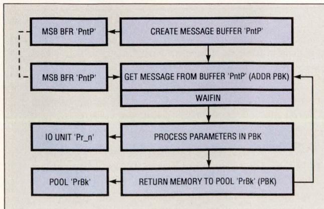
Fig 3—A typical consumer task receives the address of information (a parameter block) from a message buffer, then processes the information and returns the parameter-block area to a memory pool.
