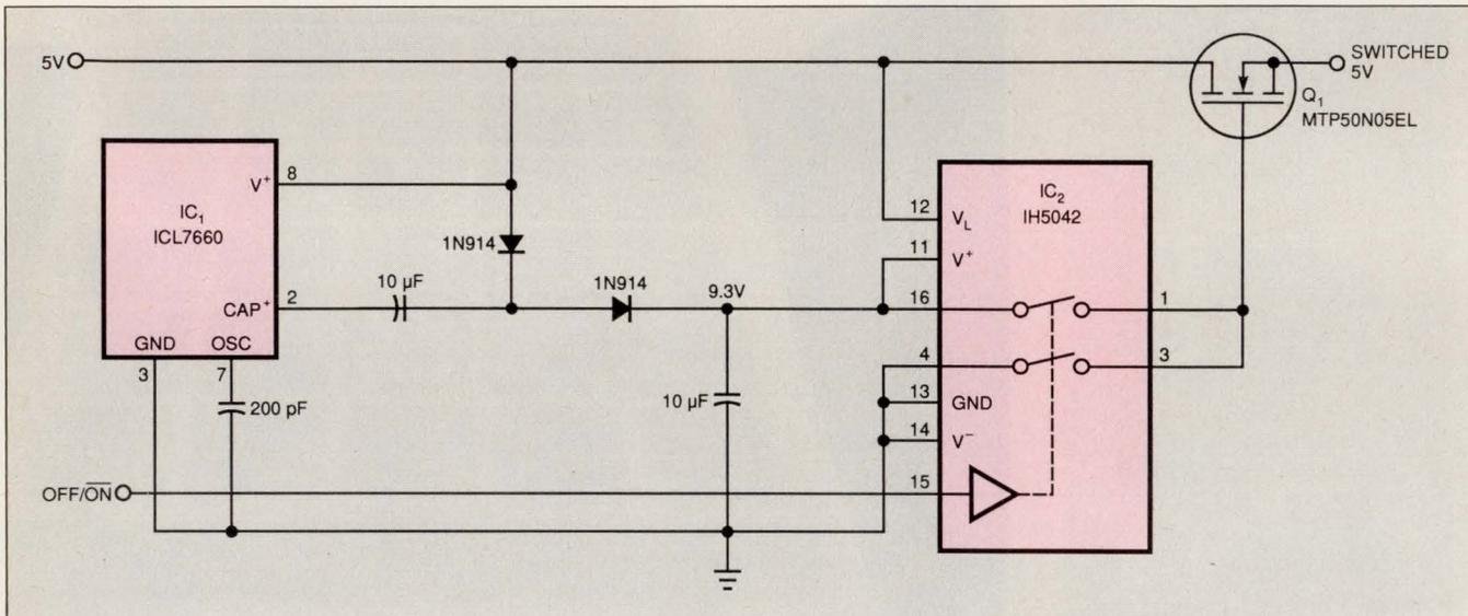
Fig 2—Employing a logic level n-channel MOSFET, this circuit switches the 5V supply and exhibits a 30-m $\Omega$  on-resistance.
