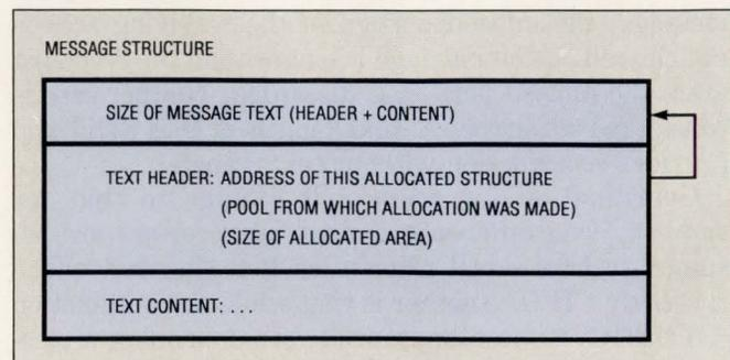
**Fig 7**—Avoid “dangling references” by having the sending task explicitly allocate a message area from a common memory pool. A message header or preamble supplies the address, plus the pool identification and allocation size.
