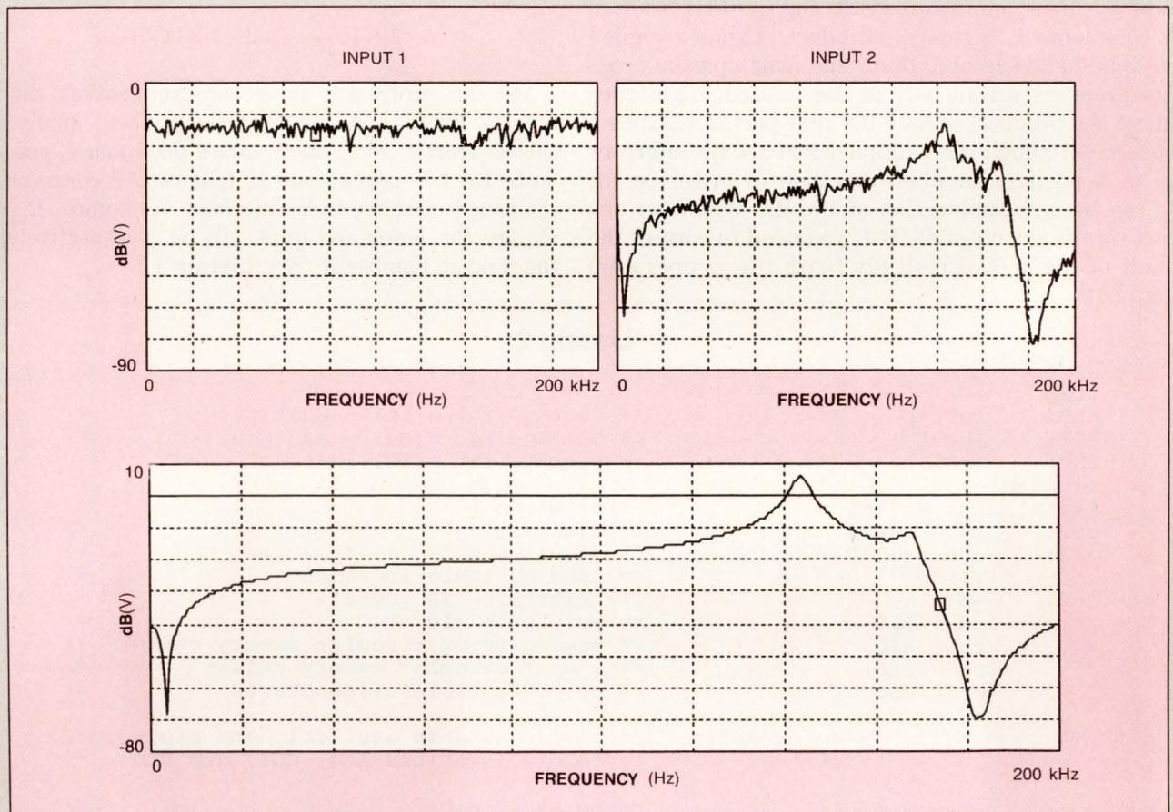
**Fig B**—A Fourier analyzer derived the lower frequency-response plot from the upper two input and output waveforms.
