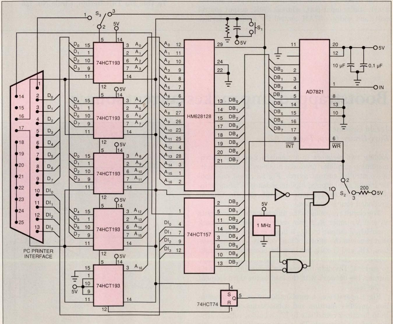
**Fig 1**—Using a fast ADC and an SRAM controlled by external logic, you can input analog data into your IBM PC that takes full advantage of the ADC's sampling rate.
