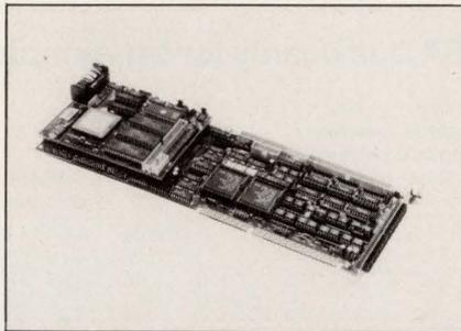
*For fast loop sampling times and complex motion profiles for many axes, consider a board that uses a DSP chip for motion control. The PMAC boards for the ISA bus and VMEbus from Delta Tau Data Systems employ a DSP56001 IC. The boards can be daisy chained to synchronize as many as 128 axes and update the servo loop in as little as 50  $\mu$ sec.*
