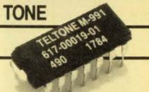
**M-991** generates precise dial tone, busy tone, reorder tone, ringing, and other call routing tones for use in telephone systems, test equipment, callback security and other telecommunications systems.
