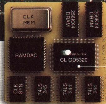
This full 16-bit CL-GD5320 lets you implement 16-bit or 8-bit VGA capabilities on your motherboard with as few as 5 other chips and two 256K x 4 DRAMs. Get a complete solution that saves time, space, power, and expense. You still get all the speed, features and flexibility you're looking for.
