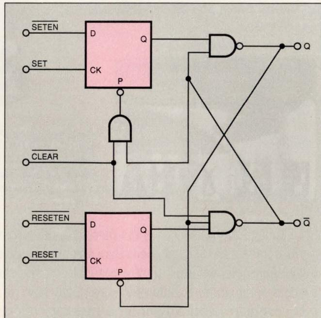
**Fig 1—This circuit forms an edge-triggered, set-reset flip-flop.**
