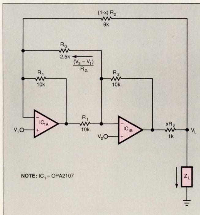
Fig 1—A voltage-controlled current source results when you combine an instrumentation-amplifier structure with bootstrap feedback.
