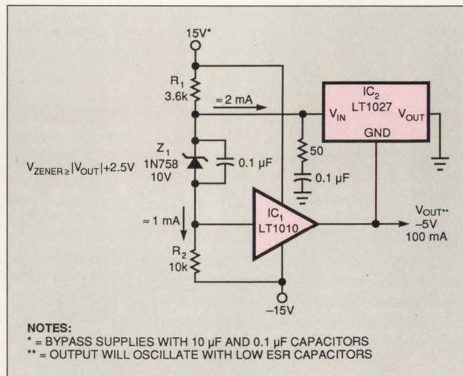
**Fig 1**—A power buffer, IC<sub>1</sub> in the feedback loop of a negative voltage reference, IC<sub>2</sub>, boosts the reference's output current to 100 mA.
