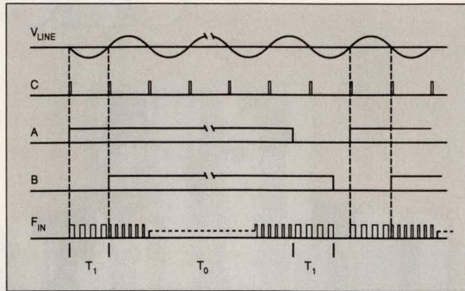
**Fig 2—Depending on the state of the outputs of a pair of counters, the circuit integrates (counts up) either the output of the V/F converter or the output of the V/F converter divided by two.**
