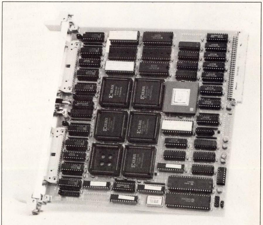
*Designing custom parallel interfaces based on the MB2-PGA56T board simply requires you to program gate arrays. The Multibus II-compatible board includes a local 8086  $\mu$ P, 128k bytes of RAM, and 128k bytes of EPROM.*
