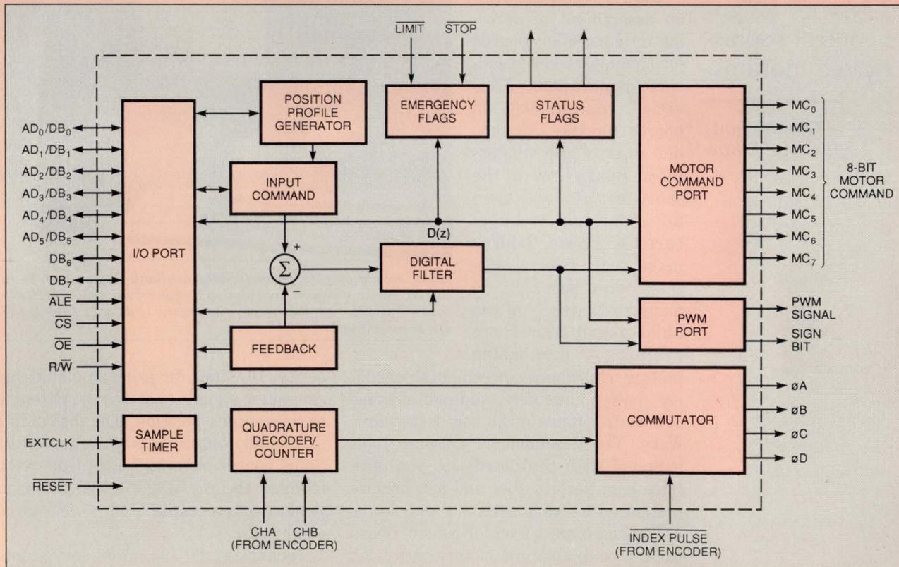
**Fig A—Commercial motor-control ICs can perform all of the functions needed to control a servo motor. Hewlett-Packard's HCTL-1000 decodes quadrature encoder signals; provides a loop filter; delivers parallel, PWM, and phase-commutated motor commands; and includes an interface to a  $\mu\text{P}$ .**
