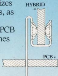
Fewer assembly steps. Dramatic reduction in rework. Lower overall costs. Increased product reliability. These are a few of the advantages of the new NAS "claw" grip solder and flux bearing edge clips — the only interconnects that assure 100% solderability.
