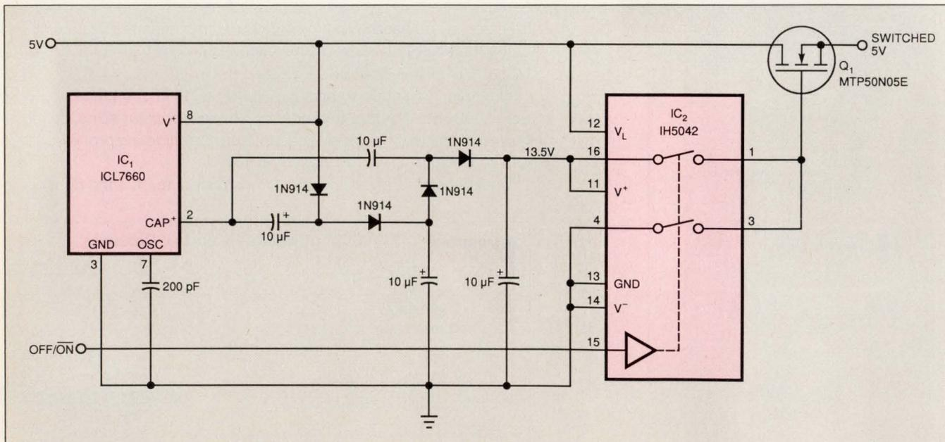
Fig 3—Additional stages in the voltage-multiplier section of this high-side switch provide a higher gate voltage, allowing use of a conventional NMOS switching transistor.
