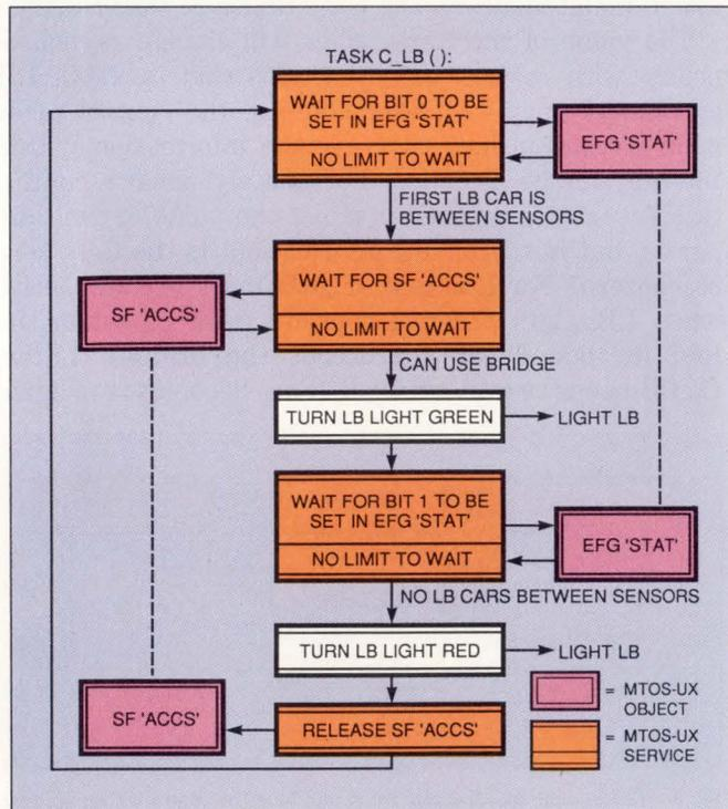
Fig 9—This implementation model shows details of a task that controls left-bound traffic on a 1-lane bridge. The details are hidden in Fig 8, which shows only overall tasking and coordination.
