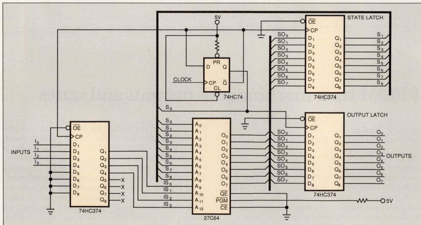
Fig 2—By adding a latch and a flip flop, this 2-phase state machine uses both clock edges to make better use of the PROM address space.
