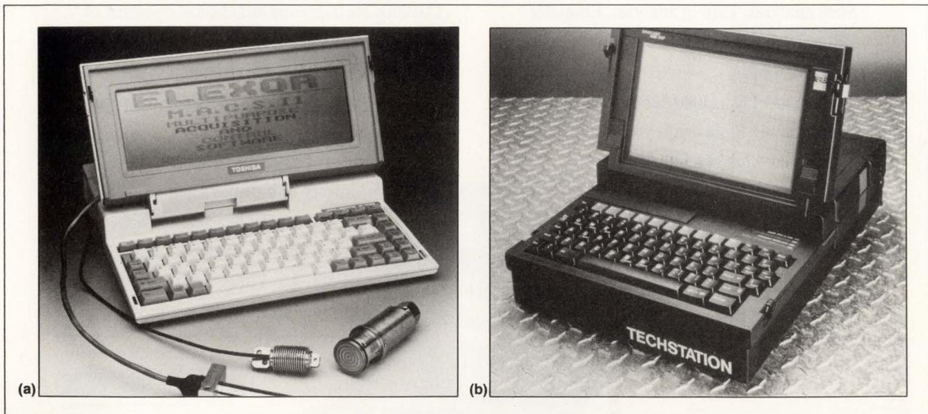
*Add sensor, will travel should be the motto of these PC-based systems. The TD-4000 (a) from Elexor Associates and the Techstation (b) from Onsite Instruments are complete analog data-acquisition and processing stations, including software.*
