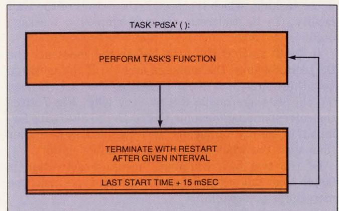
Fig 4—Periodic self-activation is one way a task can become active. When the task completes its function, it issues a call to the operating system to terminate itself and to restart itself after a given interval, in this case 15 msec.
