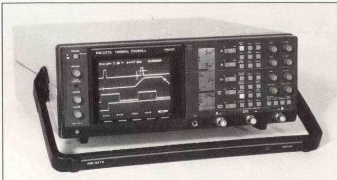
The 100-MHz, 250M-sample/sec PM 3375 is one of seven low-cost DSOs offered by Philips. This model performs nine automatic measurements in addition to cursor measurements.
