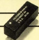
Line Sense Relays connect in series with Tip and Ring and provide a relay closure in response to loop current flow. For on-hook, off-hook monitoring, switchhook flash detection, and rotary dial pulse counting. Simple design, rugged construction.
