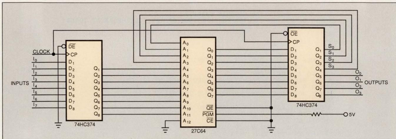
Fig 1—This simple state machine is limited to 8 bits for both output and state-feedback lines.
