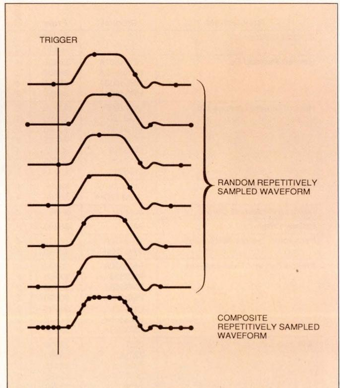
Fig 1—Repetitive sampling builds a composite waveform from data points taken from multiple waveforms. With random repetitive sampling, the form of repetitive sampling typically used by low-cost DSOs, the DSO can acquire data before the trigger because data is continually written into memory.
