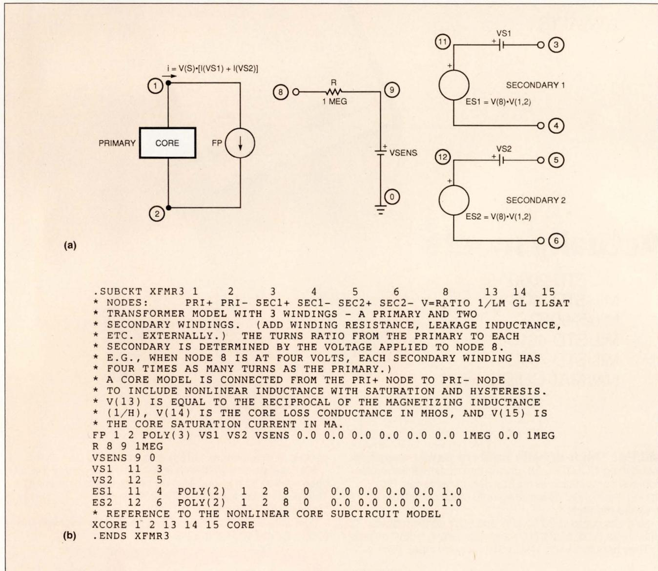
Fig 2—The Spice2 model and listing of this 3-winding transformer and the model in Fig 1 use 2-dimensional polynomials to implement the voltage-controlled turns ratio.
