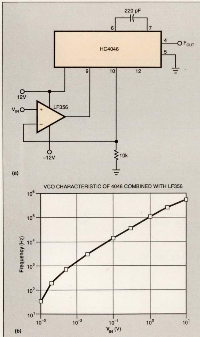
Fig 1—Using the HC4046's internal transistor (a) instead of an external component achieves the linearization in b.
