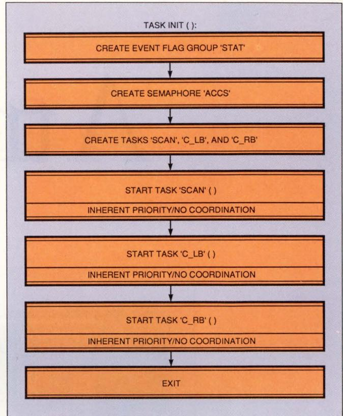
Fig 11—The initialization task creates all the elements of Fig 8's overall tasking and coordination and then terminates itself.
