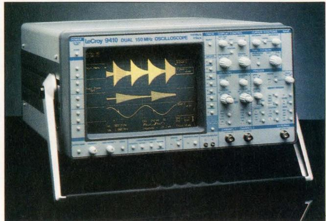
Extensive automatic-measurement features, a memory-card mass-storage system, and a 4000 × 4000-pixel display are key features of the LeCroy 9410 DSO. The 150-MHz unit provides 2% vertical accuracy and a 150M-sample/sec digitizing rate.
