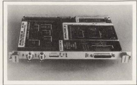
channel. The unit's equivalent input noise in a 700-kHz bandwidth is  $\frac{1}{2}$  LSB  $\pm 50 \mu\text{V}$  rms. Harmonic distortion is  $-92$  dB at 10 kHz. The board includes a sequencer that can work with multiplexer boards to expand the unit's capacity to 256 channels. \$4500. Delivery, 8 to 10 weeks ARO.
