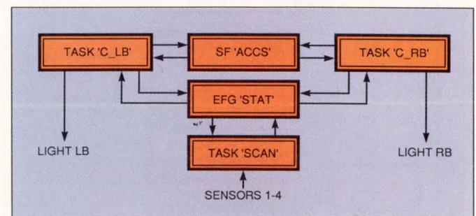
Fig 8—Tasking and coordination are at the heart of controller applications. This example shows tasks that control left-bound and right-bound traffic on a 1-lane bridge. Event-flag group 'STAT' keeps a tally of cars. Semaphore 'ACCS'—which only one task at a time can "own"—grants task access to the bridge.
