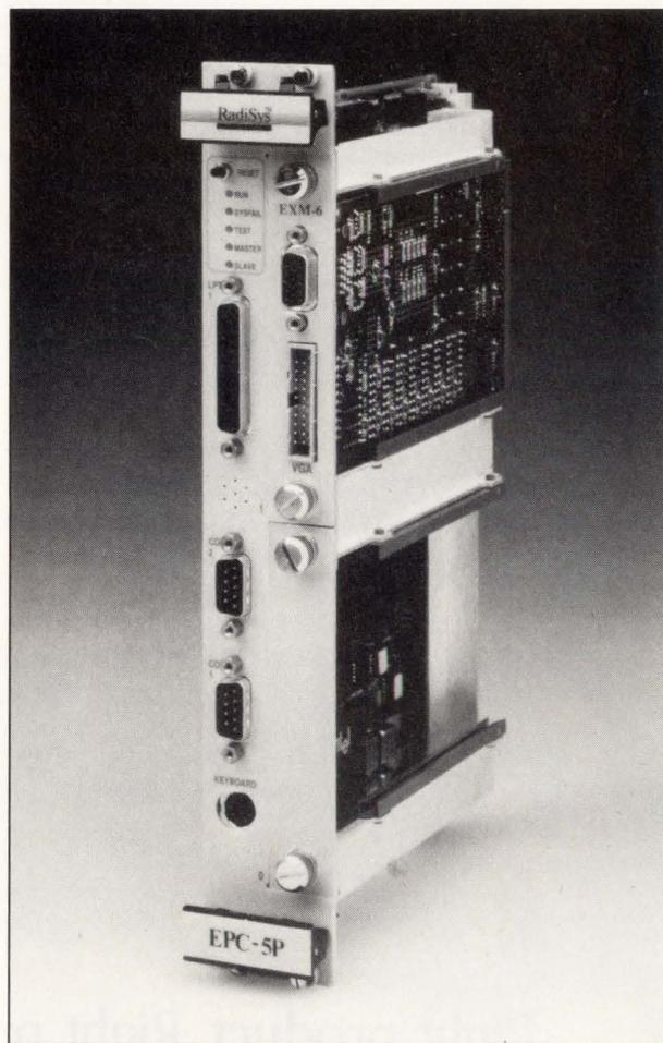
The 6×9×3.2-in. 80486-based VMEbus EPC-5 suits applications as a front-end computer in industrial control and other embedded-computer applications.
