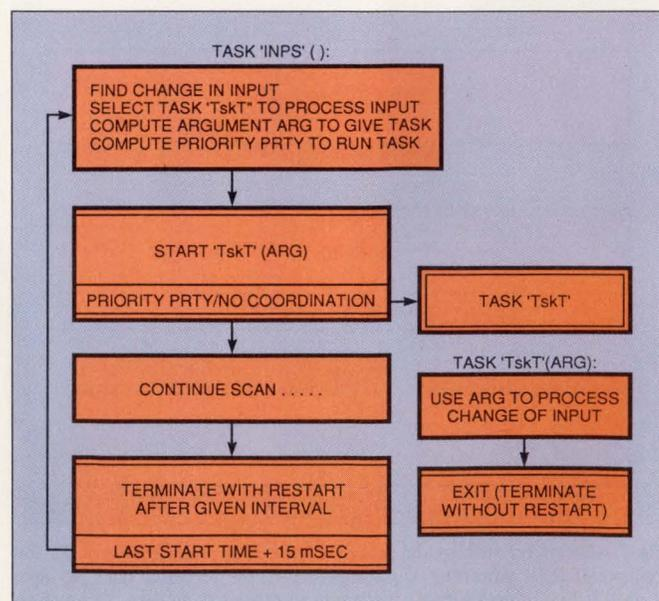
Fig 5—This typical input-scanning task is periodic. It runs every 15 msec, and it starts another task to process any change-of-input information.
