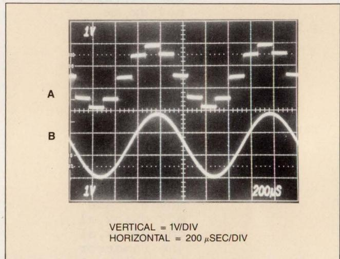
Fig 1—The output of Fig 1's multiplexer (trace A) emerges from the lowpass, continuous-time filter as a clean sine wave (trace B).
