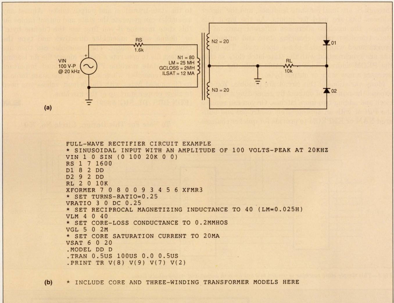
Fig 4—Nonlinear core and transformer models are useful for modelling this full-wave rectifier circuit (a) and Spice code (b).
