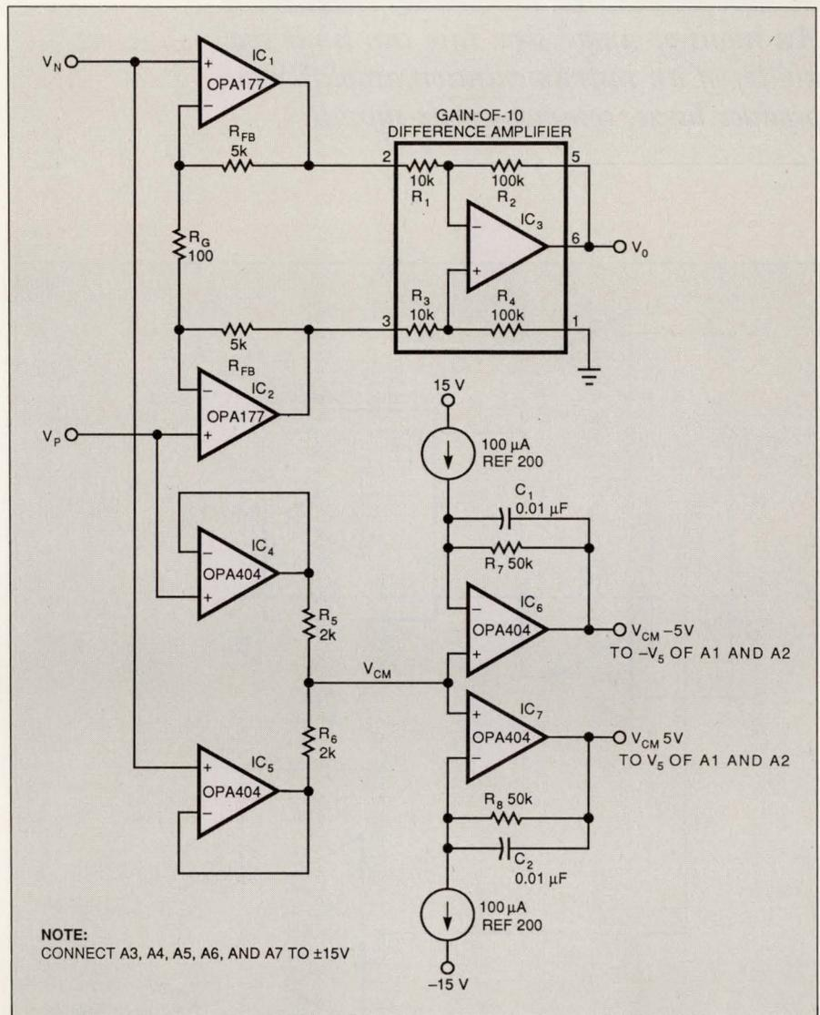
**Fig 2**—A common-mode voltage buffer connected to a resistor divider network drives the subregulated supplies that power the enhanced instrumentation amplifier.
