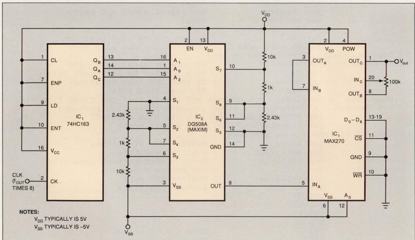
Fig 2—This circuit produces a pure,  $-80$ -dB THD sine wave with a frequency equal to the  $f_c$  of IC<sub>3</sub>'s filter.
