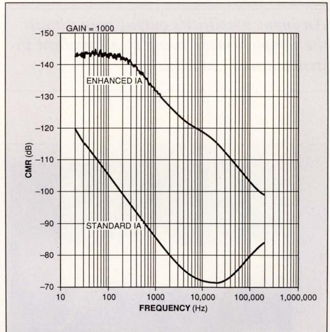
Fig 4—With a gain of 1000V/V, an enhanced instrumentation amplifier offers common-mode rejection of better than 120 dB at frequencies below 8 kHz.
