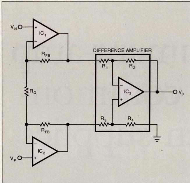
**Fig 1**—A 3-op-amp instrumentation amplifier boosts differential signals by a gain of  $R_2/R_1$ , if  $R_2/R_1$  matches  $R_4/R_3$ .
