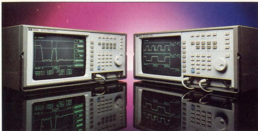
Trading off sampling rate for vertical resolution, both of these DSOs are priced at \$6450. Hewlett-Packard's HP 54502A has 6-bit resolution and samples at a maximum rate of 400M samples/sec. The 8-bit HP 54504A samples at a maximum rate of 200M samples/sec. Both DSOs offer a 400-MHz bandwidth for repetitive waveforms.
