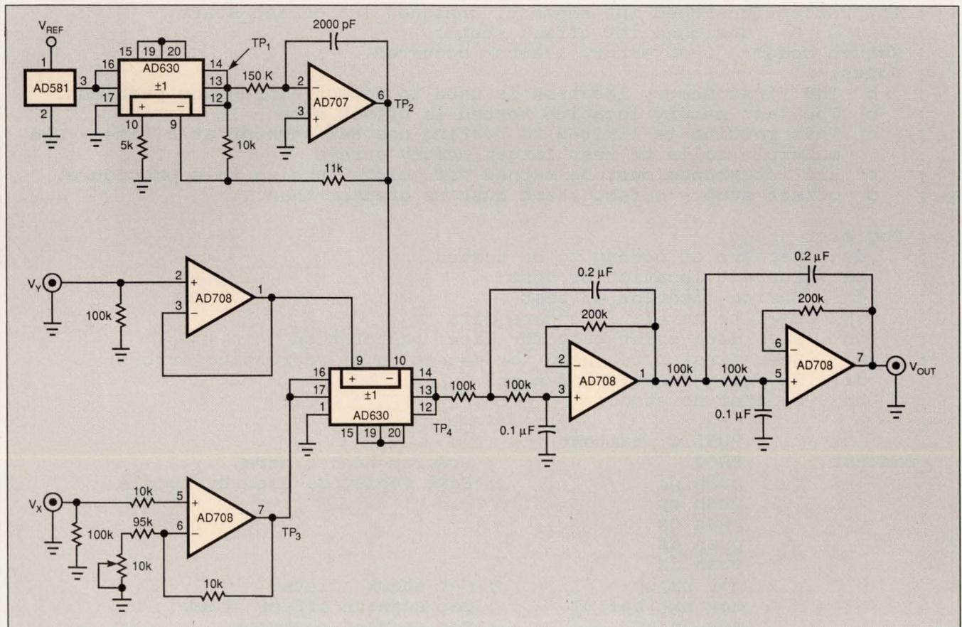
Fig 1—Two commutating amplifiers join a reference, an integrator, and a 4-pole filter to implement a 0.015%-accurate multiplier.
