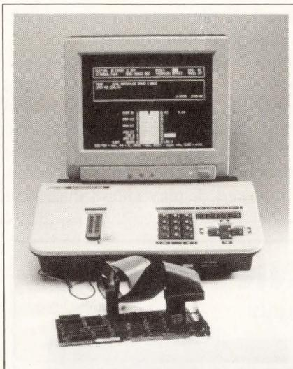
the tester back-drives the outputs of the surrounding devices. The tester can also check ICs not mounted on boards and can compare a board under test with a known-good board. The unit's library of device tests includes those for most TTL ICs. You can set logic
