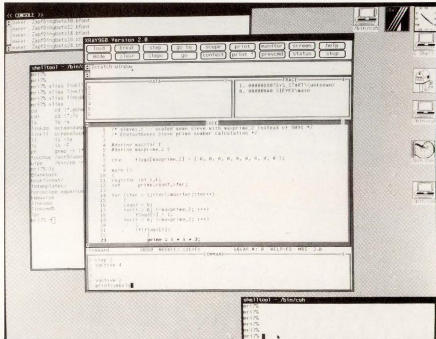
*You can invoke commands for a windowing debugger, such as Microtec Research's Xray, by using a mouse more quickly than you could with older command-line interfaces.*
