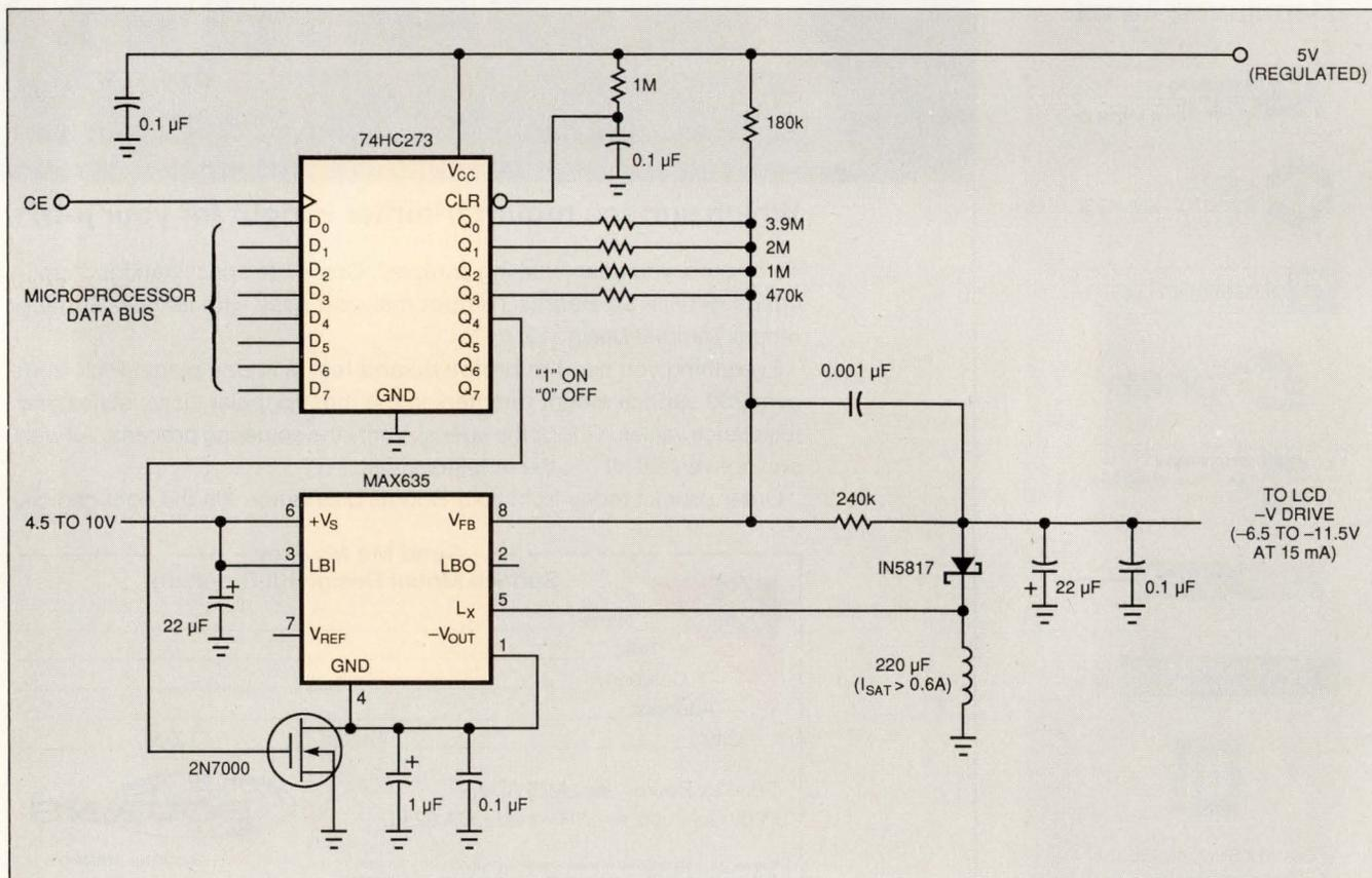
**Fig 1**—Using a resistor-ladder DAC and a voltage regulator IC, this circuit uses the system's positive battery supply to generate a digitally variable negative voltage.
