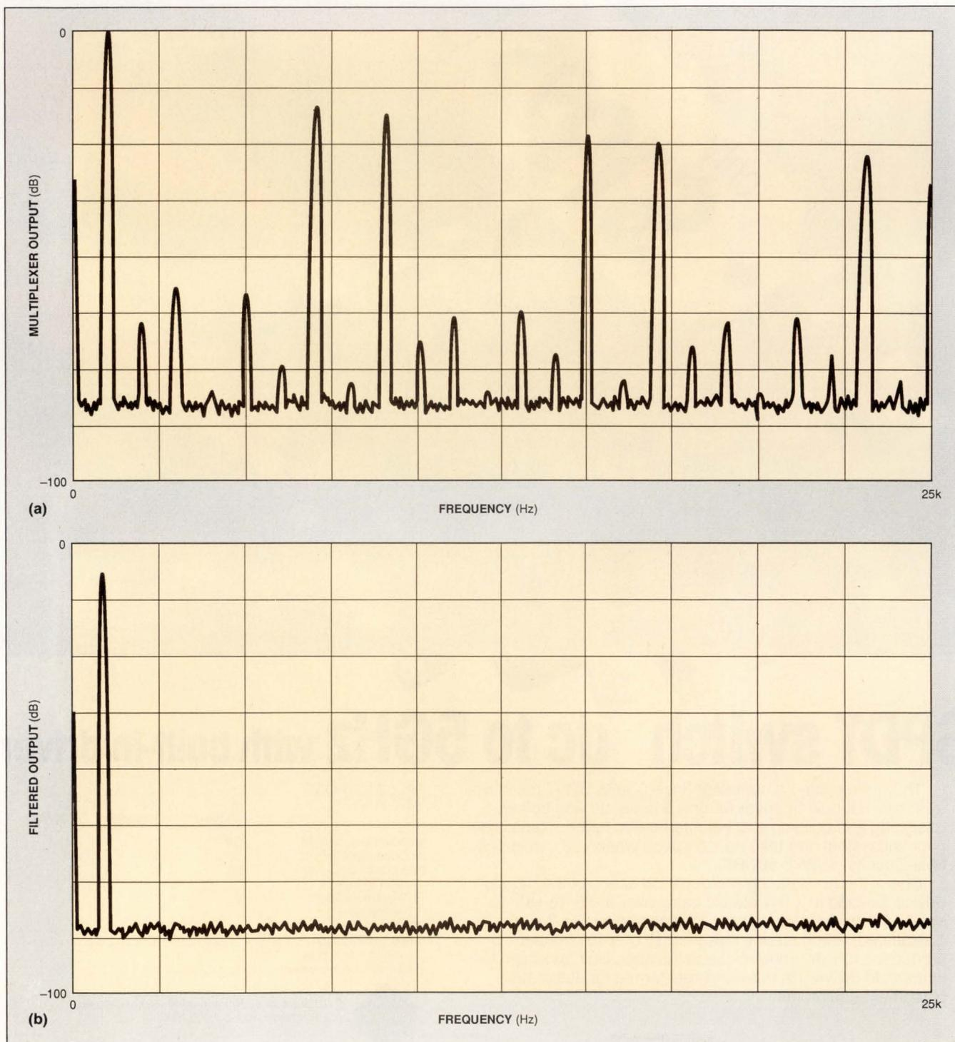
**Fig 3**—The circuit's approximation process generates large harmonics in the multiplexer's output spectrum (a), which the filter attenuates to below the spectrum analyzer's noise floor (b).
