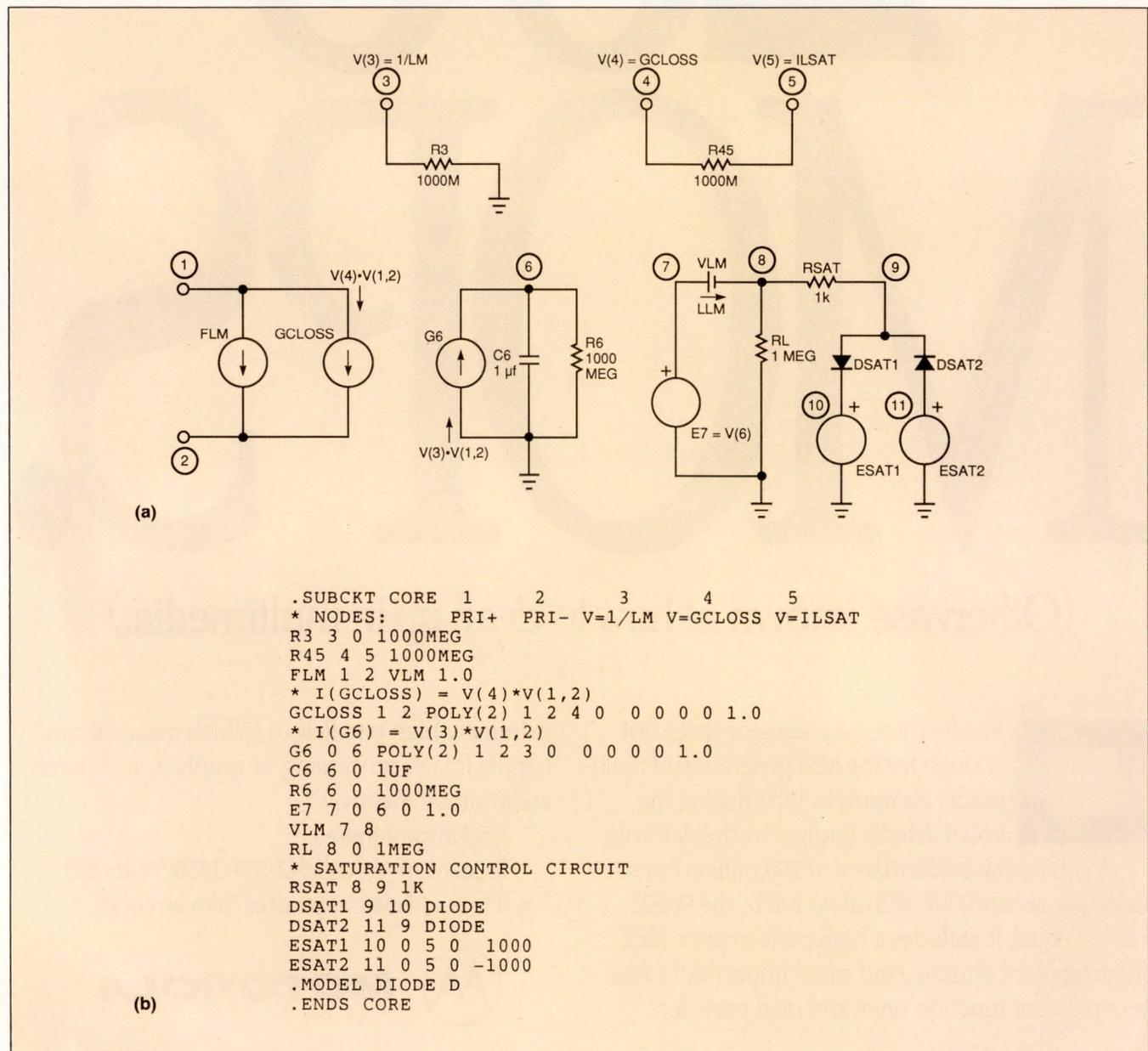
Fig 3—This saturating-core equivalent circuit (a) and model (b) include components that simulate core-loss conductance, magnetizing inductance, and current saturation using externally supplied dc voltages.
