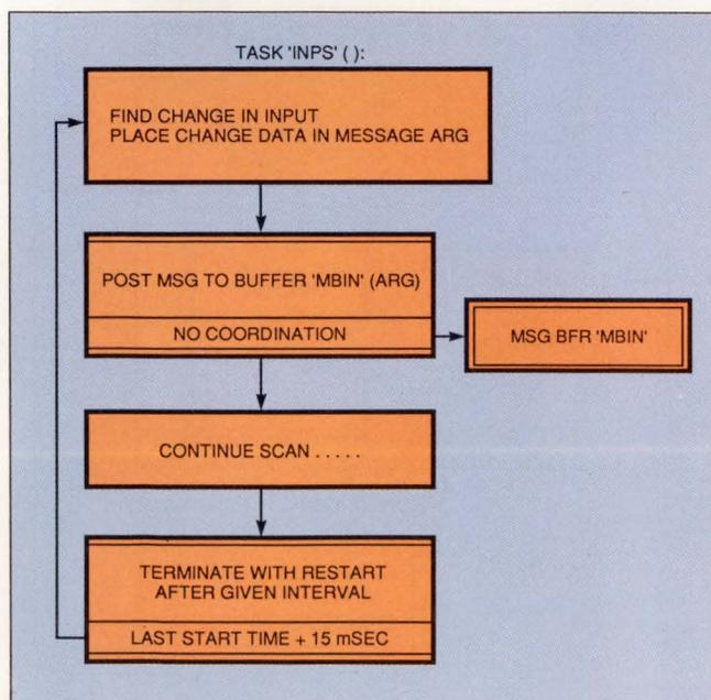
Fig 7—This message-based formulation of an input task passes a message regarding changed inputs to the processing task of Fig 6.
