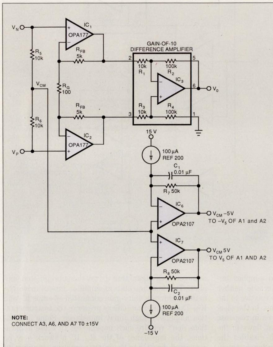
**Fig 3**—If you don't need high input impedance, removing the common-mode voltage buffers will still provide better common-mode rejection than standard instrumentation amplifiers and do it at a lower cost.
