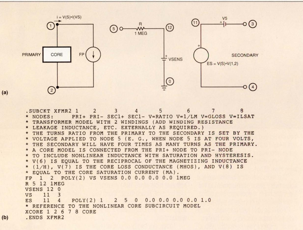
**Fig 1**—The voltage at node 5 controls the turns ratio of this 2-winding transformer equivalent circuit (a) and Spice model (b).
