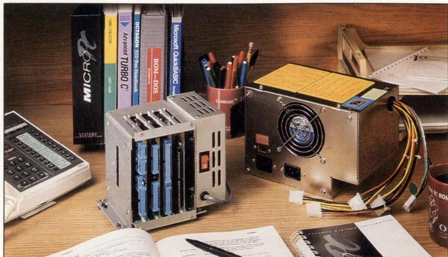
*The 4-slot card cage and power supply of the Micro-PC require less space than an IBM PC/AT's power supply.*
