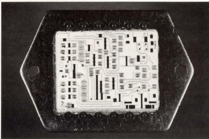
*Claimed by its manufacturer to be the highest voltage op amp available, the PA89 from Apex Microtechnology delivers an 1100V output swing to its load. Along with high output voltage, the device offers precision dc specs.*
