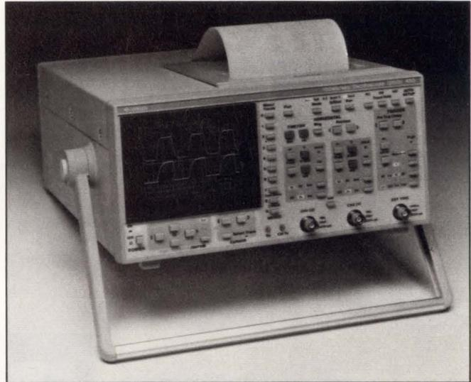
An optional internal plotter is available on some of Gould's DSOs, such as the 450. The 50-MHz, 100M-sample/sec DSO weighs 14 lbs and can operate from ac power or a portable battery pack.
