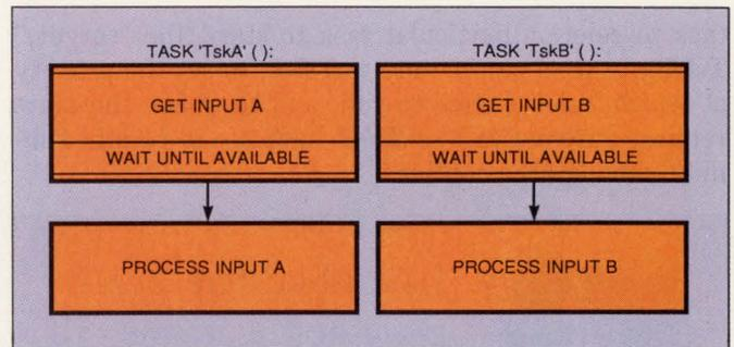
Fig 3—Parallel processing of real-time inputs improves on Fig 2's serial approach. In this example, in which the processing of B doesn't depend on A, the processor can get B without waiting for A.
