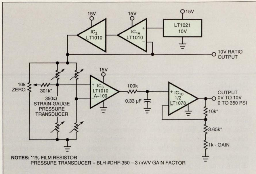
Fig 2—This typical bridge application uses an instrumentation amplifier, a voltage reference, and buffer amplifiers to provide signal conditioning for a 350Ω transducer.
