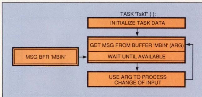
Fig 6—A cyclic task never terminates. In this example, it simply waits for input—in this case a message in a buffer—from another task. Use of this cyclic task contrasts with the approach taken in Fig 5, in which an input-processing task gets restarted with each new input.
