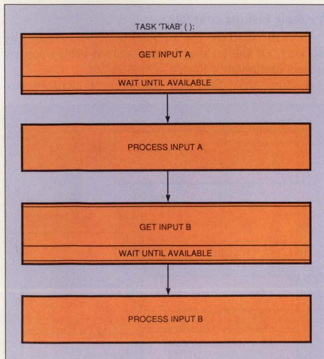
Fig 2—Always try to keep the processor busy with productive work. In this example of serial processing of real-time inputs, the processor can't get input B until it has finished with A. If there is no other task to keep the processor busy until A comes in, then the processor will be idle. If the processing of B doesn't depend on A, the scheme shown here is wasteful.
