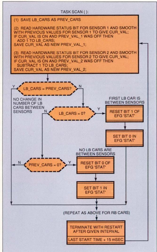
Fig 10—Details of the scanning task that appears only as a block in Fig 8, are shown in this implementation model.
