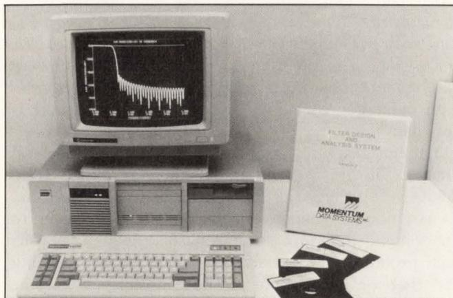
A filter-design software package can aid your introduction to DSP. The Filter Design and Analysis System (FDAS) from Momentum Data Systems helps you design and analyze filters and will even generate the program code needed to create the filter.
