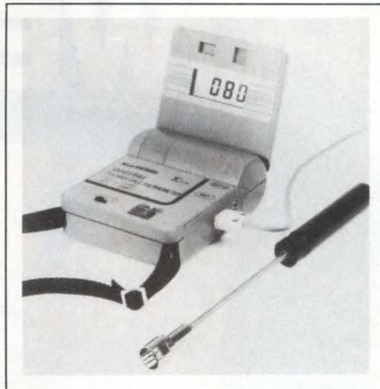
12 oz and measures from -58 to +1999°F and -50 to +1350°C. Its resolution is 1°F or C, and its accuracy equals ±0.2% of reading ±1 digit. A kit is available that includes the meter, a general-purpose temperature probe, and a carrying case. The meter, \$159; the kit, \$219.
