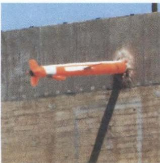
In a Navy test, a Tomahawk cruise missile exploded into a concrete building. When the dust settled, little remained but gravel and fragments of casing.
