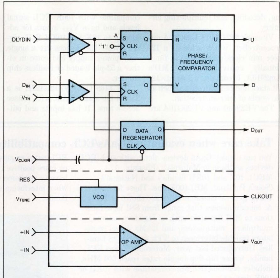
Fig 1—This clock- and data-recovery circuit, the 16G040 from Gigabit Logic, can operate at 2.4G-bps data rates.
