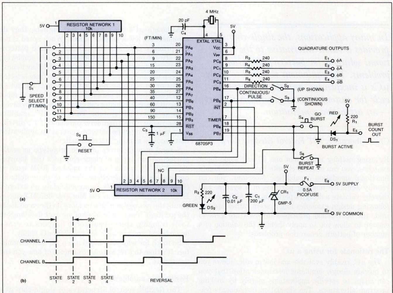
**Fig 1**—To accurately measure the direction and velocity of cable payout in well-logging applications, this optical-encoder simulator circuit (a) provides 11 discrete speeds having an accuracy within 0.5%. The phase relationship between the two output signals (b) contains direction information; the velocity is proportional to waveform frequency.
