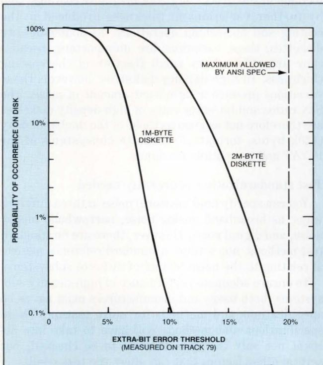
**Fig 1**—Noise characteristics of 2M-byte diskettes closely approach the ANSI-specified limit, whereas 1M-byte diskettes provide a greater safety margin.
