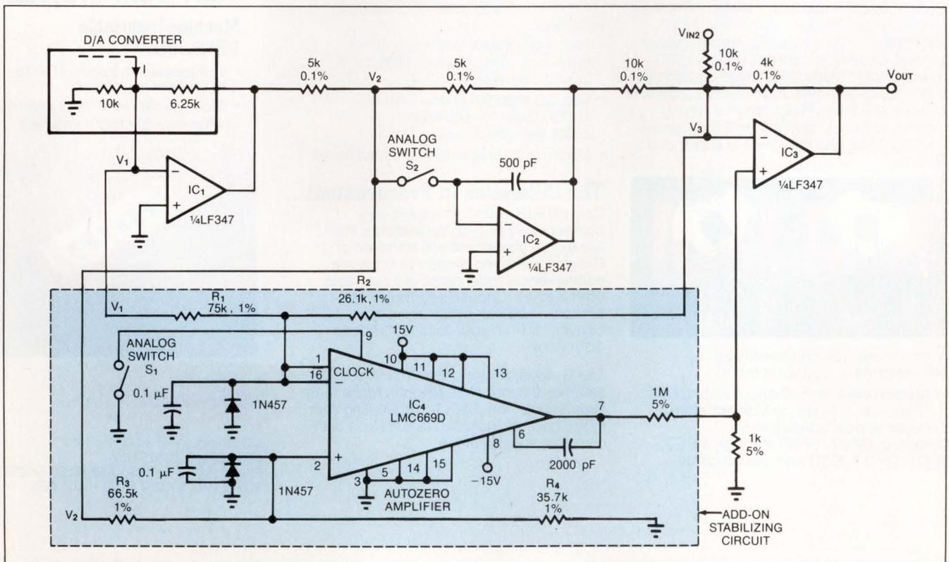
Fig 1—Addition of the stabilizing circuit (within the dotted lines) eliminates offset at  $V_{OUT}$  by adjusting the offset at  $IC_4$  to null the combined offsets of  $IC_1$  and  $IC_3$ .
