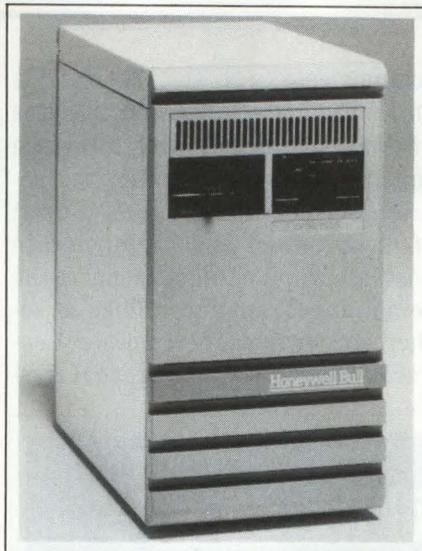
ry to achieve execution of 1 MIPS. You can select a 37M-, 68M-, or 142M-byte fixed-disk storage unit for integration into the system. \$17,130 for Model 211 with 32-bit CPU, 2M bytes of memory, six asynchronous communications ports, a peripheral controller, a 37M-byte hard disk, an integrated streaming tape drive, and an HVS 6 Plus operating system .
