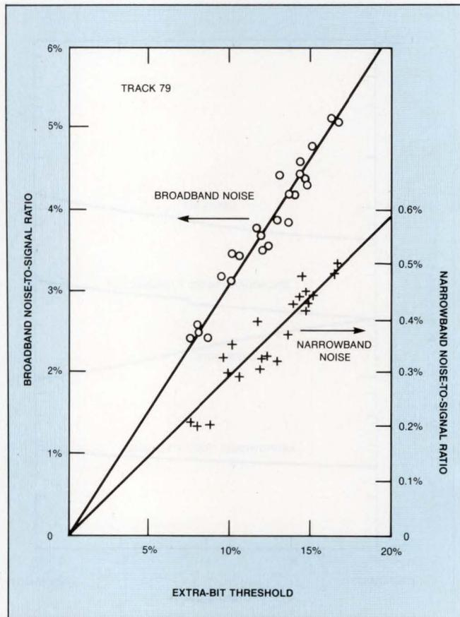
Fig 3—Results of narrowband and broadband analog noise tests correlate to extra-bit tests, but you must tightly control test bandwidths if this correlation is to be predictable.
