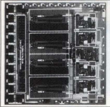
four DACs are functional, an ATE application can, during calibration, read data stored in the DAC latches. A reset command returns the DAC outputs to zero. The IC operates from  $\pm 12V$  and 5V supplies and features 400-mW power dissipation typ. Industrial grade, in a 28-pin DIP, \$60.80; in a 44-pin LCC, \$70.18 (100).
