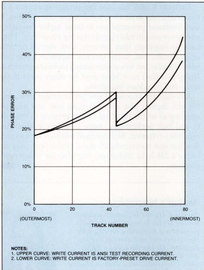
**Fig 4—Digital phase-error noise is greatest on track 79.** The step between tracks 43 and 44 is caused by internal bandwidth changes in the drive electronics.
