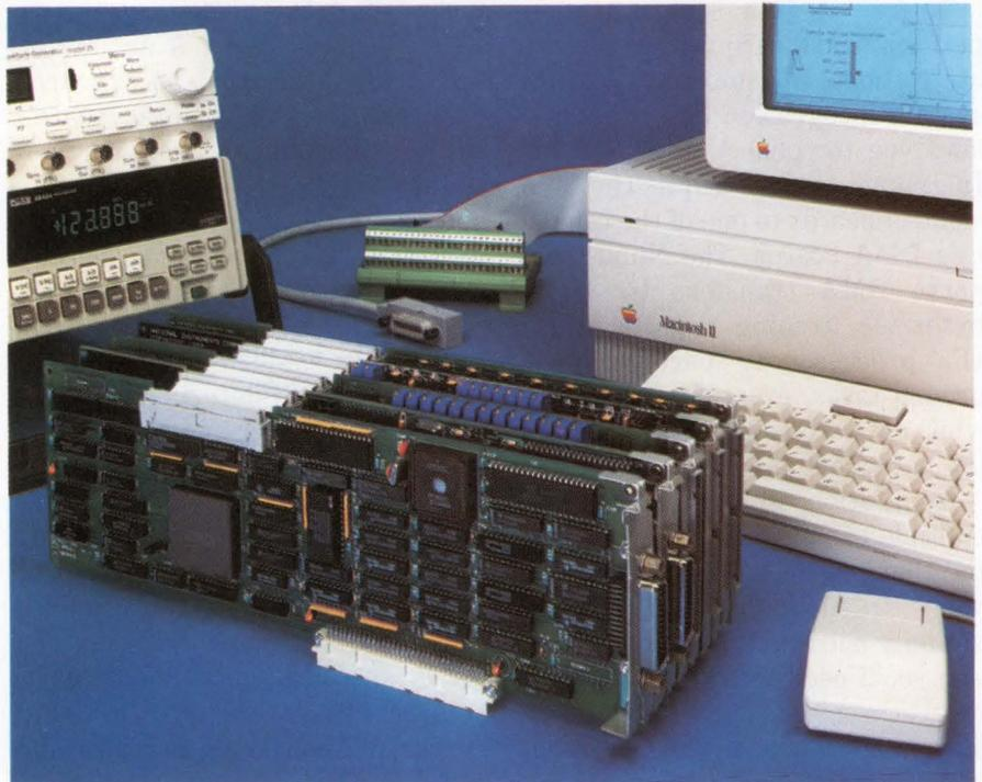
*A ribbon cable connects the real-time system-integration bus on these data-acquisition and -control cards from National Instruments. The bus can link as many as five data-acquisition and -control cards, providing synchronization and DMA capability.*
