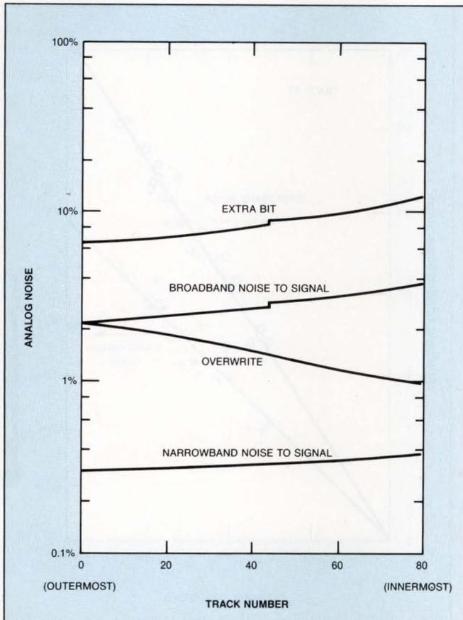
**Fig 2**—The slight jogs in extra-bit and broadband noise levels that occur between tracks 43 and 44 are related to internal changes in the bandwidth of the drive electronics.
