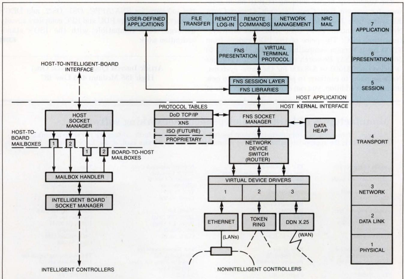
Fig 1—This TCP/IP-based network operating system from Network Research Corp runs on a variety of systems including personal computers, Unix-based systems, and DEC and IBM mainframes.
