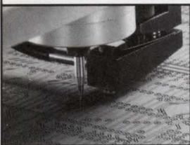
Paths of insulation around copper traces are created by the precision router. The LPKF unit also performs drilling and contour milling to complete the circuit board production.
