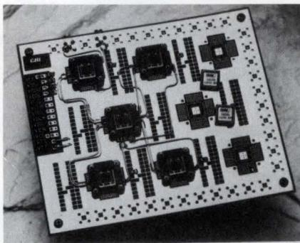
*A 16-bit, 2-nsec adder residing on a Gigabit Logic 90GUPB prototyping board makes use of the 10G100, a 1.3-GHz expandable 4-bit adder, and the 10G101, a 1.4-GHz carry-look-ahead generator.*
