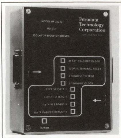
using EIA RS-232C and CCITT V.24 communications protocols. The model provides 1500V optical isolation between input and output ports that eliminates common-mode voltages and ground loops. The unit also functions as an RS-232C repeater, which doubles the length of the communication line. As a repeater it can retransmit data bidirectionally at rates to 19.6k baud. The unit has
