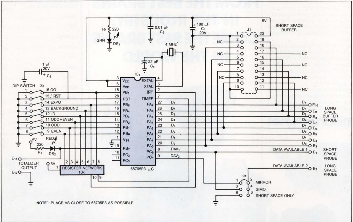
**Fig 4**—When intrinsic data is the important factor, rather than the relative speed of acquisition,  $\mu$ C-based simulators can be especially useful. This circuit illustrates how you can use a  $\mu$ C to replace two A/D converters in a spectral litho-density tool.
