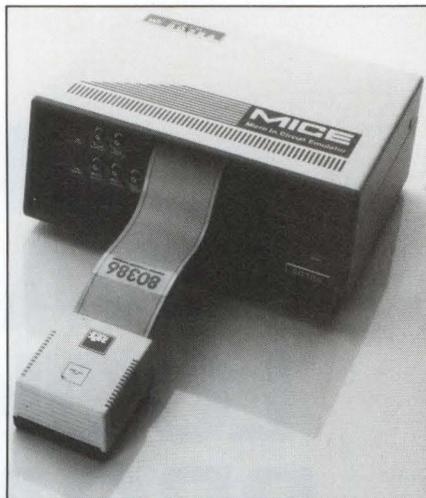
*Using an active probe, Microtek's Mice-32/80386 permits operation of the target system with a 20-MHz clock. It operates in several modes, without inserting additional wait states.*
