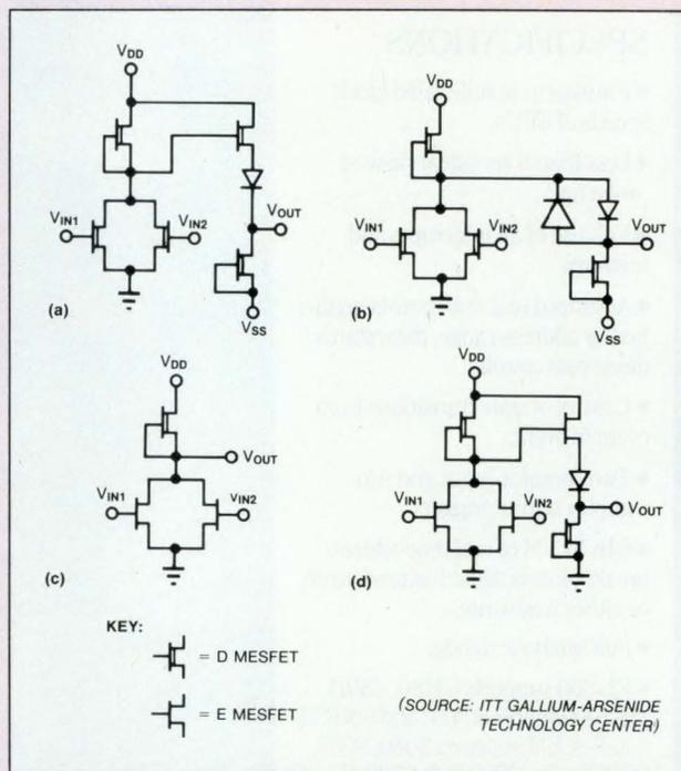
Fig A—Four 2-input NOR-gate configurations—the BFL (a), the CBFL (b), the DCFL (c), and the LPFL (d)—for GaAs logic circuits exhibit tradeoffs between speed, power, and manufacturability.
