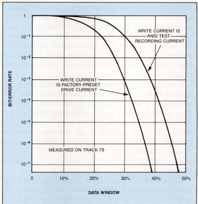
**Fig 5—Phase-margin test results are easy for a user to understand.** This test should be a part of all quality-assurance and media-evaluation programs.
