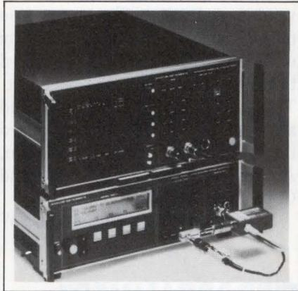
2 GHz. From 2 to 20 GHz, the unit holds harmonics and subharmonics to -40 and -60 dBc min, respectively. The vendor claims that you can calibrate the instrument in 15 minutes by using a counter interfaced to the sweep generator via the IEEE-488 bus, and a power meter. \$21,950. Delivery, 60 days ARO.
