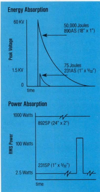
Regardless of the pulse shape, we have the resistor. Our Type SP handles large amounts of power from 60 cycles through VHF. Type AS can absorb huge amounts of energy in millisecond pulses. Type A solves high resistance problems in high voltage situations.
