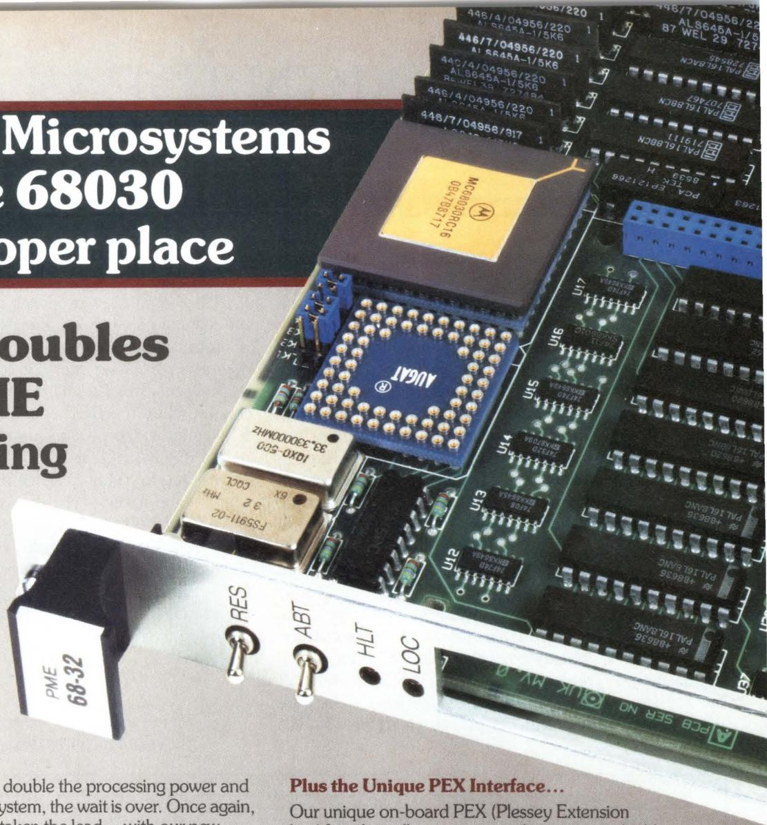
If you've been yearning to double the processing power and throughput of your VME system, the wait is over. Once again, Plessey Microsystems has taken the lead... with our new 68030-based PME 68-32 VME Single Board Computer. It puts all the power of the 68030 into the industry's fastest, most powerful and versatile VMEbus processor board. And we're not talking about a board that's under development. The PME 68-32 is here...right now!
