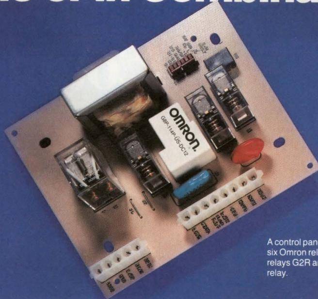
A control panel of a major appliance manufacturer shows six Omron relays—a general purpose LY2, power PCB relays G2R and G8P, as well as a G6E signal control relay.
