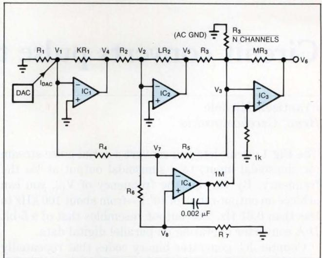
Fig 2—You can build low-drift amplifiers such as that of Fig 1 by using this simplified schematic and Eq 7 in the text.
