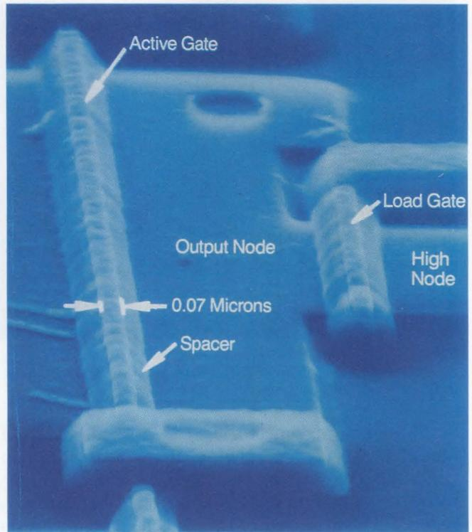
**Fig 5**—Built with a minimum feature size of 0.07  $\mu\text{m}$ , (which is about 10 times smaller than the geometries of today's commercial ICs), this NMOS FET developed at IBM's T J Watson Research Center exhibits excellent transconductance characteristics, proving that such small devices are indeed feasible.
