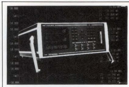
RAM. The oscilloscope can acquire data at 20M samples/sec with 8-bit resolution and at 2M samples/sec with 10- or 12-bit resolution. The computer incorporates a 1.2M-byte floppy-disk drive and, optionally, a 20M- or 40M-byte hard-disk drive. Further, the scope can run data-analysis applications such as Asyst, Asystant, and ILS. \$8000 to \$11,000.
