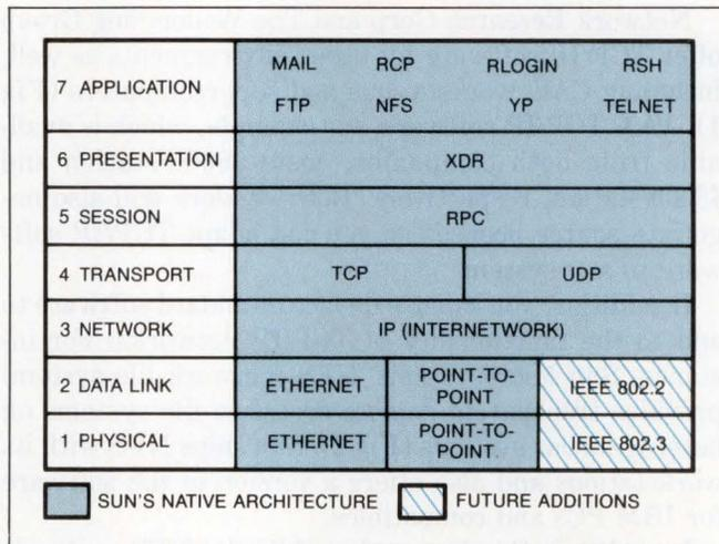
**Fig 2—The application-layer NFS software (layer 7) that Sun Microsystems offers has become a de facto standard for file services among heterogeneous systems.**
