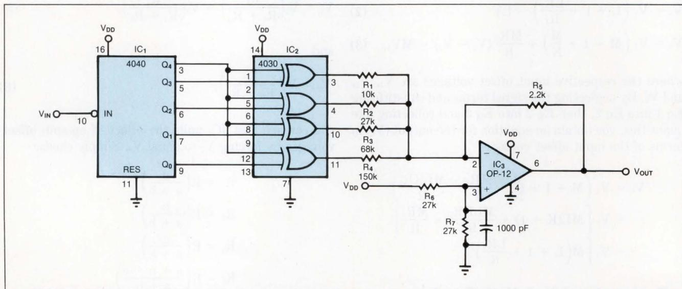
Fig 1—This circuit converts an input pulse train to a sinusoidal output, producing a signal similar to that of a 5-bit D/A converter.
