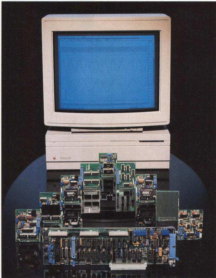
*By plugging as many as three modules into the MacAdios II data-acquisition and -control board from GW Instruments, you can add extra A/D converters, D/A converters, filters, and analog-input multiplexers.*
