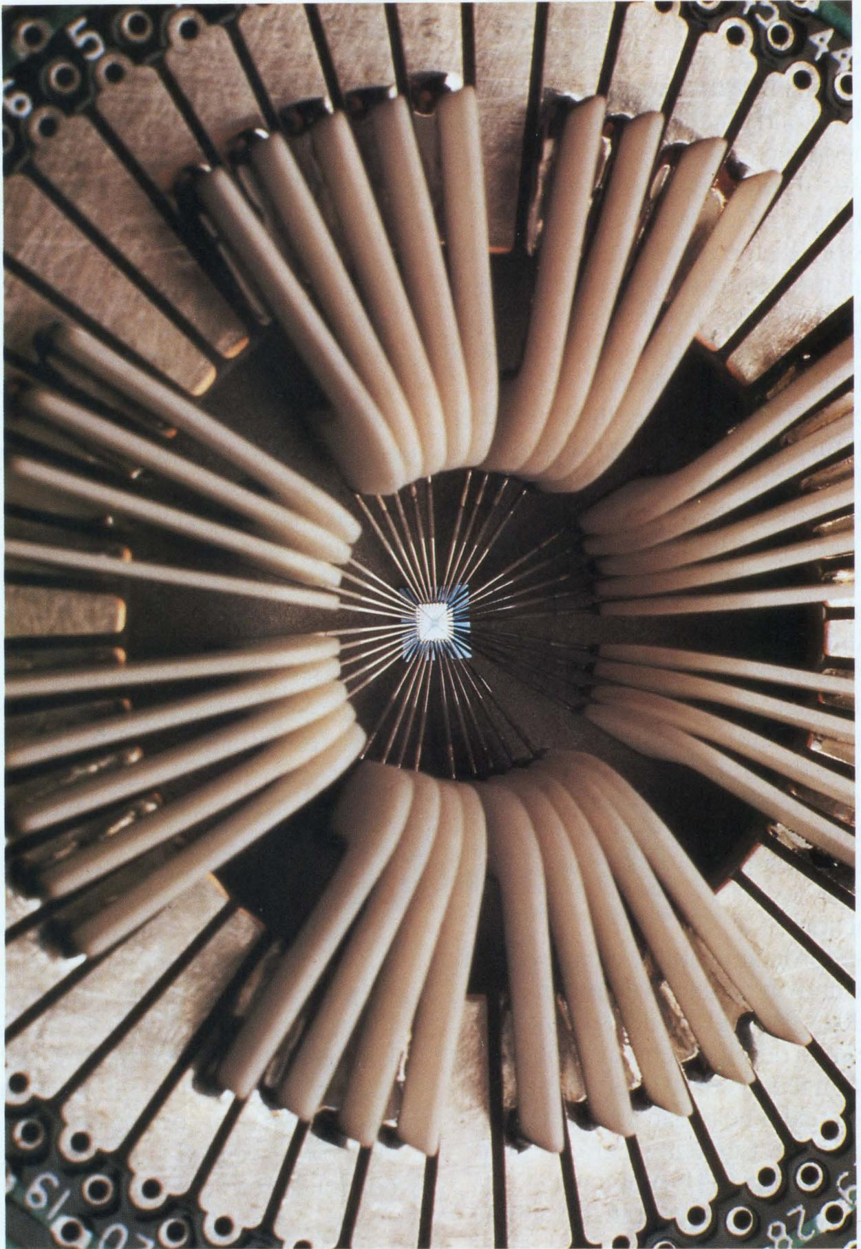
*The world's smallest FETs, having feature sizes smaller than 0.1  $\mu\text{m}$ , undergo testing at IBM's T J Watson Research Center. Devices such as these minuscule transistors promise to revolutionize system design by making it possible to design ICs incorporating as many as 1 billion transistors per chip.*
