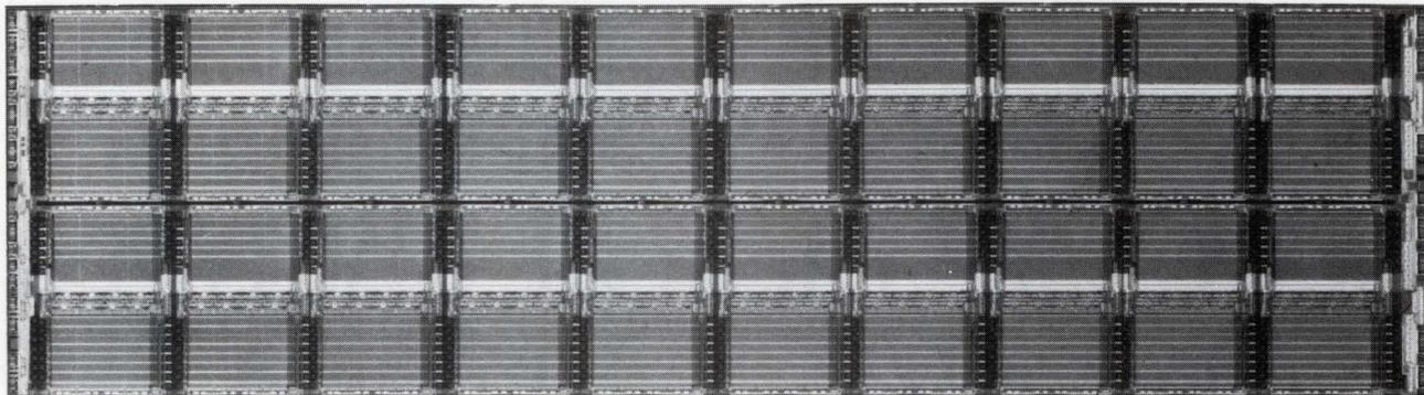
*Fig 1—Only 32 of the 40 available 4k-byte blocks must be good for Inova to create a fully functional 128k-byte static RAM on its S128K8 die. A laser isolates bad blocks in the first layer of metal interconnection before the second layer links the remaining good blocks.*
