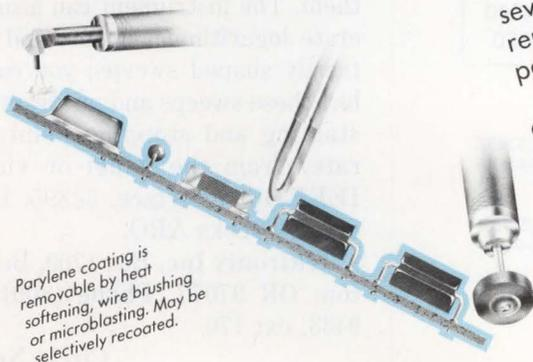
Parylene coating is removable by heat softening, wire brushing or microblasting. May be selectively recoated.
