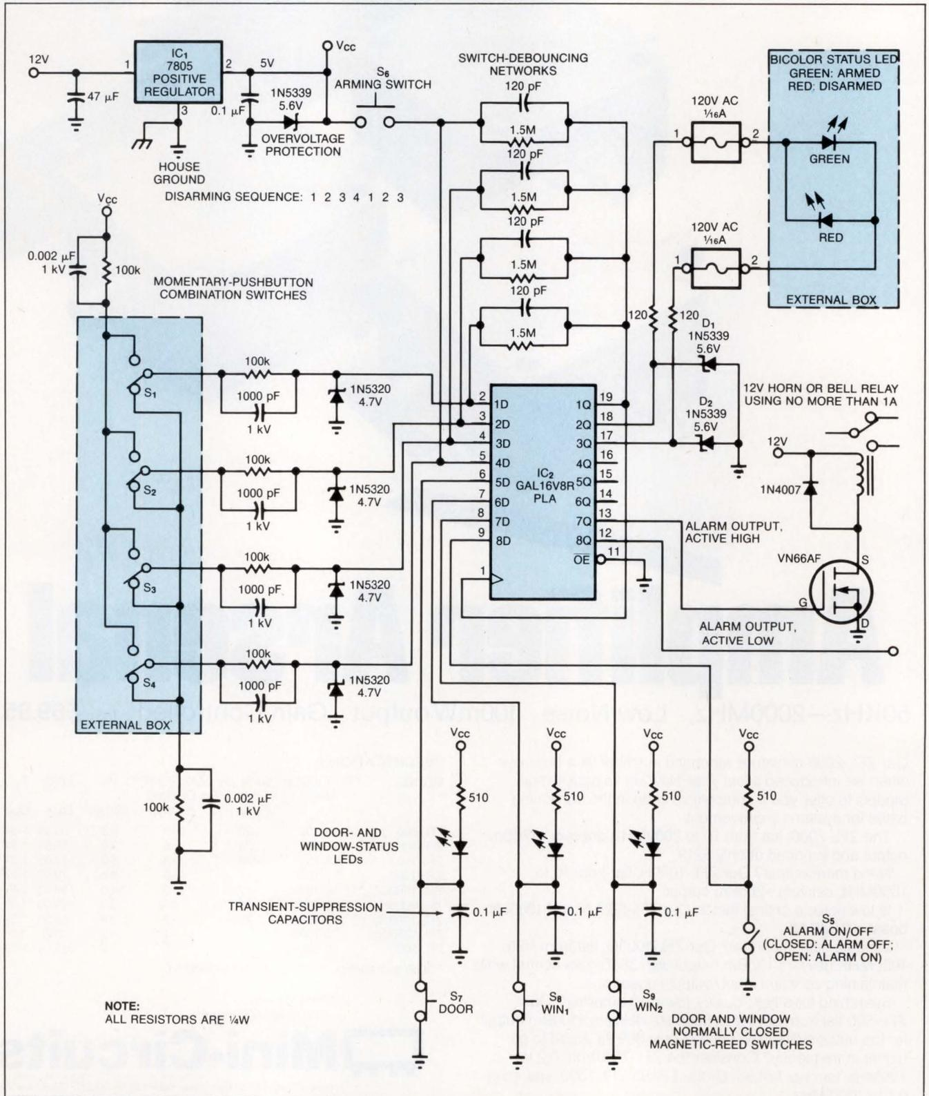
Fig 1—This burglar alarm can be deactivated by pressing the correct 7-digit sequence on pushbutton switches  $S_1$ - $S_4$ .
