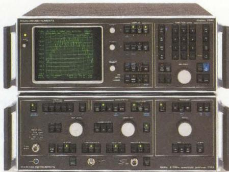
4.2 GHz Spectrum Analyzer—Model 2383
