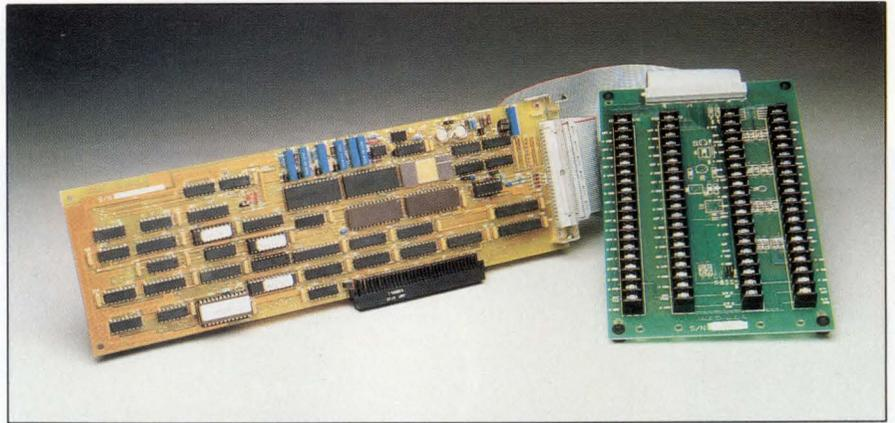
At \$795, the *Forerunner* data-acquisition board from Data Translation includes two 12-bit D/A converters and a 12-bit A/D converter that samples at 40k samples/sec.
