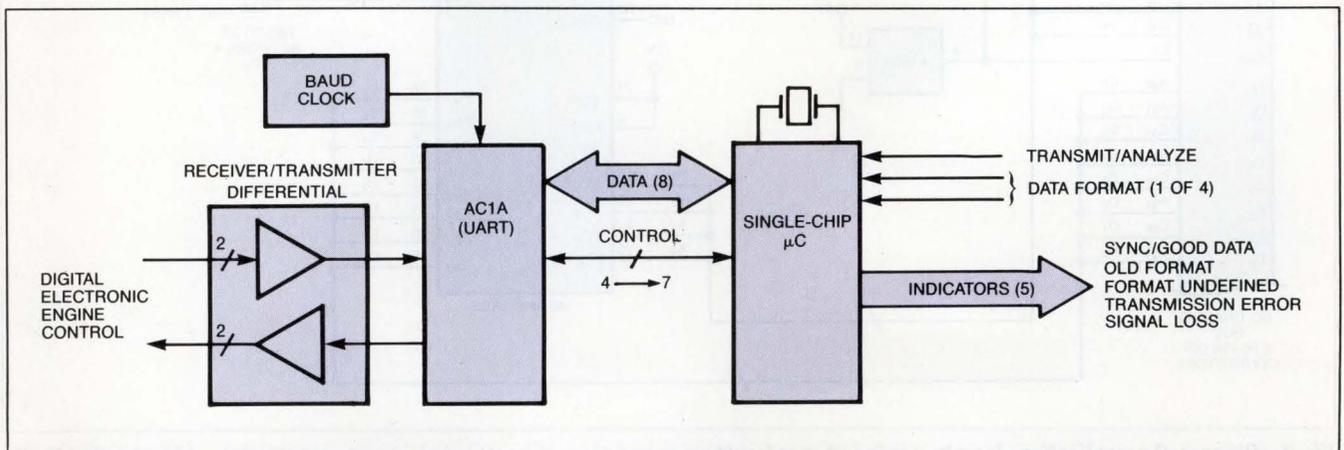
Fig 2—The  $\mu$ C in this serial-data simulator operates in two modes. In one, it analyzes the data frames output from a jet-engine control unit. In the second mode, the  $\mu$ C generates four test patterns to simulate the same unit.
