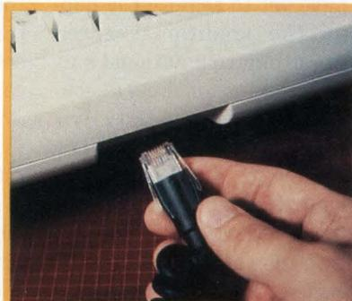
*Molex's first shielded interconnection system, SEMCONN, provides protection from electrical noise.*
