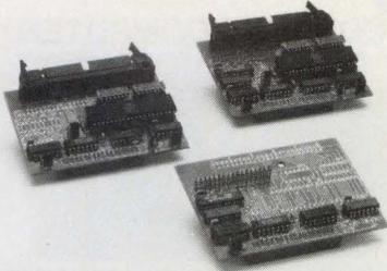
We've upgraded our SBSxSCSI module to support Block-Mode Pseudo-DMA transfers. That means CPUs without DMA can increase transfer speeds by not polling for READY on every byte. We've also added an optional Centronics-compatible printer port (SBSxCEN/CEN). If you only need the printer port, save money with our low-cost SBSxCEN module. We also offer a Floppy-Disk Controller module (SBSxFDC) that handles 3 1/2", 5 1/4", and 8" drives with SD, DD and HD formats.
