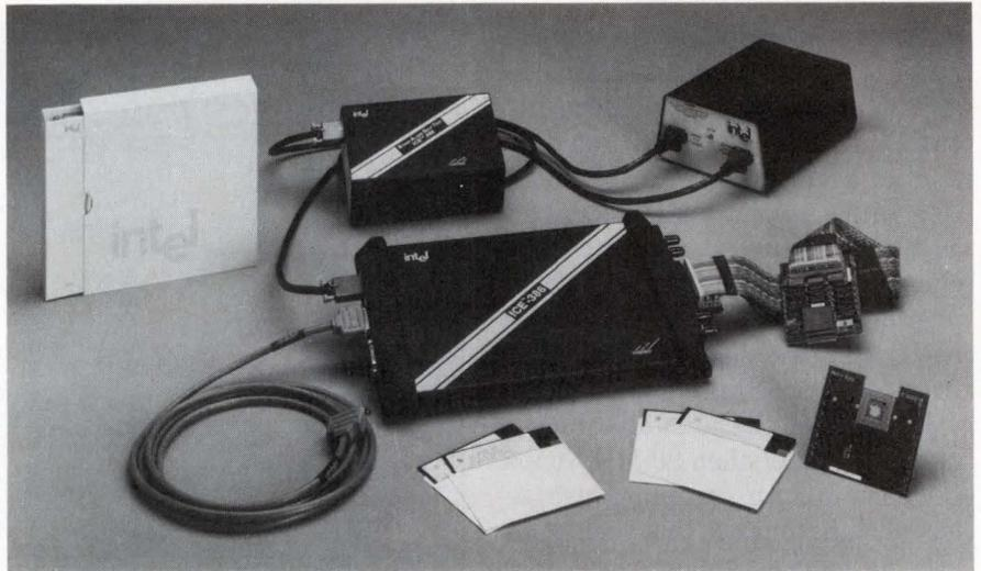
An in-circuit emulator from Intel, the Ice-386, consists of a control unit with RS-232C cable, power supply, user cable assembly, signal-access board with removal tool, optional isolation board, and a stand-alone self-test unit.
