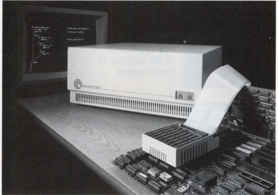
*This 80386 in-circuit emulator, the HyperIce-386 from Microcosm, features a probe built with surface-mount technology to achieve low profile. Trigger circuits in the probe are realized with custom CMOS gate arrays.*
