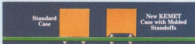
The new KEMET CKR06 meets all applicable requirements of MIL-C-39014/02 for military components, yet maintains the same overall dimensions as standard units (.300" x .300" x .100"). The result: better solderability performance and greater productivity, without increasing board space.
