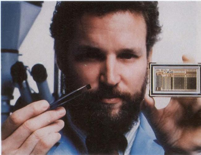
**Fig 4**—Using a piece of silicon about the size of a credit card (shown in mock-up form on the right), TRW's "superchip" contains approximately 34.7 million transistors, dwarfing a conventional IC. The superchip incorporates redundancy and built-in self-test/self-configuration circuits that allow the device to circumvent inoperative circuitry.
