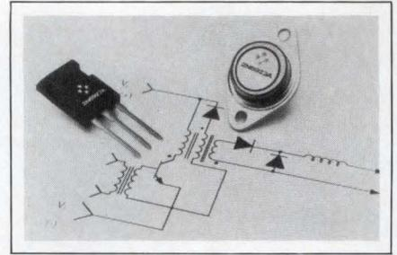
collector current ratings of 10, 15, and 25A, and a maximum  $V_{CE(sat)}$  of just 1V at 25°C. All models have the ability to switch peak-rated current (20 to 50A) at 500V. At 25°C, the units feature maximum voltage rise time and a current fall time of 30 nsec, and a maximum crossover time of 50 nsec. At 100°C, the maximum crossover time is only 70 nsec. For applications where 550V  $V_{CEV}$  is sufficient, you may order each model without the A suffix. \$5.33 to \$21.45 (100).
