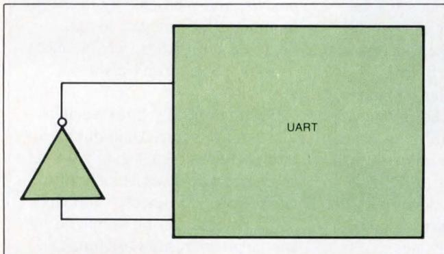
**Fig 3—In this configuration, the inverter establishes an unbreakable feedback loop between two pins of the UART. Test patterns that drive both these pins simultaneously would produce glitches and unrepeatable results.**
