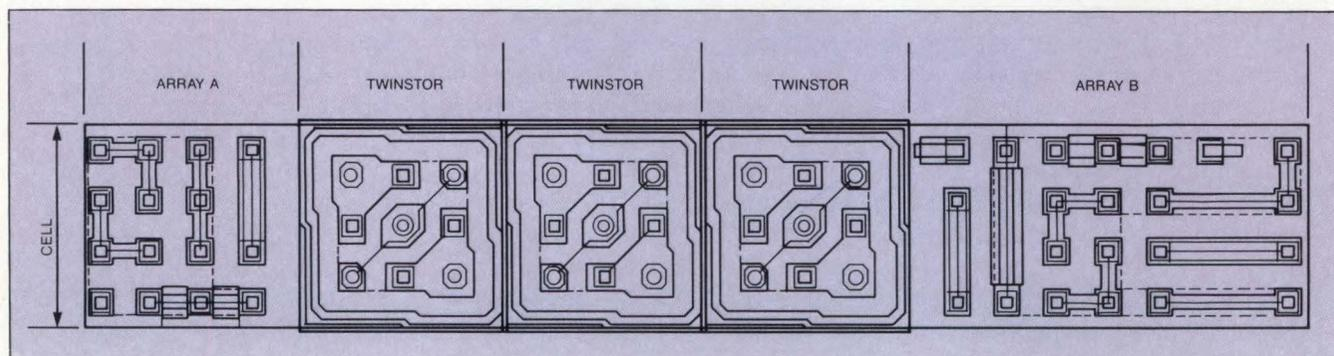
*One of the most versatile linear arrays is the Flexar Series from Exar. Shown here is a single cell containing three Twinstors and two resistor arrays. You can use the Twinstor as a pnp or npn transistor or as a resistor.*
