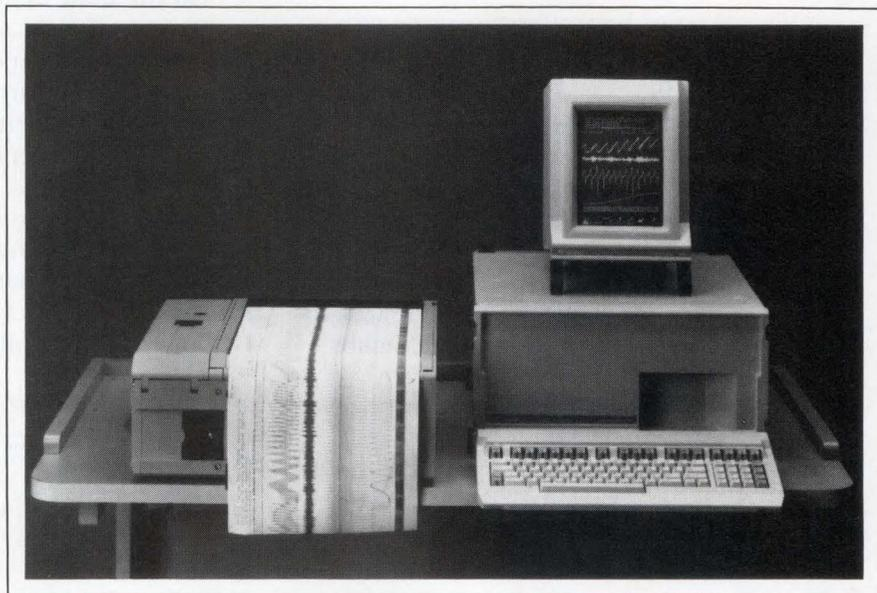
tions). In its program mode, the monitor displays menus for configuration; in its graphics mode, it displays traces, text, and grids in real time. From \$18,700. Delivery, 60
