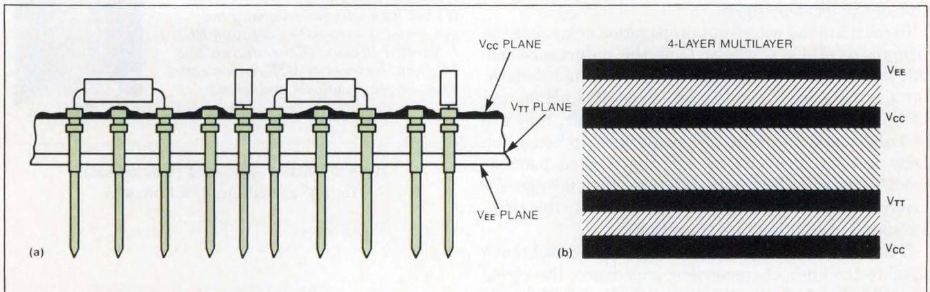
**Fig 3—To accommodate the needs of ECL circuit designers, some manufacturers offer panels that have three voltage planes—one each for  $V_{CC}$ ,  $V_{TT}$ , and  $V_{EE}$  (a). Some also offer boards that have a fourth voltage plane (b), which you normally connect to  $V_{CC}$ .**
