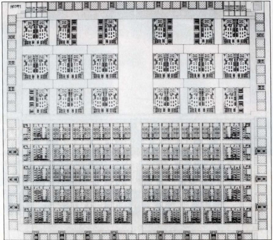
*To meet the demand for high-speed semicustom chips, Tektronix introduced the QC-4. It contains 300 ECL gates with propagation delays of less than 400 nsec; its analog portion contains npn transistors that have a typical gain-bandwidth product of 6.5 GHz.*
