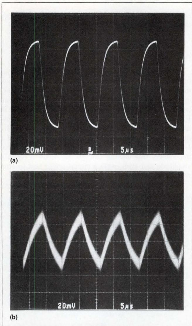
**Fig 2**—A true representation of a low-level signal from a high-impedance source (a) changes drastically when hookup wire replaces the scope probe (b). The amplitude decreases due to increased resistive and capacitive loading, and noise is added because the wire is unshielded.
