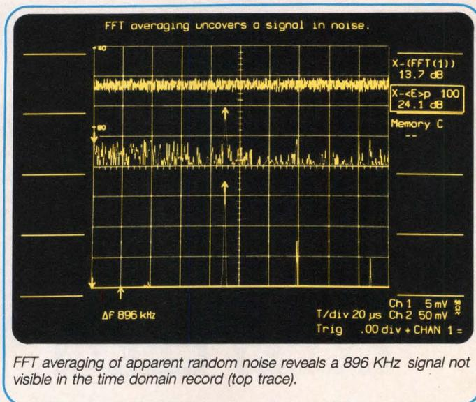
FFT averaging of apparent random noise reveals a 896 KHz signal not visible in the time domain record (top trace).
