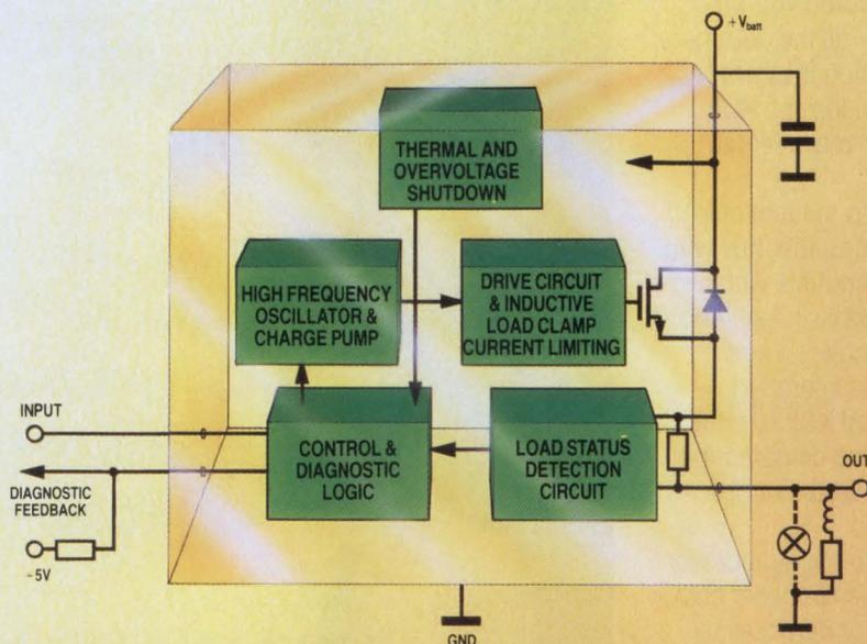
SGS, of course. In fact, the L9801 High Side Driver is an impressive example of what SGS Multipower-BCD™ (Bipolar, CMOS, DMOS) can do in automotive lamp, solenoid and motor driver applications.
