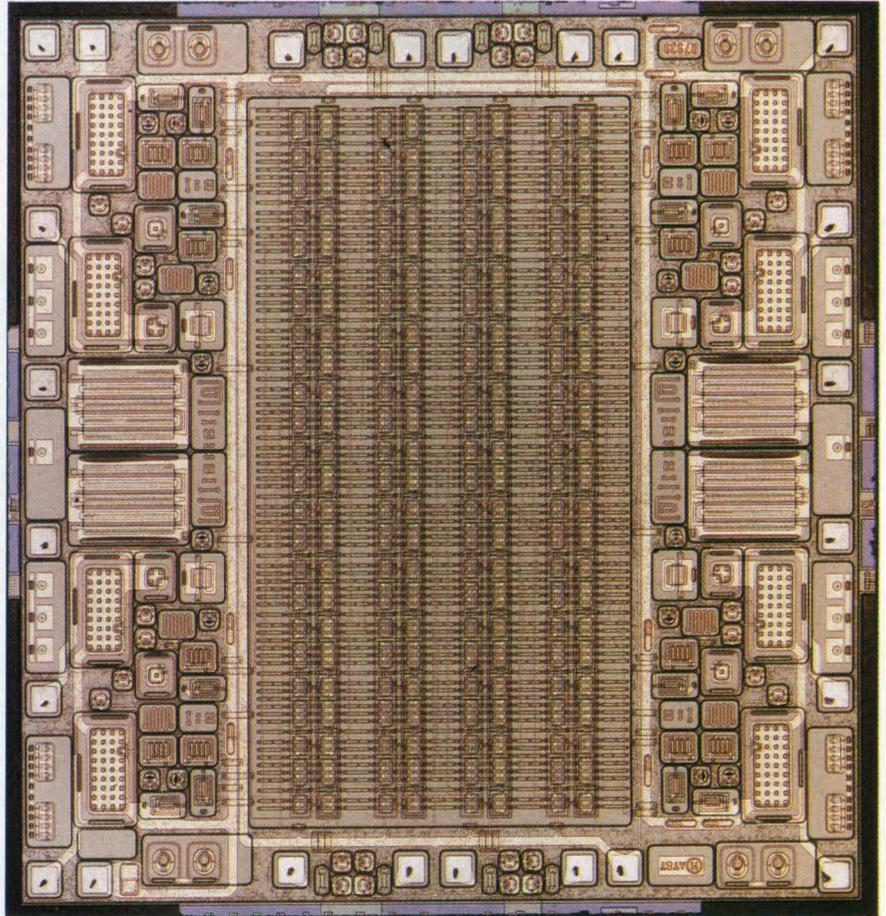
*Standing above all others in the high-voltage hierarchy, the ALA500 from AT&T has a rating of 250V. Fabricated in a BCDMOS technology with dielectric isolation, the chip includes 120 CMOS gates, 16 DMOS transistors, eight bipolar transistors, and 32 NMOS/PMOS transistors.*
