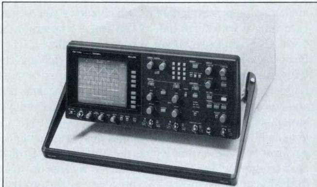
Offering 3-nsec glitch capture and 10-bit resolution, Philips's 200-MHz PM 3320 also provides an autosegment feature.
