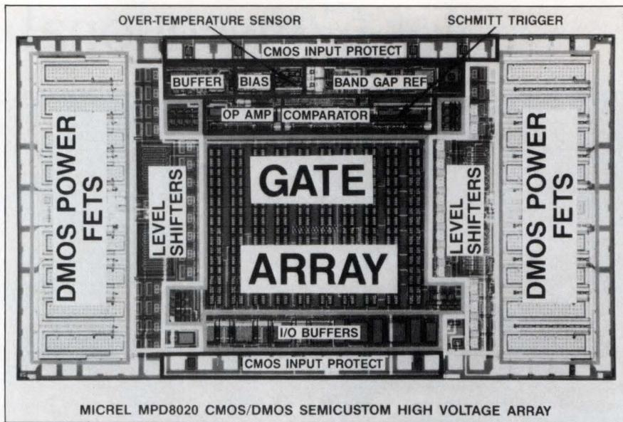
*Employing a modular construction, the MPD-8020 from Micrel includes 16 fully floating 100V/200-mA vertical DMOS transistors, 16 115V/20-mA level shifters, 200 CMOS gates, 12 TTL/CMOS I/O buffers, three op-amp/comparator cells, and a bandgap reference.*
