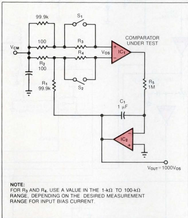
**Fig 1**—The conventional op-amp test circuit lets you measure  $V_{OS}$ ,  $I_B$ , and  $I_{OS}$ . By varying  $V_{CM}$ , you can measure these parameters' sensitivity to common-mode voltage.
