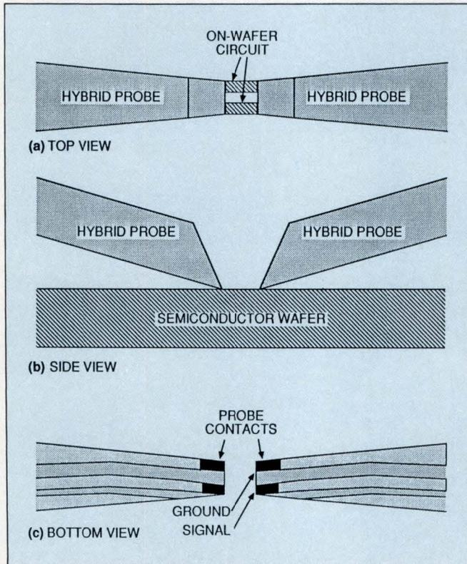
**Fig 8—A new type of high-frequency probe** maintains good transmission-line qualities all the way to the probe tip by using tapered parallel strip lines on a ceramic base. The two outside strips are connected to ground.
