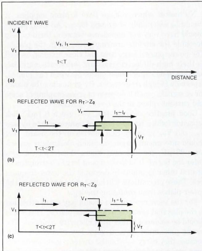
**Fig 4—Line terminations won't have any effect on initial current flow impressed on a transmission line that is relatively long for the signal rise time (a). For shorter lines that are improperly terminated, the reflected wave will either add (b) or subtract (c) from the incident wave, depending on whether the reflected wave is in phase or out of phase.**
