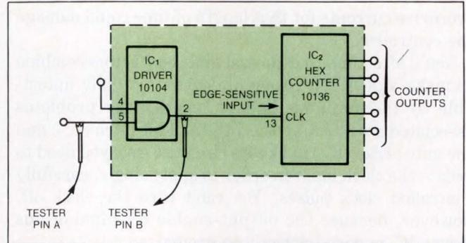
**Fig 4—ECL counters must have very fast edges to avoid false triggering. No tester could produce a fast enough edge by overdriving  $IC_1$  (via test probe B) because of the stray capacitance added by the probe. You can test the two ICs as a cluster via test probe A, however.**
