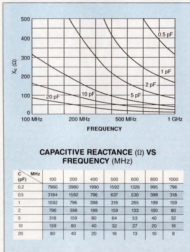
Fig 5—Impedance associated with capacitive reactance varies with frequency. The lower the reactance, the higher the susceptance and the greater the loading of the circuit under test.
