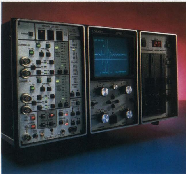
*A disk-drive plug-in for Nicolet's 4094 allows you to store many waveforms and run extensive analysis programs on them.*
