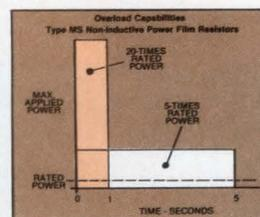
For even higher overload situations, Type MS resistors can be subjected to 20-times the rated power for one second.
