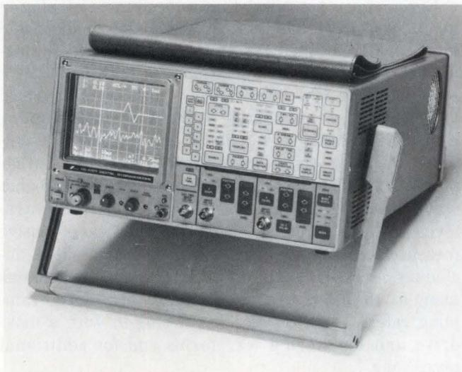
*Go/no-go testing of waveforms allows Iwatsu's 6121A to capture glitches.*
