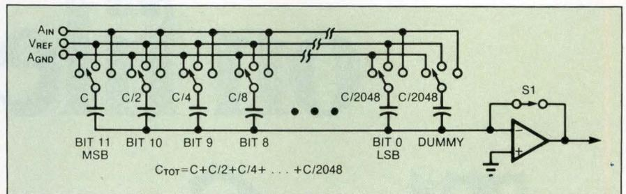
**Fig 1**—A charge-redistribution D/A converter employs an array of binary-weighted capacitors rather than a resistor-ladder network to effect a D/A conversion. One advantage of the capacitor approach is that it eliminates the laser-trimming process step that the resistor-ladder method requires.
