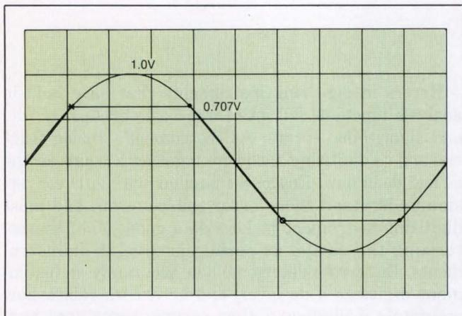
*Fig 1—Different interpolation schemes introduce different amounts of error when determining waveform characteristics that occur between sample points. For example, straight-line interpolation could result in an error of as much as 30% when the algorithm is estimating the peak of this waveform.*
