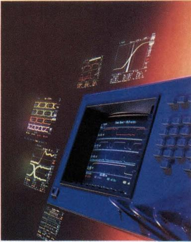
*On the cover: Digital storage oscilloscopes can no longer be considered niche-market instruments. DSOs now feature 1-GHz bandwidths and digitizing rates to 1G samples/sec; prices have also dropped during the last couple of years. See pg 90. (Photo by Reg Francklyn; art direction by John Aylor; photo courtesy Hewlett-Packard)*
