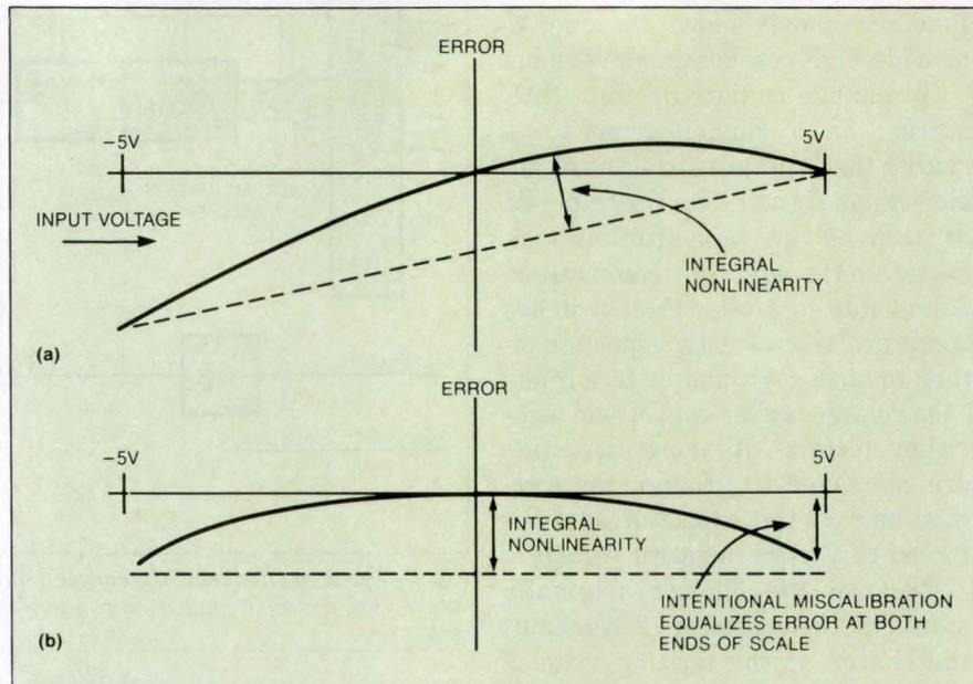
**Fig 3—**You can distribute the integral nonlinearity of the AD1170 A/D converter in a way that minimizes the nonlinearity for positive voltages (a), or you can distribute the nonlinearity over the entire operating range of the ADC (b).
