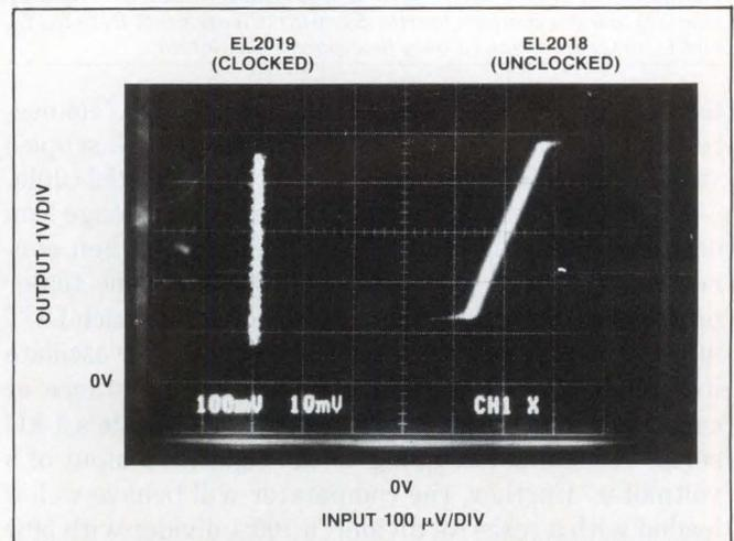
**Fig 5**—This double-exposure photo shows the transfer functions for the EL2019 comparator (while its internal master-slave flip-flop is being clocked) and the EL2018 comparator (while its internal latch is being held in the transparent, or unlocked position).
