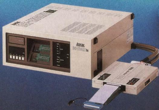
Ziltek continues to meet the growing needs of technology with the ICE-ENGINE/bx-8, a new generation of real-time In-Circuit Emulators.
