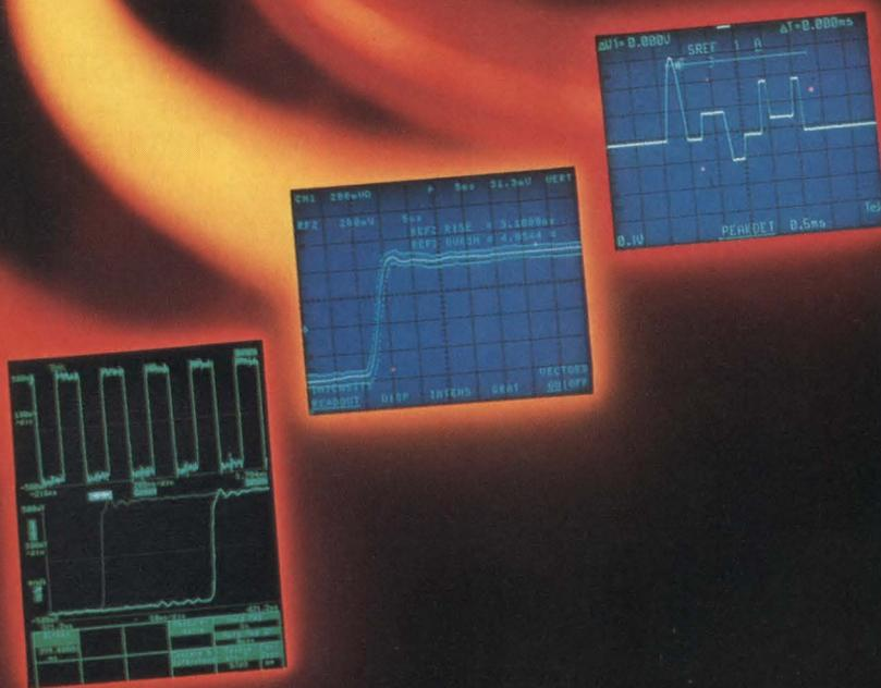
*Offering a spectrum of measurement features, such as manual or automatic cursor measurements, linear and curve interpolators, pretriggering and post-triggering, and equivalent time sampling, the latest digital storage oscilloscopes provide bandwidths to 1 GHz and digitizing rates as high as 1G samples/sec. (Photo courtesy Tektronix Inc)*
