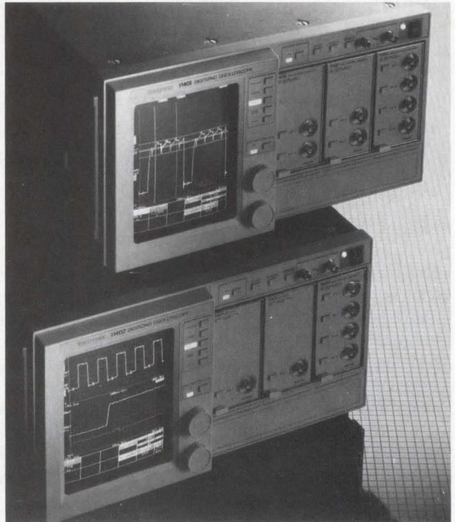
*The 1-GHz bandwidth of Tektronix's 11402 and the 500-MHz bandwidth of the company's 11401 combine with the scopes' 10-bit vertical resolution and 10-psec horizontal resolution to give you precision measurement capability.*
