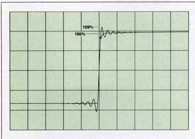
**Fig 2—Gibbs's phenomenon results in overshoot** when the digitizing instrument performs waveform reconstruction with a sinc function on nonbandlimited data. In this example, Gibbs's phenomenon causes an error of 9% for a nonbandlimited signal.
