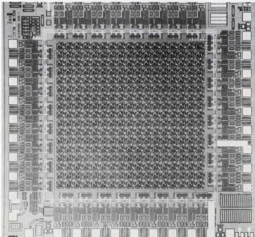
*Composed of matrix cells and peripheral cells, the ULA-6P from Ferranti Interdesign includes 578 gates, 281 npn transistors, and 300 resistors with a combined value of more than 37 M $\Omega$ . Unlike Ferranti's G Series, the P Series emphasizes applications requiring more digital functions.*
