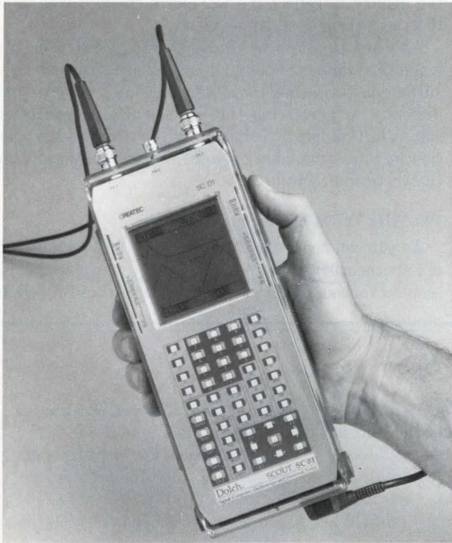
**Packing a surprising amount of capability** into a 25-oz, handheld DSO, Dolch's SC01 gives you two 5-MHz channels that sample at 20M samples/sec simultaneously and provide cursors and readout.
