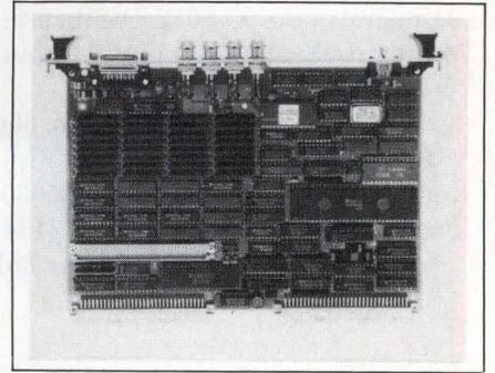
ously displaying 16 colors from a palette of 64k colors. Video output is via RGB and composite sync outputs. Graphics capabilities include hardware zoom, vertical and horizontal smooth scrolling, clipping, hitting, blinking, and conditional blinking. A light pen interface is also provided. A software package for GKS (Level 2b) support, operating under Unix or the PDOS real-time operating system, is currently being ported to the board. Around DM 3400.
