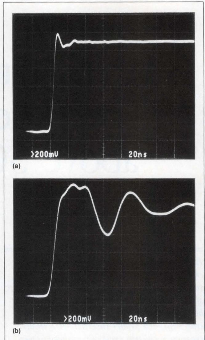
**Fig 1—Loading a 500Ω impedance source with a 10-MΩ, 10-pF probe produces a 6-nsec rise time (a). Replacing the probe with two 2m lengths of hookup wire changes the loading to 1 MΩ and about 20 pF, and slows the rise time to about 10 nsec—in addition to ruining the transient response (b).**
