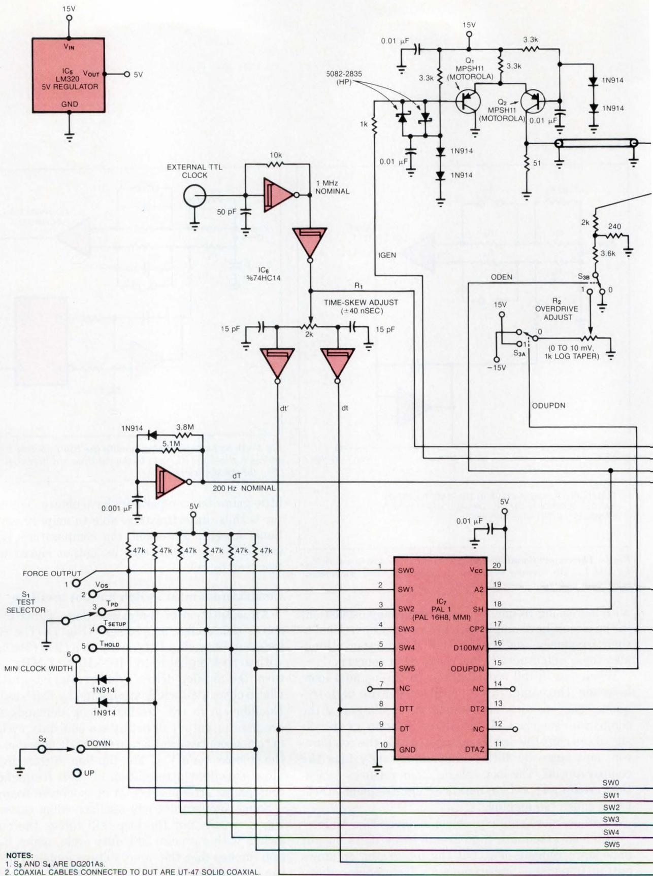
**Fig 3—This comparator-test circuit incorporates the basic loop of Fig 2, but uses two programmable-array logic chips (IC<sub>7</sub> and IC<sub>8</sub>) for sequencing the tests.**
