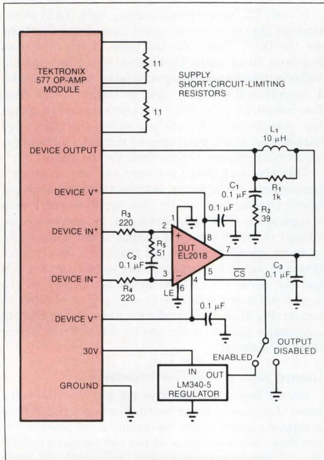
**Fig 6**—This test circuit shows the brute-force methods necessary to modify an op-amp tester (Tektronix's 577 curve tracer with op-amp module) to test a comparator (the EL2018). Components  $R_1$  to  $R_5$ ,  $L_1$ , and  $C_1$  to  $C_3$  are required only to suppress oscillation.
