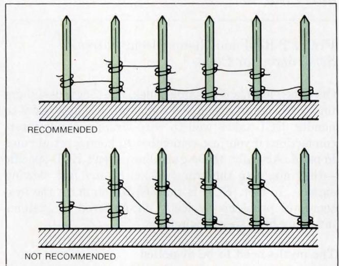
**Fig 2—To simplify any reworking, you should make sure that a wire that starts at one level on a wire-wrapped pin travels to the same level on the pin at the other end of the run.**
