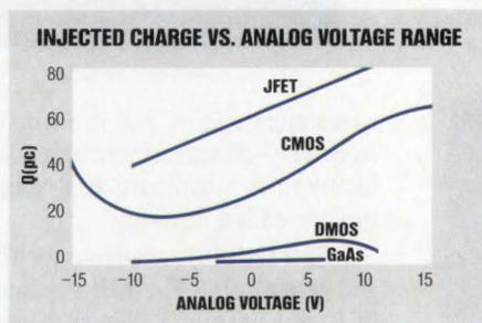
*Circuit accuracy is a function of charge injection. The DMOS process significantly outperforms CMOS, JFET and bipolar in this critical parameter.*
