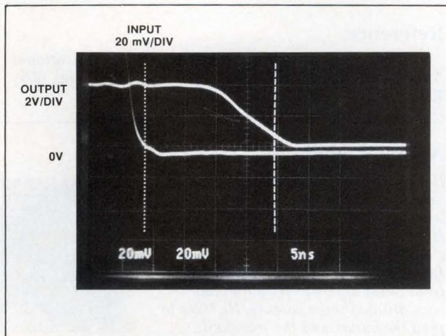
**Fig 4**—This scope photo shows the propagation delay for an EL2018 comparator by displaying the output waveforms (attenuated by a factor of 100) and the input waveforms. **Fig 3** shows the actual test setup.
