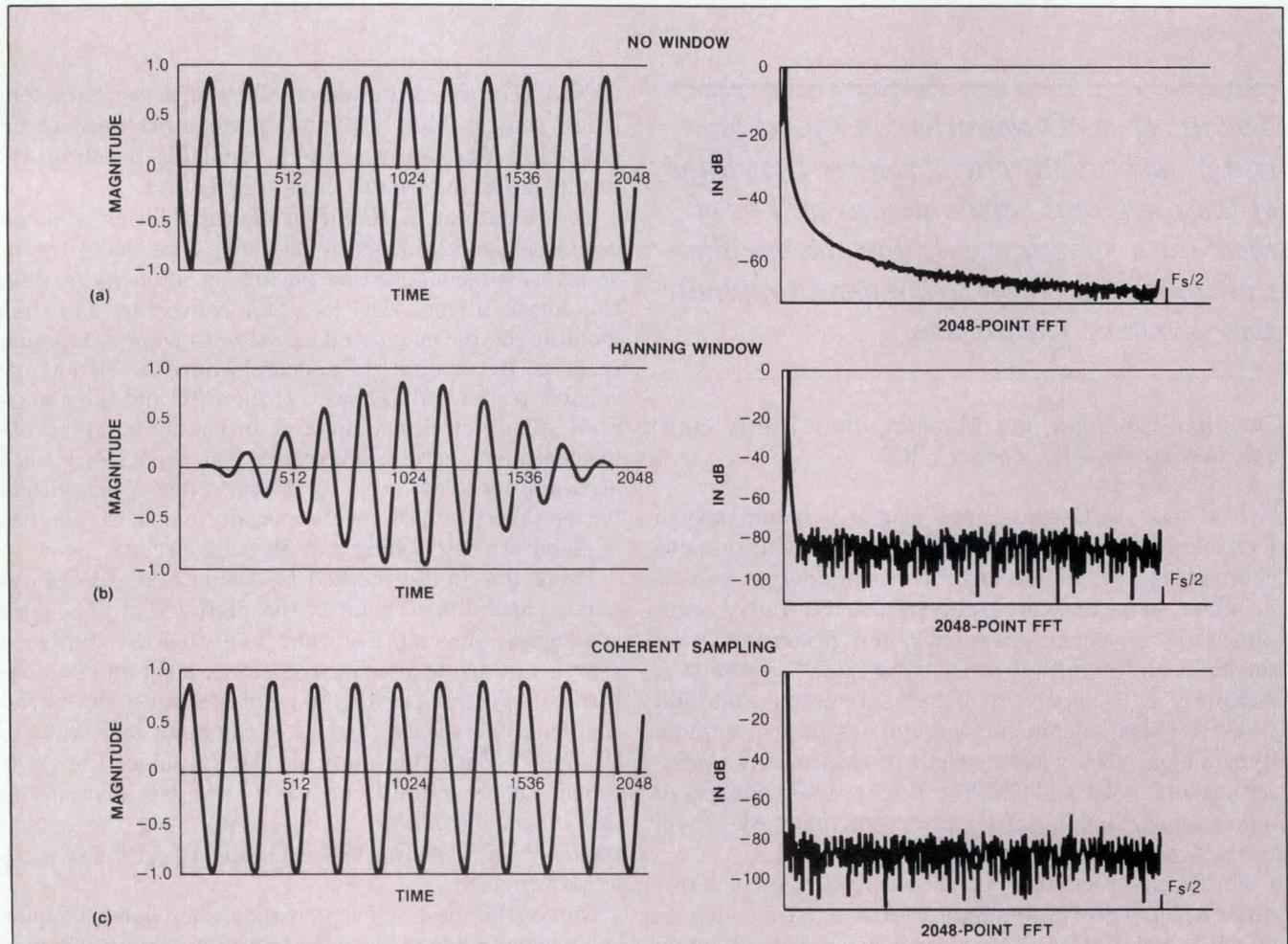
**Fig 1—A 10-bit A/D converter took these samples. Noncoherent sampling without window compensation is shown in (a), noncoherent sampling with a Hanning window is shown in (b), and coherent sampling is depicted in (c).**
