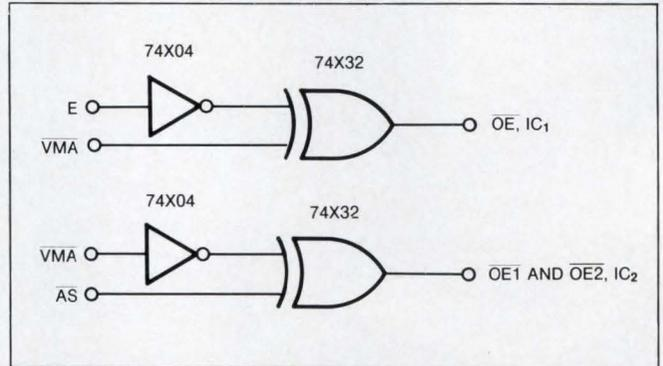
Fig 2—These circuits show an alternate way to derive the output enable (OE) signals required for buffers IC<sub>1</sub> and IC<sub>2</sub> in Fig 1.
