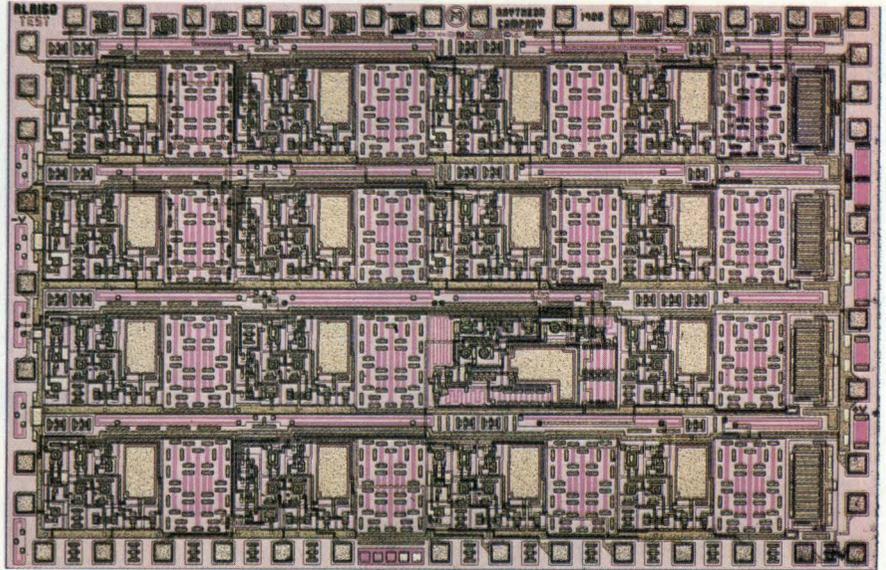
*A relative newcomer to the linear semicustom field, Raytheon has recently introduced the RLA160 macrocell array. Among its other components are 15 user-configurable gain cells (each containing 10 transistors) and four large (200-mA) npn transistors. The thin-film resistors used in this array exhibit better tolerance and temperature-drift characteristics than do the diffused resistors used in most semicustom chips.*
