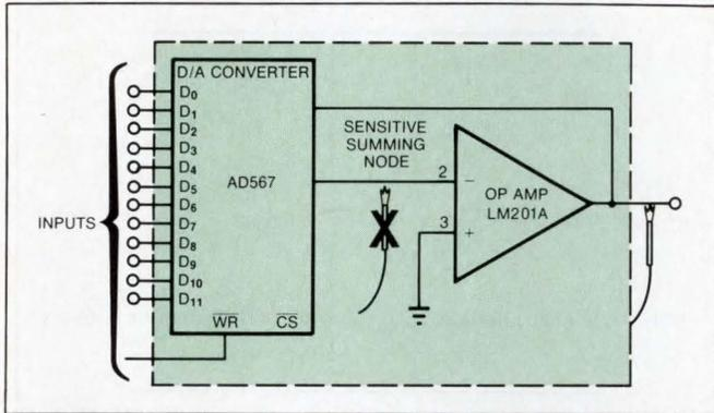
**Fig 5—In this circuit, you can't test the op amp in its linear region because capacitance added to the summing junction by the probe will make the op amp oscillate. You can test the D/A converter and the op amp as a cluster, though.**
