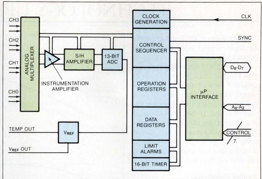
**Fig 2**—The area efficiency of a charge-redistribution DAC allows the ML2200 ADC chip to incorporate an input multiplexer, sample/hold amplifier, and  $\mu$ P interface on a single chip.
