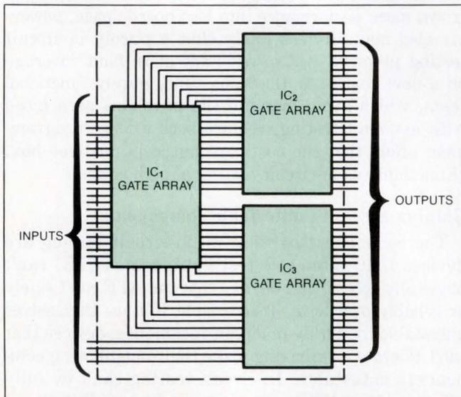
**Fig 1—You can't perform in-circuit tests of either IC<sub>2</sub> or IC<sub>3</sub> in this circuit, because overdriving so many outputs of IC<sub>1</sub> would overheat and damage IC<sub>1</sub>.**
