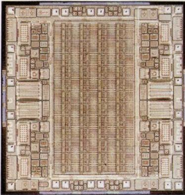
*Linear and linear-digital semicustom ICs can operate at VHF and UHF frequencies and high voltages. Moreover, many of the linear devices include built-in gates that you can use to implement digital functions on the same chip (pg 57).*
