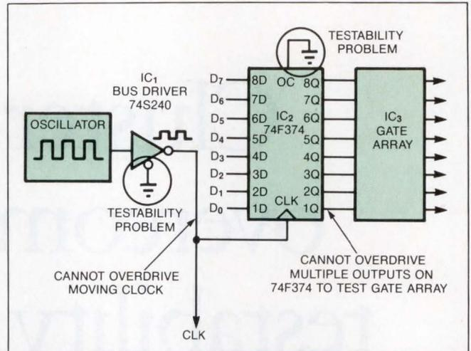
**Fig 2—This circuit is untestable by in-circuit means. You can't turn off the clock to test IC<sub>2</sub>, nor can you turn off the outputs of IC<sub>2</sub> to test IC<sub>3</sub>. Trying to overdrive a clock signal produces unrepeatable results; overdriving multiple outputs of IC<sub>2</sub> would damage it.**
