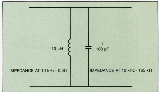
**Fig 6—Some components are invisible to a tester.** At 10 kHz, the 165-k $\Omega$  impedance of the capacitor is shunted by the 0.6 $\Omega$  impedance of the inductor—an impedance ratio of 275,000:1. An in-circuit test can't separate the two; only a frequency-response test will reveal whether the capacitor is present and has the right value.
