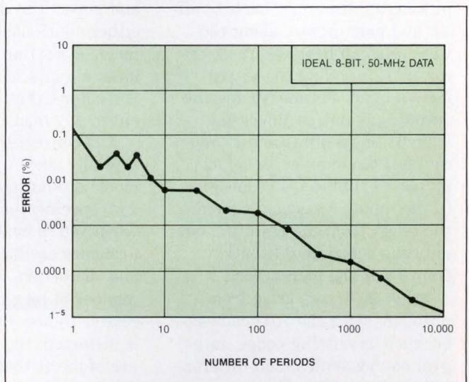
**Fig 3—This plot of worst-case timing error** (arising from the quantization-error component of total estimation error) shows that frequency estimation becomes more accurate, in a linear fashion, as the gate time increases. The sample rate remains constant, thus increasing the number of samples analyzed.
