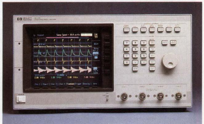
**Four channels operating at 400M samples/sec simultaneously** and a 64k-word memory on every channel allow Hewlett-Packard's 54112D to capture long, high-speed waveforms in real time.
