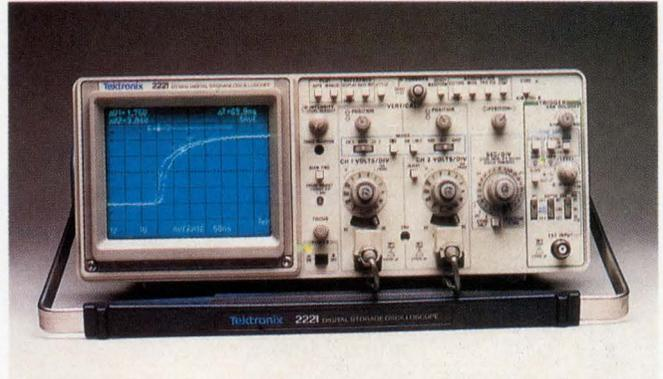
*Analog and digital functions are combined on Tektronix's 60-MHz 2221; this feature is common in many DSOs that offer bandwidths of 100 MHz or less.*
