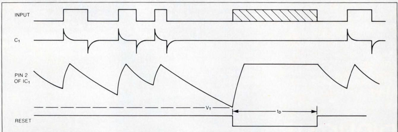
Fig 2—The waveforms of Fig 1's watchdog circuit show that a signal from the CPU (connected to the Input) prevents a system reset by repeatedly jerking the pin 2 voltage away from IC<sub>1</sub>'s  $V_T$  switching threshold. A malfunctioning CPU will allow the voltage to reach the threshold, producing a reset.
