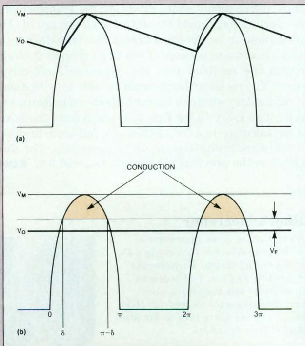
**Fig A—You are incorrect if you assume** that the filter capacitor charges to  $V_M$  at the peak of the rectifier output as **Aa** shows. **Ab**'s correct model of filter-capacitor operation shows current flowing only when the transformer's output voltage exceeds the supply's output voltage (plus the forward-voltage drop of the series diode).
