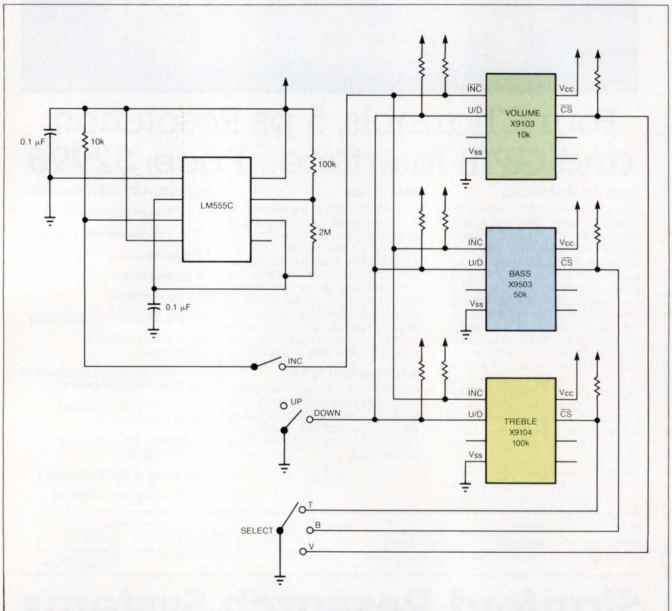
**Fig 9—This breadboard circuit** uses a 555 timer to supply a slow clock-pulse to the increment pin of each X9MME through a momentary switch. Pull-up resistors connect to each digital line, and grounding switches connect to the up/down and chip-select pins. Each step of the clock produces a 1% change in the wiper position.
