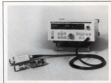
dynamic range of -70 to -20 dBm. You need only one sensor diode for these ranges. The instrument reads out in W, dBm, or dB in absolute or differential modes. The front panel features both an LED display and an analog meter. The instrument has a built-in, 50-MHz calibration source. An IEEE-488 interface is standard. ML4803A, \$2825. Sensors: amorphous, \$550 to \$1200; diode, \$840 to \$1315; millimeter waveband, \$1900 to \$6600.
