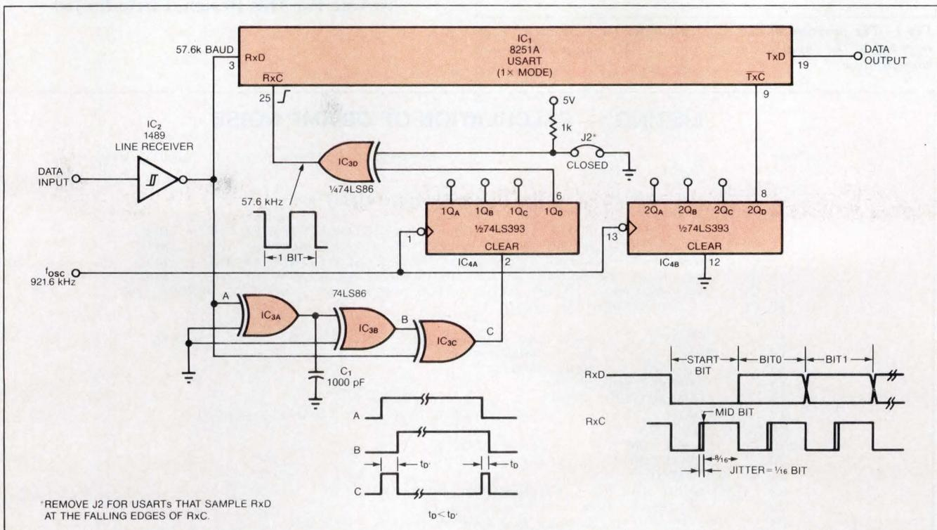
Fig 1—By using synchronized dividers and a free-running local oscillator, this USART circuit operates in the 1× clock mode without requiring a separate clock line.
