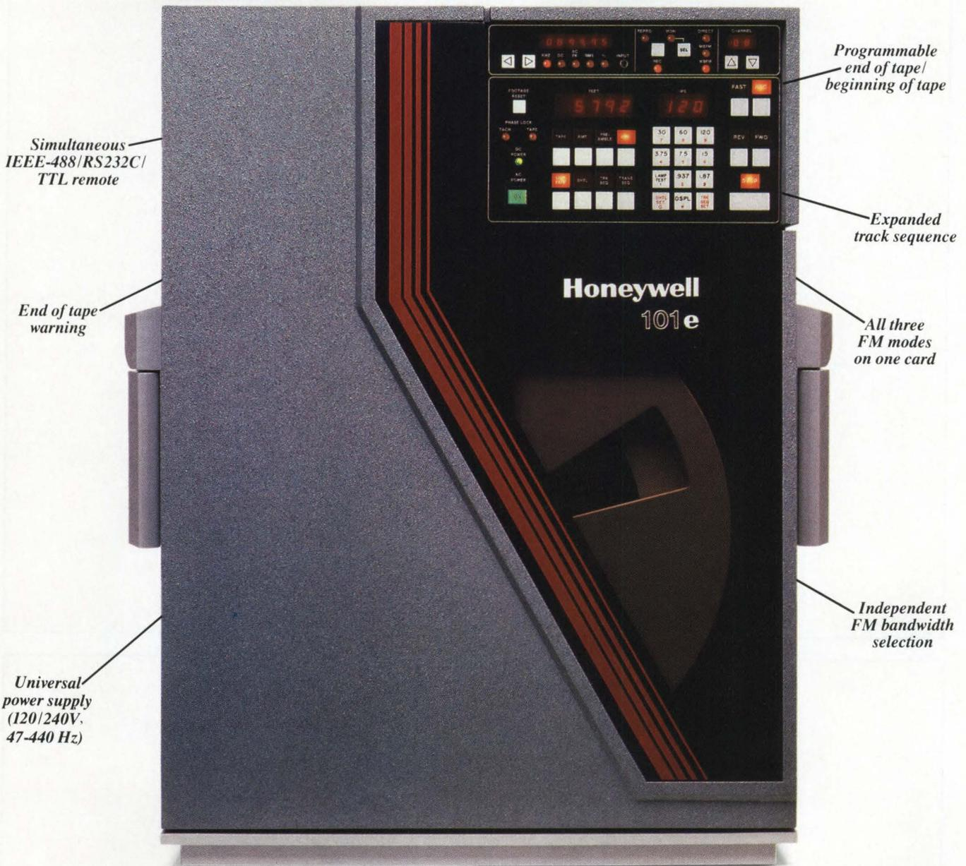
Introducing the Honeywell Model 101e—an enhanced version of the rugged Model 101 that has proven its reliability in a wide range of applications over many years.
