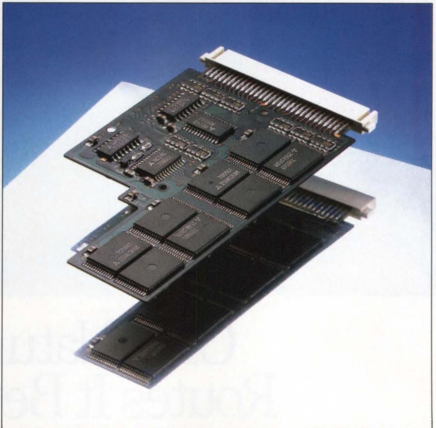
*This smart card has a 4-layer pc board and 16 VSOP ICs, which have built-in ESD protection to 25,000V. The female 2-P connector mates with male pins to provide a gas-tight seal. The card, available from Mitsubishi Electronics, can provide as much as 512k bytes of battery-backed static RAM or a maximum of 2M bytes of masked ROM.*
