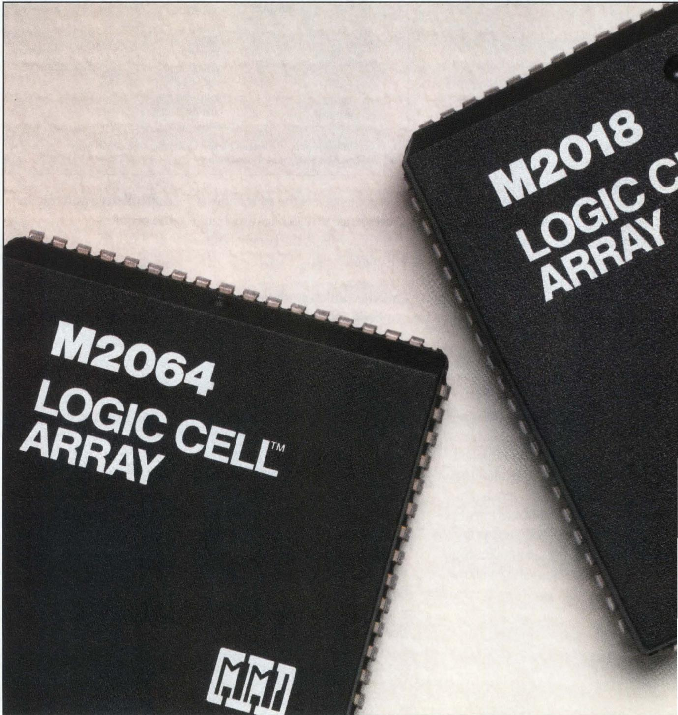
Easy answer: the Logic Cell™ Array (LCA). A new, field-programmable CMOS gate array that has a flexible, wide-open architecture. Along with true VLSI-level density.
