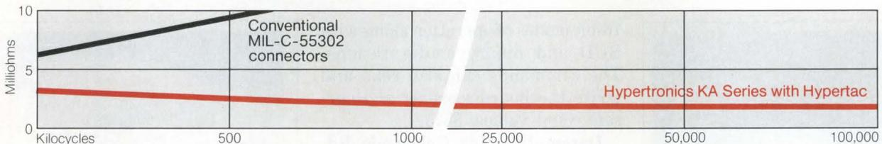
Low-force contacts for MIL-C-55302 qualified connectors, still going strong after 100,000 connect/disconnect cycles, should be good news for high life-cycle applications.
