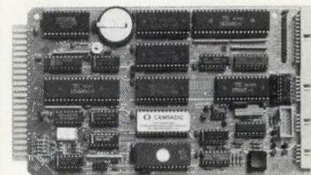
**SBS-1000** has turbo speed, 20K industrial BASIC. Runs 5 times faster than BASIC-52 systems. All CMOS with Z80 CPU, EPROM/EEPROM programmer, 96K static RAM, 2 RS-232C serial ports, 32 lines digital I/O, 4 channels-12 bit A/D, battery backed calendar clock, keypad and display ports, expansion port, autorun mode, interrupts handled by BASIC, industrial quality, 5V and stand alone operation. From **\$396** in 100s.
