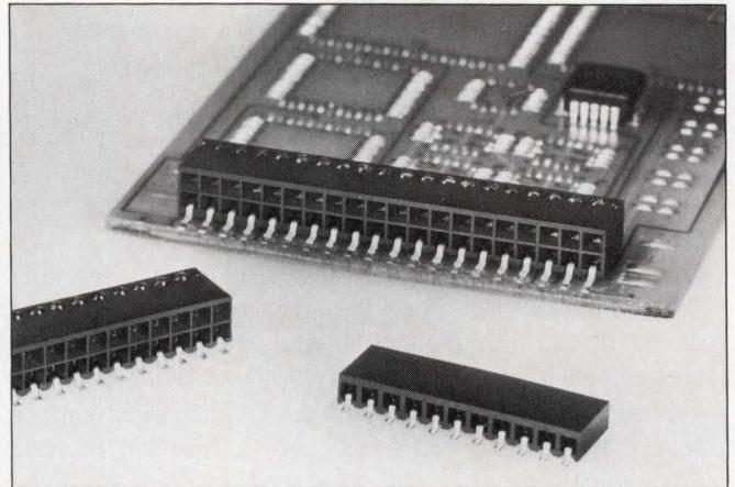
*Floating contact legs ensure positive contact of Du Pont's surface-mounted horizontal card connectors, even when you mount them on an uneven pc board. You can order either single- or double-row configurations and 0.38- or 0.76- $\mu$ m plating thicknesses.*
