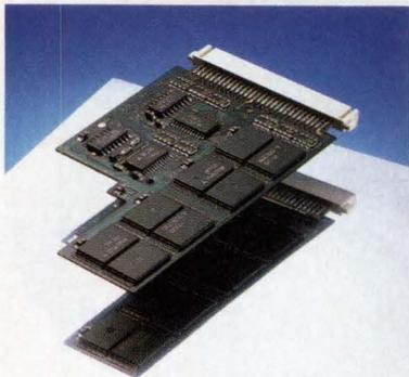
You can use smart cards for applications ranging from customization of terminals and peripherals to mass storage for computers that must run in hostile environments (pg 61).
