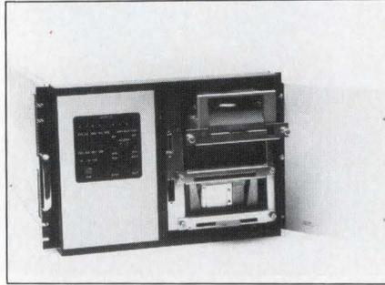
The SA-H155 incorporates a 14-slot Q bus backplane for use with either LSI-11 Series or MicroVAX systems. Five fans help secure a good wash of air over the backplane, power supply, and drives. Two of
