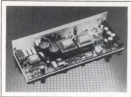
maintaining two outputs are rated at 5A each with 7A peak loads. The supply features built-in overload and overvoltage protection and remote sense capability. \$251 (100). Delivery, three to six weeks ARO.
