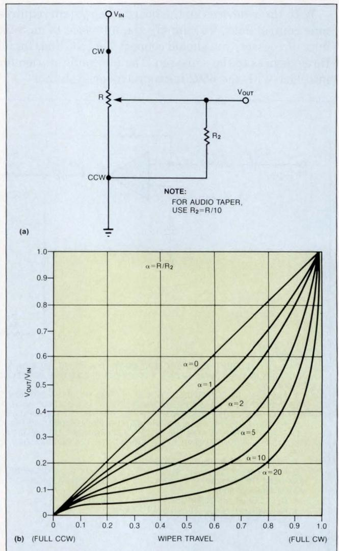
**Fig 8—A shunt-resistor from the wiper of the potentiometer to ground (a) can simulate various logarithmic tapers when used with a linear pot. The graph (b) plots the resulting curves as a function of the resistor ratios.**
