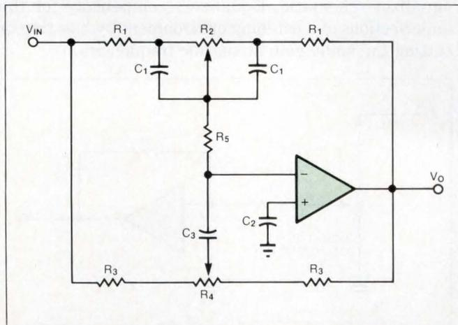
Fig 2—The Baxandall filter circuit is commonly found in high-quality audio systems. Potentiometers control the gain of an active filter to boost or cut either bass or treble frequencies.
