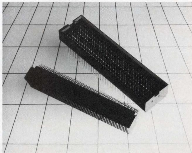
*Suitable for use with controlled-impedance backpanels, Augat/Elfab's 6-row Double Din connector boasts a mere 0.070-in. variation in the length of its conductor paths. Offering a density of 60 contacts per linear inch, this connector provides 200 to 300 individually replaceable contacts that are available in a variety of lengths and plating options.*
