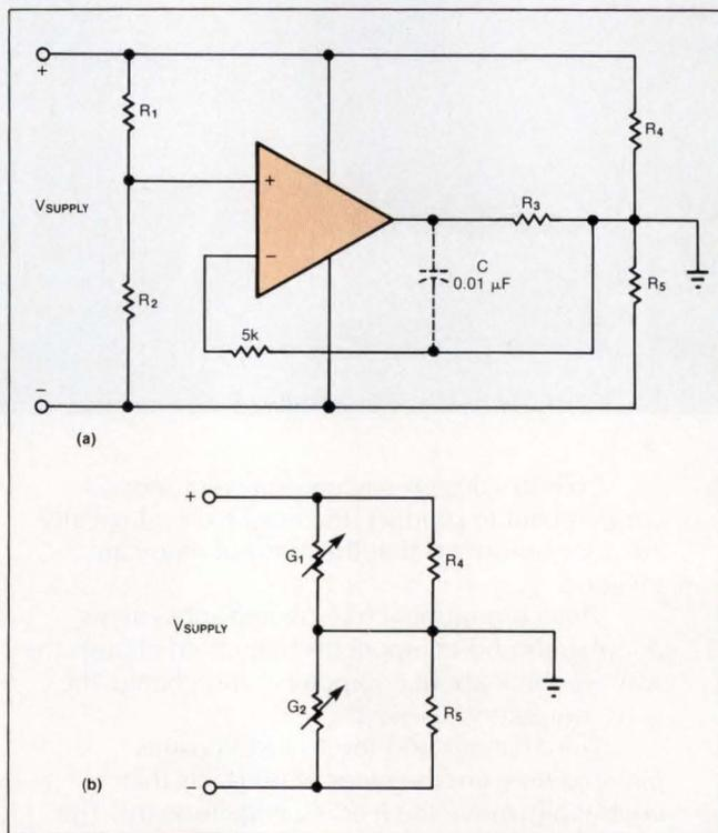
Fig 1—This circuit (a) splits a single supply into a bipolar supply and regulates the resulting voltages according to the relative magnitudes of  $R_1$  and  $R_2$ . The action of the op amp is equivalent to that of the variable conductances across each load resistor (b).
