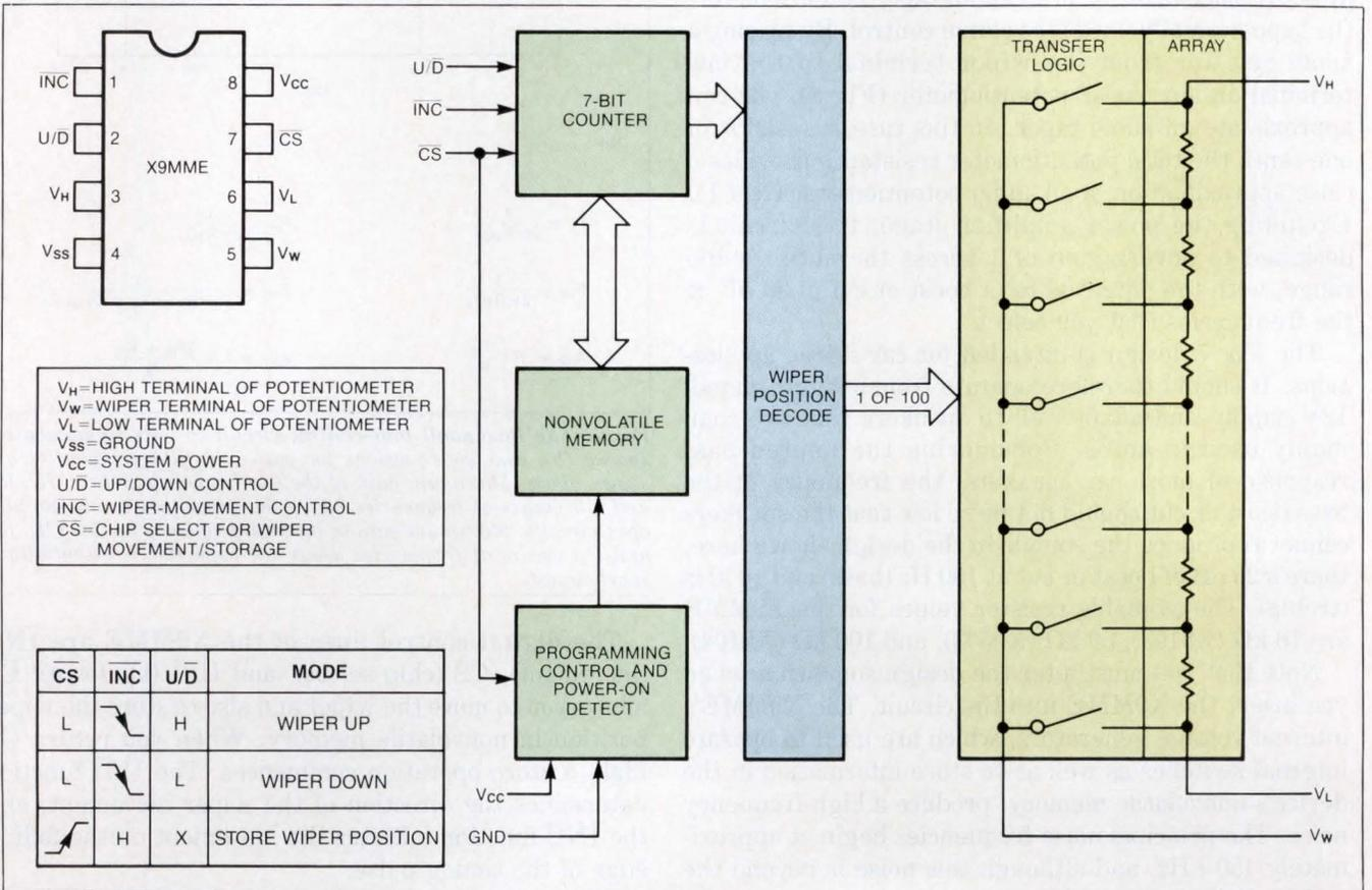
Fig 5—Digitally controlled potentiometers, such as the X9MME from Xicor, offer an alternative solution for microprocessor control of signal levels without the need for A/D and D/A converters. The X9MME combines a 99-position potentiometer with internal counter circuitry for wiper position control, and a nonvolatile memory that retains the wiper's position. It provides a conventional 3-terminal design that easily integrates into conventional designs.
