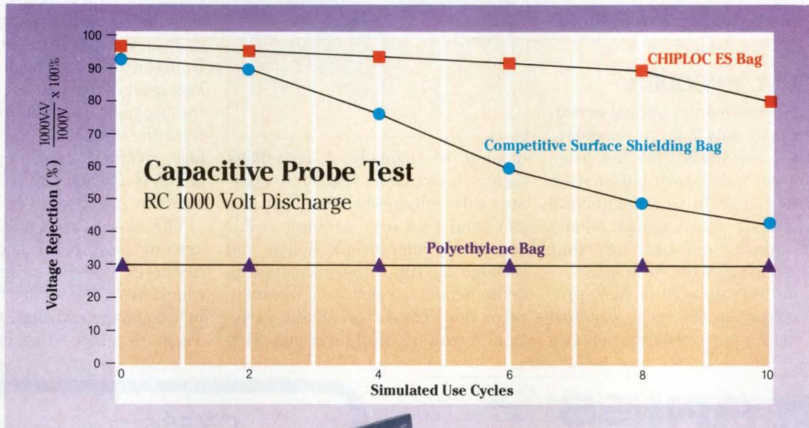
Capacitive probe tests show that CHIPLOC\* ES static shielding and dissipative packaging from Dow has up to 80% more shielding capability than the leading surface shielding bag on the market.
