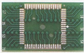
*DENSEPAK adaptors design uses no more than 25% board space than the actual chip by routing the traces under the chip.*
