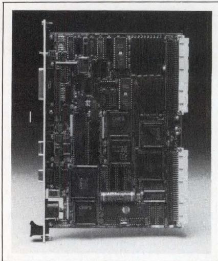
for enhanced color and monochrome graphics. The board contains the following features: a P1 VME Bus Interface, A24/D16; a P2 IBM PC/AT bus interface; a 10-MHz 80286  $\mu$ P; an 80287 coprocessor socket; a 1M-byte dynamic RAM dual-ported between the VME Bus and the 80286; and a socketed ROM BIOS (basic I/O system). By making the PC/AT bus accessible through the 96-pin P2 connector, a series of compatible support functions can be used. \$2200.
