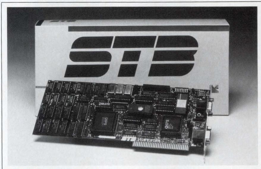
CGA, the MDA, and Hercules Graphics, the device provides a 132-column display with high-quality text (an 8×14 character cell) in spreadsheet and terminal-emulation
