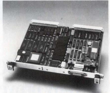
*Using bus transceivers and pipeline registers to isolate processor functions and maximize bus-activity efficiency, the Eagle VME Bus/Ethernet controller board can transfer data at speeds exceeding 30M bytes/sec.*
