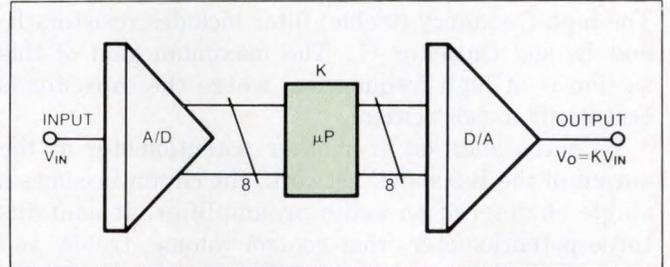
Fig 4—One method of controlling analog-circuit functions is with A/D and D/A converters using a microprocessor interface. Although it's effective, this method is complex and costly.
