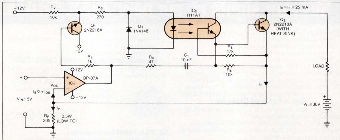
Fig 2—This voltage-controlled current source uses an optocoupler (IC<sub>2</sub>) to eliminate an error found in more conventional circuits and which is caused by the output transistor's base current.
