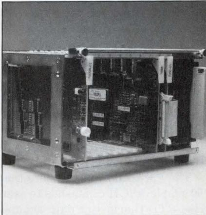
and airborne particles pose potential hazards. Model 20 has 128k bytes of CMOS static RAM (expandable to 640k bytes) and one 3½-in. floppy-disk drive; a second floppy-disk drive and a 3½-in., 20M-baud
