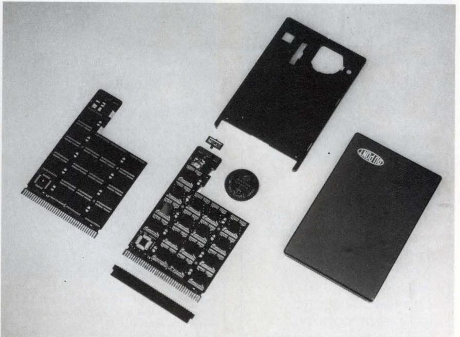
*A credit-card-sized memory cassette from Du Pont comes in RAM and ROM versions and can store as many as 1M bits. The replaceable 3V lithium battery retains data for at least 2½ years. The card is fully protected against EMI and static discharge.*
