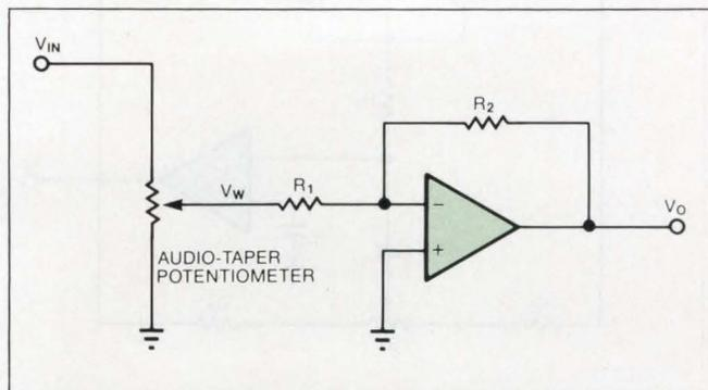
**Fig 1—Volume controls are usually simple potentiometer and resistor circuits. In this circuit, the potentiometer controls the signal level to a fixed-gain amplifier.**
