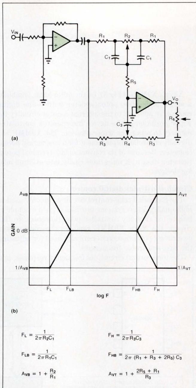
Fig 6—The Baxandall tone-control circuit (a), its frequency response (b), and the equations for gain and filter-frequencies are shown above. Maximum gain of the low-frequency section ( $R_1$ ,  $R_2$ , and  $C_1$ ) occurs at frequencies where the capacitors are essentially open circuits. Maximum gain of the high-frequency section ( $R_3$ ,  $R_4$ , and  $C_3$ ) occurs at frequencies where the capacitor is essentially a short circuit.
