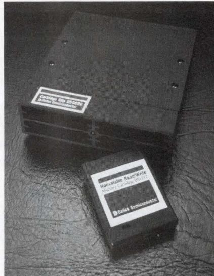
*You can put as many as eight memory cartridges into this cartridge clip from Dallas Semiconductor. The assembly fits into the space of a half-height, 5 1/4-in. disk drive and yields a storage capacity of 4M bytes of RAM. The access time is 250 nsec.*
