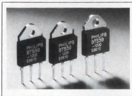
BTR59 Series currently comprises two devices with voltage ratings of 800 and 1300V; both have a circuit commutation turn-off time of  $1 \mu\text{sec}$ . Both series have a maximum controllable anode current of 50A. The thyristors are packaged in SOT-93 encapsulations. Around \$5.
