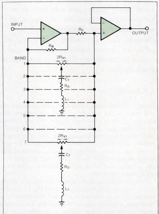
Fig 3—In a graphic equalizer, each filter has its own potentiometer to control the gain to a particular bandpass section. The potentiometers normally appear as sliders on the face of the equalizer.
