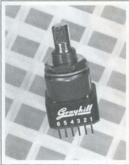
tion of rotation as well as the number of steps. You can design the software to translate the code to cursor movement on a screen or to change the value of a system parameter. The Series 61 rotary encoder switch is available with 16 or 24 detent positions. Approximately \$20. Delivery, four to six weeks ARO.
