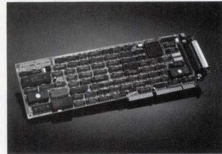
Capable of synchronous and asynchronous data-transfer modes, the AHA-1540 SCSI host adapter accommodates the high-performance disks needed for multiuser, multi-tasking IBM PC/AT bus applications.
