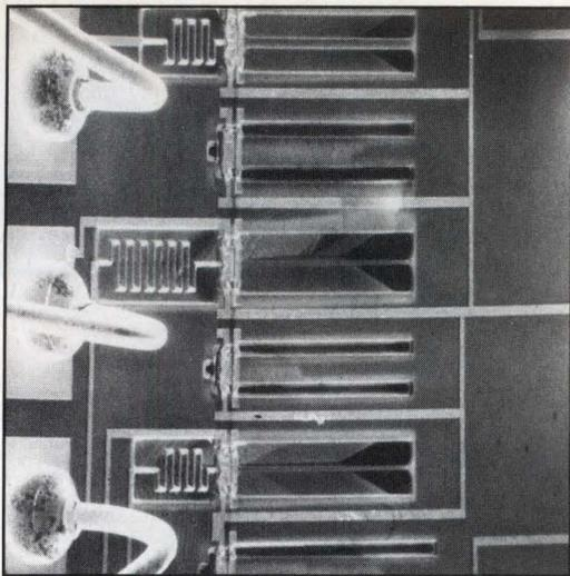
*Acceleration Switches: Cantilever beams of silicon dioxide overhang shallow wells in silicon. Beams flex under acceleration, making electro-mechanical contact.*
