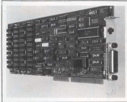
Intel/Microsoft expanded-memory specification. The board can also emulate Tektronix and Hewlett-Packard controllers. With no memory, \$795; with 1M bytes of memory, \$995.
