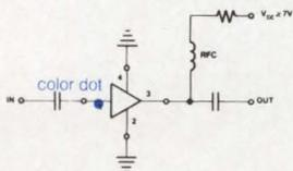
Unbelievable, until now... tiny monolithic wide-band amplifiers for as low as 99 cents. These rugged 0.085 in. diam., plastic-packaged units are 50ohm\* input/output impedance, unconditionally stable regardless of load\*, and easily cascadable. Models in the MAR-series offer up to 33 dB gain, 0 to +11dBm output, noise figure as low as 2.8dB, and up to DC-2000MHz bandwidth.
