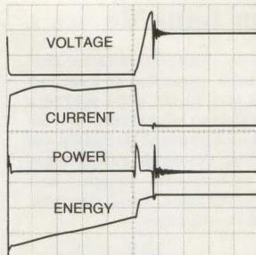
These waveforms show an IS\_SPICE analysis of a power supply snubber. Intu\_Scope was used for display and computation of power and energy. The output shown used an Intu\_Scope plotter utility
