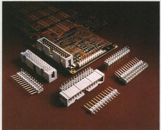
**Preformed solder inlays mounted around each pin** on these connectors from 3M allow the simultaneous reflow and bonding of the connectors' solder tails and surface-mount components during IR or vapor-phase reflow soldering. The vendor claims this scheme combines the speed and economy of reflow soldering with the bond strength of through-hole connector mounting.
