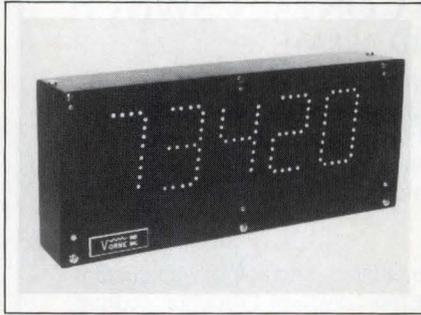
range and overrange analog-input conditions. Two sets of rotary DIP switches are available for scaling the display. One set defines the bottom of the analog-input range, and the other establishes the top. Between the two setpoints, the display is linear.
