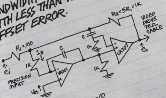
$$\begin{aligned} \text{GAIN} &= e_o/e_i = R_2/R_1 = -10 \\ A-B &= 100 \text{ KHz} - 40 \text{ MHz} \\ \text{'INPUT OFFSET} &= V_{os} + I_B - 2K \\ &= [25 + (40)(1)] \mu\text{V MAX} \\ &= 65 \mu\text{V MAX} \end{aligned}$$
