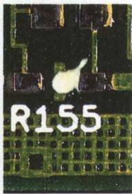
Controlled viscosity eliminates stringing and contamination.
