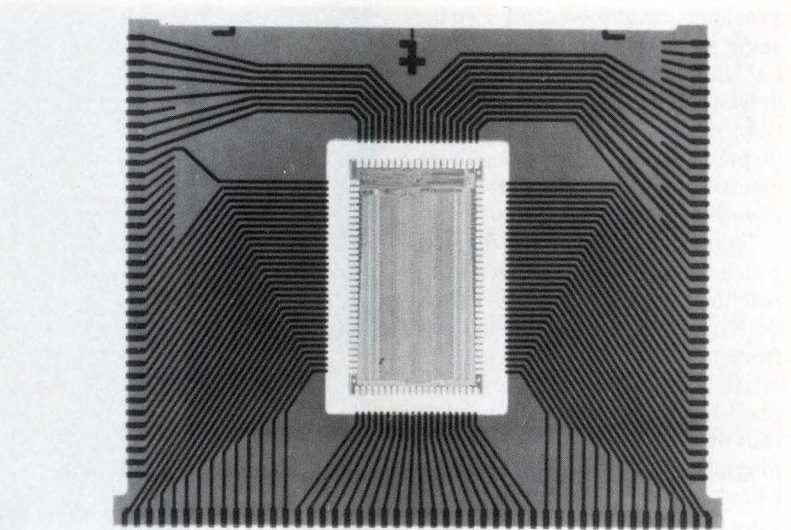
*The tape-automated-bonding package and leadouts of the PCF2201 LCD driver allow you to mount the device on the rear side of a flat-panel display, using single-plane interconnect patterns.*
