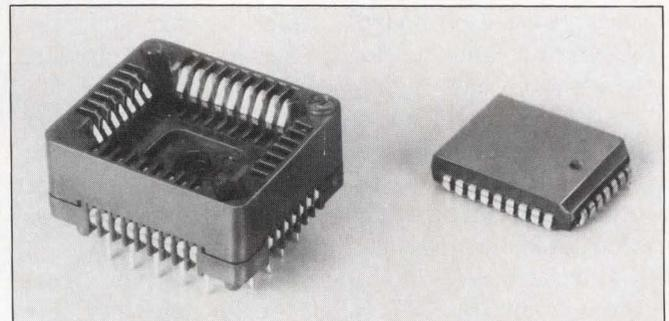
*Many manufacturers offer led chip-carrier sockets—such as this modular 32-pin socket from Methode Electronics—in both through-hole and surface-mount styles.*
