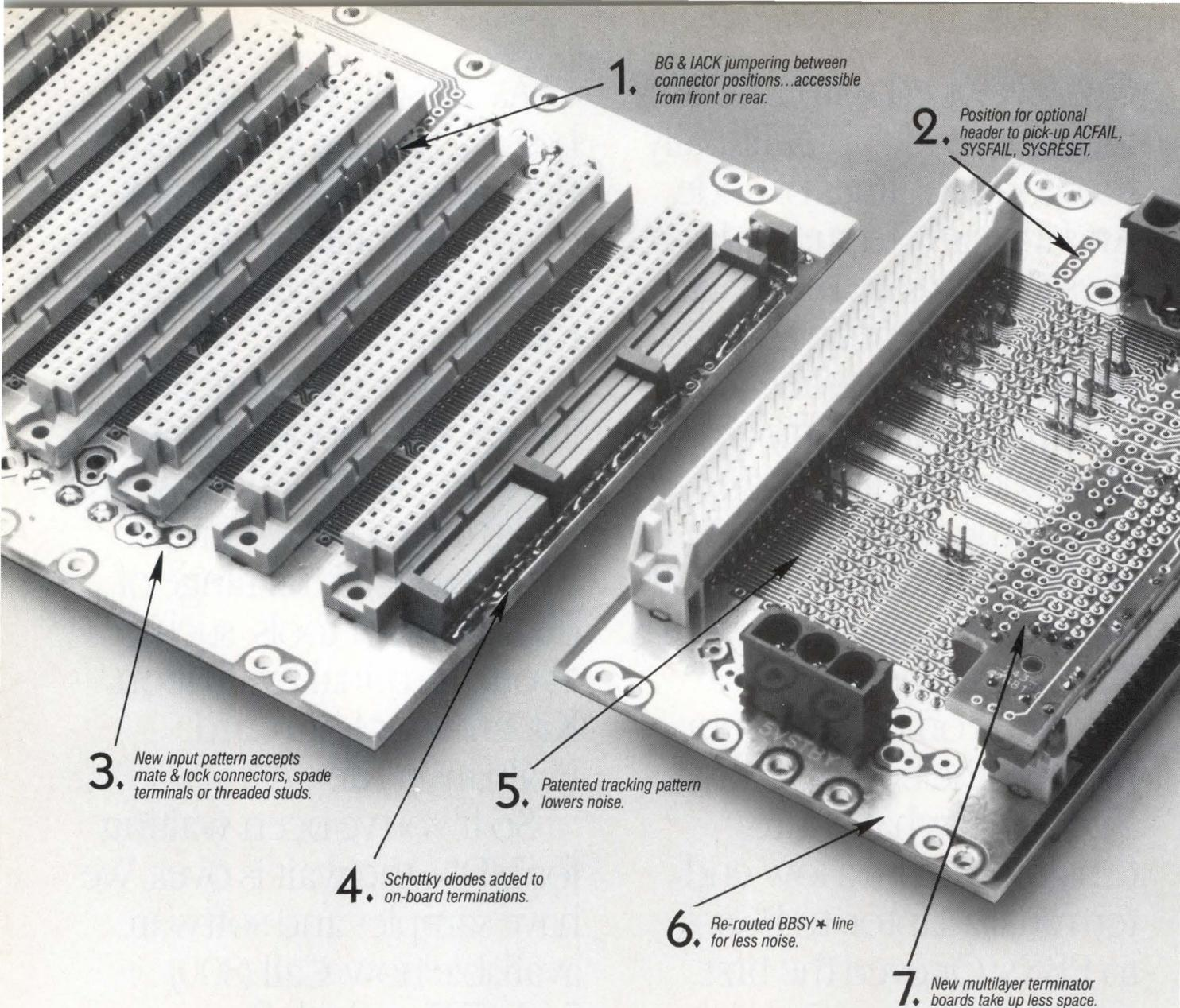
1. BG & IACK jumpering between connector positions...accessible from front or rear.
