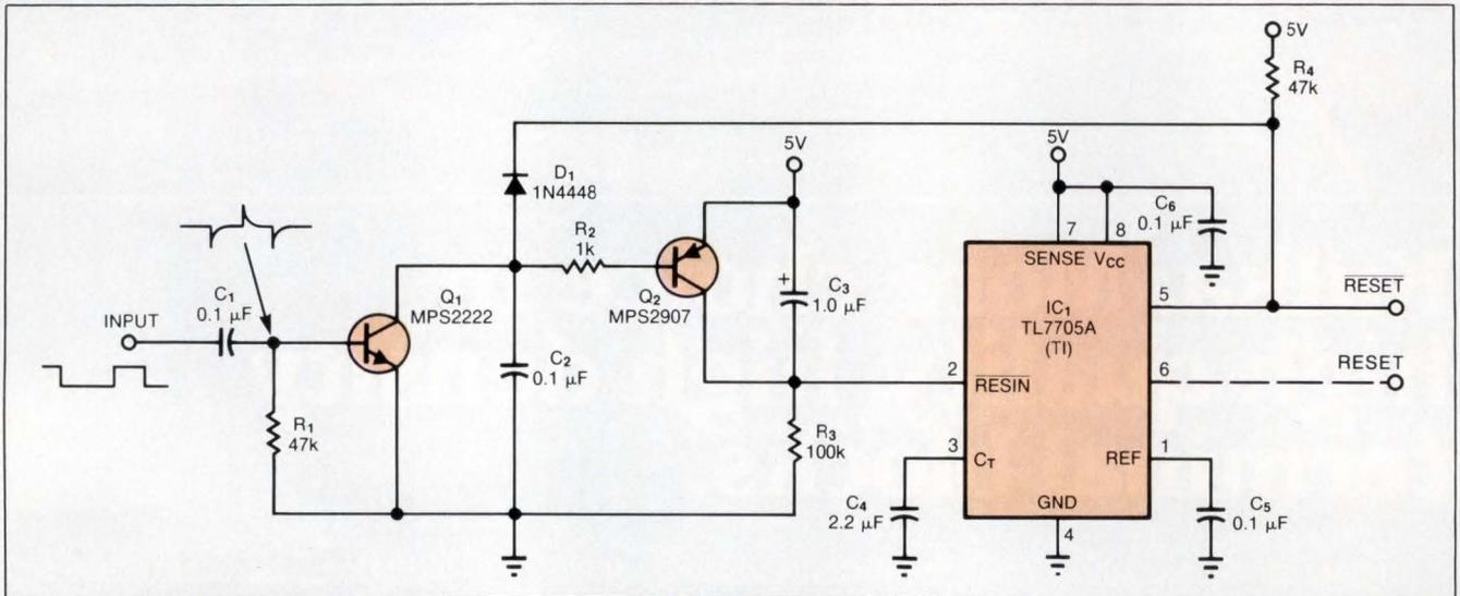
Fig 1—Combining a supply-supervisor chip (IC<sub>1</sub>) with an external watchdog circuit provides protection for a  $\mu$ P system. The circuit issues a system reset in response to a CPU malfunction, a glitch, a low-voltage condition, or a failure of the power supply.
