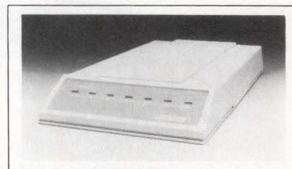
swers. The dial features include Touch Tone or pulse; programmable pause interval; and originate call from answer mode. It meets the CCITT standards for 2400-bps operation, the Bell 212A for 1200-bps, and the Bell 103 for 300-bps operation. It operates with the Hayes command set, which allows a computer or terminal to control the modem using communication software through an RS-232C interface. The modem measures 10.5×5.5×1.3 in. and is designed to fit under a telephone. \$239.
