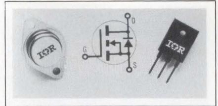
available in two package styles. The IRFAE50, IRFAF50, and IRFAG50 are housed in the TO-3 packages and are rated at 800, 900, and 1000V, respectively. The similarly rated IRFPE50, IRFPF50, and IRFPG50 are housed in plastic TO-3P packages. On-resistance measures 1.2, 1.6, and 2Ω for the 800, 900, and 1000V units, respectively. Continuous-current ratings range from 5.25 to 8.1A for the TO-3 packages and 5.75 to 8.1A for the TO-3P-packaged units. \$11 to \$14 (1000). Delivery, 10 weeks ARO.
