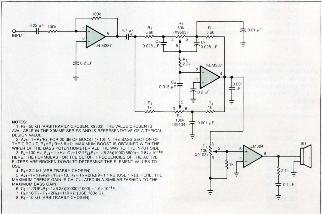
**Fig 7**—In this circuit, X9MMEs replace the conventional potentiometers ( $R_2$ ,  $R_1$ , and  $R_6$ ) of Fig 6 without any alteration of the analog design considerations. Because  $R_2$  and  $R_4$  are both linear-taper potentiometers, the X9MME provides a direct replacement. The volume control ( $R_6$ ) requires a 1-k $\Omega$  shunt resistor from its wiper to ground to simulate an audio taper.
