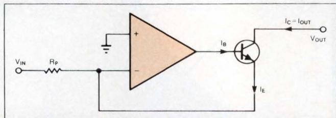
Fig 1—In this simplified V/I converter,  $I_{OUT}$  equals  $V_{IN}/R_P$  minus  $I_B$ , which varies with  $I_E$ ,  $V_{OUT}$ , and temperature.
