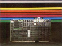
**MLZ-VDC** intelligent 640 x 480 x 4 color graphics controller based on the NEC 7220 controller chip with on-
