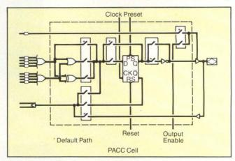
Figure 9: VLSI Technology, known best for their cell compilers, recently expanded their presence in the ASIC arena with the introduction of PACC cells. The new family of devices is based on CMOS tecnology and uses EPROM cells instead of fuses.
