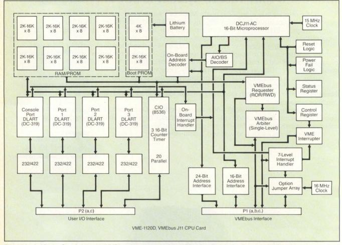
Figure 1: Logical Design Group's J-11-based VME board incorporates a full VME Bus Data Transfer Bus Requester, VME Arbiter and a seven-level interrupt handler.
