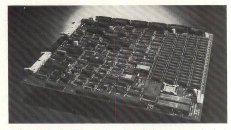
which would adapt the CPU core to the Multibus. There are 512 Kbytes of parity protected dynamic RAM on-board, expandable to 2 Mbytes. In addition to the GS-32 SBC, Goodspeed is manufacturing a development system aimed primarily at OEMs designing in the singleboard computer.
