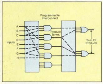
Figure 1: After PROMs were introduced in the early 1970s, field programmable logic arrays (FPLAs) were the first user-programmable ASICs. Both the AND array and OR array are fuse programmable and thus offer product sharing among all outputs.
