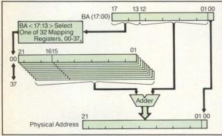
Figure 2: Construction of the physical address on the N1100 Unibus board is achieved through a set of mapping registers.
