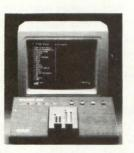
The new OMNI 64 has 10A. 80V software configured bipolar pin drivers on every pin. Pin drivers so fast and accurate that they can program every EPROM, PROM, PAL, FPLA, or single chip uP manufactured today without a single family pack or configuration module!
