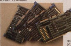
**MLZ-91A** single board CP/M<sup>TM</sup> system with on-card floppy disk drive controller, winchester interface, optional AM9511, streamer tape interface, two serial ports, one parallel port, 64K or 128K bytes RAM with parity, two EPROM sockets, and GPIB CONTROLLER.
