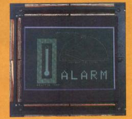
Vacuum Fluorescent Graphics Module. Controller has dual processor pipelined architecture for fast speed. 320 x 240 pixels.
