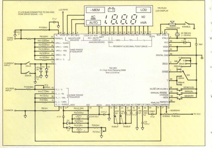
Figure 2: The TSC805 is the only active component in this five function, 22 measurement-range digital multimeter.
