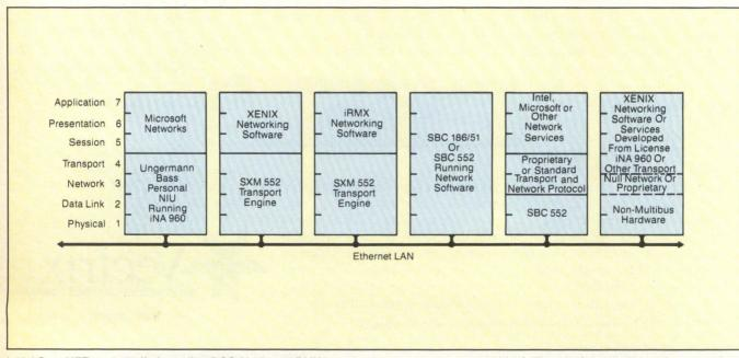
Initial OpenNET product offerings allow DOS, Xenix and RMX-based computers to access each other's files. Hooks are built into the protocols to allow development for non-Ethernet networks and computers with other operating systems.
