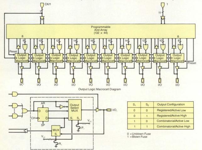
Figure 7: AMD expanded the basic PAL architecture by including programmable macrocells on each output of the firm's 22V10. Also adding to the device's flexibility are the varying number of product terms found at the ten outputs.
