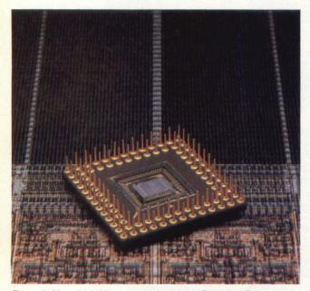
Figure 8: Monolithic Memories claims the 64R32 MegaPAL is equivalent to 5000 gates. The accuracy of this number has been the subject of recent debate among PLD competitors throughout the industry.
