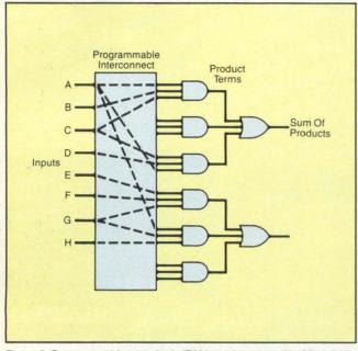
Figure 2: Programmable array logic (PAL) was introduced by Monolithic Memories shortly after FPLAs. Since the AND plane is hardwired to the OR array, device programming is simplified.
