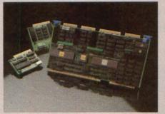
HK68<sup>™</sup> powerful and versatile single board UNIX<sup>™</sup> (System III or V) or CP/M-68K<sup>™</sup> system with 68000/68010 CPU (8Mhz or 10Mhz), MMU, quad channel DMA, four serial ports, 128K, 256K, 512K or 1M bytes of on-board RAM with parity, up to 128K bytes of on-board EPROM, user acces-
