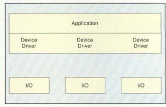
Figure 1: Conventional graphics programs are a monolithic piece of code with device drivers embedded with the object code. This is typically done for optimum performance, but hinders portability.
