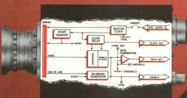
Reticon's LC300 Series cameras offer you an easy solution to industrial vision applications. These low-cost rugged modular cameras also feature binary output, wide dynamic range, differential line drivers, a sealed industrial case, and plug-in compatibility with Multibus<sup>TM</sup> and <u>Q-Bus<sup>TM</sup> p</u>rocessors.
