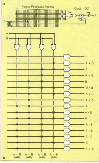
Figure 4: (a) By including an XOR gate at the input to the D-register, carries from previous operations can be XORed with two variable sums generated by the PAL array. This architecture allows the user to implement arithmetic operations. (b) When the PAL architecture of (a) is programmed as shown, the circuit provides the corresponding 16 Boolean combinations.
