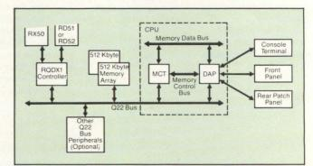
Figure 4: Early limitations of the MicroVAX-1 included a low-performance disk controller and lack of tape support.
