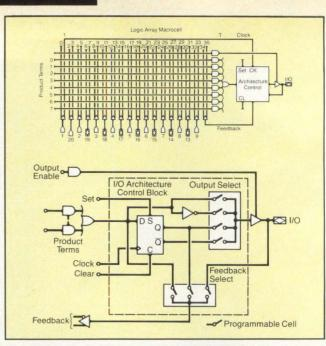
Figure 10: (a) Altera's EP300, which is based on CMOS technology and uses EPROM cells as opposed to fuses, incorporates eight of these macrocells in a single device. (b) The internal structure of Altera's architectural control section shows the output and feedback selectors that provide 12 operating configurations for each sum term. Both registered and asynchronous outputs can be configured to be inverted or noninverted by programming the output select multiplier.
