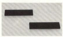
Designed to support CP/M and MSX operating systems, the HD64180 8-bit CMOS CPU incorporates an on-chip MMU and two-channel DMAC. The
