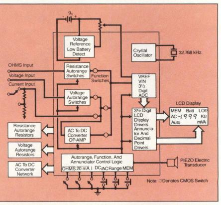
Figure 1: A simplified block diagram of the TSC805 identifies the main components of the input conditioning, 31/2 digit A/D converter and control logic subsystems.
