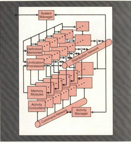
Figure 3: The Personal Sequented Inference machine is intended to provide researchers with a programming environment for the development of software. It can process 16 million 40-bit words.
