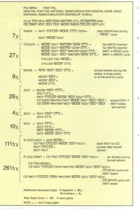
Figure 3: These Boolean equations and number of 2-input equivalent gates for each section of the DP84412 demonstrate how the 165-gate figure is reached.
