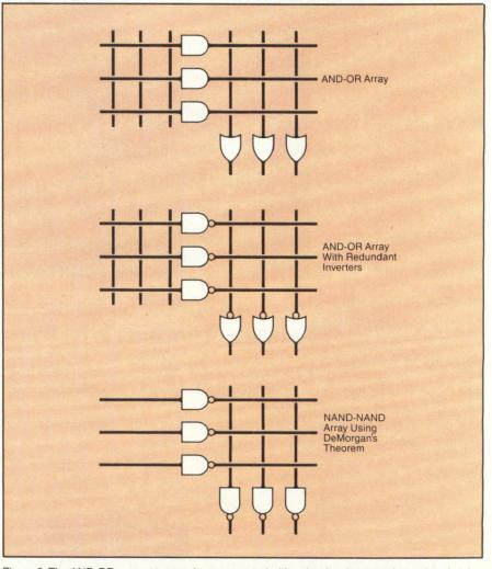
Figure 2: The AND-OR array at top can be represented with redundant inverters (center) and, using De Morgan's theorem, as a NAND-NAND array.
