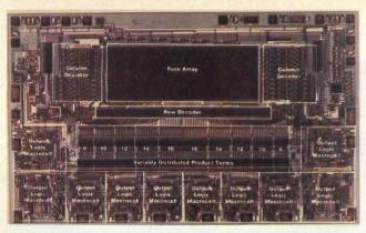
Figure 6: A die photograph of AMD's AmPAL22V10 illustrates the various sections of the device.
