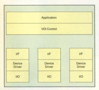
Figure 2: The Virtual Device Interface (VDI) separates device independent code (application programs) from the routines that drive specific plotters (device drivers). The VDI interface then translates system calls to physical commands.
