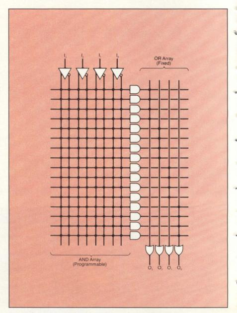
Figure 1: Set up of a PAL having four inputs, four outputs and 16 products.
