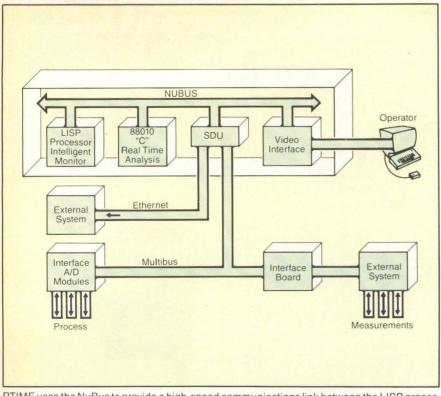
RTIME uses the NuBus to provide a high-speed communications link between the LISP processor and the 68010 real-time processor. Links to the outside world occur through peripheral boards on the Multibus chassis, or via Ethernet to other distributed systems.
