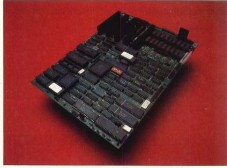
Figure 1: The Mostron PC motherboard includes up to 256 Kbytes of RAM.
