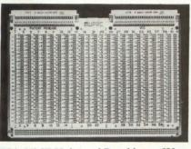
This VME Universal Panel has a  $6U \times 160$  mm deep wire wrappable panel layout and four layer, true multilayer construction. With copper foil around each pin on all layers and plated through holes to equalize current flow throughout the power bus system, the component side V<sub>cc</sub> plane around each pin allows in-
