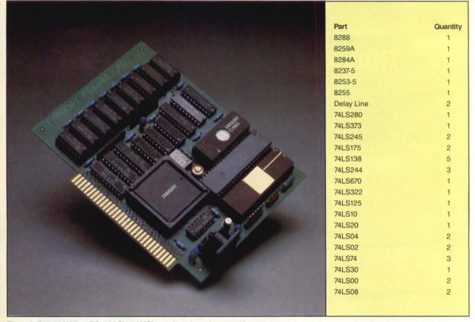
Figure 2: Faraday's Micro PC: 39 LSI and MSI parts have been integrated into a gate array.
