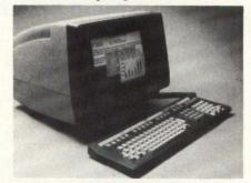
Designed for use with the firm's 932 Supermicro family, as well as with other UNIX-based systems, this color display terminal, the ColorScan 90, allows simultaneous display of up to eight active tasks, each with vertical and horizontal scrolling. Eight background and eight foreground colors display data in 64 combinations. The 12" nonglare screen presents characters and images in 80- or 132-columns. Price is \$1,995. **Datamedia**, Nashua, NH **Circle 170**
