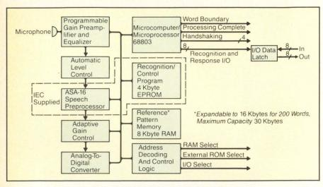
Figure 2: Interstate Voice Products' VRC100-2 simplified block diagram.
