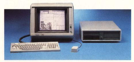
The standard Tektronix 4404 Artificial Intelligence System, listed at \$14,950 (U.S. only), features a monochrome bit-mapped display; keyboard; mouse; 32-bit microprocessor with virtual memory management; hardware floating point; 1 Mbyte RAM; and a 20-Mbyte hard disk with a single 5½ floppy disk. The system comes with the Smalltalk-80 (a trademark of Xerox Corporation) language, an interactive, graphics-oriented exploratory programming language.
