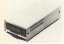
This series of 5 ¼ ″ half-height removable cartridge tape subsystems have storage capacities ranging from 10 to 60 Mbytes. Designed to interface with standard Winchester and SA450 floppy disk drives, tape drives are compatible with IBM personal computers and compatibles. The tape systems use a MFM or GCR data encoding model. 12 Interface, Canoga Park, CA Write 170
