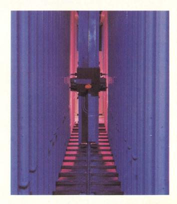
Figure 1: Increased use of automation is improving throughput and quality at many Winchester disk drive manufacturing facilities, and helping to keep more manufacturing plants on-shore. Above, a Litton ToteStacker system moves nearly completed Winchesters through a series of final tests at Priam's new automated manufacturing facility in San Jose, CA.
