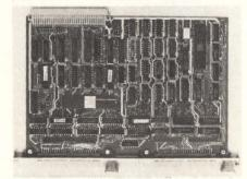
The IoVME-402 is a VME Bus Master which interfaces the VME bus to most 9-track tape drives and has SCSI interface, dual RS-232 I/O ports and vectored interrupts. The interface has an AM9516-based dual channel DMA controller. All DMA functions are programmable and chain loadable including: 24-bit addresses, 16-bit transfer counts, 8- or 16-bit data transfers and byte to word funneling. Price is \$1,850. Io Incorporated, Tucson, AZ Write 192
