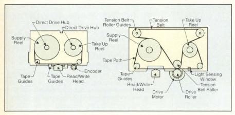
Figure 2: The D/CAS cassette is only  $4'' \times 2^{1/2}'' \times 7/16''$ , compared to  $6'' \times 4'' \times 11/16''$  for a standard tape cartridge.
