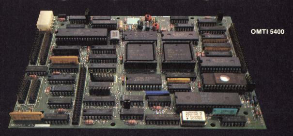
Our OMTI 5400 SCSI (SASI) controller offers Winchester, floppy and tape support all on a single 5% footprint PC board. By using our proprietary VLSI chip technology, we were able to squeeze all these functions onto a board size that most controller companies are still using for single function controllers. This means increased capability and improved cost-effectiveness in your application.
