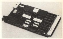
The Gesmpu-4A is a microcomputer board built around the MC68000 16-bit microprocessor. The microprocessor operating at an 8MHz clock rate. Clock frequency is generated by an onboard crystal oscillator. The board has four JEDEC sockets to accommodate 128 Kbytes of EPROM and 16 Kbytes of static RAM. The Gesmpu-4A has a triple 16-bit timer and an RS-232-C serial interface with fully programmable baud rate. Price is \$475. Gespac, Mesa, AZ
