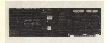
Figure 2, above: Sky Computer's TMS320 based co-processor.
