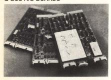
The III4AD is a Q-Bus compatible III4AD board which has 8 software programmable ranges from IOmV full scale to IOV full scale. The III4AD has unrestricted mixing of high and low level signals plus 12-bit resolution. For fixed and changing I/O environmnets, the III4AD has software selection by channel of thermocouple type, RTD, load cell and strain gauge inputs. Companion boards provide expansion to 128 channels with 250V common mode protection. Adac, Woburn, MA Write 213
