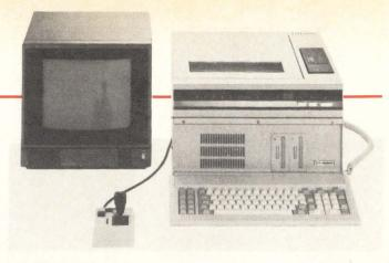
from 0 to 100 %. The LPC-1000 includes a high resolution color graphics generator ( $640 \times 400$  or  $320 \times 400$ ) which can be overlaid onto the video disk picture. In its microcomputer mode the LPC-1000 is used as a general purpose 8086-based microcomputer with CP/M-86 operating system and Pascal, Fortran and C high level languages. The laser optical disk is used as archival 2 Gbyte ROM. The dig-
