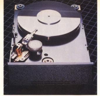
Figure 3: Manufacturers of half-height, 20-Mbyte Winchesters are hoping that IBM's announcement of a 20-Mbyte drive in their PC-AT will create a big market for their drives, just as IBM's PC-XT created a huge demand for 10-Mbyte Winchesters. Cogito's PT925, shown here, is designed for portable applications, and features Whitney-style minislider heads, thin film media, and 12-watt power consumption.
