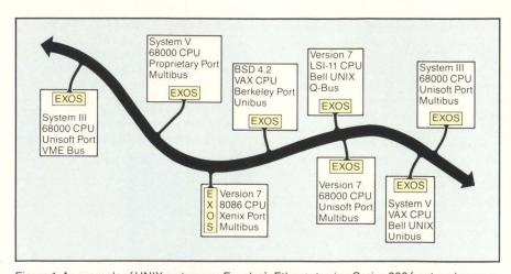
Figure 1: An example of UNIX systems on Excelan's Ethernet using Series 200 front-end processors and their 8010 IP/TCP protocols; file transport, remote copy, login, shell, and electronic mail are available to all users.
