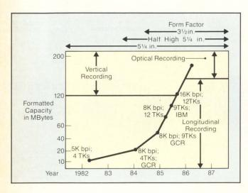
Figure 3: Capacity of digital cassettes has room to grow; by using vertical or optical recording technology, Winchester capacities are rivaled
