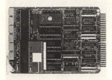
The ZT8806 is an 8088-based processor board for automation applications. MAX mode operation allows the addition of the 8087 Numeric Data Processor using Intel's iSBC 337 piggyback processor option. Five 28-pin byte-wide JEDEC memory sockets provide space for up to 64 Kbytes of PROM and 32 Kbytes of static RAM. The I/O capabilities include one serial port, 5 counter/timers, two 8-bit parallel I/O ports, and an interrupt controller. Price is \$465. **Ziatech**, San Luis Obispo, CA Write 210
