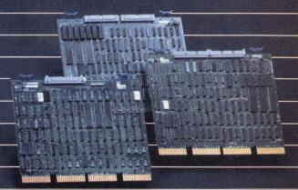
1/2" TAPE—CONTROLLER/COUPLER PERTEC I/O
