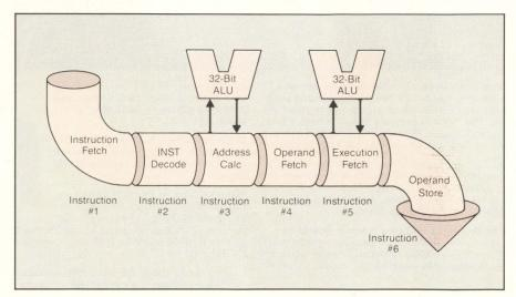
Figure 5: This instruction pipeline will be used in Zilog's new Z80,000 32-bit microprocessor (to be introduced in February 1985). Keeping a pipeline full is critical to exploiting its usefulness.
