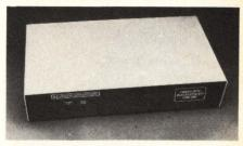
The CBE-202 Fiber Optic Interprocessor Link comprises a parallel-to-serial multiplexer and a Bus Interface Module (BIM) which plugs into DEC PDP and VAX backplanes. A duplex fiber optic cable links the two multiplexers. The link operates at 250 kilowords/sec and can be as long as 2 kilometers. The Bus Interface Modules are software compatible with the DEC DRII-B or DRII-W modules. Price is \$4,500. Canoga Data Systems, Canoga Park, CA
