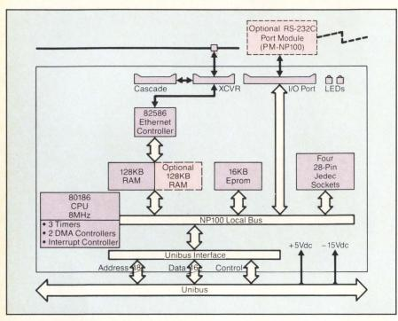
Figure 2: Interlan's NP100 board for Unibus systems, as well as those for other buses and Excelan's 200 series boards, provide Ethernet protocols on board in EPROM. With the power of an 80186 processor and 128 or 256K RAM, host systems are offloaded of communications processing.
