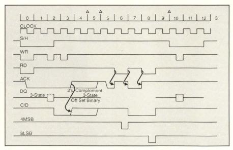
Figure 2: Analog to digital conversion cycle showing power up initialization — states 0 to 2, start of conversion — states 3, conversion cycle — states 5 and 6, and latching of data from conversion — states 6 and 8. The first entry point is the power up sequence in state 0 and the second is in state 9. In states 5 and 9 the clock does not run until conversion is complete or an external conversion is requested, respectively.
