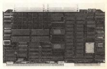
The Am 96/3500 is an eight-channel serial communications controller board, featuring an 80186 CPU. The Am96/3500 can operate as a slave controller or a bus master. The Am96/3500 has eight independently programmable serial channels based on the Z8530 serial communications controllers and is compatible with RS-232C and RS-423 protocols. The SCCs can be programmed to handle all asynchronous and synchronous formats. Price is \$2,795. Advanced Micro Devices, Sunnyvale, CA
