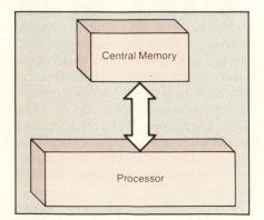
Figure 1: The link between the processor and central memory of a von Neumann computer is known as the von Neumann bottleneck.
