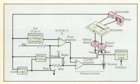
Figure 1: Only four moving parts comprise the design of the drives; tension is electronically controlled.
