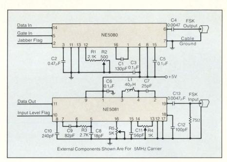
Figure 1: Connection of the NE 5080 and 5081 as a DC to 2 Mbaud full-duplex modem.
