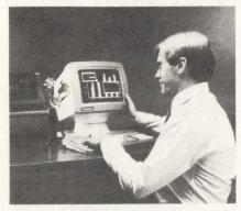
The 925E terminal provides 925 compatibility. The 925E meets DIN standards, has a tilt and swivel screen, a buffered printer port and 16 function keys that can be shifted to 32. An optional graphics board is available. Price is \$795. **TeleVideo Systems**, Sunnyvale, CA Write 175
