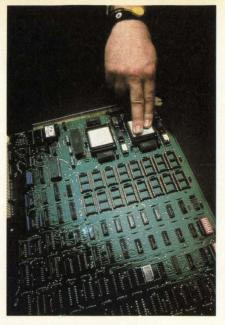
Above: Bubble memory chip on a processor board.
