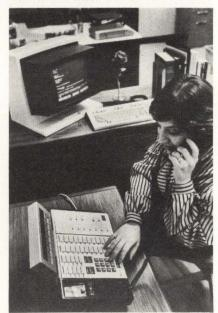
The System 75 communications system combines voice, high-speed data, and communications and system management features into an integrated system. It is designed for installations of 300 lines and can be upgraded. The system 75 can transmit voice and data simultaneously over one line at 64,000 bps. The system has a system management capability for customization in different applications such as diagnostics. **AT&T**, Morristown, NJ **Write 130**
