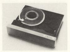
The PCT-1000 is a IBM-format compatible 9-track streaming tape drive, that provides backup of 138 Mbytes for Winchester hard disks, read/write access to archival data banks, and intercomputer data interchange. The PCT-1000 can handle formats including 800 NRZI, IBM and ANSI; 1600 cpi PE, IBM and ANSI; and dual-density, 3200/1600 cpi. Price is \$2,256. **IBEX Computer Corp.**, North Hollywood, CA Write 176
