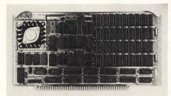
Dual Systems (Berkeley, CA) 1 Mbyte RAM board makes use of 256 Kbit devices. Access time is 220 ns.
