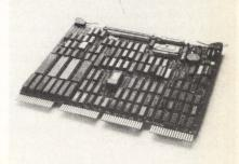
The Model DQ215 Winchester disk controller interfaces two 8" and/or 14" SMD I/O compatible drives to LSI-II thru II/73 and MICRO/PDP-II computers. The quad module operates when it is plugged into one Q-Bus slot and connected to drive(s) by flat cables. The controller has universal formatting, 56-bit ECC, 22-bit addressing for 4 Mbyte data access and is compatible with RT-II, RSX-II and RSTS operating systems. Price in quantities of 50 is \$1,50. **Dilog**, Garden Grove, CA **Write 206**
