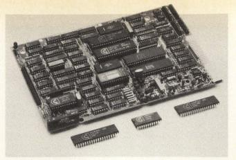
Adaptec's ACB-550 5<sup>1</sup>/<sub>4</sub>" Winchester disk controller with SASI/ANSI SCSI support.
