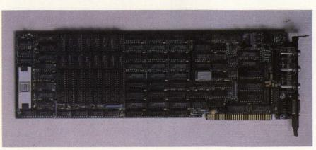
Figure 3: Featuring the NEC 7220 chip and 128K of memory, the IDEAgraph color graphics board from IDEAssociates allows the PC or XT to be used in CAD/CAM applications.
