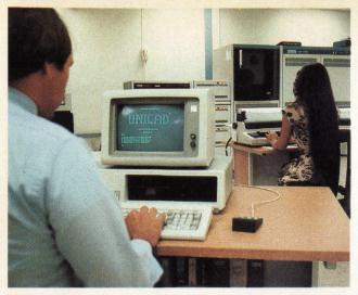
Universal Semiconductor's UNICAD I CAD system includes an IBM XT for schematic capture, netlist generation and local simulation. For larger simulation tasks, the PC can be linked to Universal's VAX.
