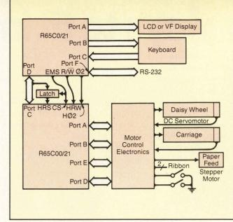
Figure 2 (above): Typewriter/Telecommunications system with dual processor host and peripheral controller.
