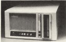
The Series 8600 incorporates the DEC KDJ11-AAbased LSI-11/73 processor into its operating systems. The system has a 41.6-Mbyte fixed/removable hard disk drive and 256 Kbytes RAM expandable to four Mbyte. Most current LSI-11 and PDP-11 operating systems and application software are compatible with the 8600. Plessey, Irvine, CA Write 141
