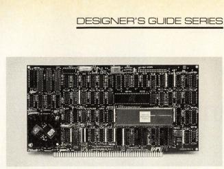
Cromemco's dual processor card features a 68000 and a Z80.
