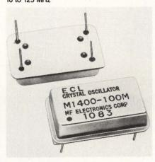
These Crystal Clock Oscillators are for commercial or industrial applications and are available in frequencies of 10 to 125 MHz. The metal package is hermetically sealed by resistance weld, with a glass-to-metal seal connector which may be soldered or plugged into a socket. The oscillators have monolythic ECL 10,000 outputs and come in four-teen models that cover .0025% thru 1.0%. **MF Electronics**, New Rochelle, NY **Write 200**
