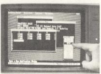
The Point-I Color Kit includes a 13" diagonal touch screen, intelligent controller and an RS-232C serial interface. The screen, available for the IBM PC color monitor is fully programmable and supported by software development tools. With the screen, users can select from menus, position the cursor and create and manipulate graphics by touching the IBM Color Monitor with a fingertip. Price in OEM quantities is \$650. **MicroTouch**, Woburn, MA **Write 178**
