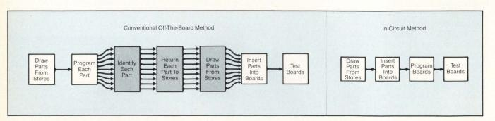
Figure 2: Comparing the manufacturing steps required for the off-the-board and in-circuit programming methods.
