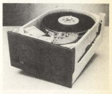
Models 1353, 1354, and 1355 are Winchester disk drives with capacities of 85, 127, and 170 Mbytes, respectively. The series is compatible with drive controllers available from major controller firms and average access times are less than 30 msec. Prices, respectively, are \$1,469, \$1,669, and \$1,837 in OEM quantities. Evaluation units will ship in the fourth quarter of the year. **Micropolis Corp.**, Chatsworth, CA **Write 210**
