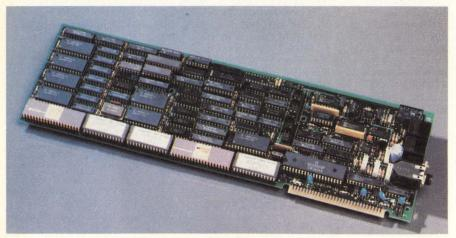
Figure 8: The VPC 2000 voice card from Votan brings voice I/O functions to the PC.
