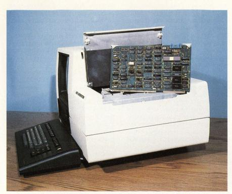
Figure 2: Interlan's NI3210 Multibus Ethernet Communications Controller.
