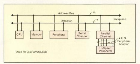
Figure 2: Am26LS38 utility in a processor complex.
