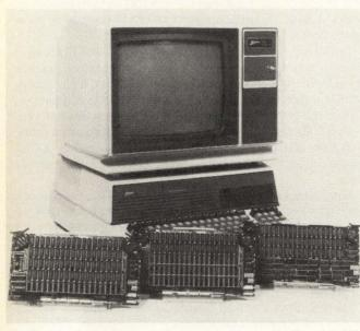
The Z-series from Macrotech International boosts the Zenith Z-100 microcomputer main memory up to a full Mbyte.
