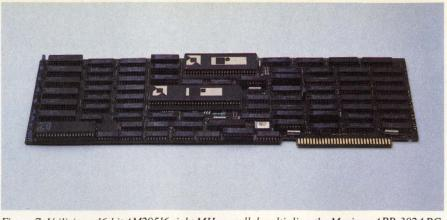
Figure 7: Utilizing a 16-bit AM29516 eight MHz parallel multiplier, the Marinco APB-3024 PC adds array processor functions to the IBM PC.
