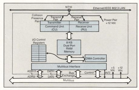
Figure 1: NI3210 functional block diagram illustrating command and receive units implemented with the Intel 80582 chip.
