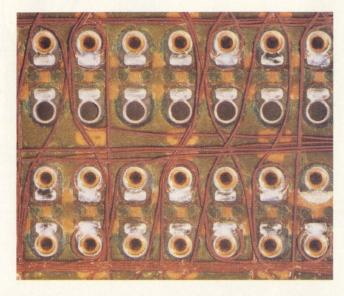
boro, MA). The concept bridges the gap between wire wrap and multilayer printed circuit boards. Computer storage of design information used in conjunction with premanufactured board modules allows new designs to be started in wire wrap for prototyping and converted directly to Unilayer 11 wiring for production requirements, thus eliminating the cost and time normally associated with production redesigns.
