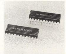
The MCM93422A and MCM93L422A are 1024bit bipolar RAMs with access times of 35ns and 45ns, respectively. The parts have a power dissipation of 0.26 m W/bit and provide 3-state outputs to drive bus-organized systems and/or highly capacitive loads. The series is TTL compatible and is offered in JEDEC standard 22-pin, 400 mil wide plastic or ceramic packages. Price in quantities of 100 is \$9.50 (plastic), and \$10.76 (ceramic). **Motorola**, Phoenix, AZ **Write 188**
