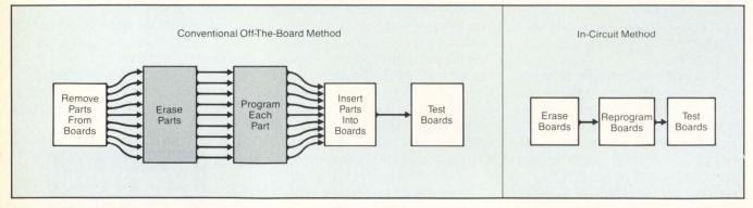
Figure 3: Reprogramming memory boards, comparing off-the-board method to in-circuit method.
