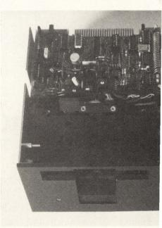
Tape drives to the D/CAS standards, like the Memtec Companion 500 Series, fit into a standard 5<sup>1</sup>/<sub>4</sub>" form factor and hold 10 or 20 Mbytes.
