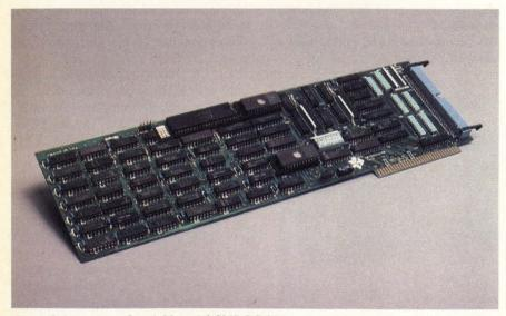
Figure 5: Interphase Corp.'s Maverick SMD PC-80 is a rigid disk controller which allows the PC to support the SMD interface.
