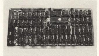
Adaptec's Intelligent host adapter, the AHA-1510, supports the S-100 bus.
