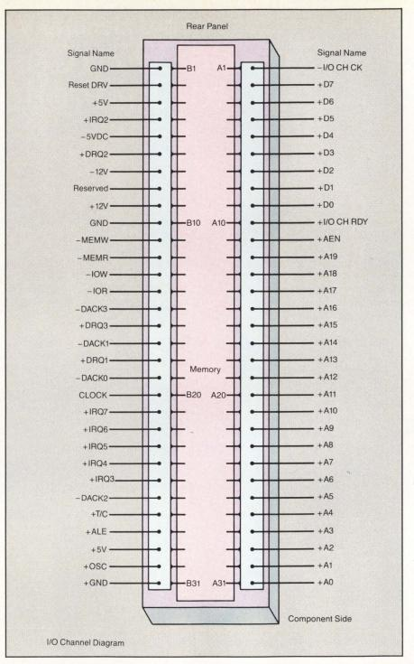
Figure 6: Diagram of the I/O channel which is an extension of the 8088 microprocessor bus. The I/O channel is bused across the system's five I/O slots.
