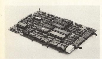
Adaptec's ACB-5580 SMD rigid disk controller with SASI/ANSI SCSI support.
