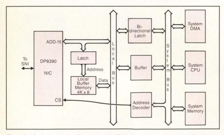
Figure 1: A few low cost external components is all that is needed to interface the NIC to the host system with local memory. Even the control signals for the buffers and the latches shown are provided by the NIC. A direct interface to the system bus (without a local memory) requires even fewer components.
