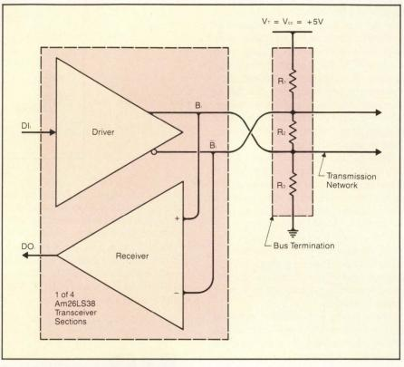
Figure 1: System connection diagram.
