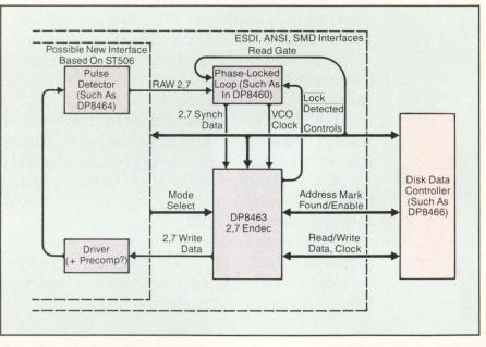
Controller system block diagram using National's four-chip set for 2,7 RLLC encoded (DP8463 2,9 Endec chip) Winchester disk drives.
