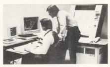
The System 25 is a CAD system with a 32-bit central processing unit, distributed processing and a modular building approach that enables system expansion. The system can be organized into singleuser, stand-alone, multiuser or mainframe-based configurations. The main design station consists of two displays, a 12" alphanumeric screen and a monochrome or color graphics screen. Price is \$65,000. Calcomp, Anaheim, CA Write 146
