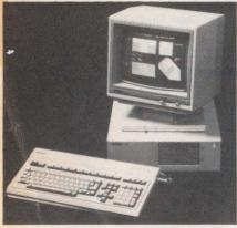
The T300 Computing System includes a 192K computer with Intel 8088 microprocessor, 640K 5-1/4" floppy disk drive and a 12" green screen display. The system includes a 10 Mbyte hard disk, a memory expansion to 512K, a clock/ calendar, and a 16 color palette. The 12" monochrome display has a resolution of 640 × 500 and the same feature is included on the optional 14" color display. Price is \$2,495. **Toshiba**, Tustin, CA Write 136
