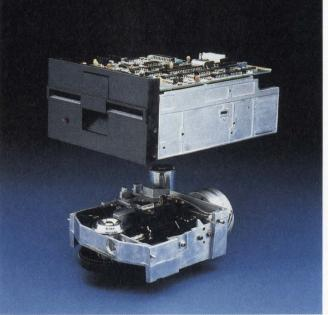
Figure 11: Micropolis' minifloppy drive uses a chassis-within-achassis construction to increase durability.
