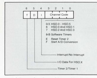
Figure 3: Diagram shows format of Command Tag. The lower four bits specify the basic operation and the remaining three bits are options to the basic operation.
