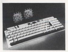
The KS-200E keyboard is designed with patented twin bifurcated contacts and has a rated life of 50 million cycles. The KS-200E is available with tactile or linear feel. Keys have a .120" stroke and typical bounce is less than one msec, with a five msec bounce over the switch life. The KS-200E is available as discrete switches or arrays assembled with or without keycaps, or assembled and soldered to a PC board with or without electronic encoding. Stackpole Components. Farmville, VA. Write 172
