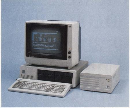
Winchester disk StorageMaster<sup>™</sup> subsystems from Control Data provide 18 or 30 Mbytes of storage to the IBM PC.
