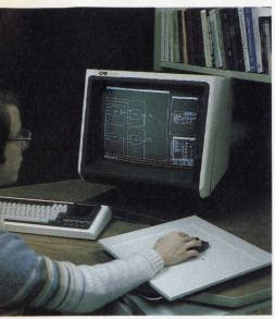
Figure 6: CAE 2000/420 used in logical design for VLSI.
