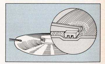
Figure 3: The stretched flexible media of 3M's experimental Keystone drives dimples immediately beneath the R/W heads. This dimpling, 3M claims, disperses particulate contaminants.
