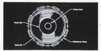
Figure 9: Amlyn's 170 tpi flexible disk drive uses a reference track  $\rightarrow$  with 8 windows for accurate R/W head positioning.
