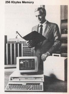
The Apricot is an 8086-based IBM-compatible 16-bit microcomputer. It has 256 Kbytes of main memory, three operating systems (MS-DOS, CP/M-86 and concurrent CP/M-86) and 3.5" Sony MicroDrives, each with 315 K bytes of storage. The Apricot also includes an integral calculator and bundled executive software. An 80-character MicroScreen is built into the keyboard and displays two 40-character lines. Price is \$2,495., **ACT**, Santa Clara, CA **Write 132**
