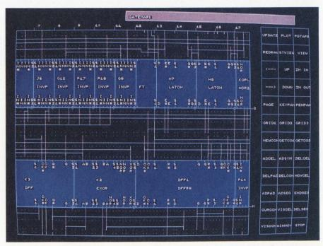
Figure 7: The GATEMARK system from Matra Design Systems provides schematic entry, fault test generation, automatic layout and PG/Calma art layout.
