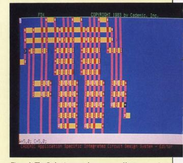
Figure 1: The Cademic aproach uses entry of logic expressions in micro cell form on a matrix instead of the more common schematic diagram.
