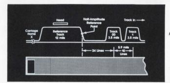
Figure 10: The 12-mil reference track on the edge of Amlyn diskettes allows the R/W head positioning system to compensate for physical eccentricities.
