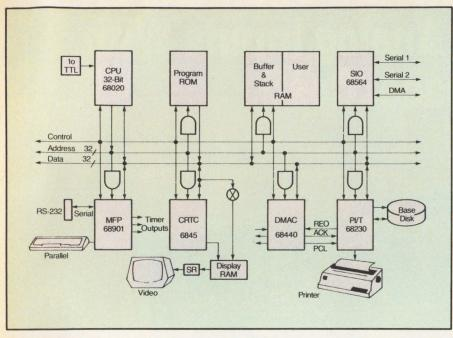
Figure 3: An engineering workstation using the 68020.
