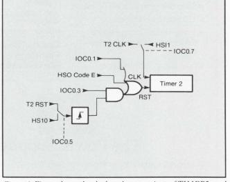
Figure 4: Figure shows the clock and reset options of TIMER2 used by the High Speed Output unit.
