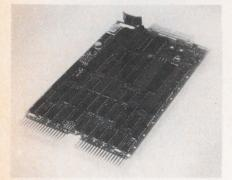
The DQ619 5 1/4" Floppy Disk Controller interfaces LSI-11-11/23PLUS, MICRO/PDP-11 computers to one or two 96TPI double sided, double density 51/4" floppy drives having a SA450 interface. The controller is con-
