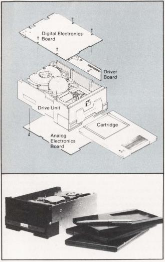
Figure 4: Iomega's Beta-5 uses a floppy disk cartridge to pack 5 Mbytes into a 5 1/4" format drive.
