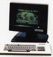
The Modgraph GX-100 Graphics Terminal offers the serious graphics user extensive capabilities for little more than the cost of an intelligent alphanumerics terminal.
