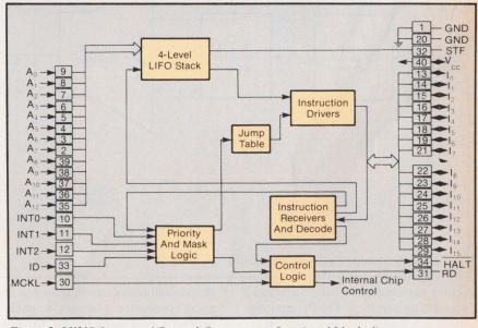
Figure 2: 8X310 Interrupt/Control Coprocessor functional block diagram.
