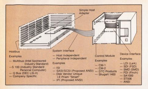
modules support the command and status block protocols. Although differences in performance occur in the control modules, they can all connect to the same adaptor and perform the same basic seek, write, read and format comFigure 3: Interface terminology.
