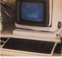
The Florida Computer Graphics Beacon terminal line was one of the first to incorporate both 16/32 bit processors and second generation bit slice devices.
