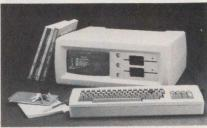
The MD3 is a CP/M-based portable computer which includes two floppy disk drives and eight software packages. Features of the MD3 include 64 Kbytes of RAM, two double-sided, doubledensity, 5.25" floppy disk drives (400 Kbytes each), a 5 × 9" monitor with an 80-character by 24-line display, two ports, a detachable keyboard, and character-map graphics. **Morrow**, San Leandro, CA **Write 138**
