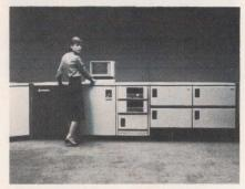
The Mapper 10 is a solutions-oriented processor with 4th generation, interactive software. The Mapper 10 system configuration consists of a CPU with 524K words of memory, two fixed disk drives with a total storage capacity of 460 Mbytes, a streaming tape, one 0789 printer and a console. The system will be available in April, 1984. **Sperry**, Blue Bell, PA **Write 143**  WORKSTATION Supports One Gbyte Memory
