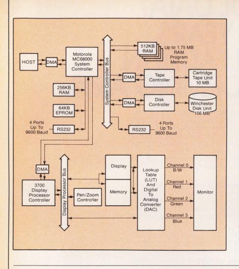
Figure 2: Viewstation functional block diagram.
