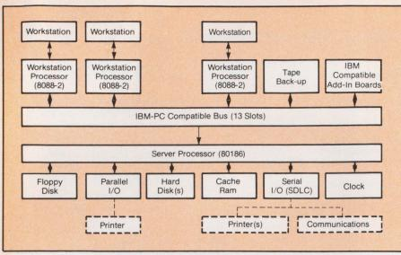
Figure 2: PC/XT compatible Dimension from North Star allows multi-user application without networking through multiple 8088-2 processors on the PC bus and an 80186 server processor for memory, clock and I/O.
