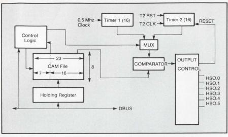
Figure 2: Block diagram of the High Speed Output hardware.
