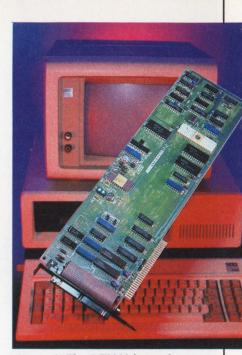
Figure 1: The DT2808 brings low cost analog and digital I/O functions to the IBM PC. This single board peripheral fits in one of the host computer's expansion slots.
