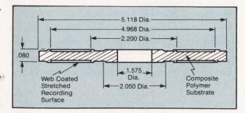
Figure 2: 3 M's new Keystone technology, designed for use in either fixed or removable disk drives, uses media consisting of a rigid polymer composite substrate with 10-mil raised rims at the periphery and center hole. Flexible diskette media is then stretched between these rims.
