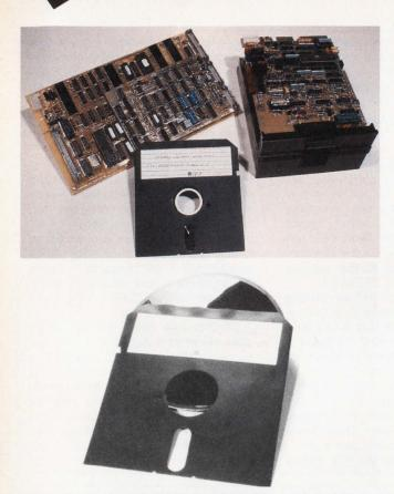
Figure 7: Vertimag's VSC530 (top) looks like a standard Shugart drive, but uses perpendicular recording techniques to store 5 Mbytes on a dual-sided 5 1/4" diskette. Their media (bottom) is a sputtered cobalt-chromium alloy.
