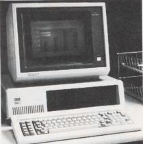
The Color IV is a high-resolution color monitor compatible with the IBM Personal Computer and DEC Rainbow computers. It is available in two versions with either RGB analog or digital input. The monitor, using a separate interface, will display 16 colors and will accept the RS 170A, RGB signal of the DEC Rainbow. The monitor has 720 × 420 resolution and a .31mm dot pitch CRT. The unit has a 96 × 24 character display. Price is \$995. **Amdek Corp.** Elk Grove Village, IL **Write 128**
