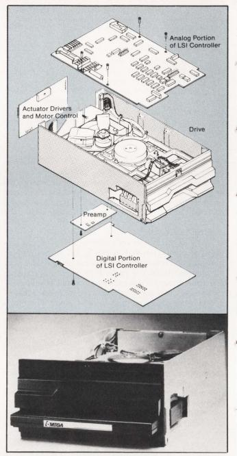
Figure 5: In addition to their standard Alpha-10 8" flexible disk drive, storing 10 Mbytes on a cartridge, Iomega now builds a 10.5 Mbyte version compatible with DEC's RL02.
