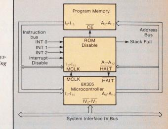
an interrupt request which may be serviced when sampled by the ICC once each instruction cycle of the MicroController. When an interrupt request is serviced, the ICC forces the MicroController to jump to one of three fixed locations in program memory.
