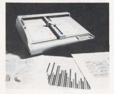
The Lotus 1.2.3 software driver directly drives the Amplot II, six-color, X-Y coordinate plotter. The Amplot II is a microprocessor intelligent plotter accepting ASCII commands. It has builtin software for arc and circle generation, windowing and other functions. The plotter has RS-232-C and 8-bit parallel interface. It has a 10" x14" plotting range and automatic pen selection and is designed for business graphics or engineering applications. Amdek Corp. Elk Grove Village, IL. Write 170
