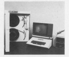
Apple users will now be able to communicate with most IBM-compatible large mainframes utilizing 9 track (NRZI 800 cpi and/or 1600 cpi PE) magnetic tape. A typical 2400′, 10½″ tape reel will accommodate over 40 Mbytes of formatted data for any application, including backup. Innovative Data Technology, 4060 Morena Blvd., San Diego, CA 92117.
