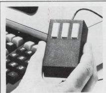
The HAWLEY X063X Mouse moves the cursor in any direction on a computer display screen, in direct proportion to its own movement, with a resolution of 200 ppi. The user-friendly Mouse rolls freely on any convenient surface.
