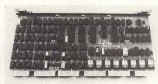
or serial line protocol processing. Its 8 channels can serve terminals, modem connections or other serial devices. Extra TIO Boards can be added as needed. **Associated Computer Consultants**, 228 E. Cota St., Santa Barbara, CA 93101. Circle 226
