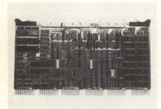
alternative that is ideal for VAX systems and works with equal effectiveness in other UNIBUS systems including PDP11, System 10 and System 20. The single hex-width board plugs into any standard hex SPC backplane slot and is diagnostic compatible with the DEC DH. Each 16-line multiplexer stands alone and runs independently. The user can install as many individual backplane-resident units as needed. **Able Computer**, 1751 Langley Ave, Irvine, CA. **Circle 127**
