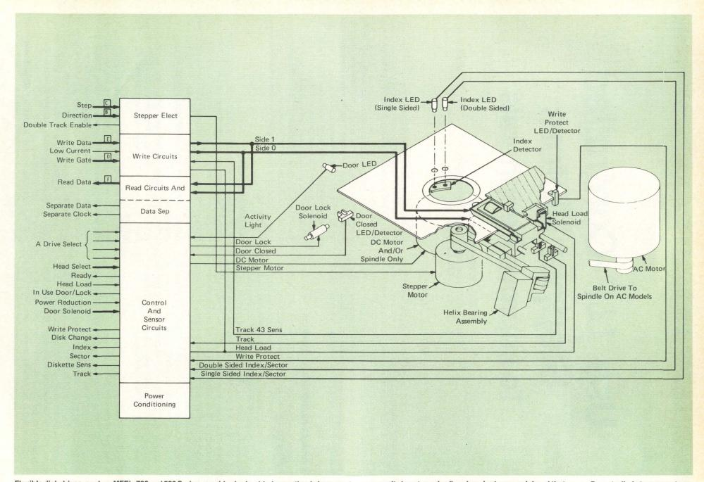
Flexible disk drives, such as MFE's 700 and 500 Series, provide single-sided operation (where maximum capacity is not required) and are just one peripheral that uses  $\mu$ P-controlled stepper motors.
