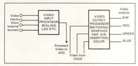
Figure 1: Analog Processor handles live incoming video.
