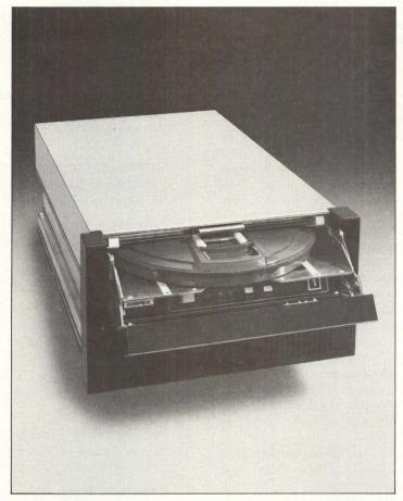
Superwinchester offers fixed disk drive tech-nology plus a built-in, removable 16 megabyte disk cartridge.
