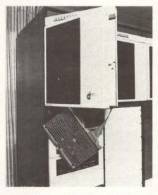
which connects to the IDT Series 1050 formatted tape transport. The complete subsystem uses a dual-density, 9-track, 45ips tape transport for either 800cpi (NRZI) or 1600cpi (PE) providing over 40 MB of data storage. **Innovative Data Technology**, 4060 Morena Blvd, San Diego, CA 92117.
