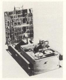
10 times before a new cartridge must be recorded. Model 6450 cartridge tape system incorporates a 6400-bpi, 30 ips cartridge drive and a  $\mu$ P-based formatter in a single compact package. With a 600′ cartridge, the 6450 has an unformatted capacity of 23MB; 17.3MB with a 450′ cartridge, 11.5MB with a 300′ cartridge. Model 6450 is \$1520 ea./100. **Kennedy Co,** 1600 Shamrock Ave., Monrovia, CA 91016. **Circle 146**
