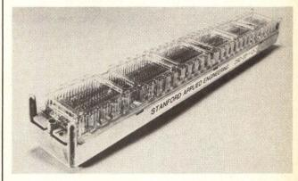
PDQ/DSC DEC compatible press-fit backplane is prewired and pretested.
