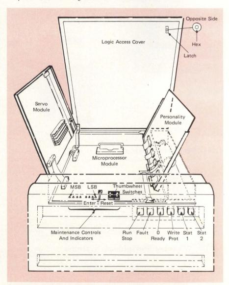
Hinged circuit module arrangement shows RM80 logic. Three main logic modules are accessable by lifting the logic access cover. The hinged module on the left-hand side is the servo module; the one on the right-hand side is the "personality module," used for intefacing to the controller, and the lowest is the microprocessor module. This arrangement enables repair personnel to reach the desired logic element rapidly and with a minimum of tools.
