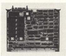
RAM. It may be used stand alone or as a master or slave in a multi-processor environment. Its two-channel serial I/O chip is capable of serial communications up to 500 kilobaud. I/O with other modules in the backplane is memory mapped. The 1868+A accepts both the 9511 arithmetic processor unit or the 9512 floating point processor unit. The module also provides direct memory access to the system's main memory. **Xycom, Inc,** 750 North Maple Rd, Saline, MI 48176. **Circle 202**
