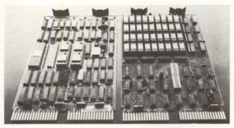
64K dynamic RAM with an access time of 240 ns and cycle time of 400 ns. Power requirement is 1.2A from a 5V supply with battery back-up operation available. The CI-1123 is \$1925 for a  $128K \times 9$  option; \$2550 for the  $256K \times 9$  option. **Chrislin Industries, Inc,** 31312 Via Colinas #102, Westlake Village, CA 91361. **Circle 194**
