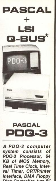
A PDQ-3 computer system consists of PDQ-3 Processor, 64 KB of MOS Memory, Real Time Clock, Interval Timer, CRT/Printer Interface, DMA Floppy Disc Controller, two 8" Floppy Disc Drives, 4 slot 11/23 Q-Bus Backplane and complete UCSD Pascal Software System. Under \$7000. Available with direct addressing to 128 KB, 8-slot backplane, and double density floppies.
