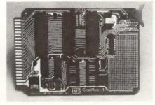
SINGLE BOARD COMPUTER. This SBC has analog, serial and power control I/O. The 4 1/2" × 6 1/2" module can be configured with analog inputs, one analog output, serial I/O, and any mix of 8 AC or DC inputs or outputs. Other features include a 6801 or 68701 MPU and watchdog timer. \$88-\$295. Wintek Corp, 1801 South St, Lafayette, IN 47904.
