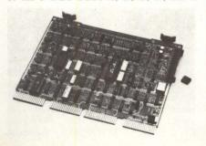
modules (i.e., RS-232-C, current loop, selectable baud rates, limited and full modem control). Selection of any of the 5 modes is made with PC mounted switches. A buffer ready/printer busy monitor circuit allows connection to a variety of low cost RS-232 serial interface printers. (\$825). MDB Systems, Inc., 1995 N. Batavia St, Orange, CA 92665. Circle 218
