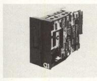
Microlite  $\mu$ C system. It is mounted within the console of the Microlite system, which is a desk-top, stand-alone, multi-function  $\mu$ C. A standard Winchester ferrite head is used, and data is recorded on the disks at 7500 bpi. The drive includes two motor assemblies (stepper and spindle), a head assembly with 4 Winchester heads, and a disk assembly consisting of two disks. **Q1 Corp**, 125 Ricefield Lane, Hauppauge, NY 11787.
