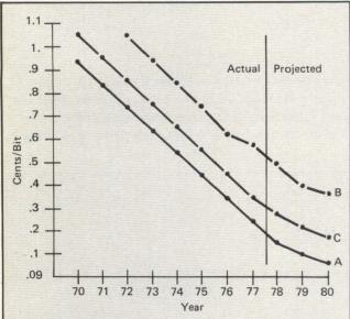
Fig 2 Typical selling prices for memory systems. A: Projected selling price of semiconductor memory cents/bit at chip level; B: Quoted selling price of computer 128K word semiconductor memory system including enclosure and power supply; C: 128K word core memory system with enclosure and power supply.
