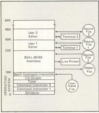
Fig 3 In this two-terminal system, the lower 48K of memory is allocated to the system tasks and the rest of the memory, to user tasks.
