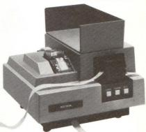
MODEL 1560-P Combination reader/punch with parallel TTL level interface.
