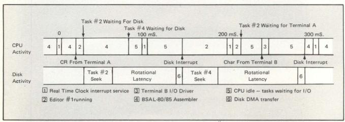
Fig 2 In an execution sequence of an event-driven OS, an editor (task # 2) is interacting with terminal A user. The lower priority
