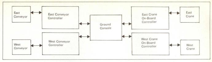
Fig 2 This block diagram shows the overall crane control system.
