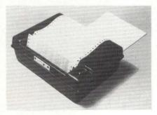
interface requiring 7 data bits, a ready and a strobe. Documentation supplied with the printer includes trouble shooting guides, installation and maintenance instructions, printer and interface schematics, plus instructions on how to wire up to the I-O parallel port. The Black Box Printer measures 4.5"H, 13"W, & 10"D, and weighs 11 lbs. Expandor Inc., 612 Beatty Rd., Monroeville, PA 15146. (412) 373-0300.
