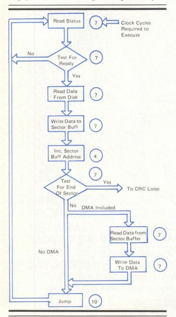
Fig 2 Program loop shows the steps taken by a MOS microprocessor-based FDC in reading data from a disk.
