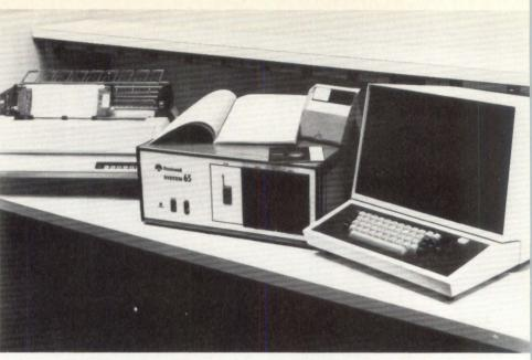
Fig 8 Rockwell System 65 development system supports R6500 microcomputer system development with dual minifloppy disk drives, 16K bytes of static RAM plus ROM-based resident system software, monitor, text editor and assembler.
