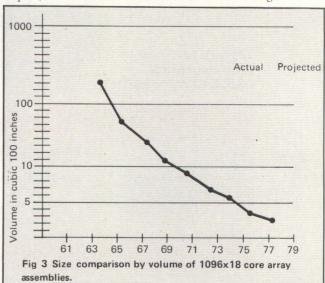
present day core memory systems. The reduced delta noise and new packaging techniques make possible the low cost 16K and 32K sense lines in new designs. Development stage testing now includes checking delta noise and minimizing it. A laboratory test that ran nineteen 16K semiconductor memories for 28 days on a 24 hours a day basis, yielded an MTBF of 1160 hours; a concurrent test using eight 16K core memories showed no system failures.
