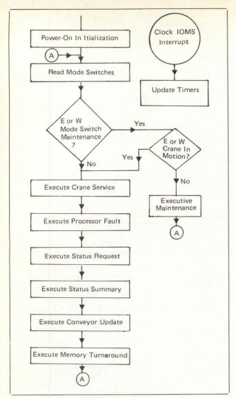
Fig 4 This flow chart shows the operation of the ground console program.
