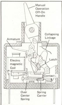
Fig 1 This drawing of the power switch/magnetic protector shows the paddle handle in the ON position, and the contacts closed.
