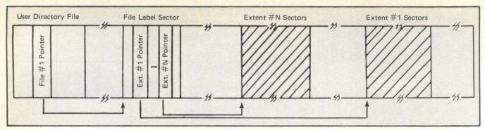
Fig 4 Each disk file in this type of organization can consist of up to 8 separate extents.
