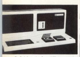
Fig 7 Information Control Microcommand System<sup>TM</sup> supports development of 8080 and Z-80 microprocessor-based systems with light pen, editor, assembler, monitor, up to 64K RAM and up to 2 Kbytes ROM, dual floppy disks, EPROM programmer, keyboard, CRT and optional In-Circuit Debugger.<sup>TM</sup>
