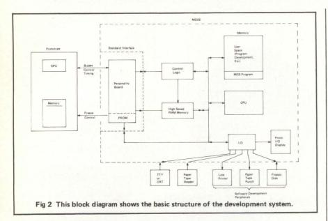
Through the use of personality boards, the MDSS can easily adapt to any microprocessor; boards currently available serve the Intel 8080, National Semiconductor's Pace and the Motorola M6800 series. ADL plans to add additional interface boards to handle other microprocessors.
