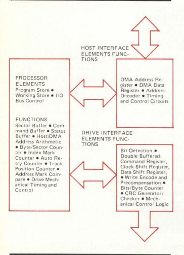
Fig 1 Block diagram of the floppy disk controller shows how the elements and functions for the 8X300 microprocessor are partitioned.
