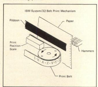
Fig 6 This printing character belt moves at constant speed. Precisely timed hammers make the impressions. The hammer may strike the belt or the paper.
