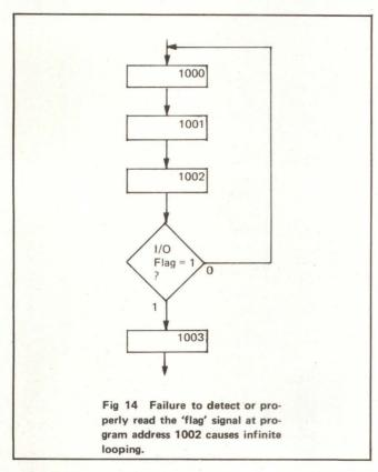
signal is to be read. Externally triggering the scope when that address occurs enables examination of the flag signal synchronized in time to the software. After establishing a state-time reference, it is a simple task to determine whether the signal arrives early or late.
