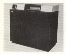
terchangable print bands using a Universal Character Set Buffer, forms spacing through a forms control buffer, vertical line spacing at 6 or 8 lines per inch and a slew rate of up to 75 ips.
