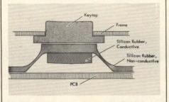
is closed, making contact. When pressure is removed from the switch, the membrane draws the disk back and the switch returns to its normally open state. Applications include calculators, TV remote control switches, cash registers, terminal equipment and
