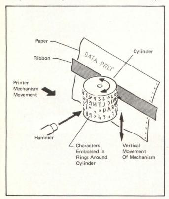
Fig 2 Part of a cylinder printing mechanism consists of a complete character set embossed in a series of rings around the small cylinder. To print, the mechanism moves the cylinder into position along the paper, rotates it and shifts it vertically, then strikes it with a hammer.
