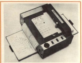
Fig 3 Model DP-11 COMPLOT digital plotter from Houston Instrument produces an 11" wide Z-fold chart across which the pen moves at about 4 ips in 4000 increments per second of 0.005", 0.0025", 0.002" or 0.001" each.
