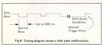
Setting the internal timebase to 200ms per sample established a delay period of 600ms. Now with the trigger set to "1" (positive edge) in the channel recording the "busy" signal, the analyzer could pretrigger record up to 15 channels of data coincident with the disc going "unstuck". Finding the errant control line then cleared up the problem quickly.
