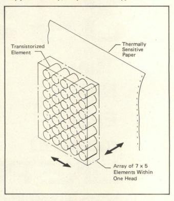
Fig 10 A single thermal matrix head moves across the paper and stops momentarily at each character position. The matrix head elements are transistors that when switched on produce heat. The hot spots force a heat sensitive dye in the paper to change color and create a series of dots.
