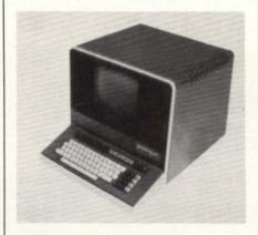
as a firmware (PROM) pre-programmed terminal, the MC77 supports up to 3K of internal program,
