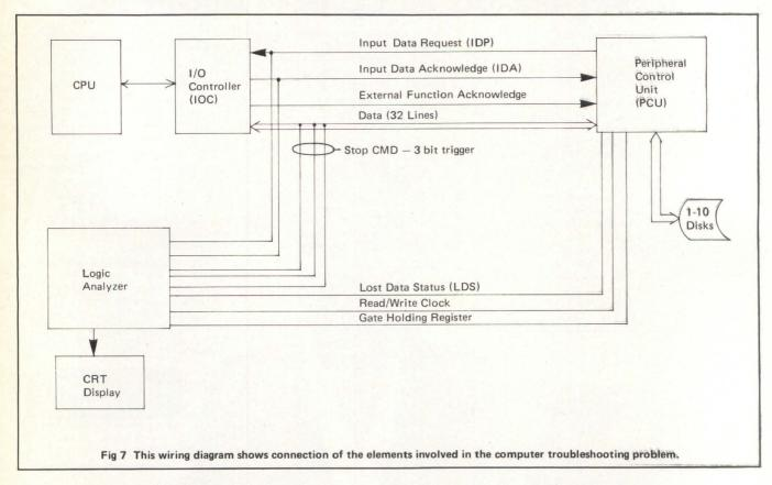
disc pack during normal and "stuck" periods. In order to trigger the logic analyzer when the disc went unstuck, it was necessary to screen out the normal busy periods up to 500ms long and only trigger when the reported busy exceeded that period of time.
