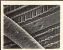
Fig 3 Using VMOS technology, computer memory transistors are so small that eight of them on an integrated circuit (bottom) will fit in the cross section of a human hair (top).
