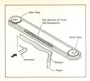
Fig 7 Similar to a belt machine, the train printer consists of a series of linked character "slugs" moving at constant speed. Precisely timed hammers make the impression striking from behind the paper.
