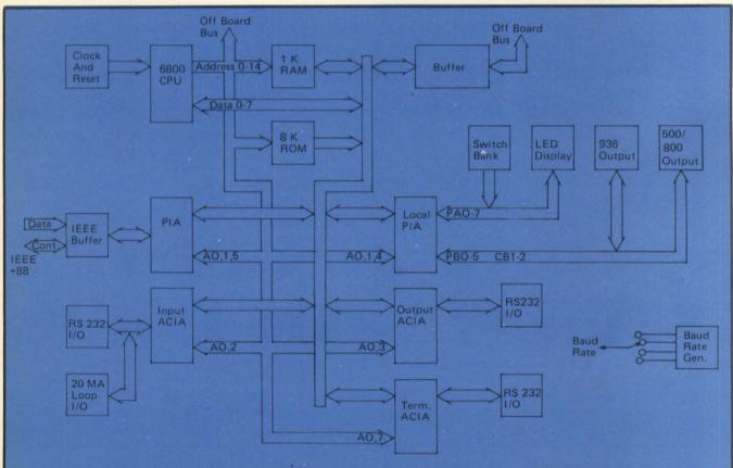
Fig 1 Simplified block diagram of CalComp Model 906 on-line controller indicates how it can provide significant flexibility for plotters. Off-board buses permit memory expansion, additional I/O circuitry, or greater microprocessing power. The bank of switches provides the operator with a means of setting parameters that define plotter type, information about I/O message headings, parity or other checking code, and a powerful self-analysis and checking capability.
