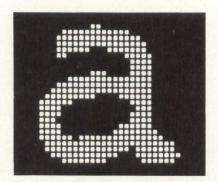
Fig 1 The OCR changes alphanumerics into a pattern of dots, and sends them to the video buffer, which circumscribes a rectangular box around each element.
