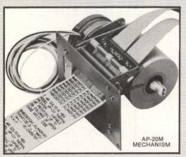
Gulton's fixed head approach to thermal printing takes advantage of the quietness and reliability of solid state switching. COMPARE: one moving part—the paper drive, independence from ink supplies and ribbon mechanisms, high character quality and/or full graphics capability versus any other printing technique such as moving head, print solenoids or wire matrix.
