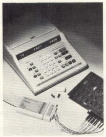
instrument requests the trigger word or address and any following delay, 0 to 65,535 clock-intervals before the data-trace, may be specified. The clip-on probe set plugs into a standard edge connector on the probe. The HP-IB option makes the 1602A totally key-programmable and able to dump its 64-word memory onto the bus on command for analysis by the computing controller. Price is \$1800. Hewlett Packard, 1501 Page Mill Rd., Palo Alto, CA 94304. (415) 493-1501. Circle 164
