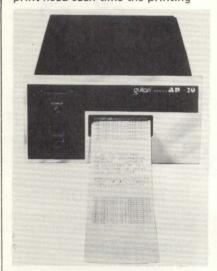
of a dot row is completed. The unit offers a permanent magnet DC stepper motor geared to increment the drive roller. The drive roller and its gearing are the only moving parts in the instrument. Gulton Industries Inc., East Greenwich, RI 02818. (401) 884-6800. Circle 137
