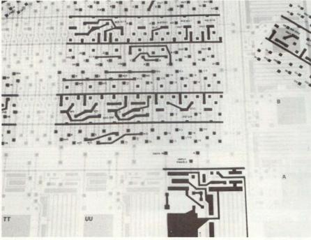
Monochip's function is defined by overlaying transparent patterns that convert the cells into specific logic functions.
