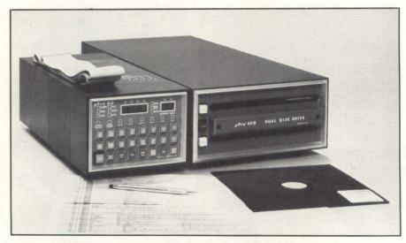
MuPro-80 Microprocessor Development System: This system supports real time emulation of 8080 programs. The control panel on the right hand unit permits the programmer to debug his code without worrying about final system timing problems.
