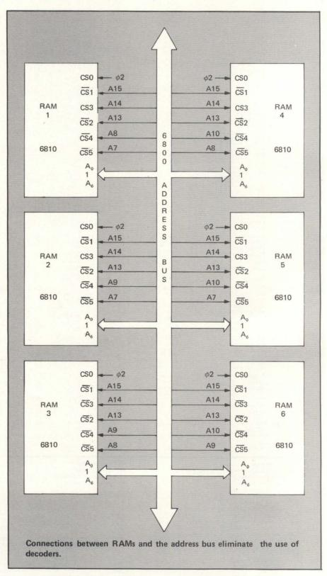
pins for RAM selection optimizes decoding. A RAM selection field n bits long should consist of m O's and (n-m) 1's, where m is the number of negative CS inputs reserved on each IC. The field can be arranged in n!/m!(n-m)!
