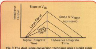
Fig 3 The dual slope conversion technique uses a single clock to govern signal and reference integration periods; thus frequency variations and drift do not affect performance.
