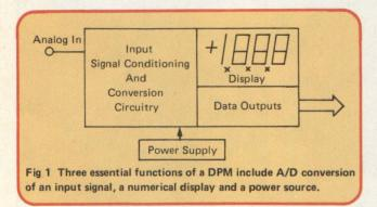
to the user as well, for further use of the digital information. Other interface signals include outputs indicating "polarity", "overrange" and "overload" and input signals including "hold" and "trigger".
