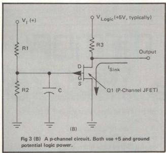
imum low TTL level (6 x 2 x 30 = 360 mV). For applications that need lower ON-resistance, you can parallel a number of FETs with a common divider. Or you can use available n-channel JFETs with an ON-resistance under 5  $\Omega$ . However, most common applications do not supply a negative voltage for sensing.
