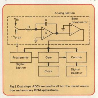
of the input signal over the measurement period is an added benefit resulting from the integration.
