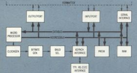
The Tandberg controller/interface is contained on one p.c. board which mounts inside the Recorder. Power is internal from the TDC 3000 built-in power supply. Two interface connectors are provided so that the Recorder can be connected both to a local I/O terminal (such as the Tandberg TDV 2100 Series CRT terminals) and a modem for remote operation.
