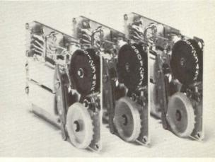
Fig 2 Wheel print mechanism has alphabetic or numeric symbols (up to 20 per wheel) arranged around each wheel's circumference. These printers are generally limited to numeric data applications and other uses requiring less than lps output.
