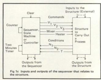
Note that in Figure 1c, there are several inputs to the sequencer. According to their origin, they can be classified as: You can use MSI shift registers to implement sequential circuits. The time for designing, mounting and debugging the circuit is small compared to other techniques – and the cost is about the same as circuits using one D-type bistable per state.
