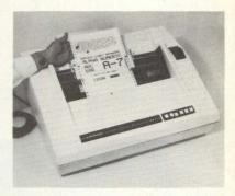
printed on either carbon or carbonless/stock, from 4-7/8" wide to standard printout size, by Dataroyal IPS-7. Print head travels with no wasted motion in this microprocessor controlled bi-directional unit to the next actual printing location. Dataroyal Inc., 235 Main Dunstable Rd., Nashua, NH 03061. (603) 883-4157. Circle 227
