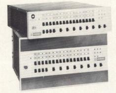
KERONIX IDS - 16 MINICOMPUTERS A 16-Bit Full Parallel Synchronous, High-Speed General Purpose, Mini Computer
