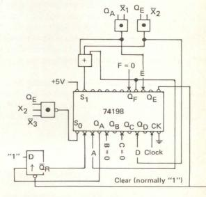
Fig 3b Sample flow diagram and state machine representing typical example of implementing - in a simple and practical way using MSI shift registers - digital sequencers for processes of relative complexity. See the sample problem in the text for equations for the above sequencer.
