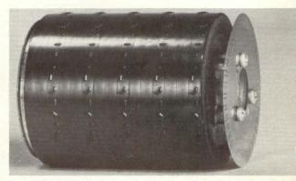
Fig 3 Solid-drum printers can output full alphanumeric data (54character ASCII) by arranging elements of a line (bar) matrix in circumferential rows. The small drum diameter permits high-speed (1.6 lps) and fast start-up (less than 0.5 sec).
