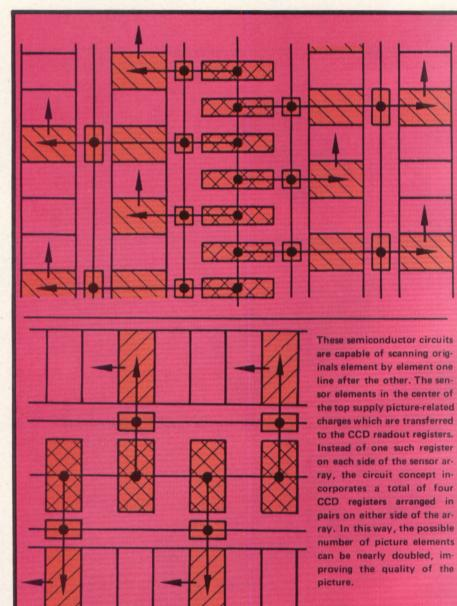
The third step transports all the information towards the output, where the electronic evaluator circuit scans the charge pattern sequentially.
