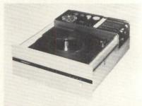
formatted capacities ranging from 14 megabytes in the single-disk version up to 70 megabytes in the three disk model. Each surface has two 350-track/inch cylinders with a recording density of 6000 bits/inch. A sealed enclosure eliminates expensive filters and blowers, yet allows operation in locations previously considered unsuitable for disk drives. Kennedy Co., 540 W. Woodbury Rd., Altadena, CA 91001, (213) 798-0953. Circle 230
