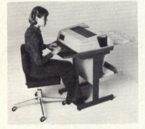
acters/second, uses an internal microprocessor that computes the shortest distance to the next print point. Standard features include switch selectable baud rates from 300 to 9600, parity checking, unattended operation, half or full duplex operation, 1K-byte character buffer and three serial interface connections. Tally Corp., 8301 S. 180th St., Kent, WA 98031. Circle 250
