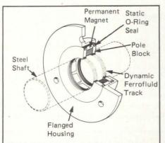
Fig 1 Aluminum casing houses two magnetic field focusing structures separated by a ring magnet. The 0.006 -- 0.007 inch diametral gap between the drive spindle and the focus structure is filled with ferromagnetic fluid. In operation, at speeds up to 6000 rpm, liquid "O" ring Ex-seal keeps helium atmosphere free of contaminants.
