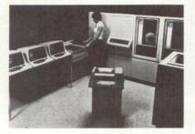
\$250,000 range come from Prime Computer, Inc., The new systems are a completely integrated mix of Prime's hardware, including the new top-of-the-line Prime 500 central processors and business software. The latter includes Prime's advanced Database Management System (DBMS), Multiple Index Access System (MIDAS), Forms Management System (FORMS), ANSI '74 COBOL, and IBM compatible RPG II. Prime Computer Company, Inc., 145 Pennsylvania Ave., Framingham, MA 01701. Circle 257
