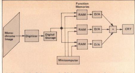
In this pseudocolor display system, the digital storage unit contains the gray-tone image in pixels. Each gray pixel reads from storage then passes through RAM function memories to be transformed into a color pixel. As these digital pixels go through the D/As, they become video signals for the color CRT.
