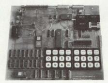
lines, 5 heavy duty relays, and Teletype and audio cassette interfaces. Plus, a 24 pad hexadecimal keyboard and a 9-digit LED hex display. All on one board. There's already an extra 1K of RAM on
