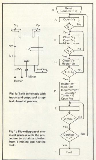
as well. We desire to repeat this process n-times, and so use a counter module-n.
