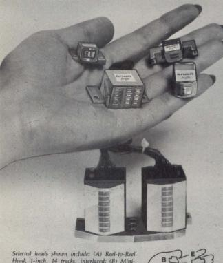
Selected heads shown include: (A) Reel-to-Reel Head, 1-inch, 14 tracks, interlaced; (B) Mini-Cartridge Data Head, full width, read/write; (C) Cartridge Data Head, 4 tracks, read-after-write, selective erase; (D) Credit Card Head, track 2 (ABA) – read; track 3 (thrift) – read narrowi write wide; (E) Cassette Digital Head, 2 tracks, read/write, with integral tape guide.
