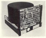
electronics for reading, writing, track selection and timing generation. The non-contact fixed head assembly can access data in an average of 8.5 milliseconds. Digital Development Corp., 8615 Balboa Ave., San Diego, CA 92123, (714) 278-9920. Circle 256
