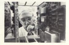
Two magnetic-bubble packages (arrows) store a 24-second "call assist" message in this experimental message unit. Checked out by Bell Labs engineer Jim Rowley, the unit can store eight such messages, one per 2-package board; each package contains four 68,121-bit bubble chips.
