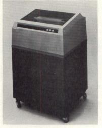
printing is produced by the controlled interaction of a constant speed rotating helix and 22 voice-coilactivated hammers. All printer functions and printed characters are electronically controlled by an integral microprocessor. Tally Corp., 8301 S. 180th St., Kent, WA 98031.
