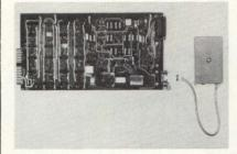
registered and is a direct replacement for the Bell system model 113B. Recent FCC rulings permit the incorporation of the data access arrangement function as an integral part of the modem if tested under FCC rules, Model VA317S enables direct electrical connection of the modem to the telephone network without externally provided telephone company data access arrangement. Unit has analog and digital loopback as well as
