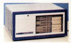
communications facilities 3MBps. It can be configured with up to six remote, full duplex links. Each 5137 channel connection provides addressing for up to 256 concurrent logical application connections between multiple mainframes. Prices range from \$45,000 to \$58,000.
