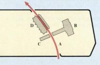
The finer points of forms printing: **A.** Straight paper path. **B.** High power ballistic printhead. **C.** Flat aluminum platen. **D.** High torque tractor feed.
