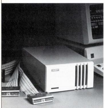
For years designers have been using our Peripheral Automatic Channel Emulator (PACE) to develop and test IBM 370-compatible peripherals quickly and inexpensively without tying up the mainframe.
