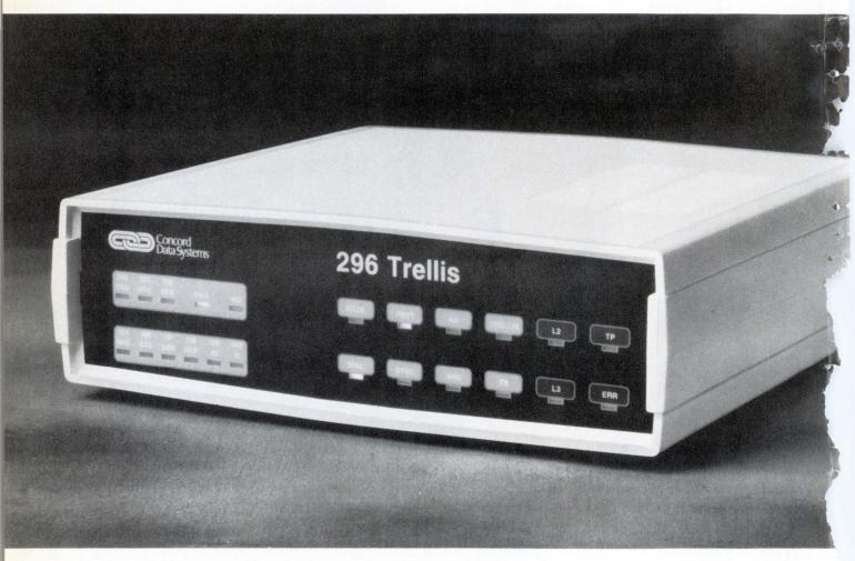
And that means faster data throughput, minimal echo delay, and lower line costs for you. That's the difference between our new V.32-standard  $296^{\text{TM}}$  Trellis modem and all the others. Plus, our new 296 Trellis modem features asynchronous/synchronous operation, MNP<sup>TM</sup> Class-4 error correc-
