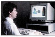
bly modeling capability, a finite element modeler, a design rule processor, materials property management, and a macro language. A Xenix operating system is included. The CP1100 supports C and FORTRAN 77 compilers and Ethernet communications.
