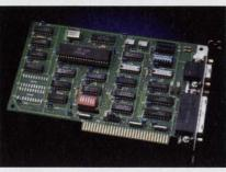
sessions, one of which can be an IBM 3287 printer emulation. ClusterNet connects to the host through an external synchronous modem, at up to 9,600bps, using either leased or switched telephone lines. It consists of a high-speed RS422 serial link and a communication protocol that supports data transmission at 19.2Kbps. ClusterNet also emulates IBM 3777 Remote Job Entry (RJE) functions to send batch jobs to the host, and to receive output directly from the host.
