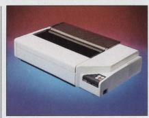
dent serial ports. OTC says any device capable of serial communication, such as computers, printers, and modems, can be connected to the printer and exchange data in RS232C or RS422 formats, at speeds up to 19.2Kbaud. The speed throughput of the printer is 240 lines per minute.
