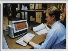
shock-mounted fixed disk storage, a 5¼inch diskette drive, a dual-mode plasma display, full-size detachable keyboard, and an optional expansion unit that can accommodate two full-size expansion slots.
