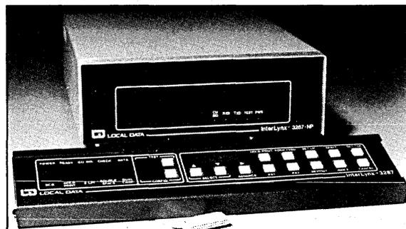
InterLynx/3287 NP is the InterLynx/3287 packaged in a smaller unit with the security of tamper-proof, no panel construction. Options are set by the portable plug-in panel.
