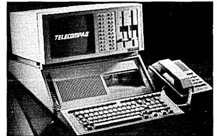
top personal computer. Designed for business managers, the products are available in six models with fixed or flexible disks and connectivity to both analog and digital phone systems.
