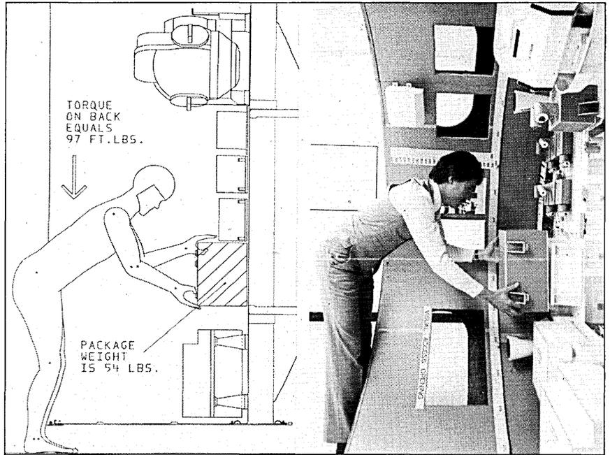
HOW SIMULATION WORKS: The computerized mannequin ADAM shows the strain put on Lockheed human factors engineer Rick Davids' back as he installs an electronics box in a section of the Trident II D-5 Fleet Ballistic Missile.
