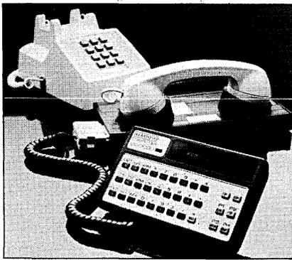
mode. The unit has an 80-character buffer and a 16-character scrolling LED display; users can enter messages into the buffer, review and edit the message, and then transmit the buffer to a remote computer. The LK-3000 with communications module (LK-2010) and acoustic coupler sells for \$525. NIXDORF COMPUTER PERSONAL SYSTEMS, INC., Burlington, Mass.
