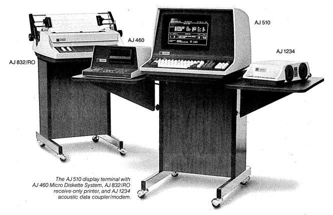
The AJ 510, the most versatile CRT terminal in its class, excels at interactive timesharing and a lot of other jobs. And with the addition of these supporting AJ products, you can greatly expand your application flexibility.
