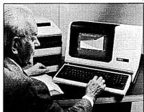
architecture are possible; by bringing up the RT-11 operating system, users can have their MiniMINC function as a network node, or communicate with other machines using 2780 or 3780 protocols. MiniMINC sells for \$9,900. DIGITAL EQUIPMENT CORP., Maynard, Mass.
