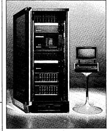
NETWORK CONTROLLER operates through a crt/keyboard terminal such as the Dataspeed 40/2 providing user of a large data communications system full diagnostic management of all Dataphone uservice data in the network.
