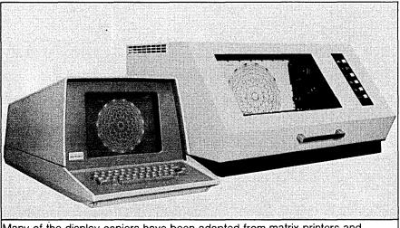
Many of the display copiers have been adapted from matrix printers and printer/plotters, like this model which Trilog adapts from a Printronix impact line printer.
