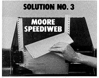
Permits immediate removal of last printed formset with no waste, while margins remain in tractors to advance next one. Individual parts of the formset can be separated at any time after removal from the printer. An audit copy can be provided if desired. Available 3½" to 11" deep and 11" to 16" wide.
