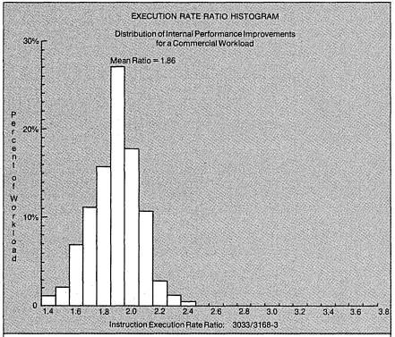
Fig. 8. According to a cycle by cycle simulation, the 3033 will run anywhere from 1.4 to 2.4 times as fast on a commercial workload as a 370/168-3 with the fast multiply feature.
