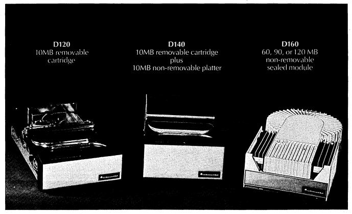
For OEMs and system builders, the D100 family of compact disk drives offers a surprising list of advantages. Two new models, D140 and D160 add capacity and flexibility to the proven performance of the D120. The D140 includes a 10MB fixed platter in addition to the 10MB removable cartridge as used with the D120. The D160 uses a sealed (non-removable) module which includes low pressure heads and carriage.
