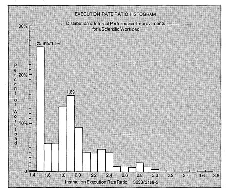
Fig. 9. On scientific workloads, the 3033 again appears to be just under 1.9 times as fast as a 168-3 with the high speed multiply feature. Some optimized FORTRAN execution steps are very well suited to the 168, however, and the 33 can manage only 1.5 times the instruction execution rate for those.
