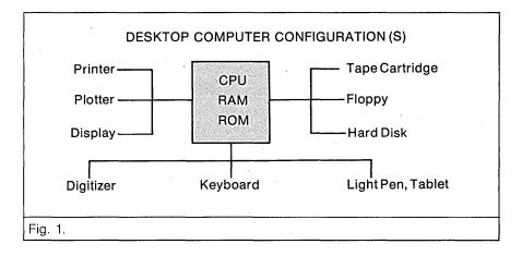
maximum of 64K bytes of RAM. A light pen is optional, as are a disk and printer system. ISC's color display systems have become very popular in process control applications where it is important to have color.
