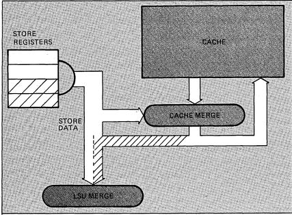
Fig. 3. On the 3168, when the data to be stored was less than a full 8-byte doubleword, the new data had to be merged with the old twice: once for main storage and once for cache. On the 3033, only one merge is necessary when the data is in the cache; the results of that operation are simply stored twice.
