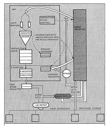
Fig. 2A. The 3168 processor has four basic elements: Instruction Pre-Processing Function (IPPF), Execution Function (E-Function), Processor Storage Control Function (PSCF), and processor storage (main memory). Buffers, registers, cache, and interleaving all are appropriate to the processor's speed.
