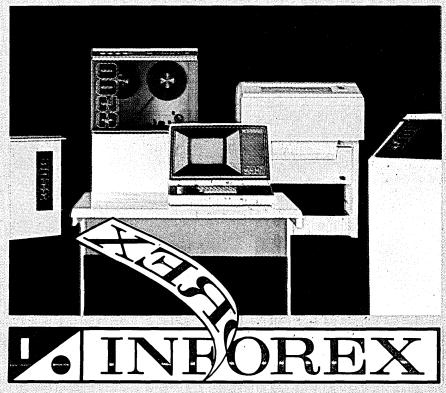
Two data entry systems designed for centralized or de-centralized high speed key-to-disc entry.
