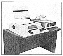
For applications requiring fully-formed characters, the model 4000B uses a daisywheel print mechanism. The 45cps terminal has an 8080A microprocessor in its controller, and can handle ASCII, ECBD, or correspondence codes. A 14-key numeric pad is standard. Peripherals, including the vendor's model 500 floppy disk, optionally can be added to the model 4000B. The basic terminal is priced at \$4,395. FOR DATA CIRCLE 434 ON READER CARD
