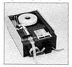
speeds are independent of each other. The dual-ported RS232 peripheral includes a 4KB buffer, automatic diagnostics, full- or half-duplex operation, and editing and duplication functions. Optional plug-in boards allow addition of more buffer memory or code conversion capabilities. The SRP-750 sells for \$2,695.
