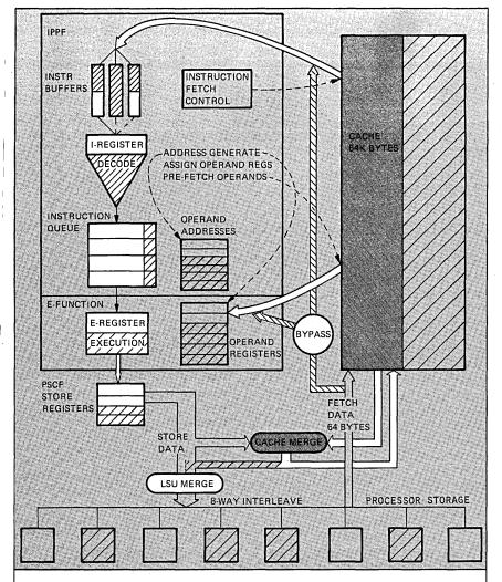
Fig. 2B. Changing the speed forces changes in the other elements as well, including adding to or lengthening buffers, registers, and cache for the 3033 (shown with crosshatching). Changes in instructions led to others in decoding and instruction execution as well.
