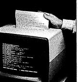
Try this on your favorite CRT! With the 2621P, you just hit a key and in seconds you have hard copy of your CRT display. The built-in thermal printer prints upper and lower case at up to 120 cps.
