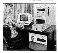
mini diskettes. An automatic stacker/loader holds up to 50 diskettes; diskettes, fed one at a time, can be tested, initialized, and then loaded with data for subsequent mass distribution. Diskettes failing the test phase are ejected into a reject hopper. The Floppy Copy is said to handle all IBM formats, as well as most other formats; formats supported include single and double density and one or two sided drives. Both
