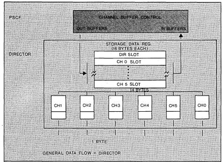
Fig. 7. The channels are handled in a multiprogrammed manner by a microprogram within each director, with the block and byte multiplexor channels being handled by different subprograms. The path width from storage to channels is 8 bytes, from channels to storage 4 bytes, from the director's registers to channels 4 bytes, and those to the outside world are 1 byte (although the first block multiplexor of any group may have a 2-byte wide path).
