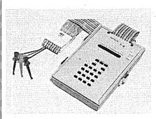
machine cycle prior to a breakpoint halt. The portable T-8 connects to the microcomputer via a 40 pin chip clip; interfaces allow connection to 8080, Z80, 2650, 6501, 6502, 8060, and 8085 based processors. The T-8 sells for \$695, quantity one; each interface is \$50. PAUTUCK INC., Pennsauken, N.J.
