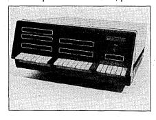
\$1,145 (quantity one) sans memory, consists of a 4MHZ Z80A cpu board with room for on-board ROM, 25 amp power supply, 22-slot shielded motherboard, forced fan ventilation, and removable front panel. Static memory can be had in 8kB increments for \$165 (450nsec cycle time) or \$195 (250nsec cycle).
