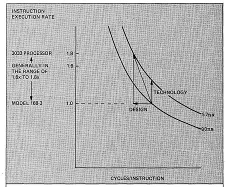
Fig. 1. A processor's internal performance is a funciton of technology and machine design. Thus the performance improvement of the 3033 over that of the 3168 is due partially to technology (reduing the cycle time from 80nsec to 57nsec leads to an increase in instruction execution rate of about 40%) and partially to design improvements which act to reduce the number of cycles per instruction.
