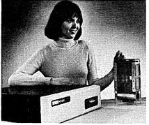
point processor chip for the LSI-11/23; depending on configuration, the new microcomputers are anywhere from two to five times faster than existing LSI-11 products. The PDP-11/23 is a packaged version of the two-board LSI-11/23.
