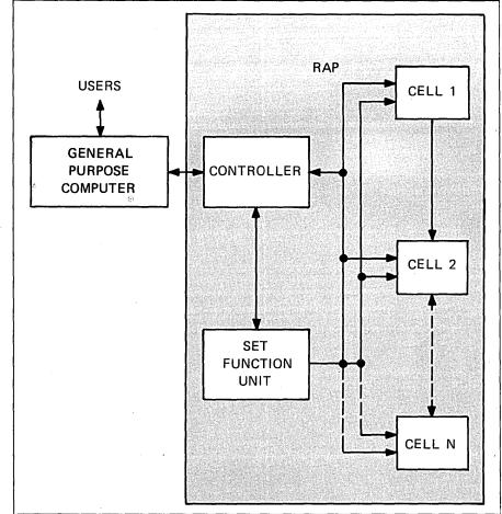
Fig. 3. RAP (Relational Associative Processor) originally was built for a relational data base system, as its name implies, but can be used in other environments as well. Its associative store (cells *1* through *N* above) is read into a buffer from disk, with mark bits set for those records selected. Records are altered as required while in the buffer, and set functions (summations, etc.) are performed before the data is transmitted to the host.
