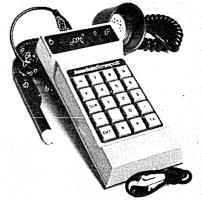
(Mod-10, Mod-11, or none). Units are offered to read several bar codes, including Codabar, UPC, and Plessey. Users can scan through memory a line at a time or search for specific product codes or partial product codes. Pricing on the Scorepak starts at less than \$1,000. AZURDATA, INC., Richland, Wash.
