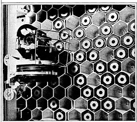
AROUND THE WORLD mass storage systems are going into more shops and at an accelerating rate, although none of the hardware vendors seems to be emphasizing it to any great extent. This is photo of the IBM cartridge storage device that IBM introduced with its 3850 mass storage system in the fall of 1974.
