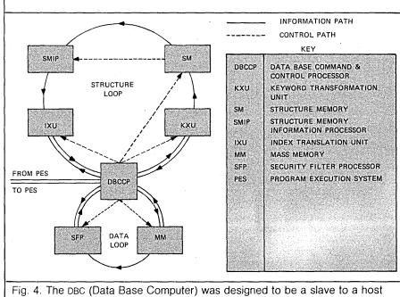
Fig. 4. The DBC (Data Base Computer) was designed to be a slave to a host cpu. It employs microprocessors for each disk track on a cylinder (one for each read head) so an entire memory may be read in parallel, and a pipeline processor architecture so that many processes may be performed on data simultaneously. A more realistic approach would be to consider not what users need, but what they will need—including distributed data bases.
