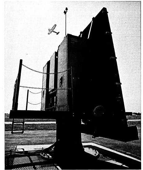
Prototype model of ITT Gilfillan PAR-80 phased array radar, which guides an aircraft through 20 miles of approach to a precise touchdown. Computer simulation played a major role in its design.
