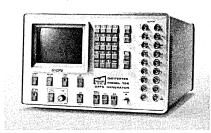
play in these formats. The unit can treat the data as either 16K bits in series or as 1K of 16-bit words. The unit outputs TTL levels at any of 15 preselected crystal-controled data rates; external clocking and a variable frequency mode (ranging from 30Hz to 20MHz) can also be used. The 725 sells for \$5,500. MOXON, INC., Irvine, Calif.
