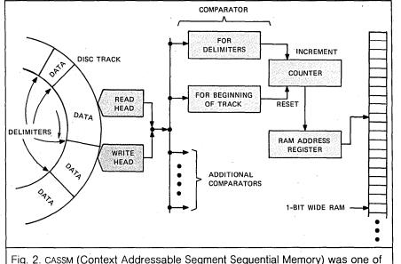
Fig. 2. CASSM (Context Addressable Segment Sequential Memory) was one of the first approaches to a data base processor. Each head on a head per track disk has sufficient logic to test the items recorded on its track, making it possible to search the entire disk in a single rotation, setting the appropriate bit in the RAM for those which meet search criteria.
