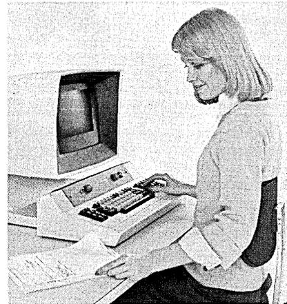
available with a numeric pad. Operators can enter, verify, correct, and update data, with communication to the host 5400 taking place in dial-up half-of full-duplex mode. A flashing cursor and audio/visual error indicator are additional features of the 5441, which displays information in 12 line by 40 character format. It leases for \$95/month and sells for \$3,735. CUMMINS-ALLISON CORP., Data Systems Div., Glenview, Ill.
