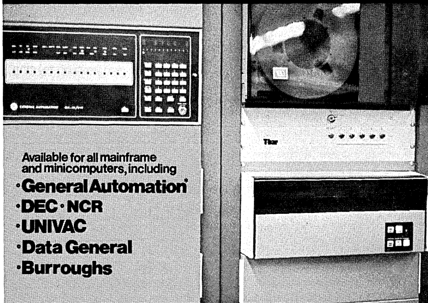
*Photograph illustrates mag tape and disk being T-BAR switched between GA-16/440, General Automation miniprocessors
