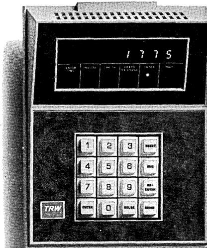
*Entry and response.* The simplest Digidata format—on the left—handles data entry, inquiry/response, and update of central files. Three response lights can be custom labelled for any application you need. In the more complex Digidata terminals, four or eight digits move from right to left, always displaying the last digits entered. They display numeric responses as well as status.
