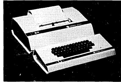
at switch-selectable speeds from 75 to 2400 baud, yielding 240-cps rates across 80 columns of friction-fed paper. The 200 recognizes the entire 128 character set of ASCII and prints 96 of them (upper and lower case) in 7x9 dot-matrix patterns. Standard features include a paper out signal and audio alarm, adjustable margin, print density control, and push-button paper advance.
