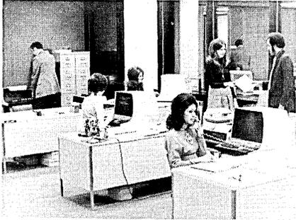
unit, showing eight lines of 80 characters, with a second model doubling the number of lines. The terminals are offered with either 64 or 96 ASCII character sets and have cursor controls as standard features, with editing functions optional. Transmission to host computers is performed at a choice of 2000, 2400, or 4800 baud. A configuration of one controller, five displays,
