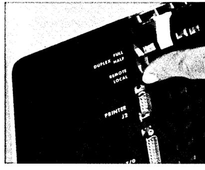
Field selection of modes, data rates, stop bits, parity, auto roll-up and line feed, display or non-display of cursor and carriage return symbol are easily made with back panel switches and jumper wires located on printed circuit boards.
