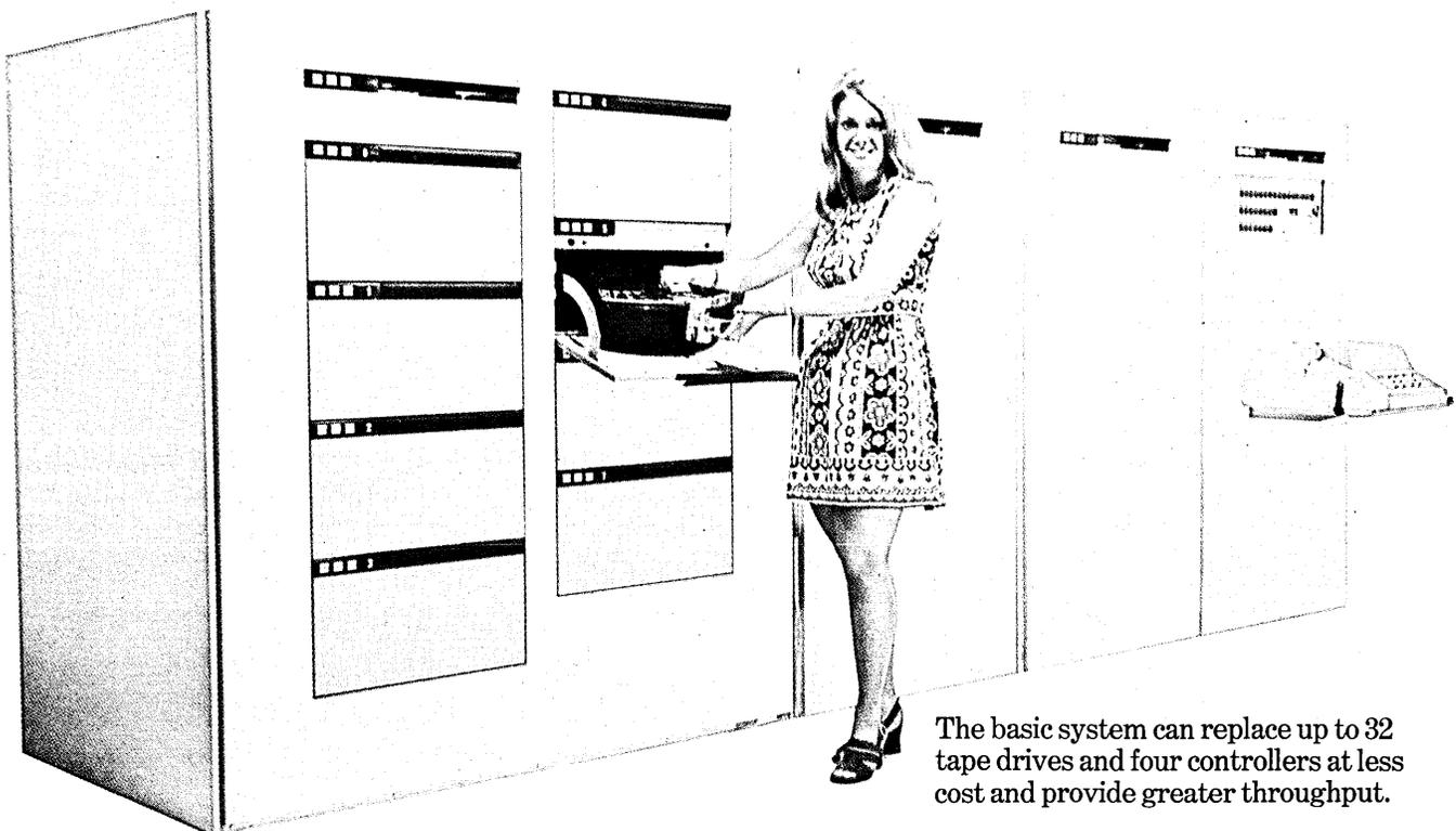
The basic system can replace up to 32 tape drives and four controllers at less cost and provide greater throughput.
