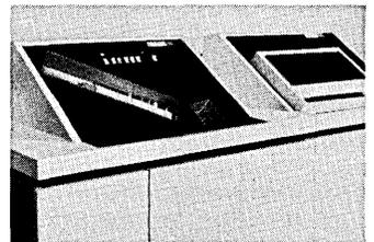
**Model 2310 Batch Reading System** is a high-speed data collection center. Reads 400 encoded tags per minute, feeds automatically, requires no tag orientation, records data on computer-compatible magnetic tape.
