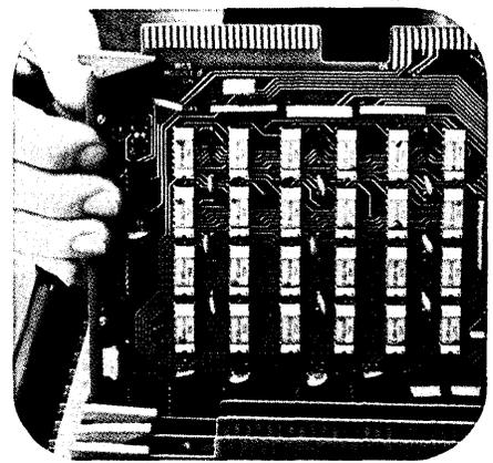
**THE COMPUTER WITHIN A COMPUTER:** A plug-in card lets you microprogram, to speed up subroutine execution of important applications. Frees valuable memory space for added problem-solving capacity.
