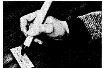
**Model 2243 Bar Code Scanner** comprises a hand-held light pen and logic for encoding the CODABAR code with an interface. Data is checked seven times in the logic to assure accuracy before being released to the interface and entered at point of sale.
