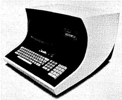
capability as an option, made possible by a screen resolution of approximately 12,000 elements. Also optional are a 30-cps printer, and a 2400-baud cassette recorder. Prices for the crt start at \$2430. Delivery is currently 45 days.
