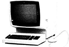
The 3270 Information Display System can be attached to the System/3 Model 10 for local and remote inquiry and data entry. When System/3 is linked to a larger system, information can be exchanged and subsequently displayed by either system.
