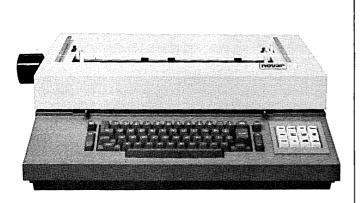
This is the new Novar 5-40 MOD II for use in on-line polling and addressing systems. It has both software and communication compatibility with 360's and 370's, and it can transmit and receive at rates up to 2400 baud.
