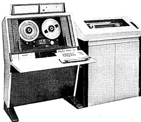
an effective rate of 3600 Baud over the dial-up network to the central computer facility, and, after processing, returned at the same efficient, cost saving rate for off-line report generation at 600 lines per minute.
