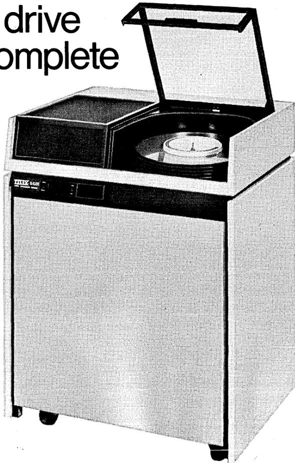
The new TELEX 5600 Disk Storage System doubles the storage capacity of present IBM 2314-type systems. The 58 million bytes per drive capacity is provided by doubling the number of cylinders, while maintaining track and format compatibility. The TELEX 5600 Controller accepts one to eight active drives plus a spare, for a total subsystem capacity of 466 million bytes.
