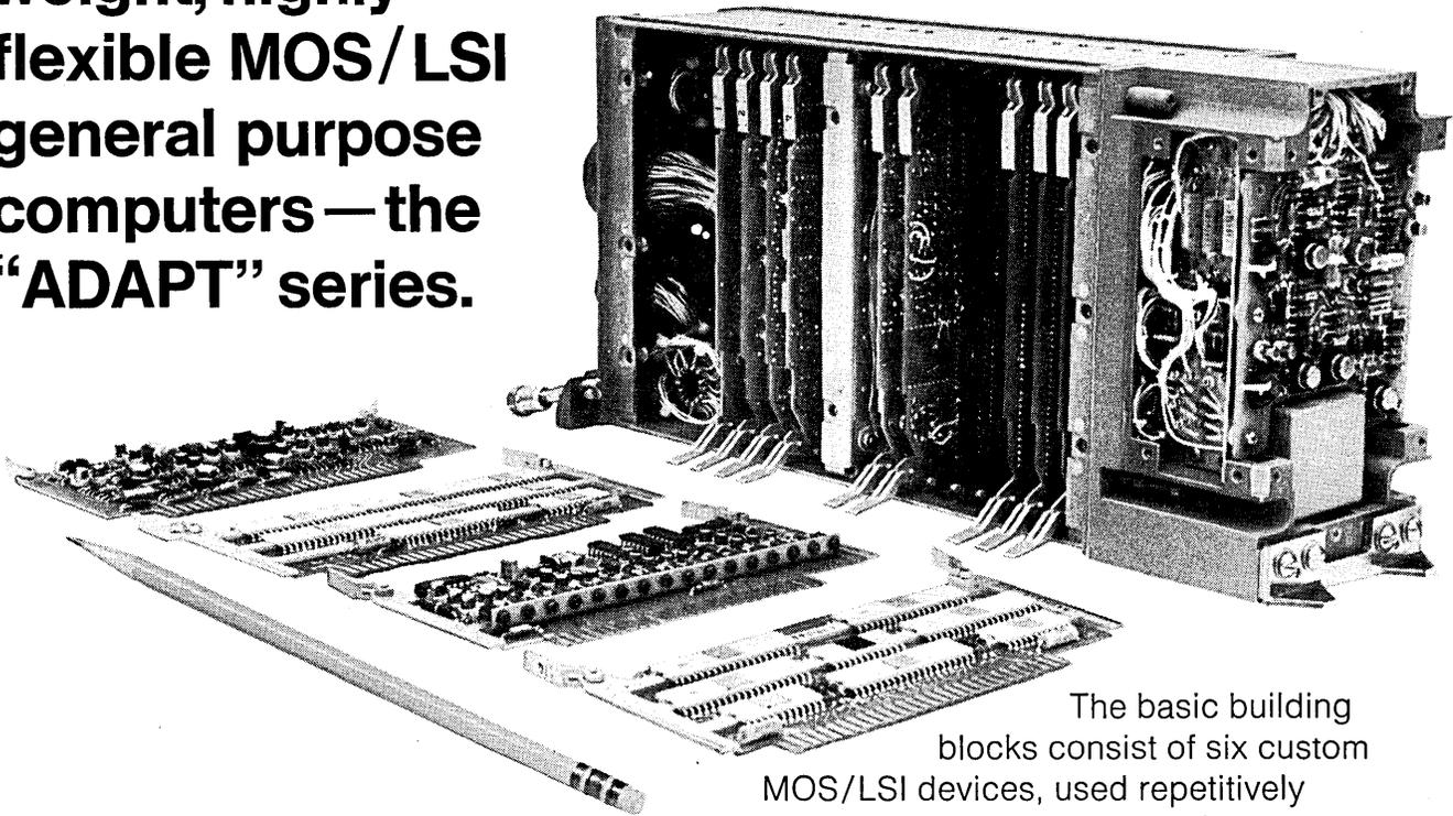
The basic building blocks consist of six custom MOS/LSI devices, used repetitively to tailor a task-oriented processor for your application with a minimum of non-recurring cost.
