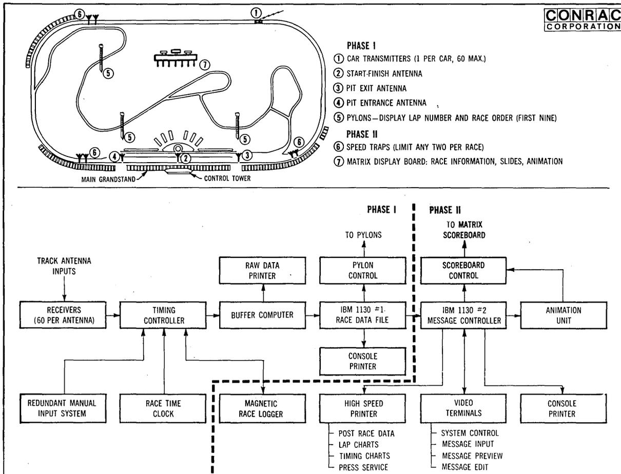
Fig. 2. Computer system overview, Ontario Motor Speedway (courtesy of Conrac Corp.).
